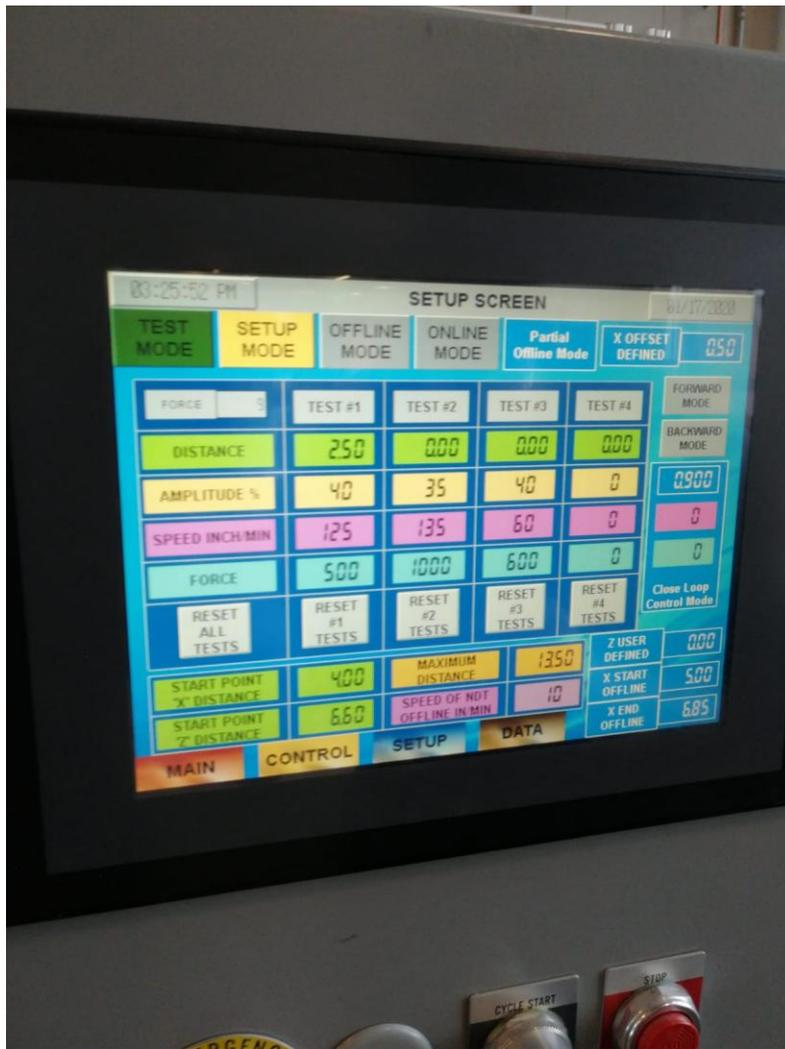
Figure 31: Welding parameters, UAM machine display
