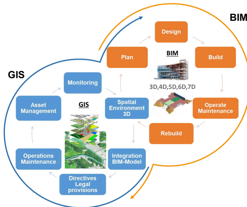
Figure 7. BIM and GIS authoring Systems interacting in infrastructure lifecycle (DR.A.Carstens, 2019).
