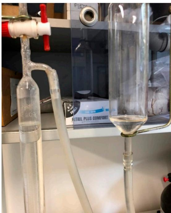
Figura 2.28 Liquid level in the calcimeter
