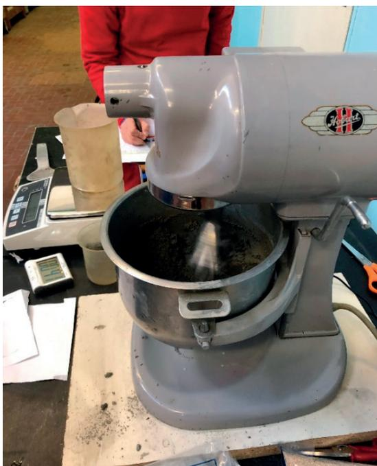
Figura 2.8 Mixer and blade in the laboratory
