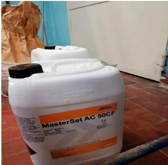
Figura 2.47 Hardener additive MasterSet AC 50CF (BASF)
