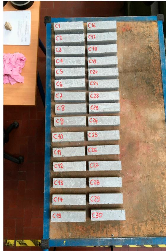
Figura 2.66 Hardened C-Fiber samples
