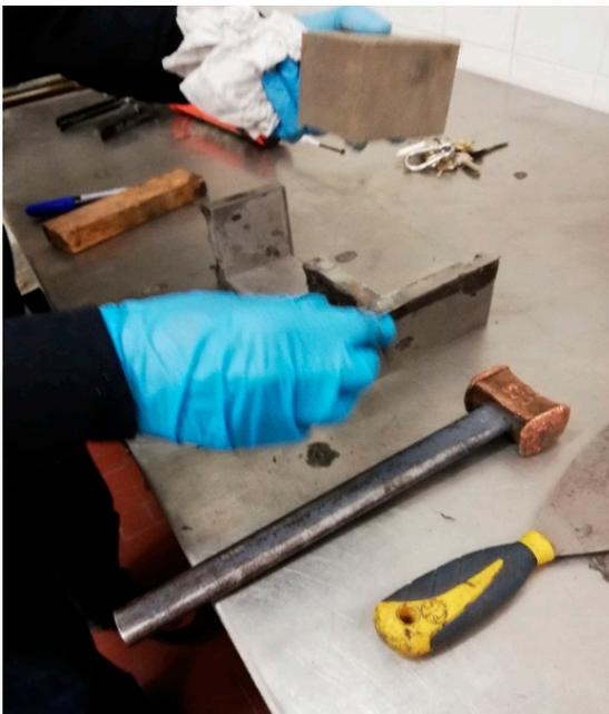
Figura 2.57 Specimen removal from the mold
