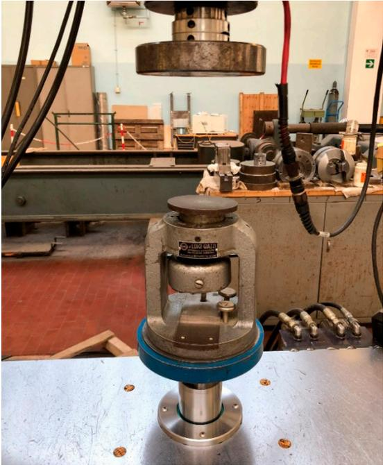
Figura 2.21 Compressive strength machine
