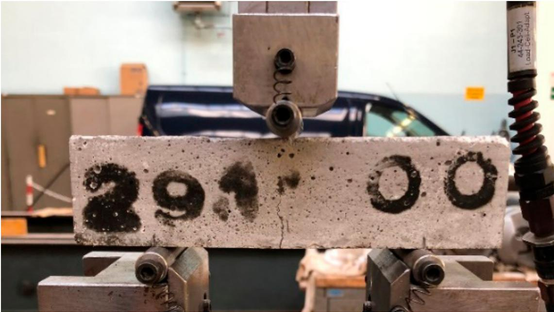
Figura 2.18 Sample in the bending machine
