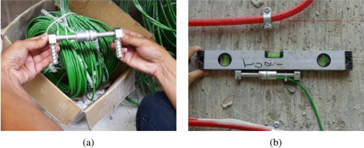
Figure 4.8: Strain gauges installation (Baralis and Barla, 2019)
