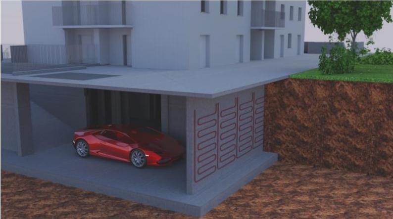
Figure 4.1: Render of the GeothermSkin energy system applied to a residential building basement (Baralis and Barla, 2019)
