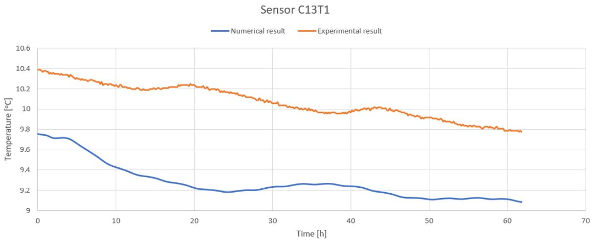
Figure 5.19: Comparison of soil temperature between two method at sensor C13T1
