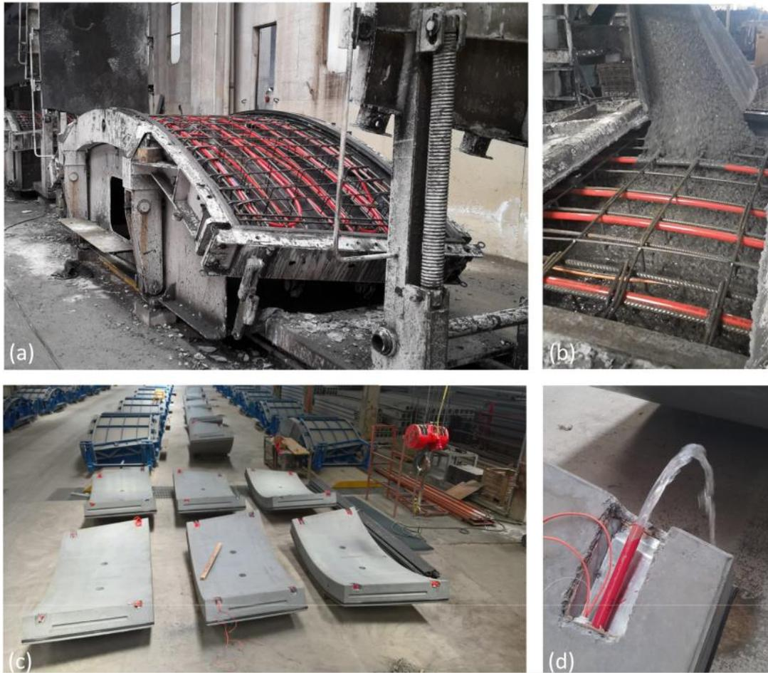
Figure 3.7: Preparation stages of energy segments: (a) moulding, (b) casting, (c) demoulding and (d) circulation test (Barla et al., 2019)
