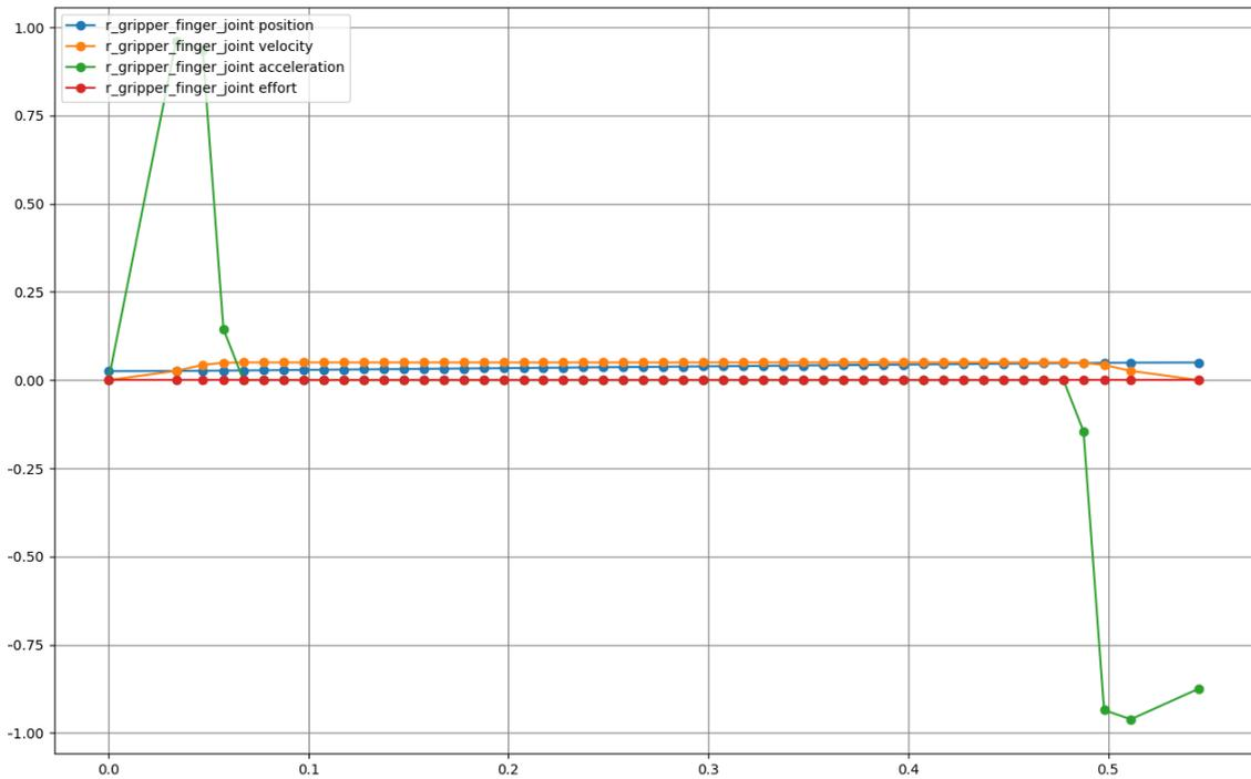
(d) Trajectory of the gripper left finger joint during placing
