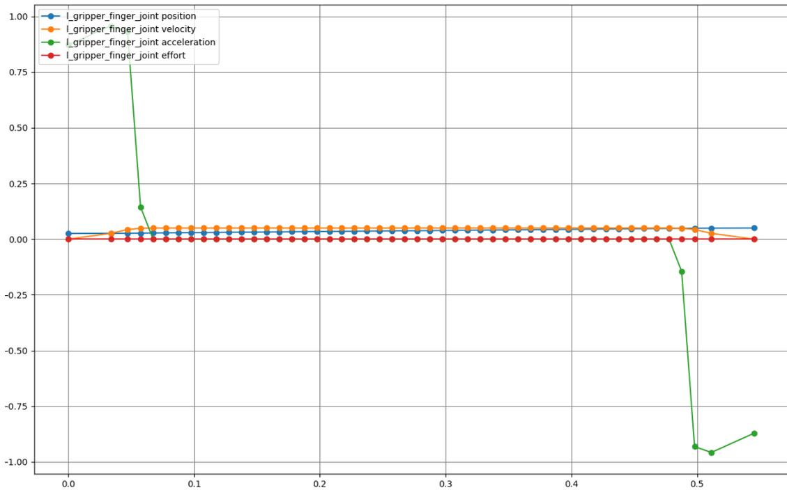
(c) Trajectory of the gripper left finger joint during placing
