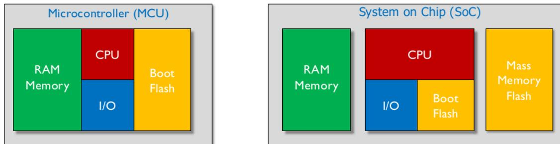
**Figure 1.2:** Schematic comparison between microcontroller and system-on-chip [source: slides of PoliTo Model-Based Software Design course by Massimo Violante]
