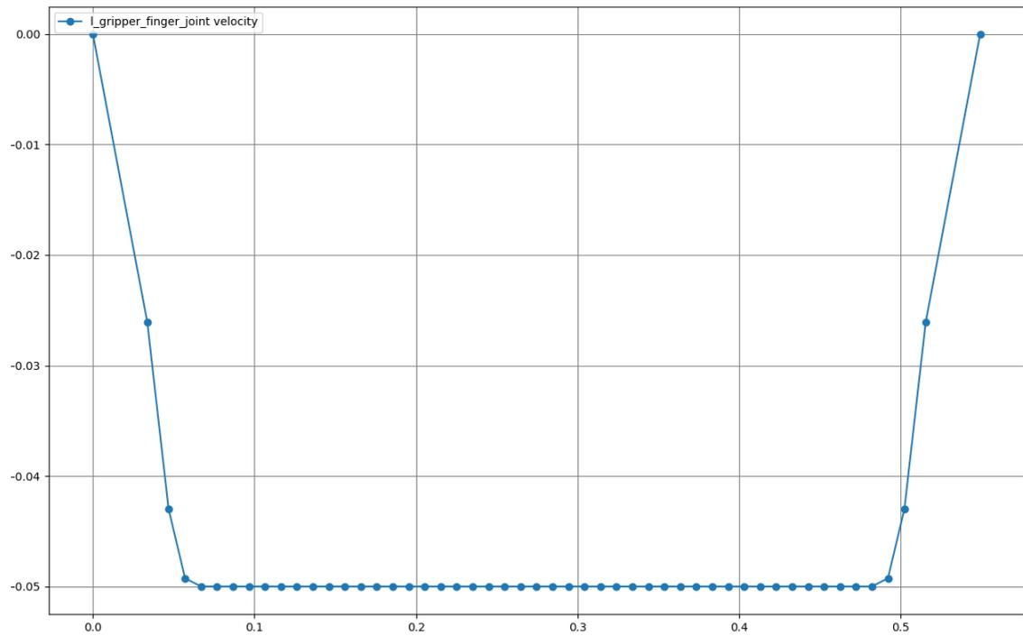
(b) Velocity for the gripper left finger during picking
