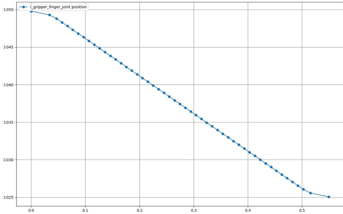
(a) Position for the gripper left finger during picking
