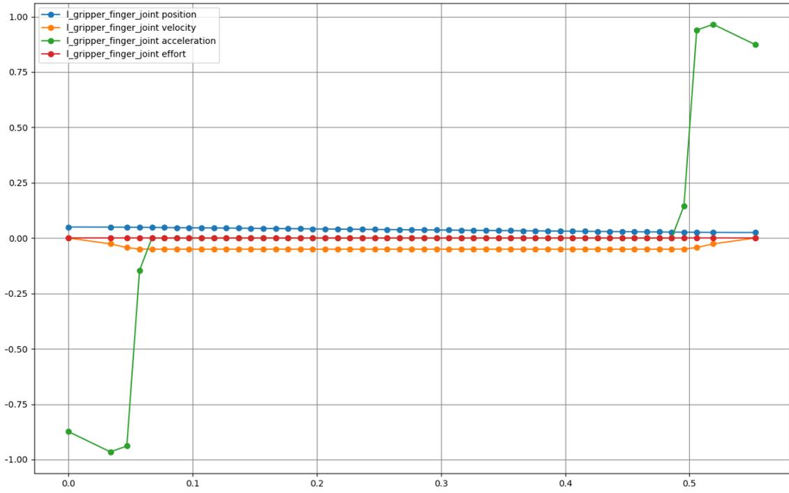
(a) Trajectory of the gripper left finger joint during picking
