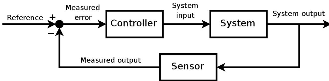
**Figure 1.1:** Closed loop (feedback) control block scheme
