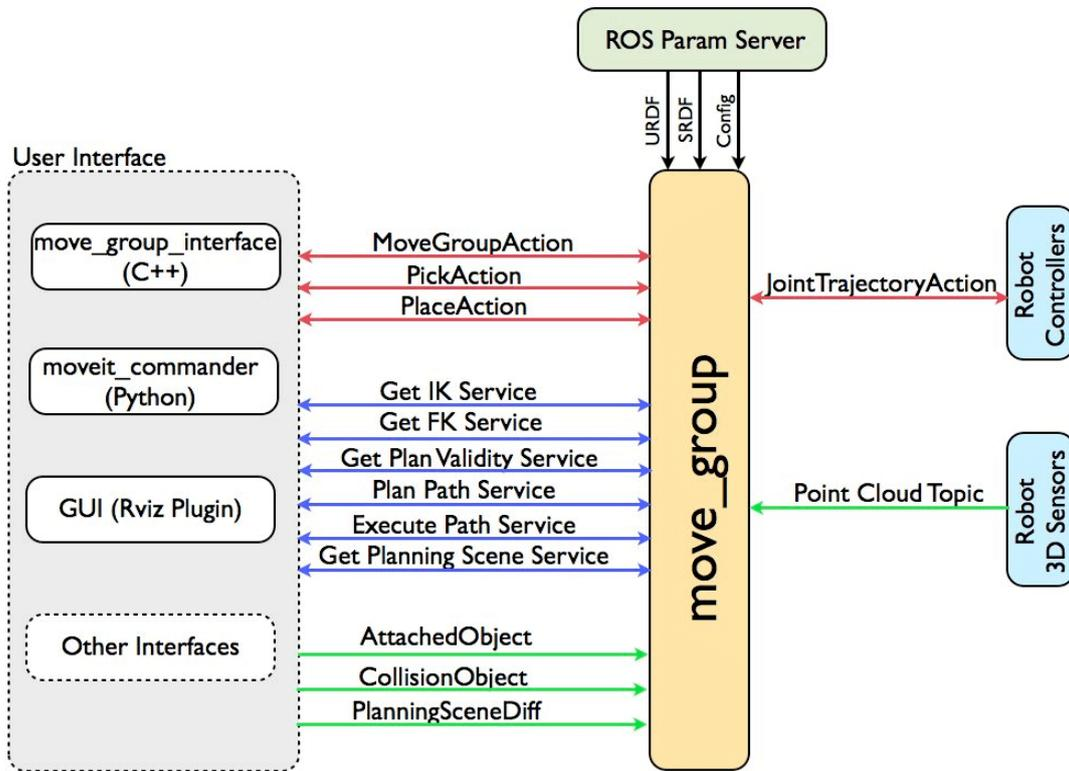
**Figure 6.2:** High level system architecture diagram of the MoveIt *move\_group* node [credits: moveit.ros.org]
