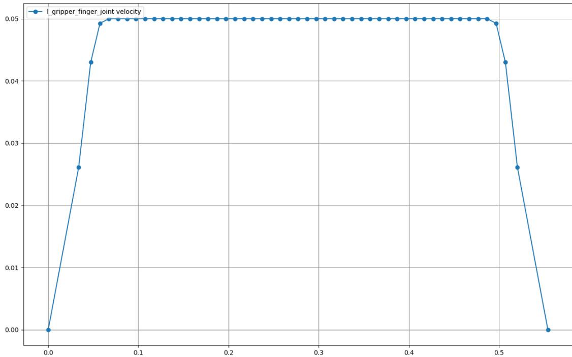
(d) Velocity for the gripper left finger during placing
