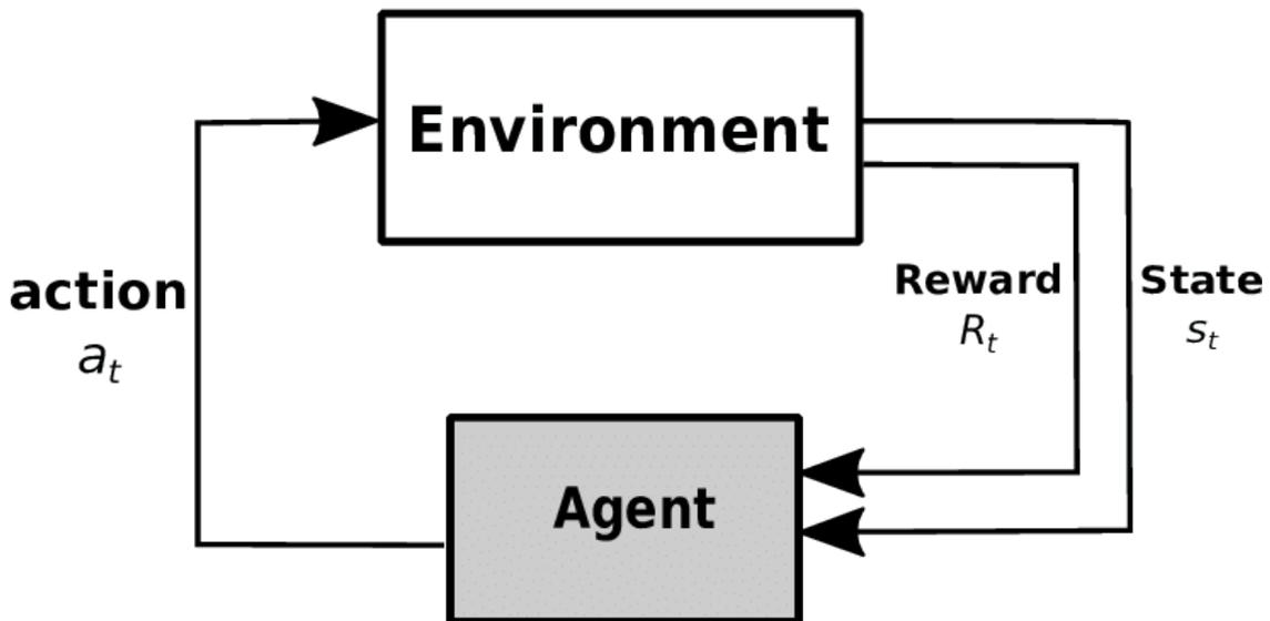
**Figure 8.2:** Reinforcement learning general block diagram
