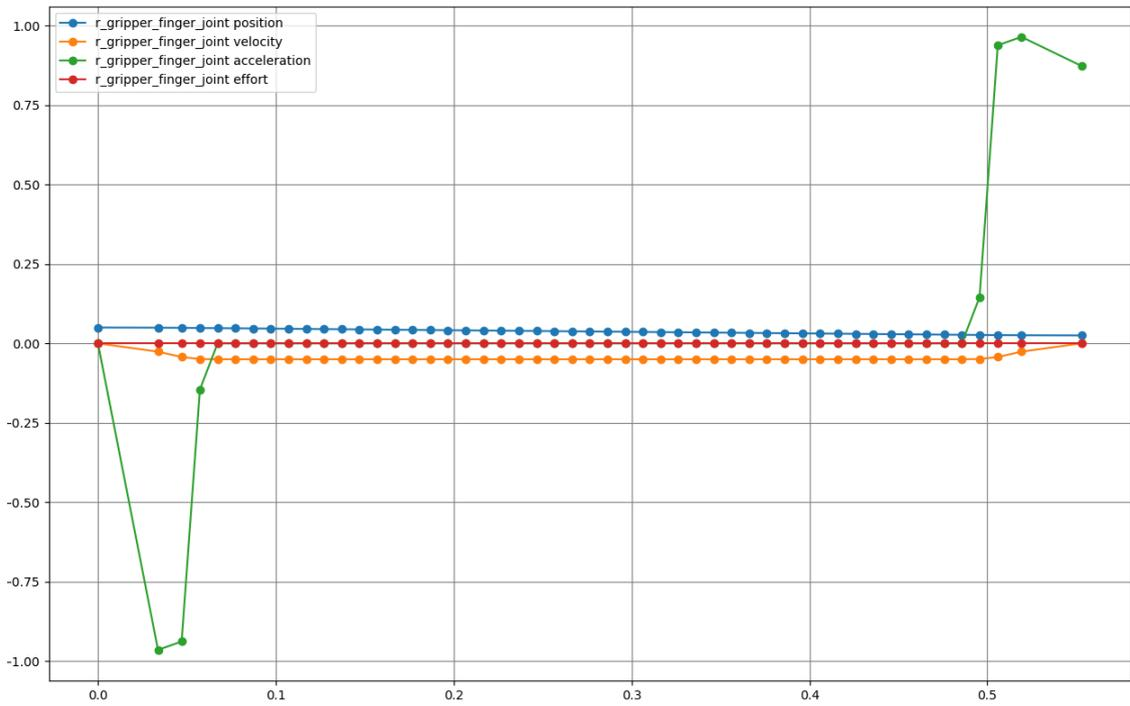
(b) Trajectory of the gripper right finger joint during picking
