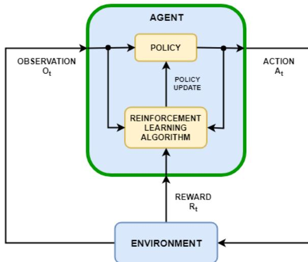
**Figure 9.1:** Key elements of a Reinforcement Learning problem
