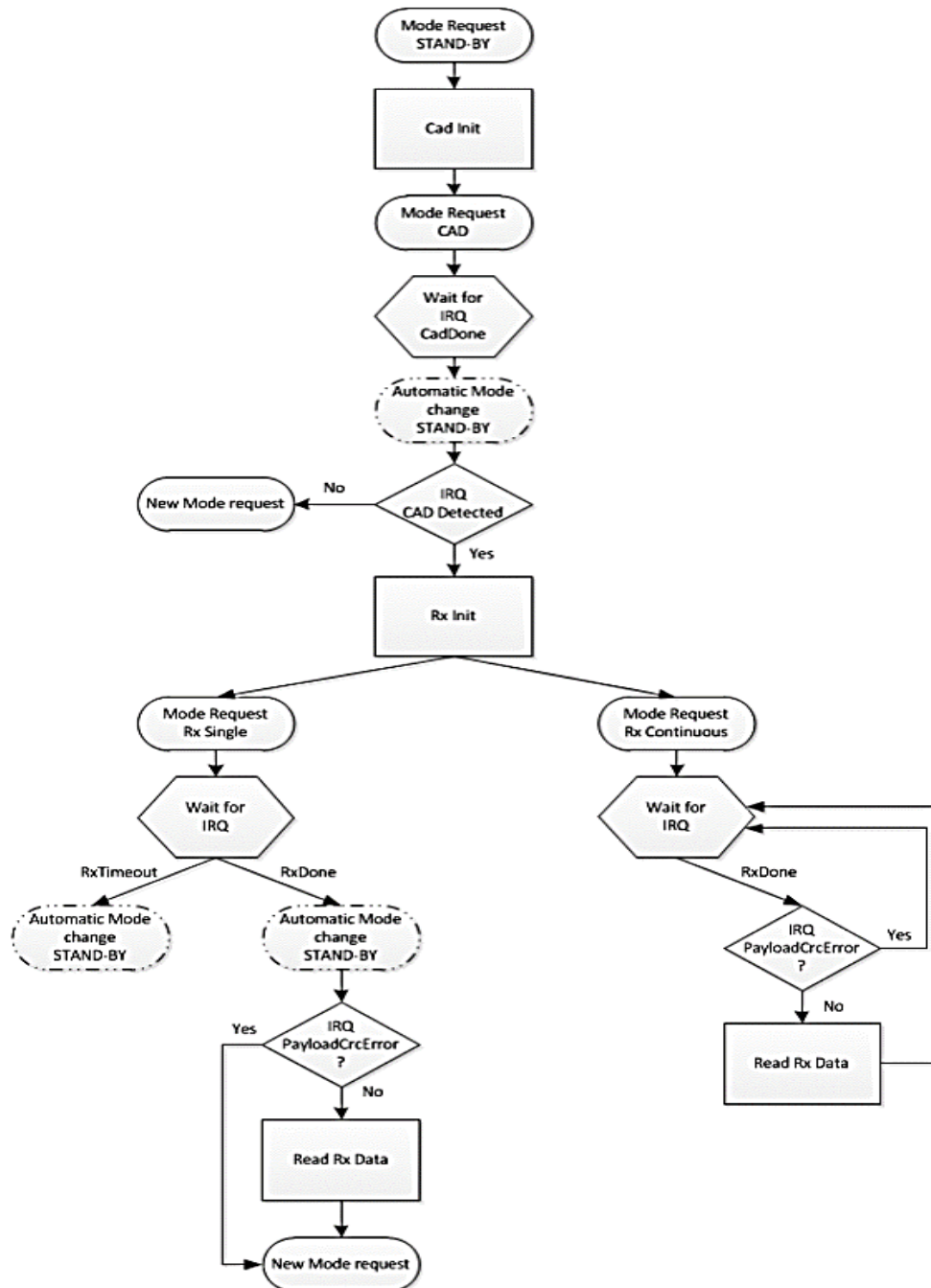
Figure 2.19: LoRa CAD flow [21]
