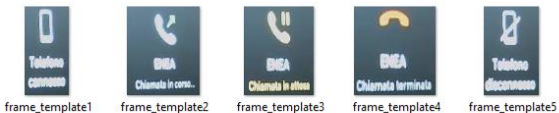
Figure 34: Template images used for comparisons by the image recognition software
