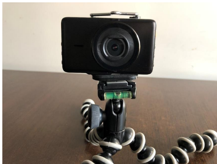
Figure 12: The camera used for the project has a maximum resolution of 720p and 30fps
