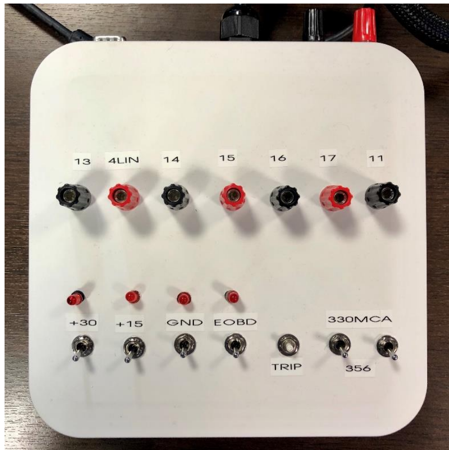
Figure 8: Home-made Breakout Box used to interface the CANcaseXL with the Instrument Panel Cluster (IPC)
