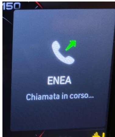
Figure 38: Second popup. It simulates the outgoing call to the user "Enea". InfoCode = 010101. It consists of two frames
