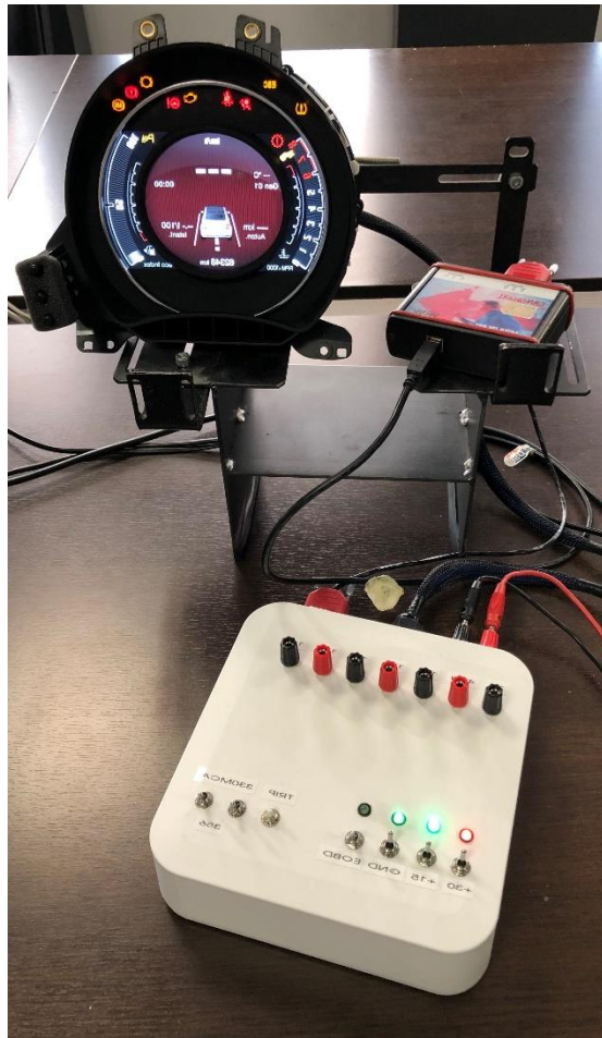
Figure 11: System composed of IPC, Breakout box, CANcaseXL
