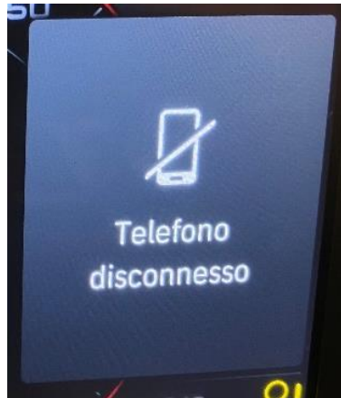
Figure 41: Fifth popup. It simulates the disconnection of the mobile phone to the infotainment services of the vehicle. InfoCode = 011000. It consists of a single frame
