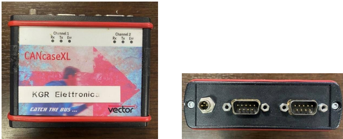
Figure 9: The hardware used to interface the Electronic Control Units simulated through the CANalyzer software, with the Instrument Panel Cluster (IPC)
