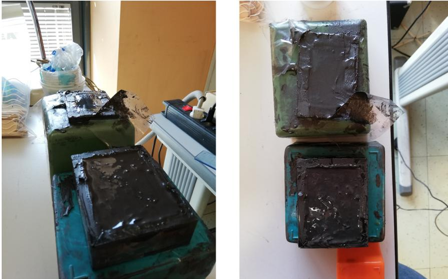
Figure 5.4: Mixture of urethane rubber and graphite powder on the mould
