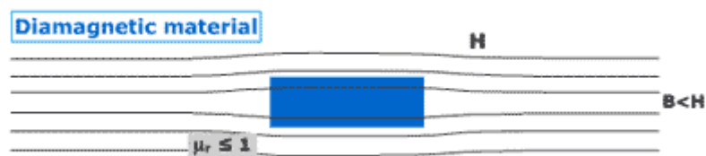
Figure 17: Field lines distribution of diamagnetic materials placed in a uniform magnetic field H 6
