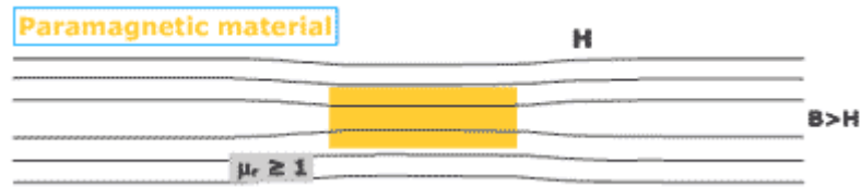
Figure 18: Field lines distribution of paramagnetic materials placed in a uniform magnetic field H 6
