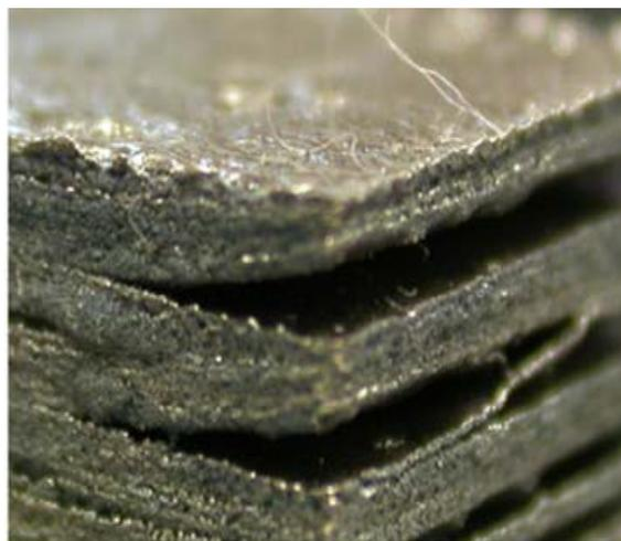
Figure 1.9: Example of Delamination [8],[16]
