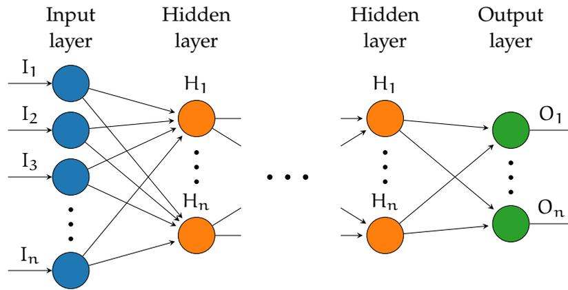
Figure 3.7: Feedforward neural network
