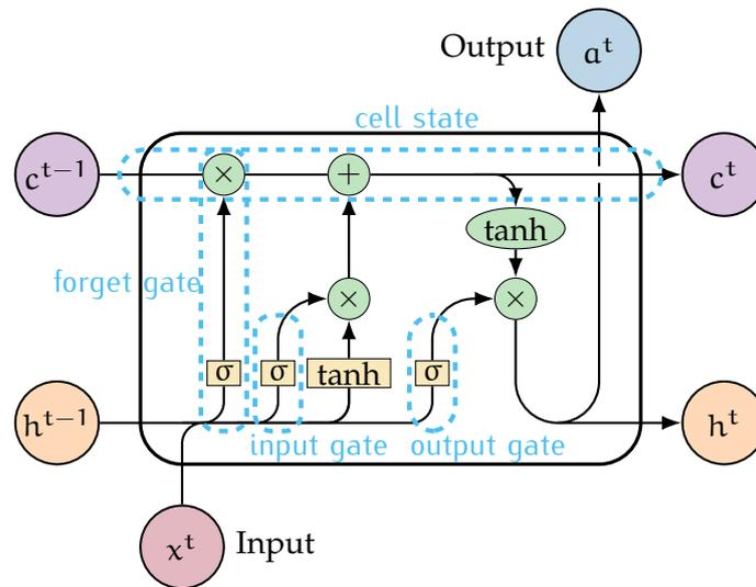
**Figure 3.11:** LSTM cell diagram. A *cell state*  $c^t$  contains information of the dependencies among elements in the input sequence; a *forget gate* decides what information should be kept or forgotten; an *input gate* decides which information is passed to the cell; and an *output gate* decides what the next hidden state  $h^t$  should be.
