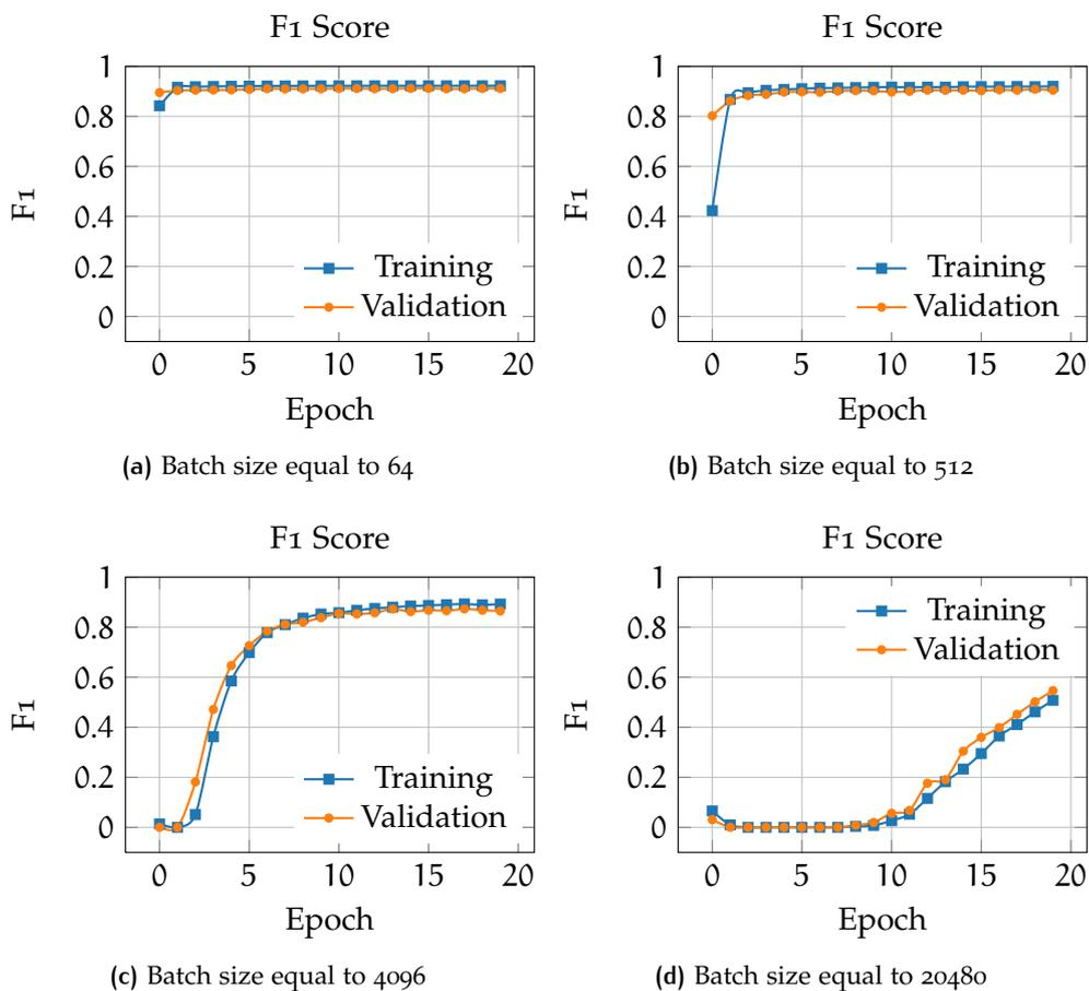
Figure 5.5: F1 score over epochs for different batch sizes. The higher the batch size, the higher the amount of epochs required to reach a convergence.
