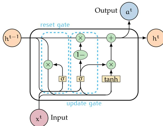
Figure 3.10: GRU cell diagram. An *update gate* decides which information of  $h^t$  is passed to the next cell, while a *reset gate* decides how much past information to forget.
