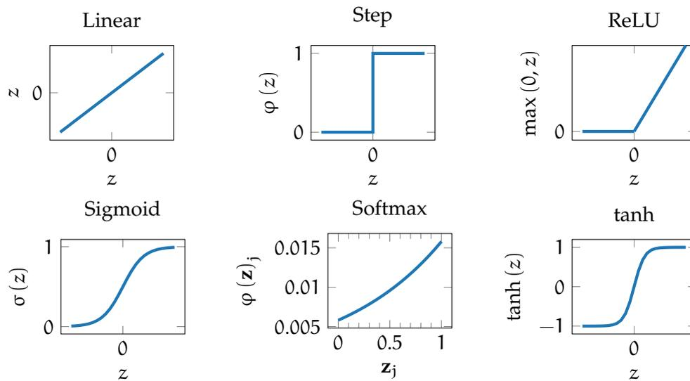
Figure 3.4: Common activation functions in neural networks. Softmax example is relative to a vector  $\mathbf{z}$  made of 100 equidistant elements in range  $[0, 1]$ .
