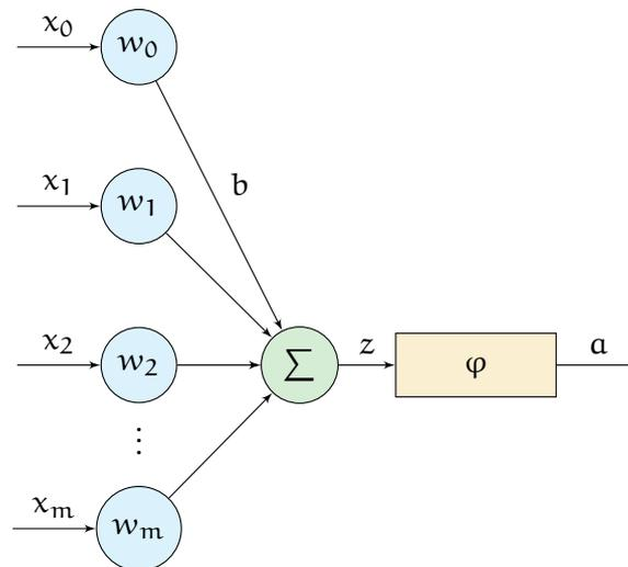
Figure 3.3: Functioning of an artificial neuron
