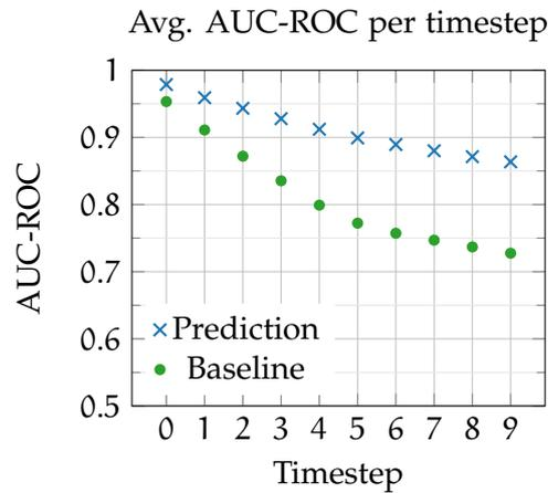
Figure 5.7: Prediction of multiple timesteps: mean AUC-ROC averaged over all notes for different predicted timesteps. Timestep no. 0 is the prediction given the very last status of the system, so it is supposed to be the most accurate one.
