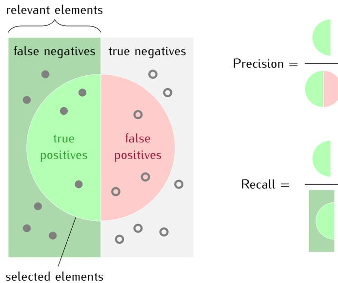
**Figure 5.1:** Precision and recall: graphical representation. Precision corresponds to how many selected items are relevant. Recall corresponds to how many relevant items are selected.
