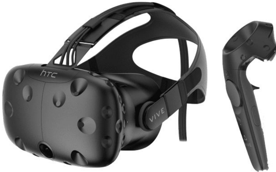
Figure 3.2: The HTC Vive headset and one of the two hand controllers. The controller provides a round trackpad (left side of controller), the grab trigger on the opposite side and three buttons. Credits: HTC™.
