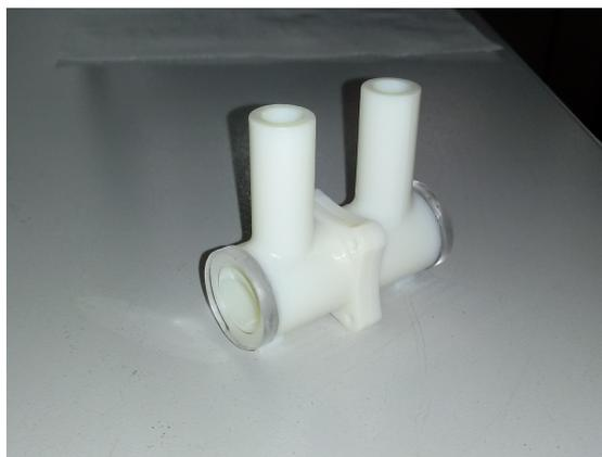
**Figure 5.3:** View of the completed H cell
