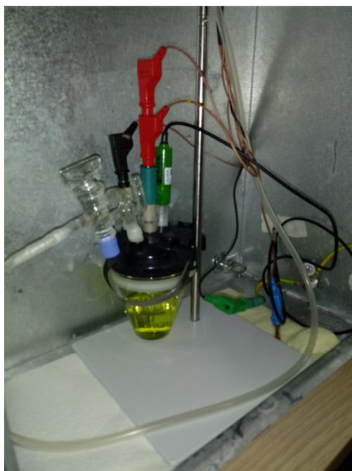
**Figure 4.1:** Apparatus used to perform measurements of diffusion coefficient of  $\text{K}_3\text{Fe}(\text{CN})_6$ .
