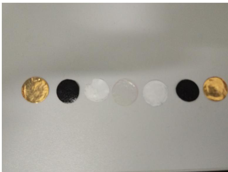
**Figure 6.16:** Expanded view of the components of the realized supercapacitor (in order from left to right: gold collector, AC disc electrode, paper separator, activated Nafion<sup>®</sup> 117 membrane, paper separator, AC disc electrode, gold collector).
