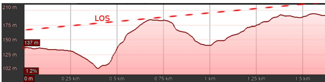
Figure 6.7: Course of the land along obstructed path and TX1B LOS.
