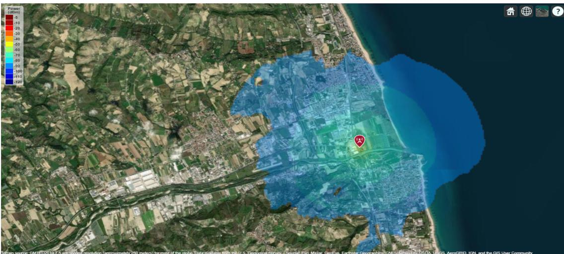
Figure 6.16: *Scenario 2*: TX2B, Output Power: 11 dBm, Receivers Height: 8 m.
