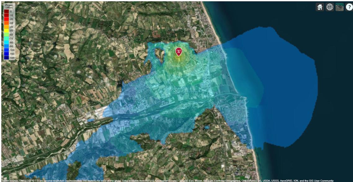
(b) TX2A, Output Power: 20 dBm, Receivers Height: 4 m.
