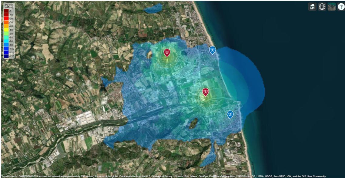
(a) TX2A & TX2B, Output Power: 14 dBm, Receivers Height: 4 m.
