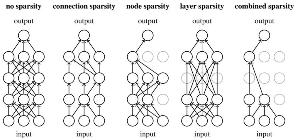
**Figure 2.1:** Feed-forward step inside Neural Networks with different types of sparsity level reported in [11]
