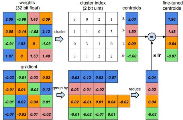
**Figure 2.3:** Weight clustering and fine-tune during back-propagation reported in [13]
