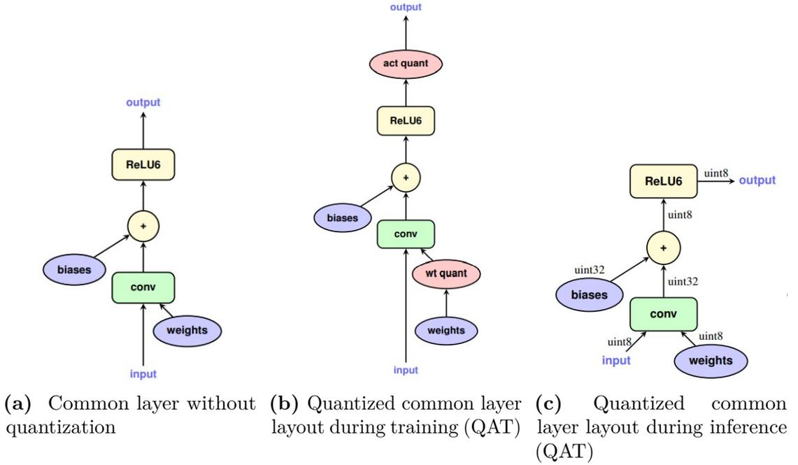
**Figure 2.5:** Quantization steps for a common Convolutional layer during *Quant-aware training* reported by [17]
