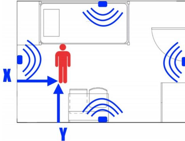
**Figure 1.7:** The four capacitive sensors positions inside the room during data collection reported by [7]
