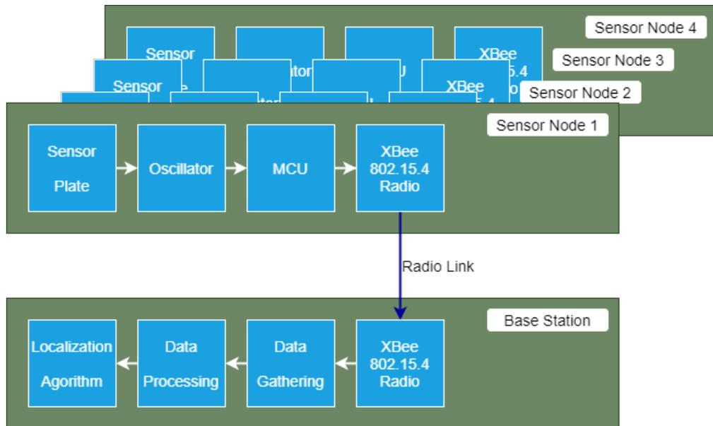
**Figure 1.6:** Main macro blocks for the system extrapolated from [7]
