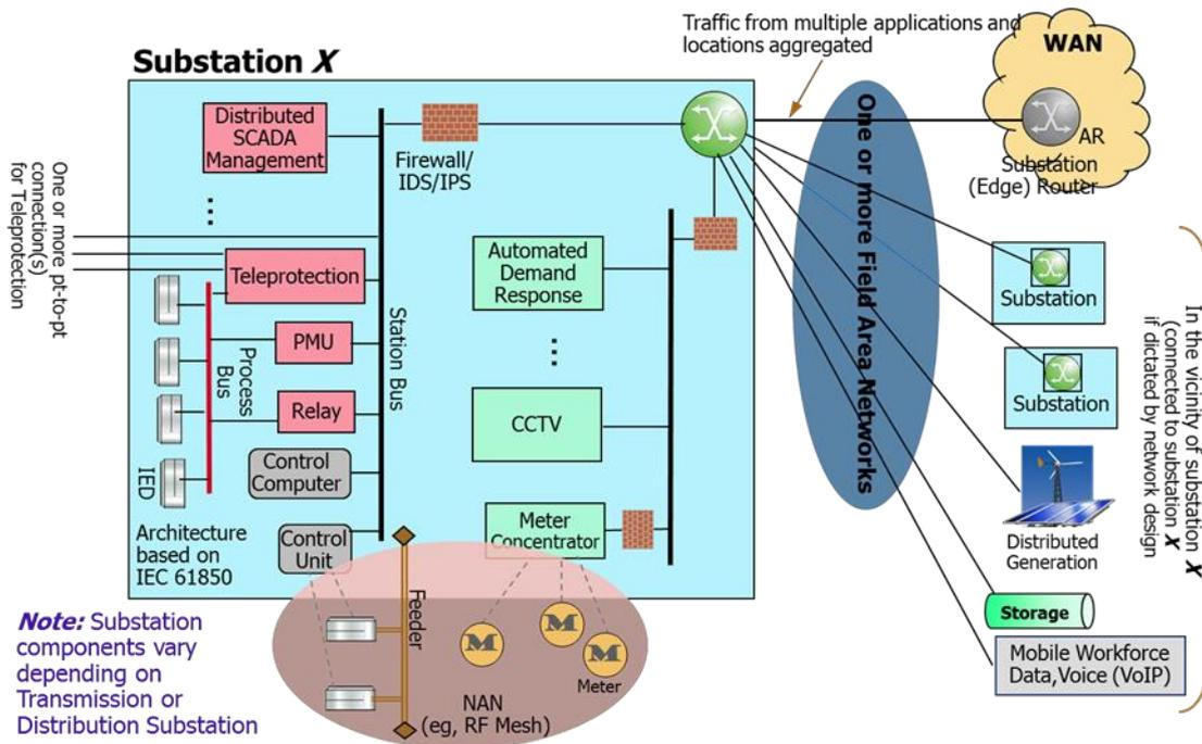
Figure (3-11) - Evolution of substation architecture based on IEC 61850 standards
