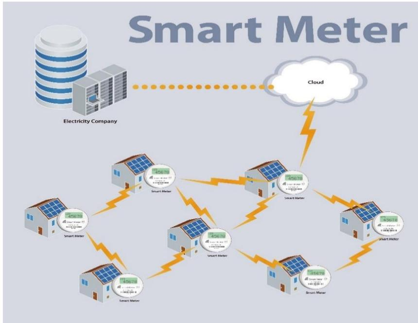
Figure (3-4) - Smart meter network configuration
