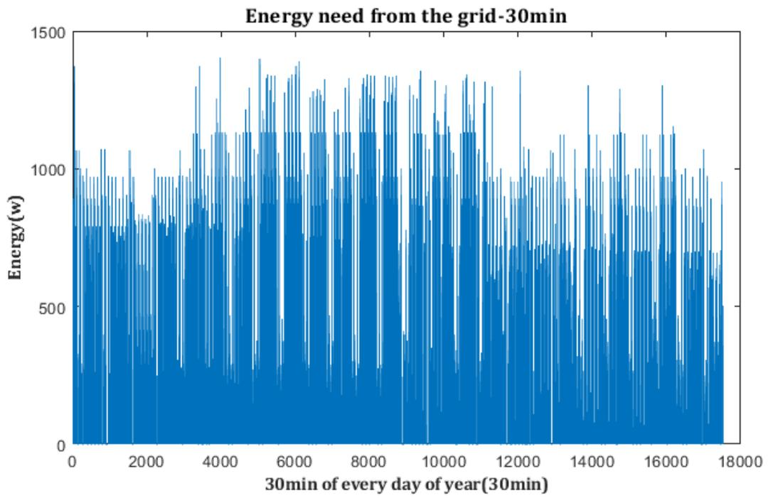
Figure (7-4) - Energy need from the grid (pv = 1, bat=5, cv=0)
