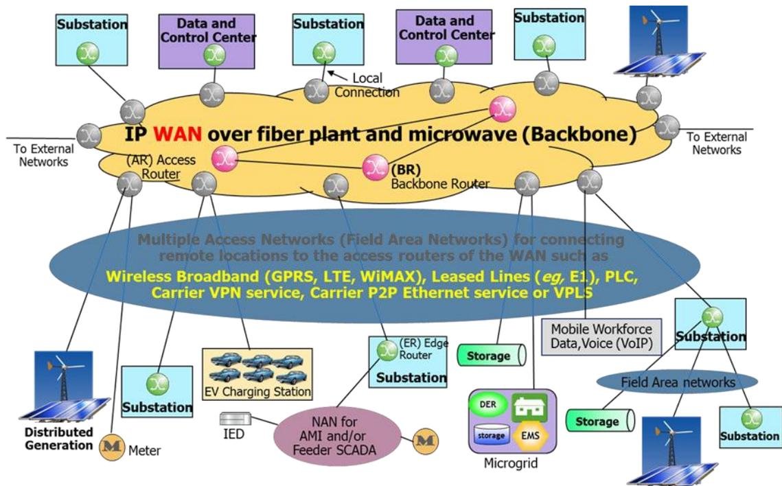
Figure (3-10) - Architecture for Integrated Communications Network for the Smart Grid
