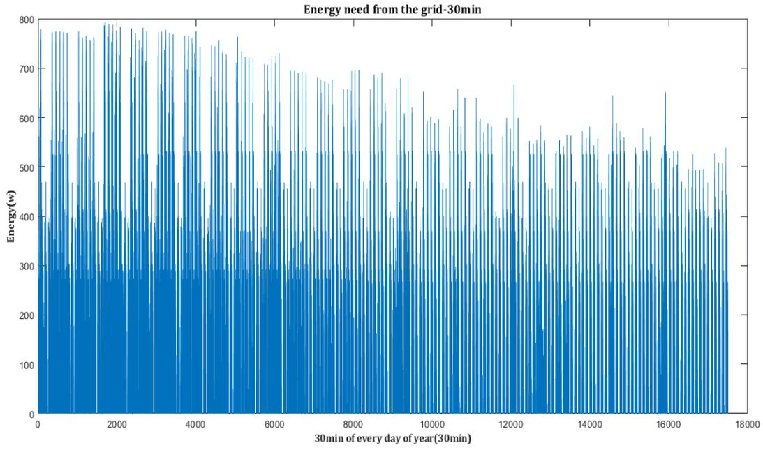
Figure (7-3) - Energy need from the grid (pv = 1, bat=0, cv=0)
