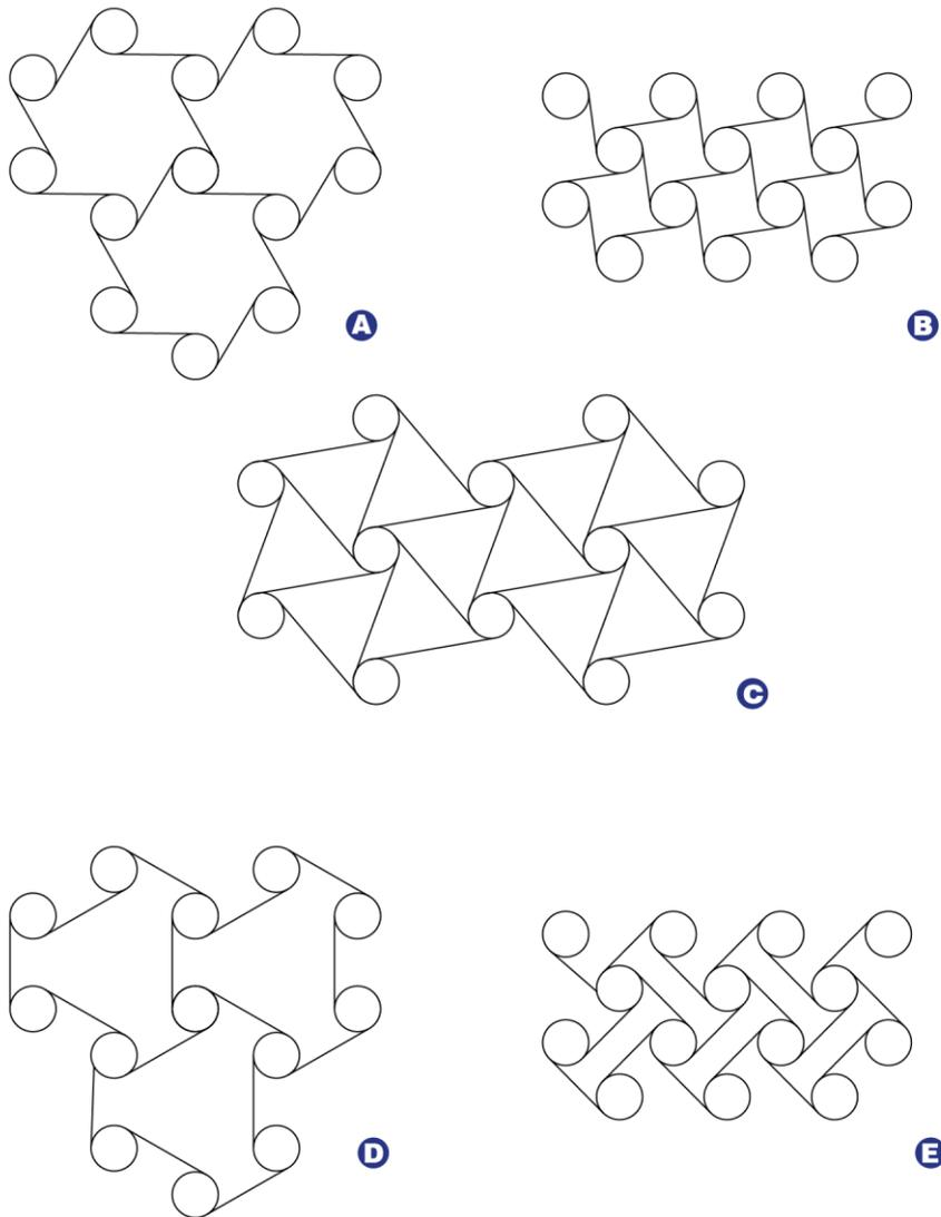
Fig. 10: 2D chiral tessellations: **a**: tri-chiral; **b**: tetra-anti-chiral; **c**: hexa-anti-chiral; **d**: tri-meta-chiral; **e**: tetra-meta-chiral
