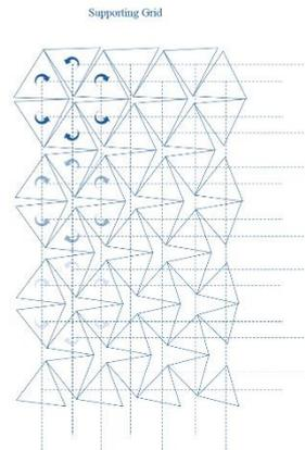
Fig. 62: Fixed support grid and rotation of proposed tessellation
