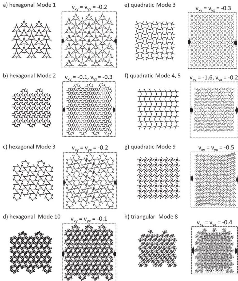
Fig. 27: Periodic lattices from the eigenmodes of figure 26 that show auxetic behavior.
