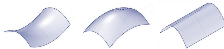
Fig. 3 Anticlastic, synclastic and monoclastic surfaces
