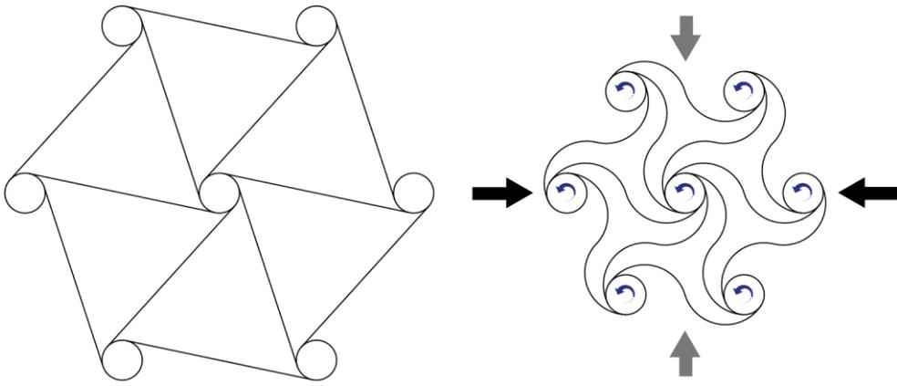
Fig. 12: Deformation of a chiral honeycomb structure under compression
