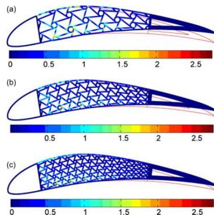
Fig. 31: Axial stress distribution ( 100 MPa) at the limit of the elastic regime of the material for aluminum alloy airfoil: (a) 2-cell configuration, (b) 3 cells, and (c) 4 cells.
