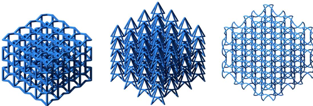
Fig. 8: 3D tessellations: re-entrant hexagons, re-entrant triangles, sinusoid ligaments
