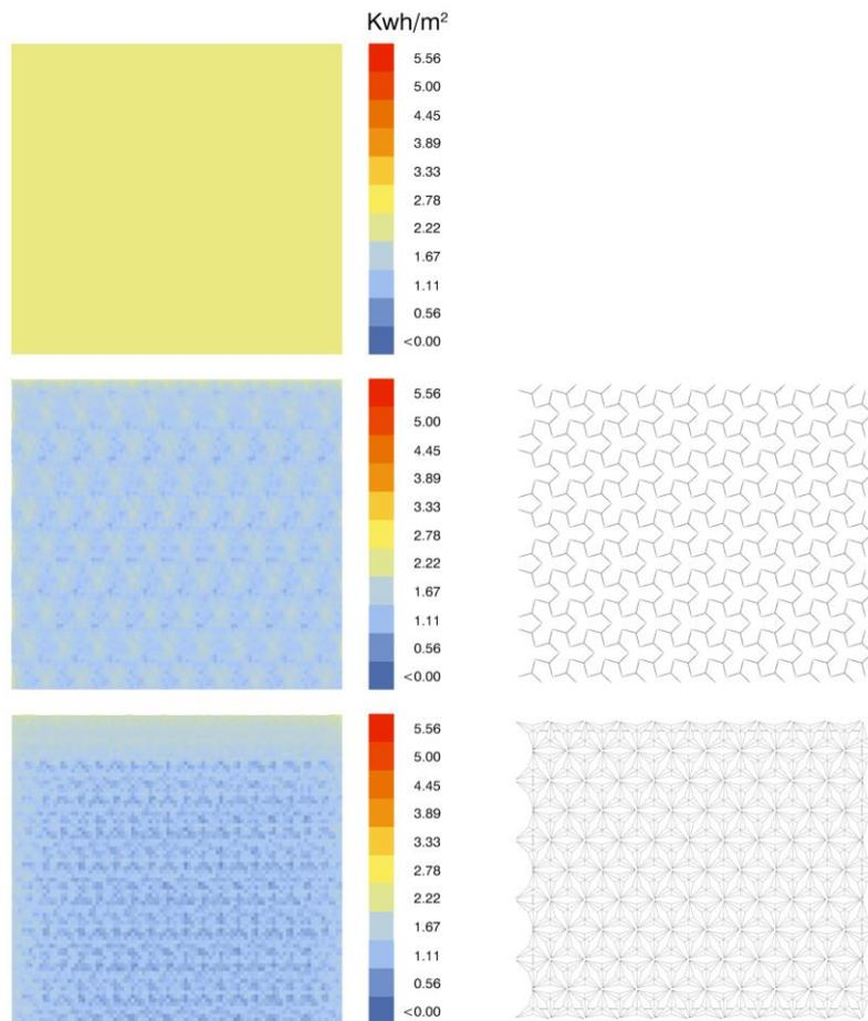
Fig. 71: Solar radiation analysis. 21/06, Turin. Fully exposed façade, open structure, and semi-closed.
