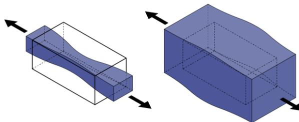
Fig. 1 : Reaction of a conventional material and an auxetic one
