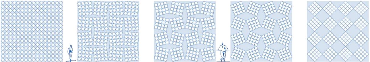
Fig. 76: Fractal pattern: proposed skin with auxetic rotating rigid units as auxetic cells
