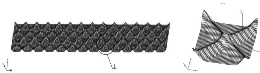
Fig. 33: Vehicle safety belt braid - CN 102729948
