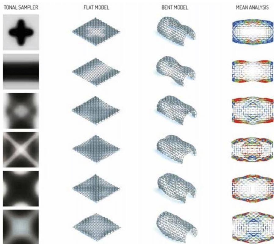
Fig. 47: Differentiation of the pattern extrusion depending on the set of gradients. For each example is shown: flat configuration, bent configuration and curvature analysis of the structure.
