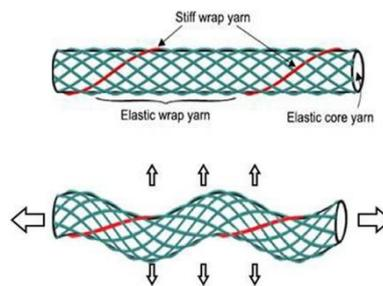
Fig. 28: Auxetic Yarn Made with Circular Braiding Technology
