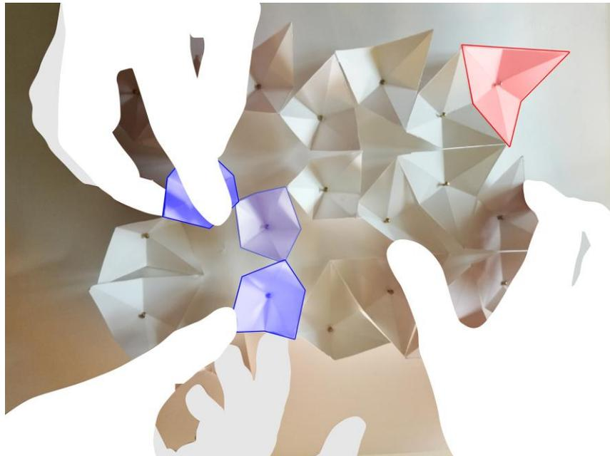
Fig. 77: Paper model, actuation by hand (blue) transmitting to the connected unit. (Relaxed state in red)
