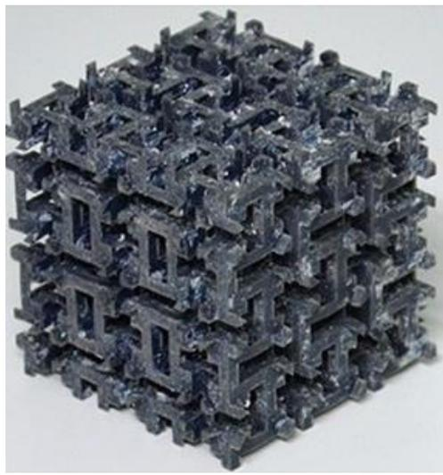
Fig. 15: Hsin-Haou Huang et al. 3D meta-chiral lattice structure
