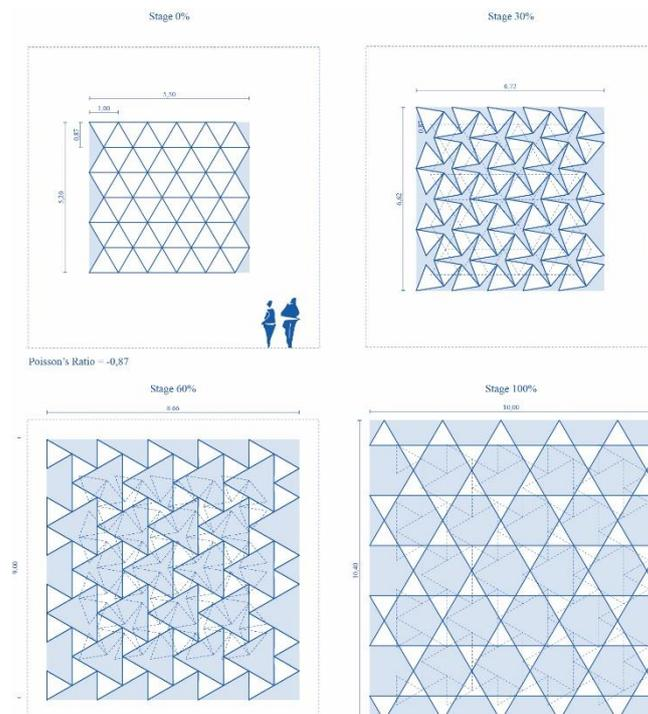
Fig. 59: Opening mechanism of rotating rigid triangles
