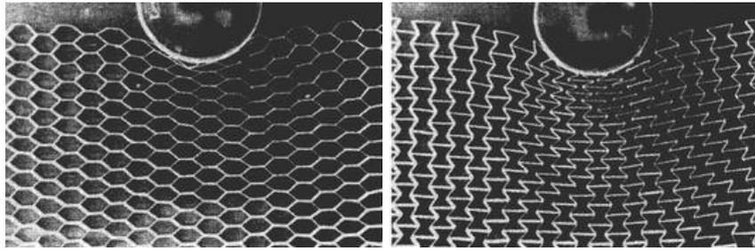
Fig. 2 Indentation resistance in a conventional material and in an auxetic one
