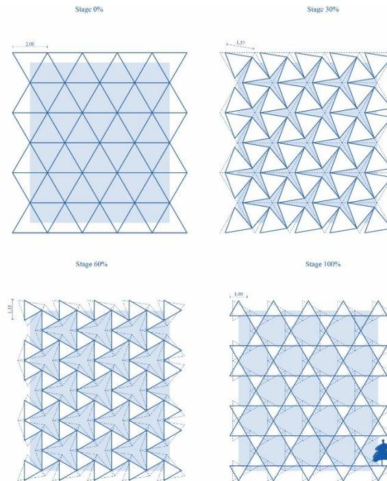
Fig. 60: Opening mechanism of proposed rotating scaling triangles
