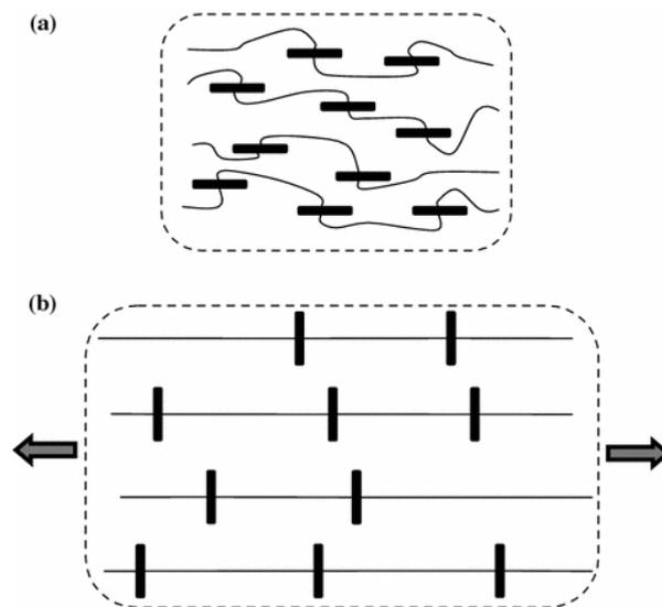
Fig. 25: Auxetic behavior of generic microporous polymer models, before (a) and after load (b)
