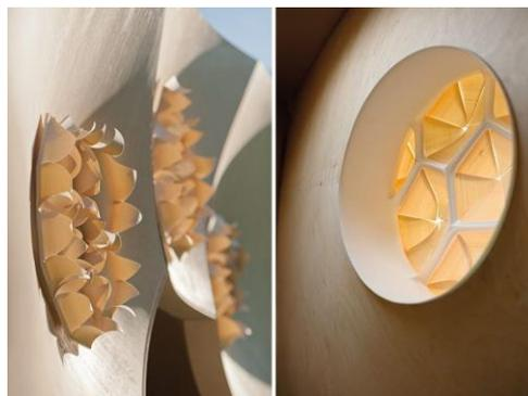
Fig. 44: Achim Menges's HygroSkin, in humid and dry atmosphere
