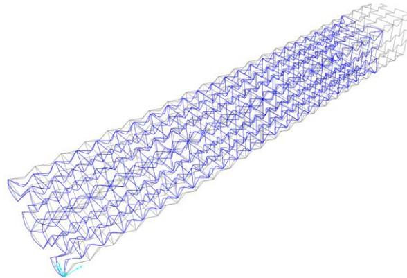
Fig. 45: 3D hexagonal re-entrant honeycomb grid for reinforced concrete beam
