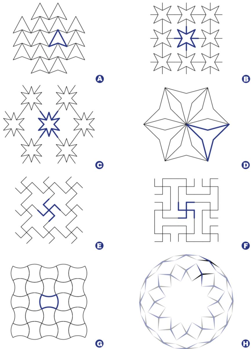
Fig. 7: 2D re-entrant tessellations: **a**: re-entrant triangle; **b**: 4-point star shape re-entrant honeycomb; **c**: 6-point star shape re-entrant honeycomb; **d**: structurally hexagonal re-entrant honeycomb; **e**: lozenge missing rib model; **f**: square missing rib model; **g**: chiral quadratic lattice structure; **h**: Hoberman circle
