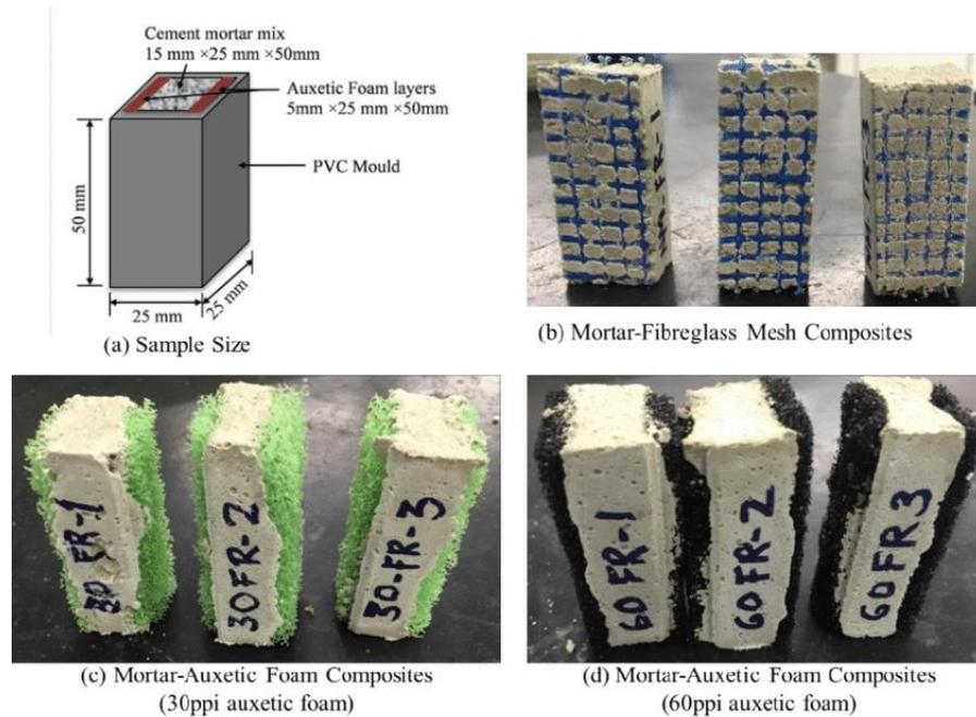
Fig. 46: Mortar-Auxetic Foam Composite Samples
