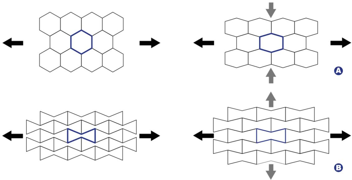
Fig. 6: Conventional Honeycomb (a) and re-entrant honeycomb (b) response to axial deformation
