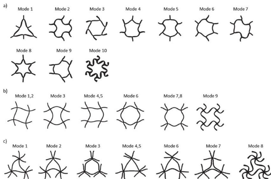
Fig. 26: First eigenmodes of the basic 2D structures with periodic boundary conditions. (a) hexagon, (b) square, (c) triangle.
