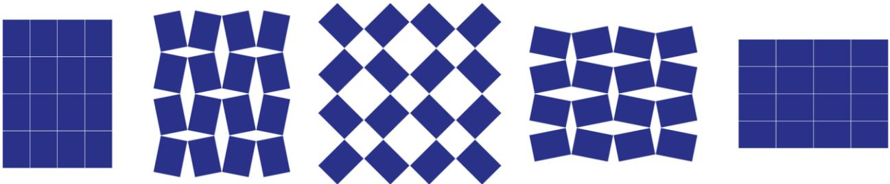
Fig. 17: Rotating rigid rectangles exhibiting both positive and negative Poisson's ratio
