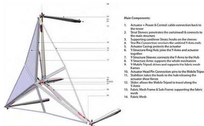
Fig. 65: Al Bahr shading system
