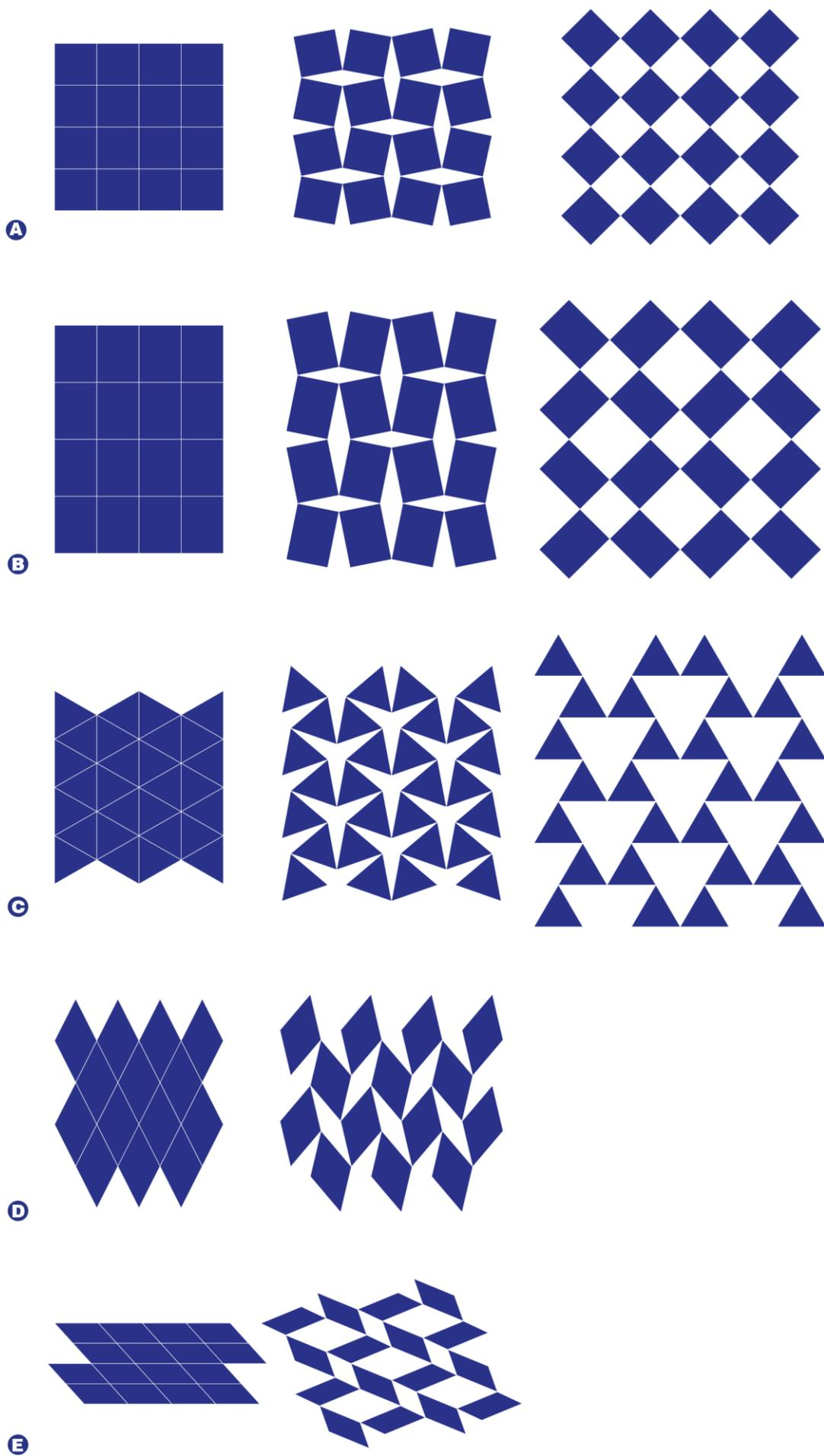
Fig. 16: Rotating rigid units models: **a:** squares; **b:** rectangles; **c:** rectangle triangles; **d:** rhombi; **e:** parallelograms
