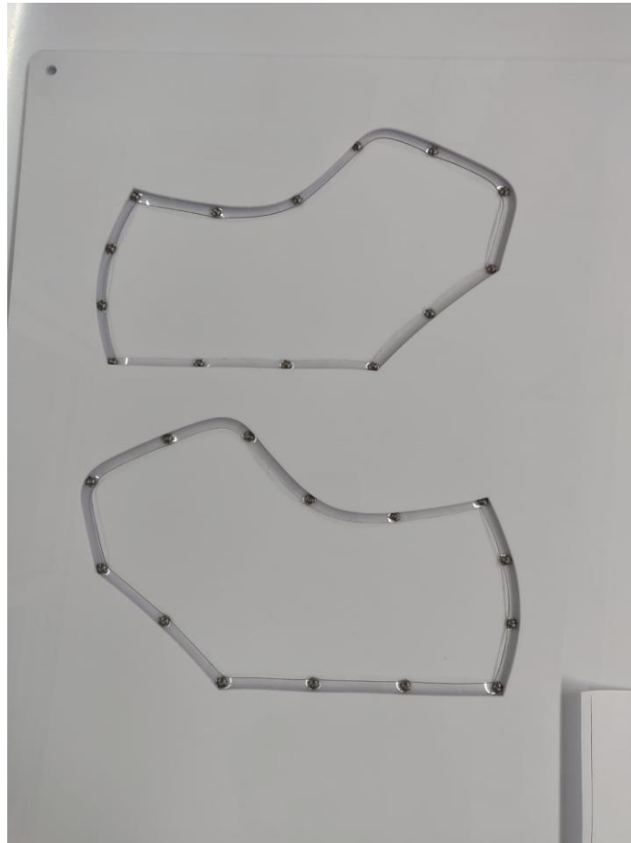
Figure III.7 It is a white and transparent table overlap detail. Here it is possible to notice how the hole in the white table circumscribes the tacks in the transparent table.
