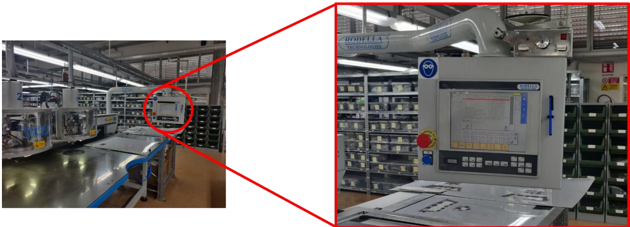
Figure IV.17 It shows the location and the machine PC with which the operator must interact to accomplish all the machine operations. In this specific case the selection of the machining file.
