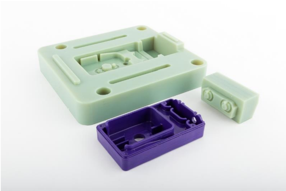
Figure 12 Example of injection mold made using a 3D printer (thefabricator.com)
