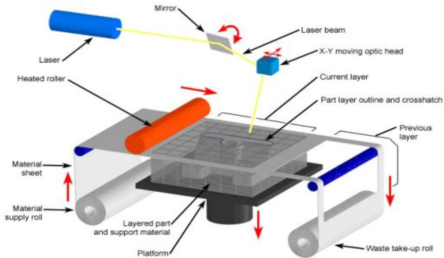
*Fig. 5. Laminated object manufacturing*
