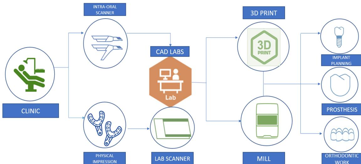
*Fig. 38. CAD/CAM Workflow*
