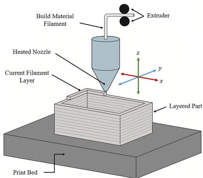
*Fig. 2. Material Extrusion process*
