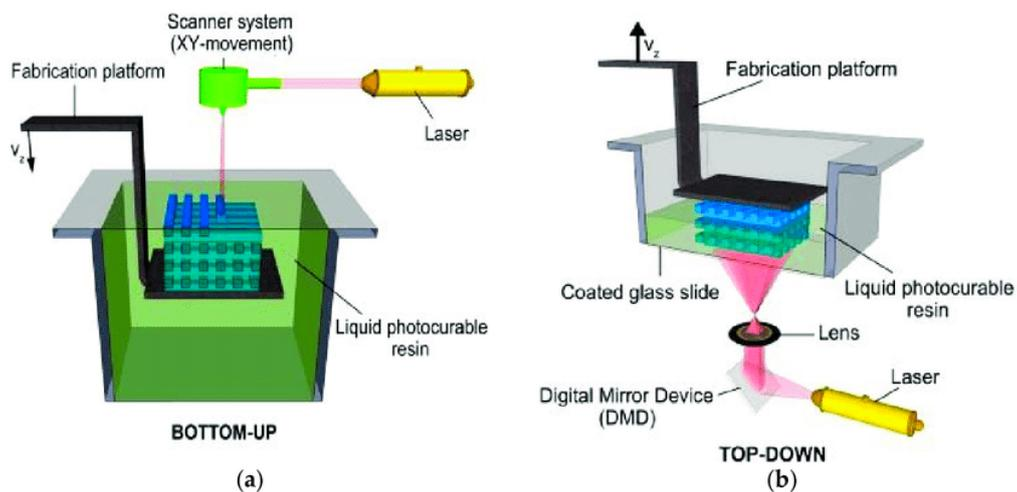
Fig. 9. Bottom-up approach (a) and Top-down approach (b)
