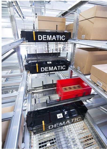
Figure 2.23 Dematic, Multishuttle in the Flex configuration with capture fingers [12]
