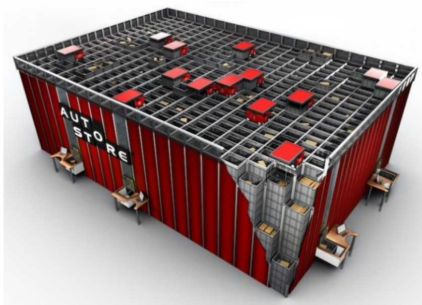
Figure 1.16 Representation of AutoStore™, i.e. Grid Based Storage System [15]
