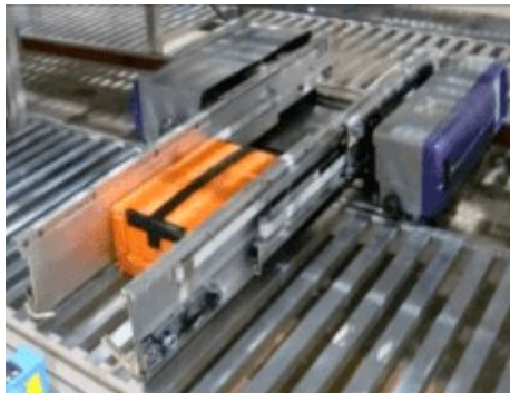
Figure 2.22 Daifuku, Shuttle Rack M, focus on clamping mechanism [11]
