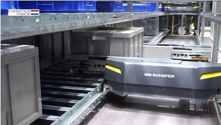
Figure 2.25 SSI Schaefer, (A) on the left Flexi; (B) on the right Navette, multi-level shuttle-based storage system [14]
