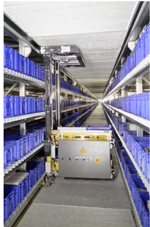
Figure 2.25 SSI Schaefer, (A) on the left Flexi; (B) on the right Navette, multi-level shuttle-based storage system [14]
