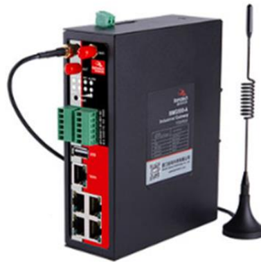
Figure 3-3 a gateway device used in factory
