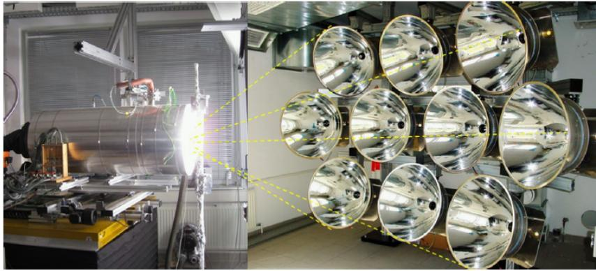
Figure 3.3: High flux solar simulator, German Aerospace Center (DLR), Germany [30].
