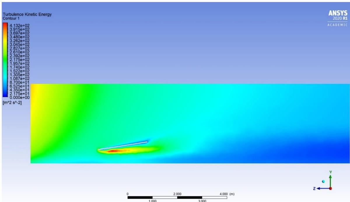
Figure 55: Turbulent kinetic energy contour when wind is impacting the 9° tilted panels from the front, plane zy.
