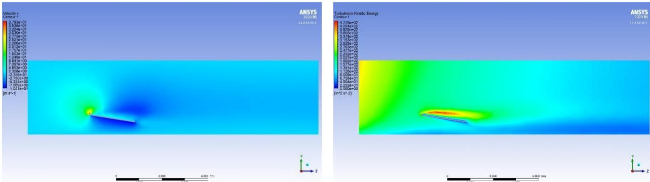
*Figures 62-63: Velocity contour in y direction when wind is impacting the 9° tilted panels from the back, turbulent kinetic energy, plane zy.*
