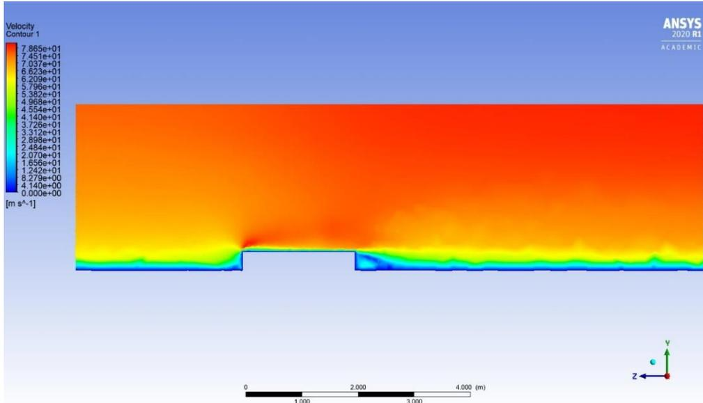
Figure 71: Velocity contour when wind is impacting the floats from the front, plane zy.
