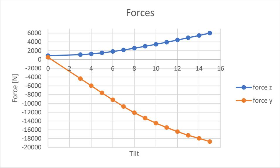
Figure 46: Drag and Lift forces of the solar panels as function of the inclination angle when wind is impacting from the front.
