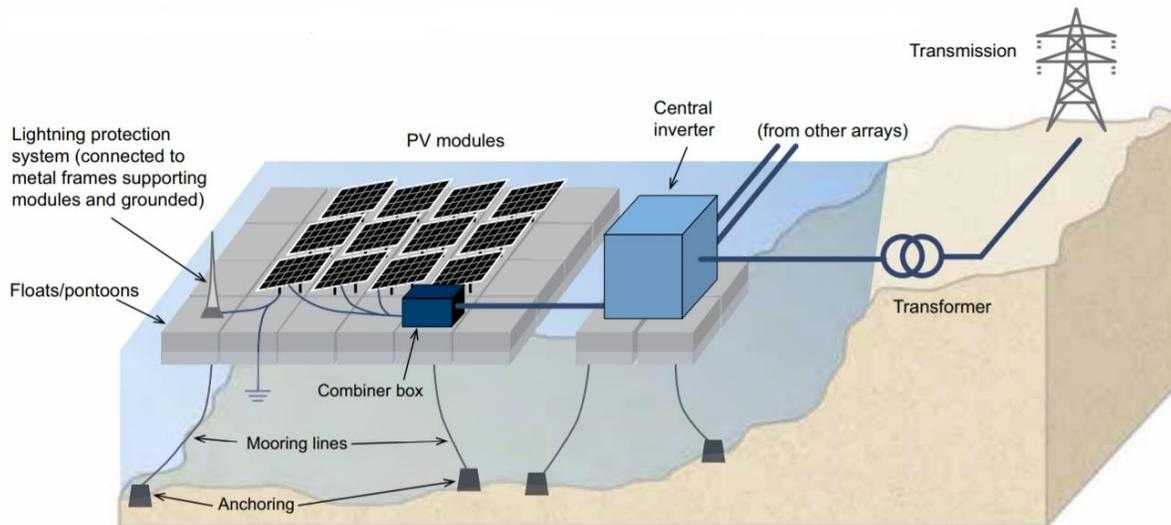
Figure 3: Floating photovoltaic system design, World Bank Group, ESMAP, and SERIS 2019 [4].
