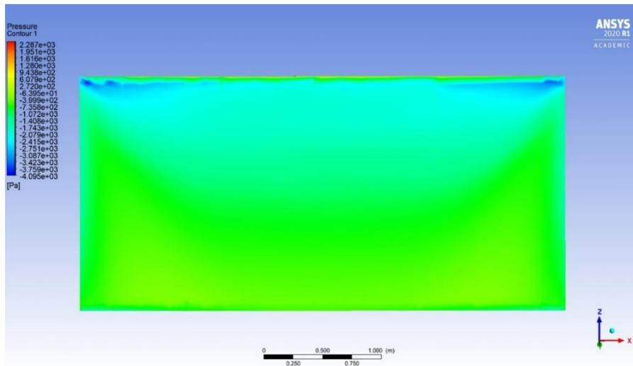
*Figure 59: Pressure contour when wind is impacting the 9° tilted panels from the front, back panel face.*
