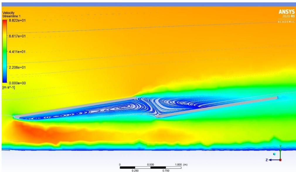
Figure 68: Velocity streamlines when wind is impacting the 9° tilted panels from the front with two panel's rows, zoom on the swirls, plane zy.
