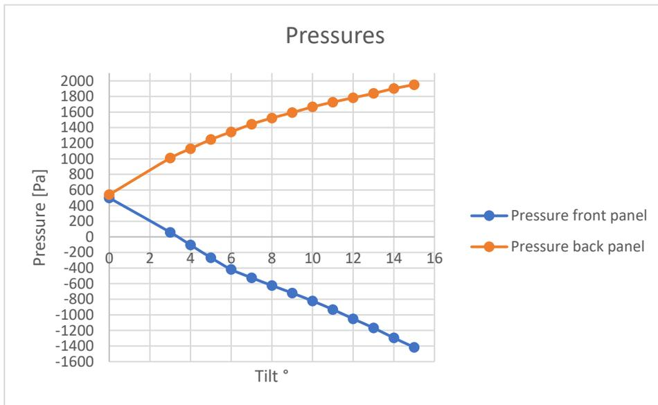
Figure 50: Pressures on the frontal and back wall of the panels as function of the inclination angle when wind is impacting from the back.
