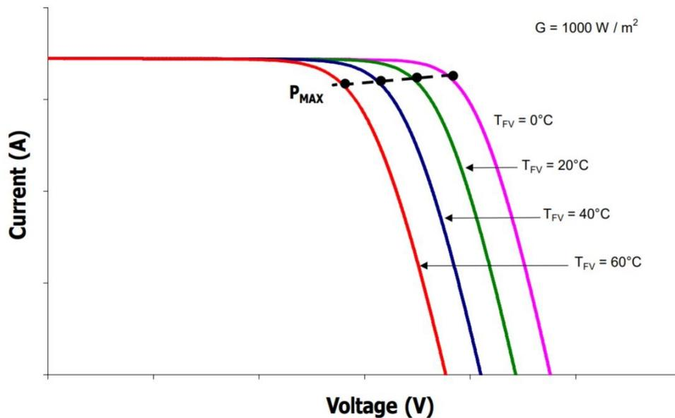
Figure 6: Current-Voltage diagram showing the effects of temperature on the solar panel power production, Spertino F., slides of the course "solar photovoltaic systems" [9].
