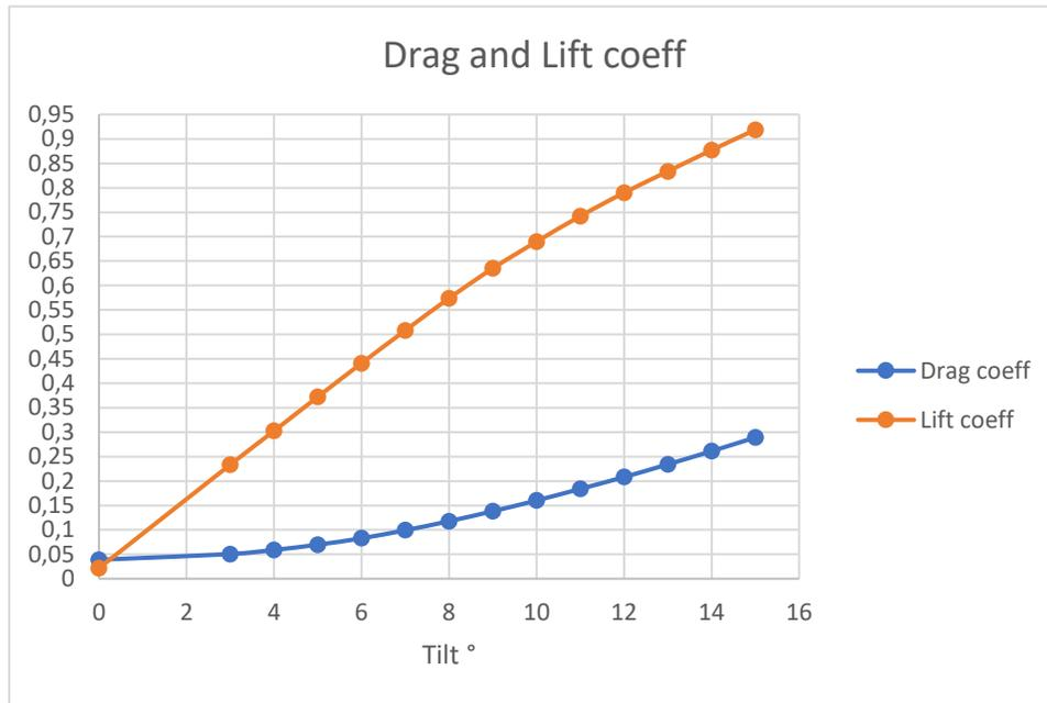
Figure 48: Drag and Lift coefficients of the solar panels as function of the inclination angle when wind is impacting from the back.
