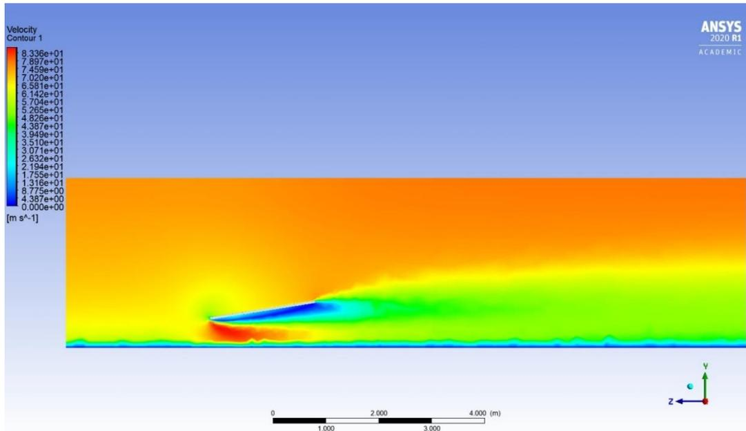
Figure 51: Velocity contour when wind is impacting the 9° tilted panels from the front, plane zy.
