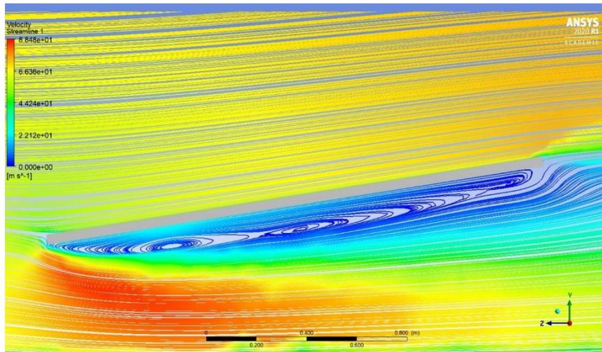
*Figure 54: Velocity streamline showing swirls under the solar panels, plane zy.*
