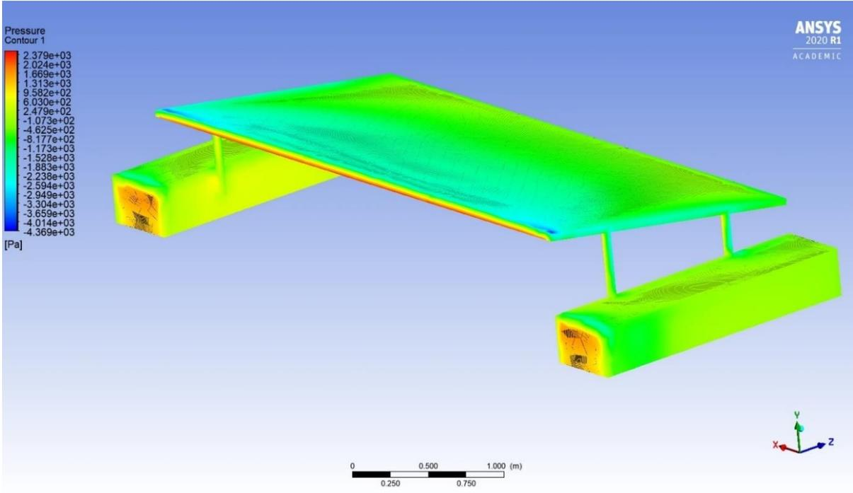
Figure 78: Pressure contour when wind is impacting the NRG island unit from the back.
