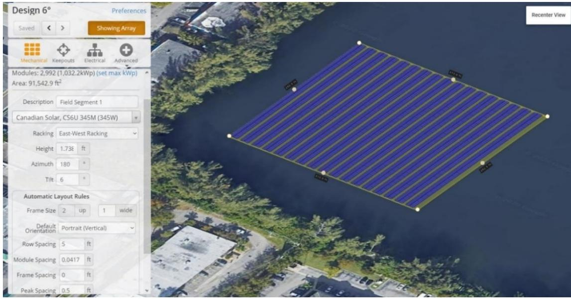
Figure 81: Floating solar farm in east west configuration 2992 panels used and 1,032.2 kWp installed, Helioscope.
