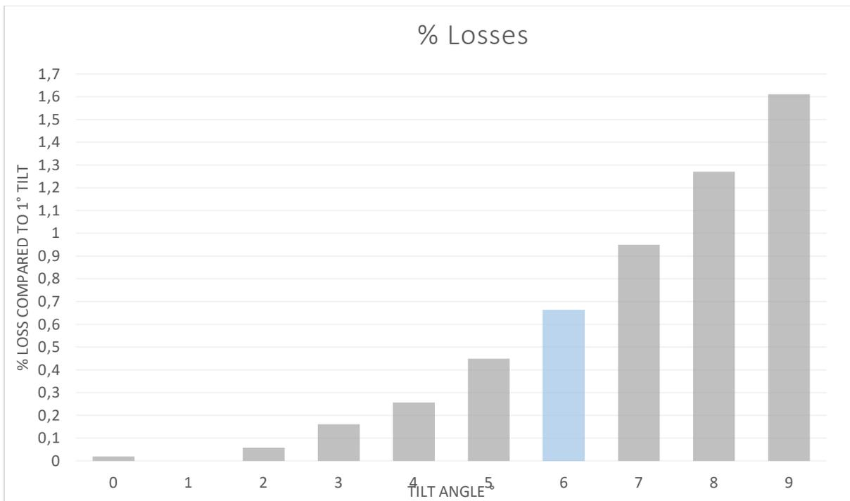
Figure 83: Histogram of the percentual losses compared to the optimal tilt which is 1°.
