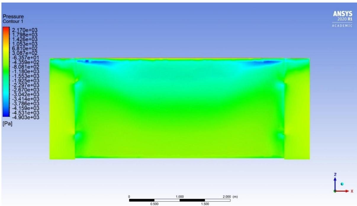
Figure 77: Pressure contour when wind is impacting the panels from the front, view from below.
