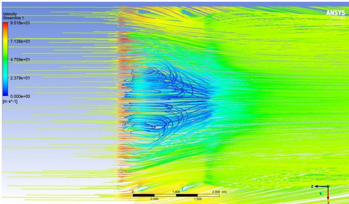
Figure 75: Velocity 3D streamline when wind is impacting the panels from the front plane under the panels, plane  $xz$ .
