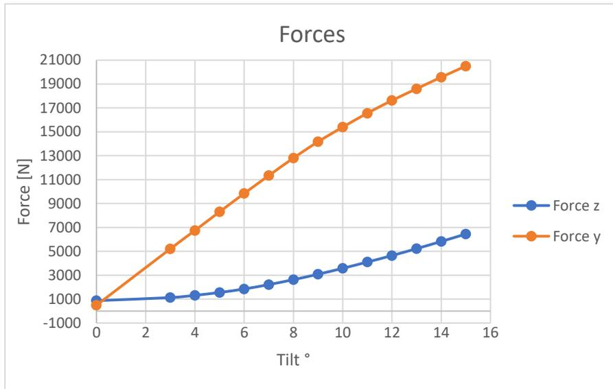
Figure 49: Drag and Lift forces of the solar panels as function of the inclination angle when wind is impacting from the back.
