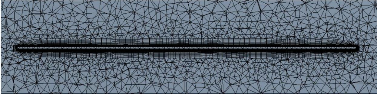
*Figure 41: Section and zoom on the solar panels set, showing the dense mesh layers near the solar panels surface.*
