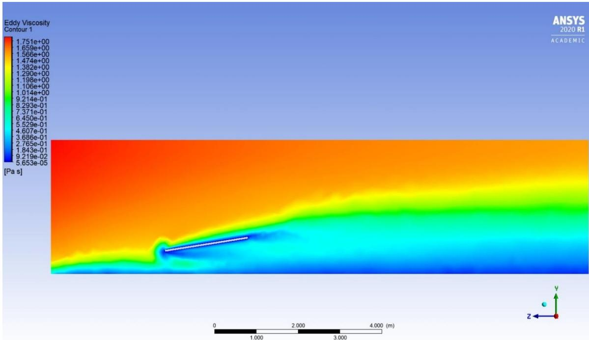
Figure 56: Eddy viscosity contour when wind is impacting the 9° tilted panels from the front, plane zy.
