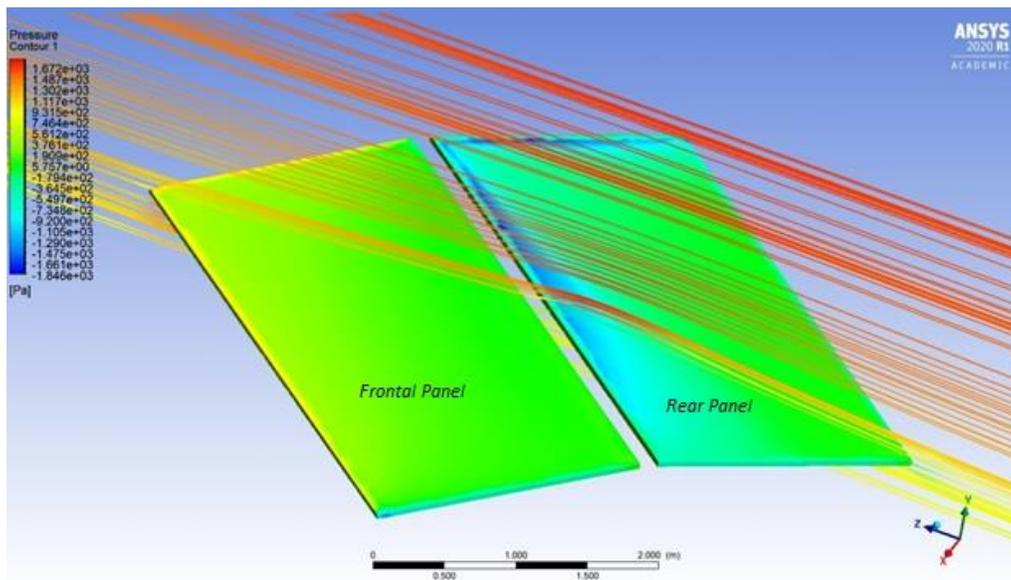
Figure 84: Velocity streamlines on the plane zy hitting the panels and pressure contour on the panels.
