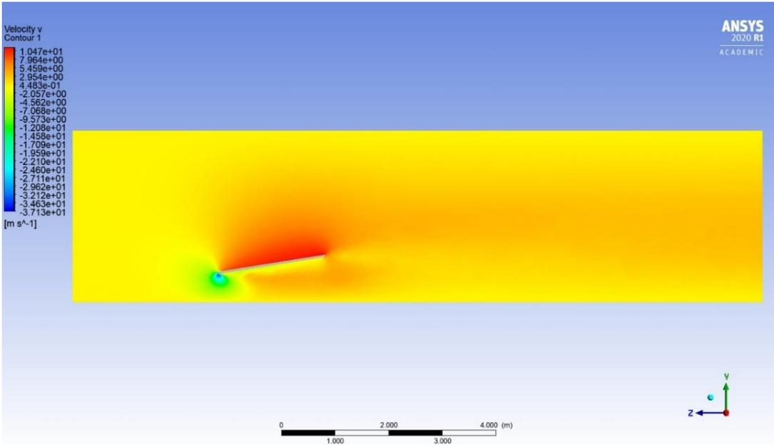
*Figure 52: Velocity contour in the y direction when wind is impacting the 9° tilted panels from the front, plane zy.*
