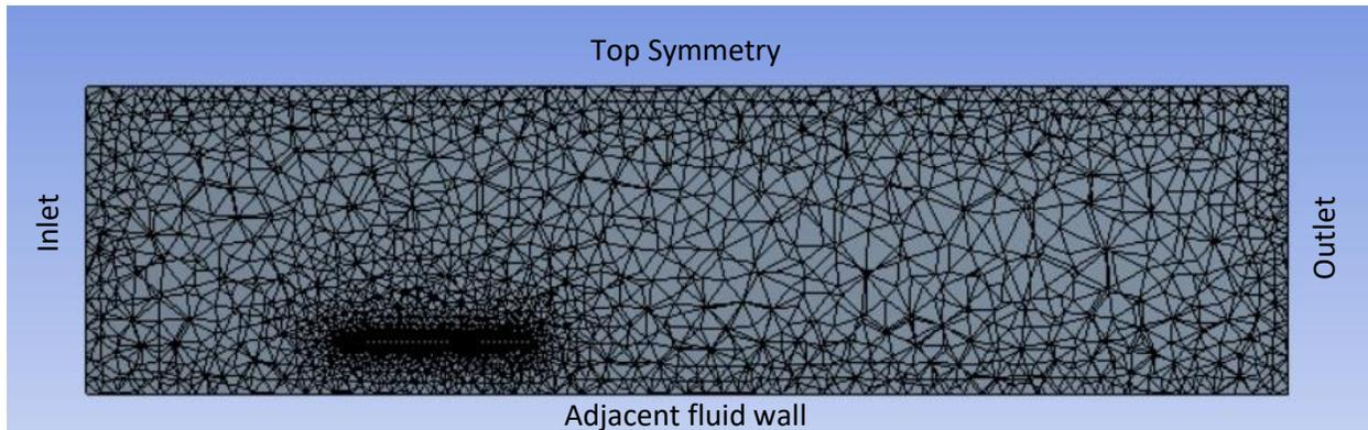
Figure 42: Fluid domain section showing the mesh, a denser mesh in near the solar panels set.
