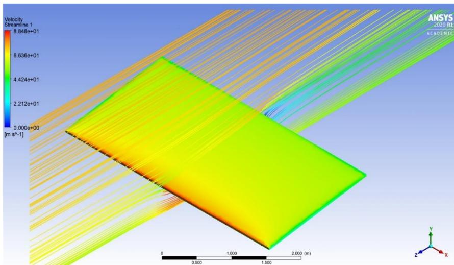
Figure 57: Wind path on plane zy and solar panels facing pressures.
