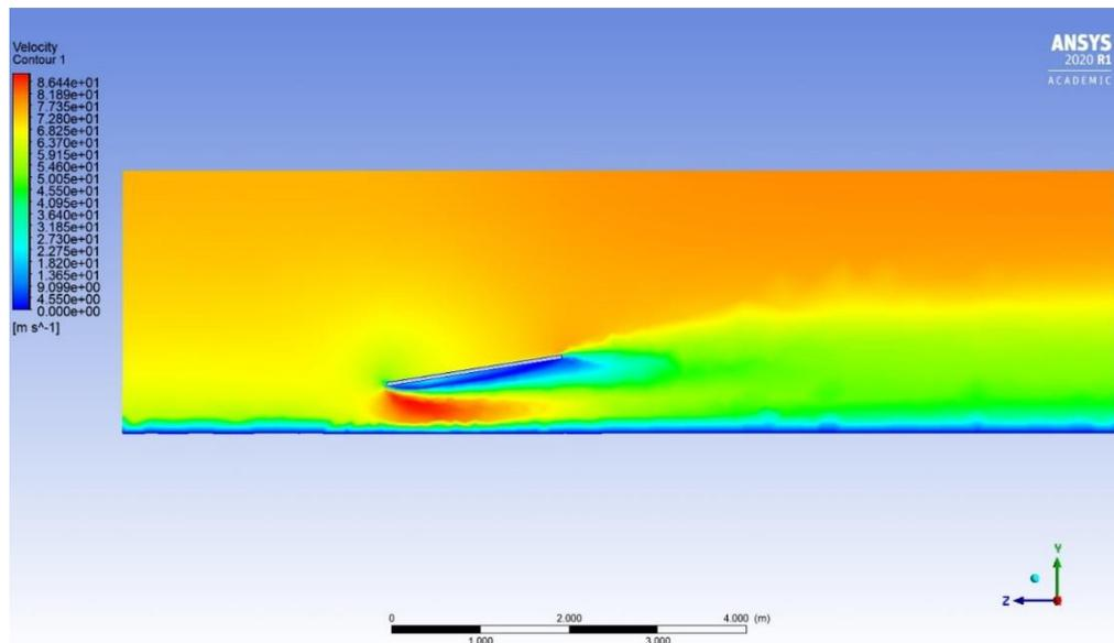
*Figure 70: Velocity contour when wind is impacting the NRG island 9° tilted panels from the front, plane zy.*
