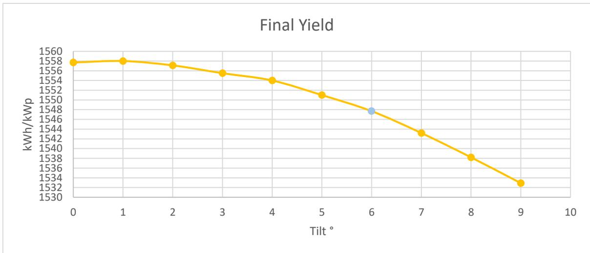
Figure 82: Final Yield as function of the tilt angle in the east-west configuration.
