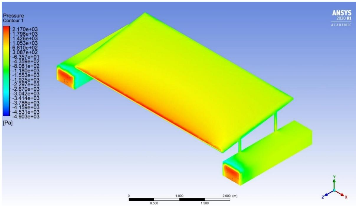
Figure 76: Pressure contour when wind is impacting the NRG island unit from the front.
