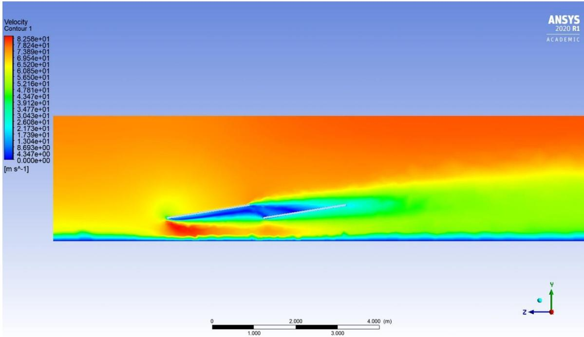
Figure 67: Velocity contour when wind is impacting the 9° tilted panels from the front with two panel's rows, plane zy.
