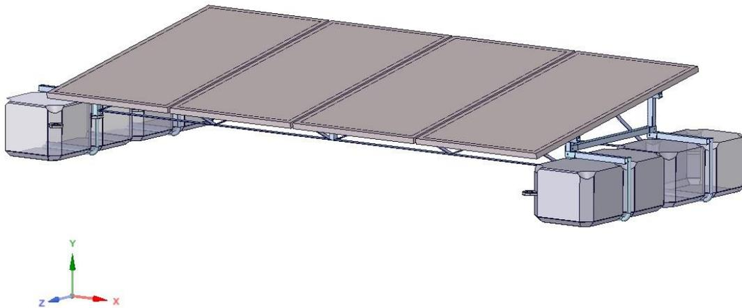
Figure 37: 3D geometry of NRG Island Unit patented by NRG Energia.
