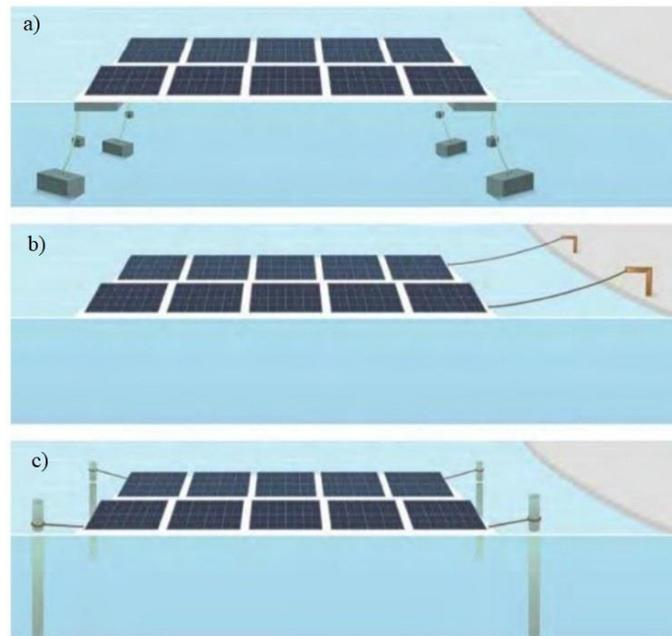
Figure 4: Anchoring and mooring techniques for FPV systems, from the top it is shown the bottom anchoring (a), the bank anchoring (b) and at the bottom the pile anchoring (c), World Bank Group, ESMAP, and SERIS 2019 [1].
