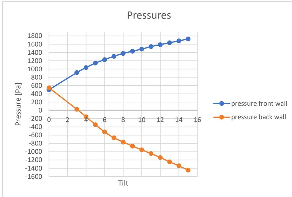
Figure 47: Pressures on the frontal and back wall of the panels as function of the inclination angle when wind is impacting from the front.
