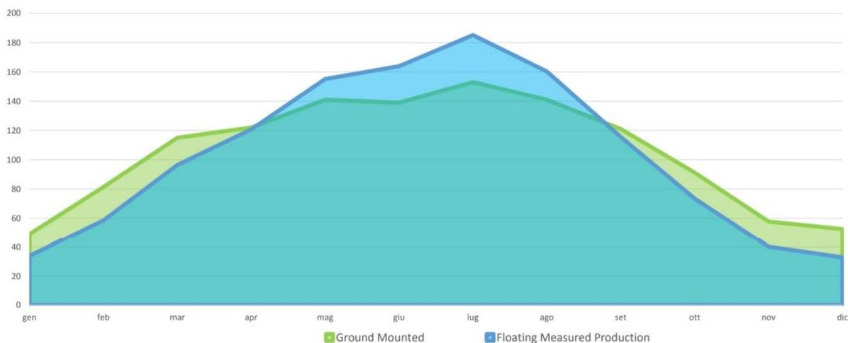
*Figure 7: Energy production of a ground mounted system and a floating mounted system over the year, test carried out by NRG Energia [8].*
