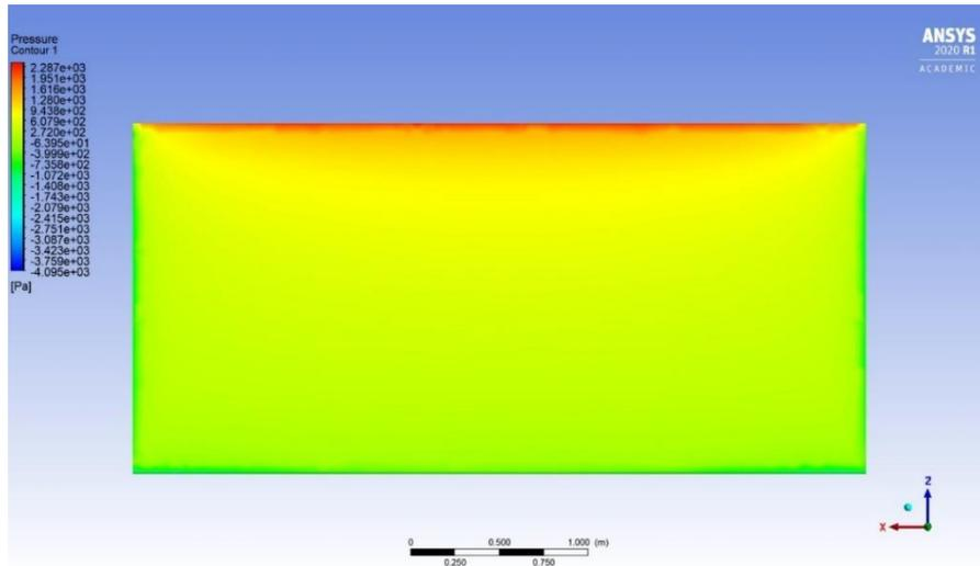
*Figure 58: Pressure contour when wind is impacting the 9° tilted panels from the front, frontal panel face.*
