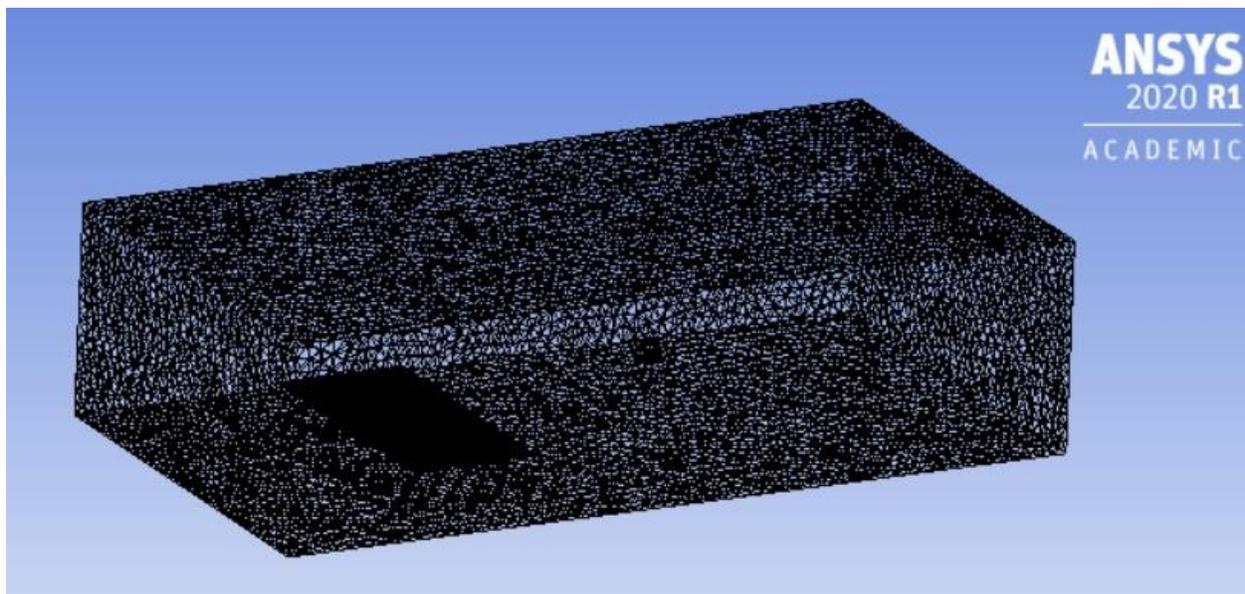
Figure 40: Mesh of the entire fluid domain, the darker part represents the solar panels set with a  $0^\circ$  tilt .
