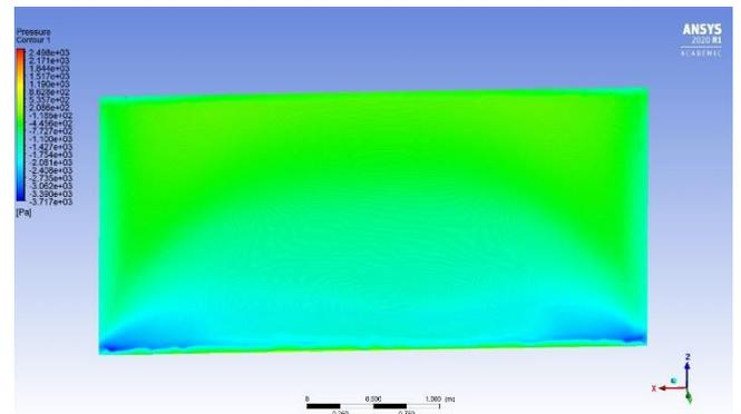
*Figures 65-66: Pressure contour when wind is impacting the 9° tilted panels from the back, back and front panels face.*
