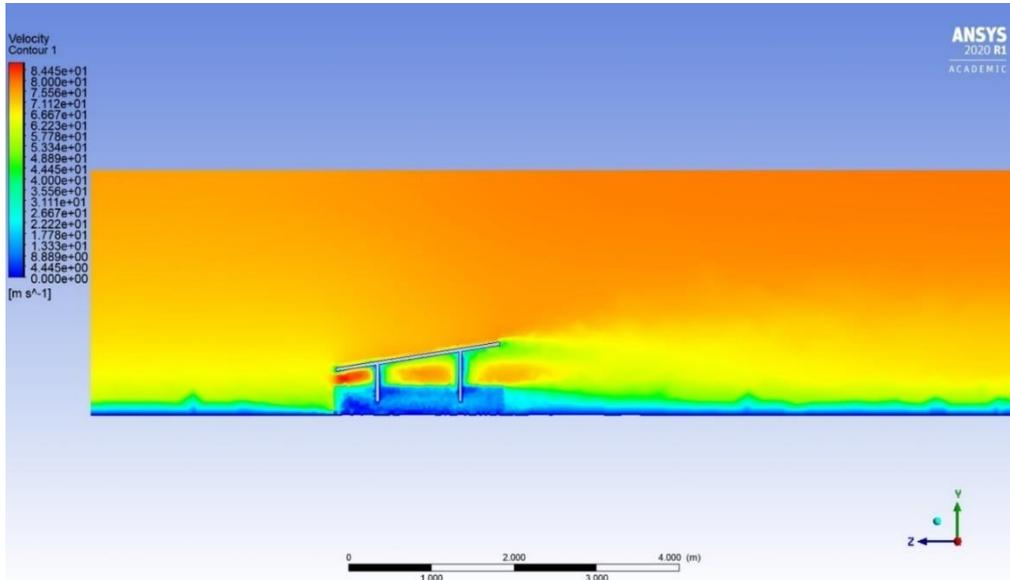
Figure 73: Velocity contour when wind is impacting the structures and panels from the front, plane zy.
