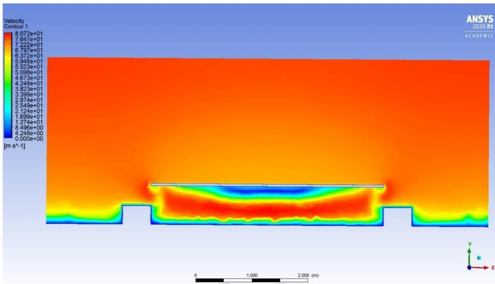
Figure 74: Velocity contour when wind is impacting the panels from the front, plane in the middle of NRG unit, plane yx.
