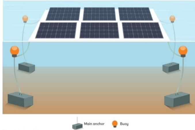
Figure 5: Anchoring using the buoy method, World Bank Group, ESMAP, and SERIS 2019 [1].
