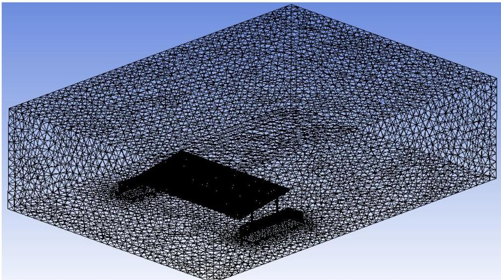
*Figure 69: Mesh of the entire fluid domain, the darker part represents the NRG island unit with  $9^\circ$  tilt panels.*
