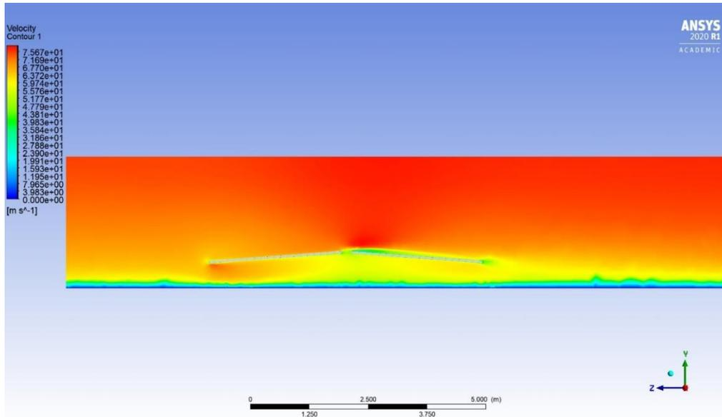
Figure 85: Velocity contour of wind is impacting east-west panels from a 45° angle, plane zy.
