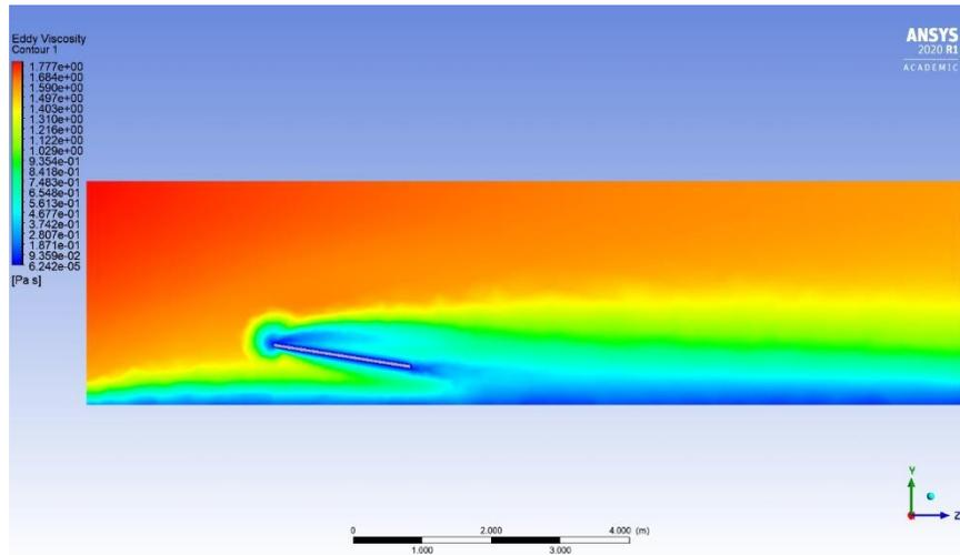
*Figure 64: Eddy viscosity when wind is impacting the 9° tilted panels from the back, plane zy.*
