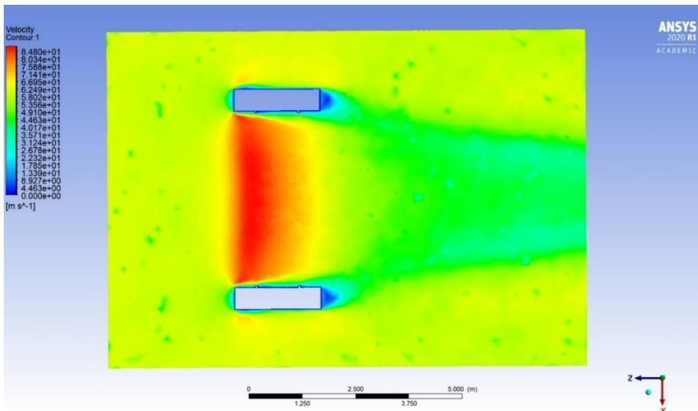
Figure 72: Velocity contour when wind is impacting the floats from the front, plane zx.
