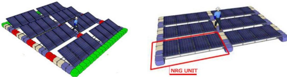
Figure 13: NRG Island Floating photovoltaic system and NRG unit, NRG Energia.
