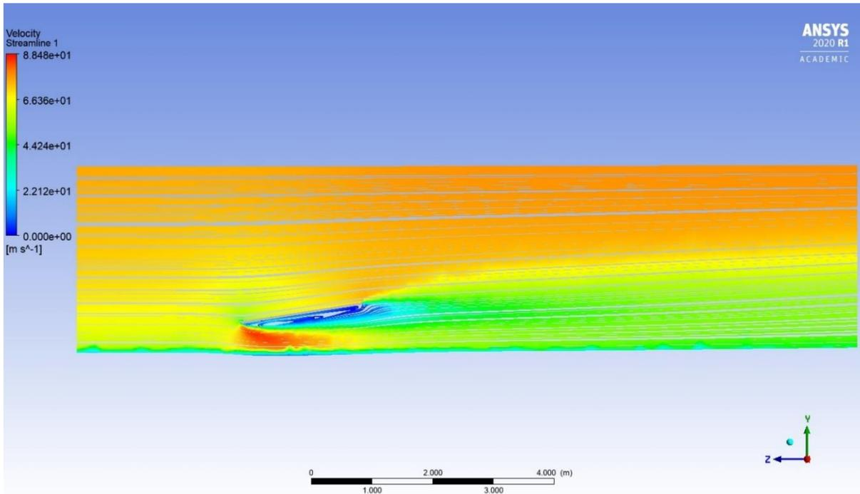
*Figure 53: Velocity streamline when wind is impacting the 9° tilted panels from the front, plane zy.*
