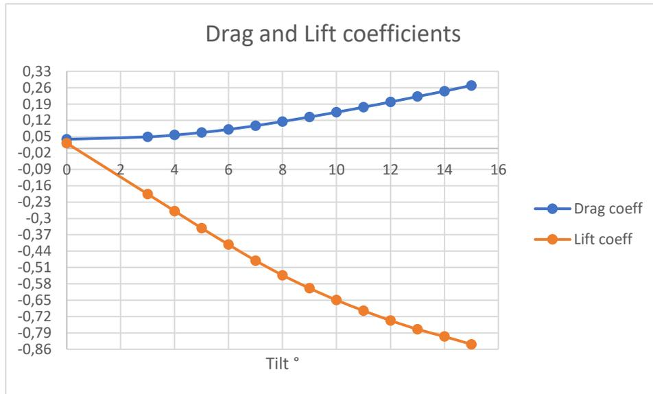
Figure 45: Drag and Lift coefficients of the solar panels as function of the inclination angle when wind is impacting from the front.
