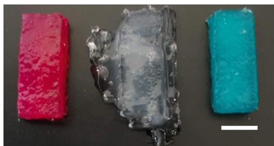
Figure 4-5 - Cubic samples printed with formulations containing methyl red (left), no dye (center), and brilliant green (right). Ref bar: 10 mm
