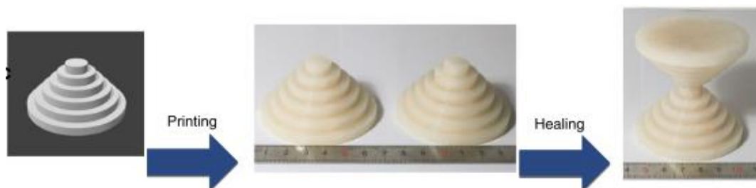
Figure 3-22 - Irregular object obtained by 3D printing with PDMS/Zn inks, followed by healing [153].
