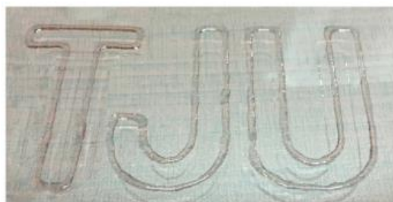
Figure 3-17 - 3D -printed patterns of T, J, U with PNGA-PAMPS/PEDOT/PSS [140].
