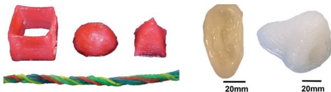
Figure 3-21 - 3D- Printed structures with alginate-PEG-nanoclay hydrogels (hollow cube, hemisphere, pyramid, twisted bundle, the shape of an ear, and a nose) [149].
