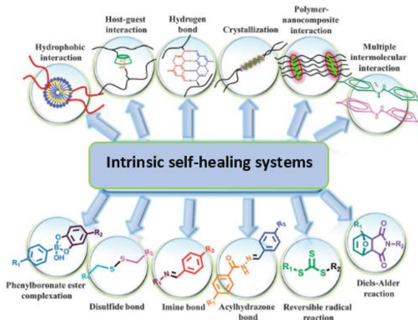
Figure 2-7 - Different available approaches to achieve self-healing in polymers. Upper part: via supramolecular interactions, bottom part: via dynamic covalent bonds [35].
