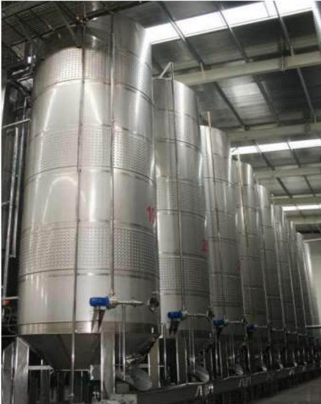
**Figura 69**, Automatic Pomace Removal Tank – *Prettech Machinery & Technology*
