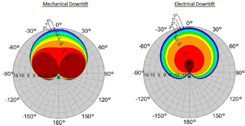
Figure 6.4: Radiation pattern for mechanical and electrical tilt. In particular, the picture shows the pattern in the horizontal (or azimuthal) plane of an antenna with an azimuth HPBW of  $65^\circ$  and an elevation HPBW of  $7^\circ$ . [14]
