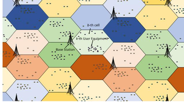
Figure 6.1: Mobile network structure. [7]
