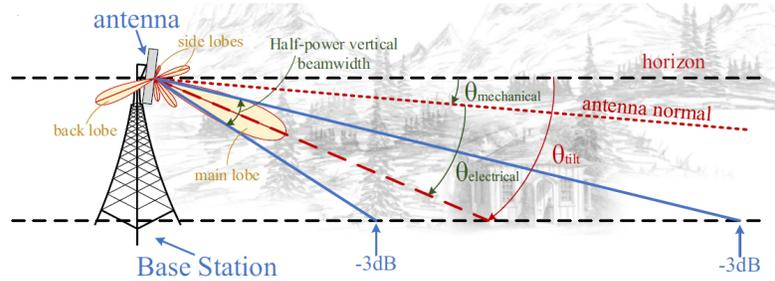
Figure 6.2: Graphical representation of a base station and one of its antenna. The main lobe of the antenna radiation pattern defines the antenna tilt. [7]
