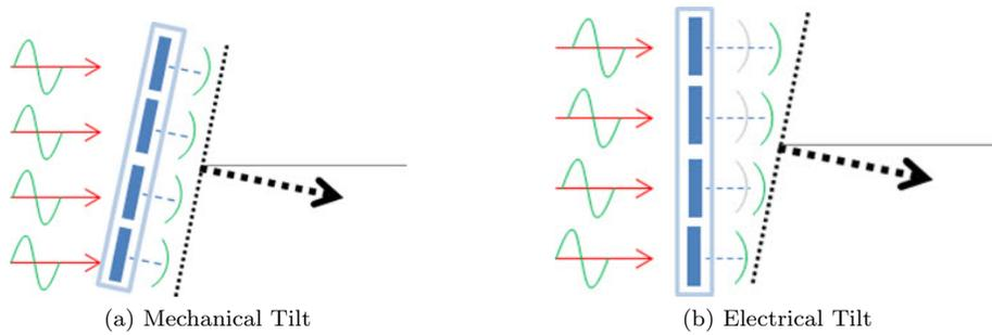
Figure 6.3: Mechanical and electrical tilt modification. In the mechanical tilt the antenna elements are physically modified, while in electrical tilt we act only on the signal phase of the different elements. [Image taken from [telecomHall](#)]
