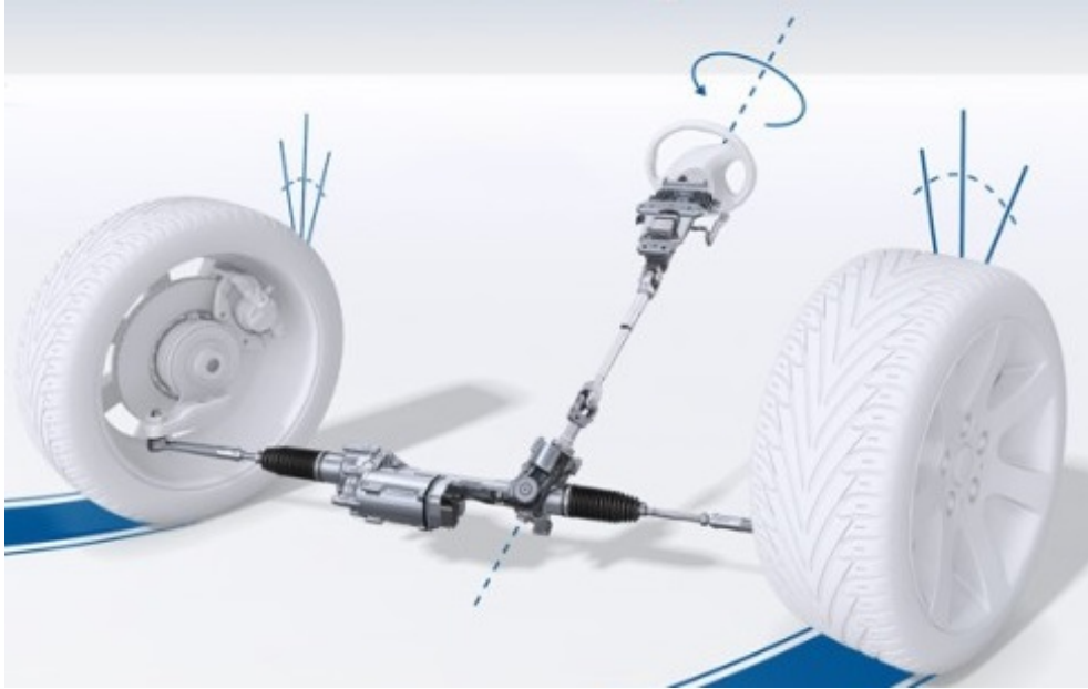
Figure 1.1: EPS from Bosch with recirculating ball drive on the rack [9]
