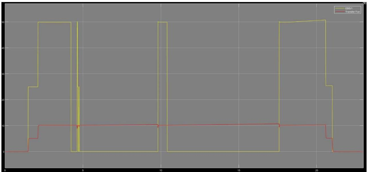
**Figure 76.** Complete simulation: Air (red) and Oil (yellow) mean pressures vs time
