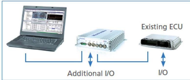
Figure 21. Bypass prototyping [30]
