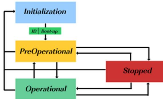
Figure 25. NMT protocol state machine [38]
