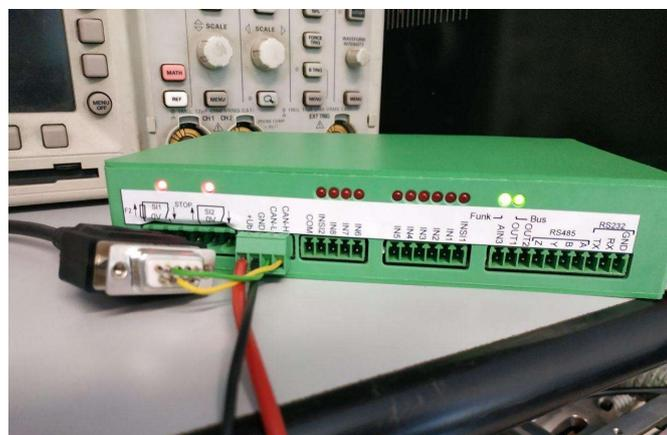
**Figure 33.** RES receiver, cabling, and CAN db9 connector
