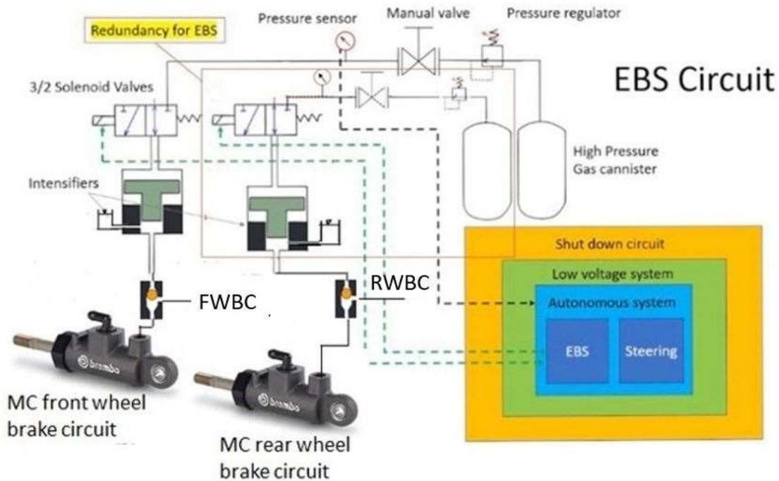
Figure 40. Hydro-pneumatic EBS scheme
