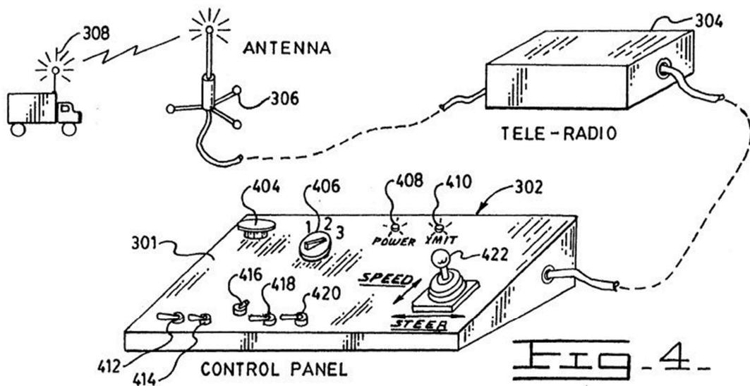
Figure 5. Tele-operation mode of an autonomous vehicle [18]
