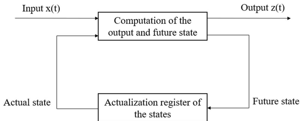
Figure 7. Finite state machine [23]
