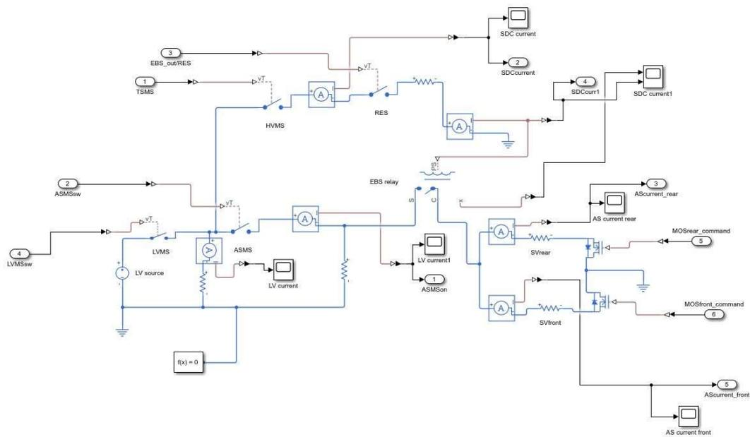
**Figure 68.** Electrical scheme with the two parallel lines
