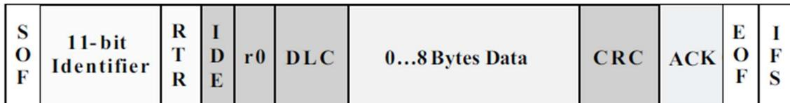
Figure 28. Standard CAN data frame [40]
