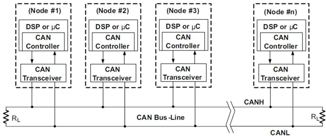
Figure 26. CAN bus physical layer [41]
