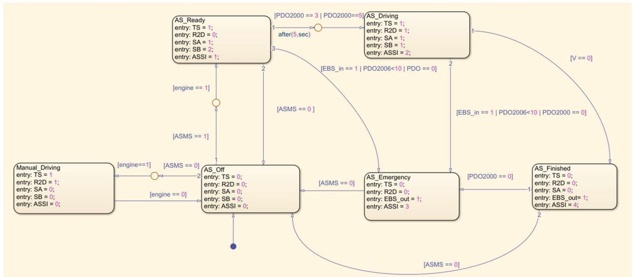
**Figure 52.** Updated AS state machine with RES inputs
