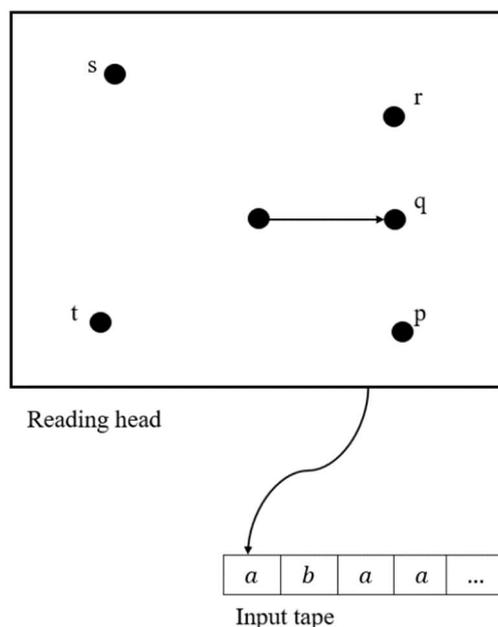
**Figure 8.** Deterministic Finite Automaton example [22]
