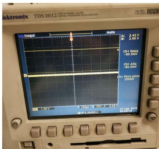
Figure 44. Oscilloscope signal: EBS disarmed (0 V)
