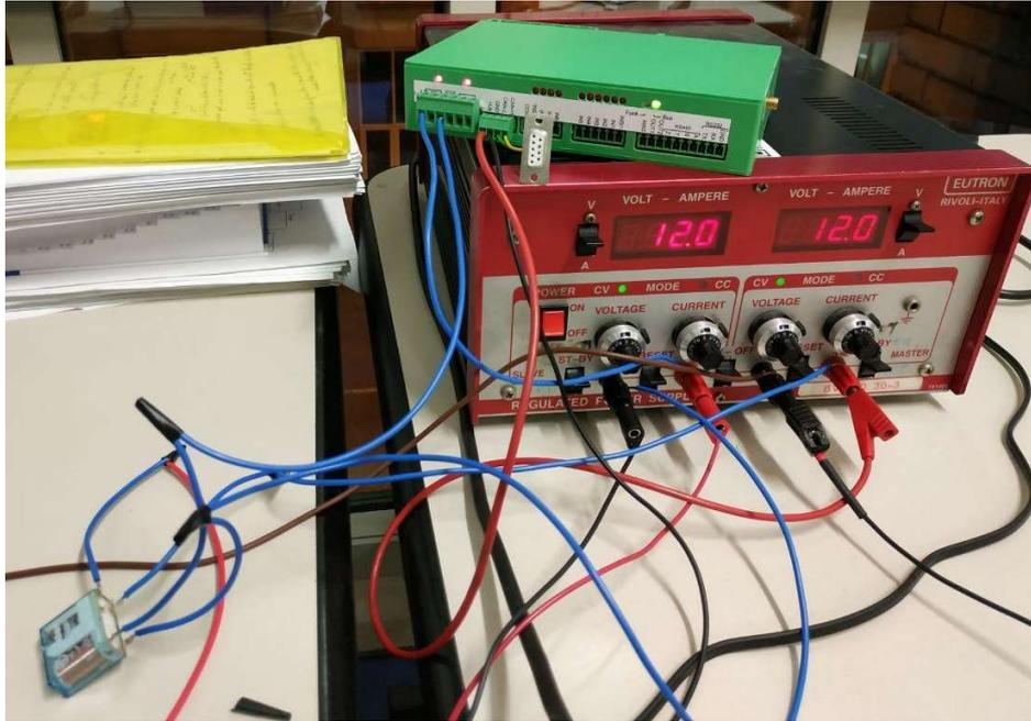
Figure 43. RES and EBS connection through the EBS relay
