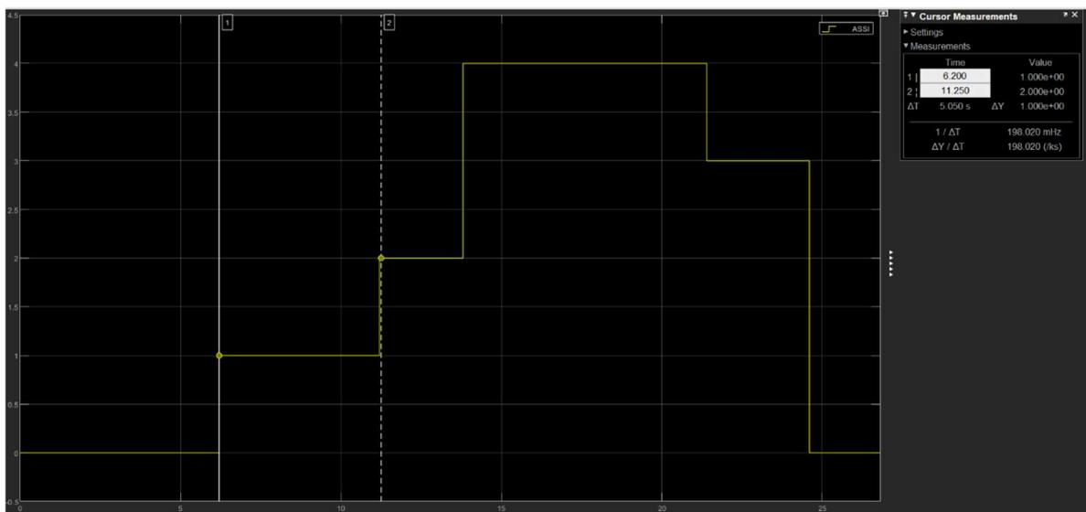
**Figure 50.** Verification of the 5 seconds delay for *AS Driving* transition
