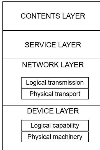
**Figure 3.** Layered Modular Architecture for digital technologies [13]
