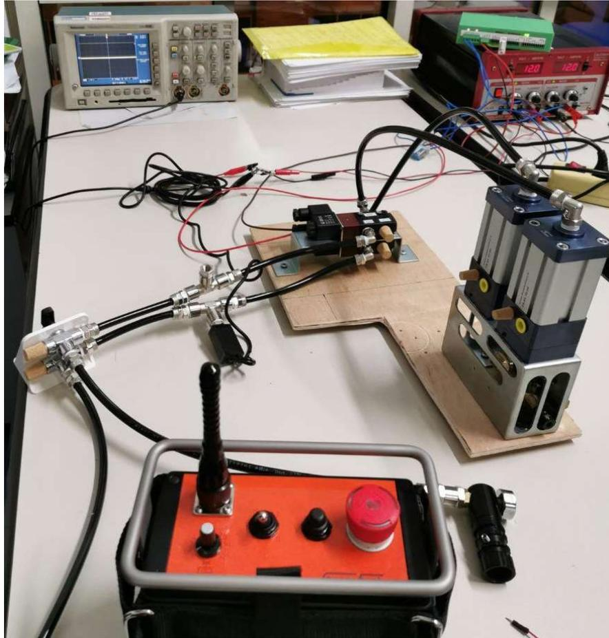
**Figure 42.** EBS and RES test bench
