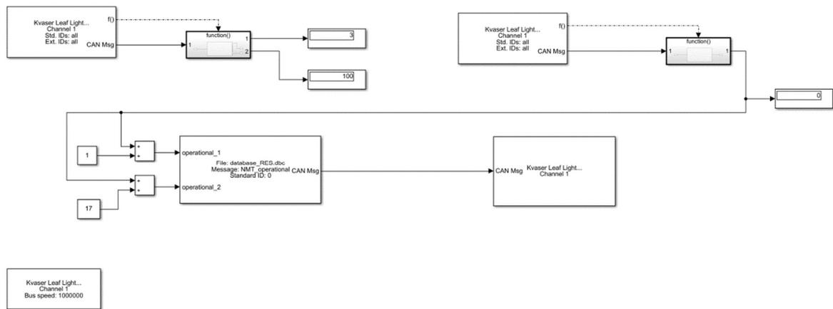
**Figure 39.** Complete RES communication model
