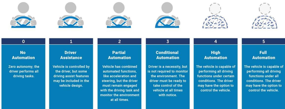
Figure 2. SAE J3016 Levels of Driving Automation [11]
