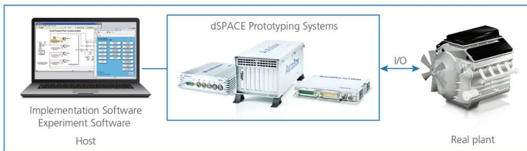
**Figure 20.** Fullpass prototyping [31]
