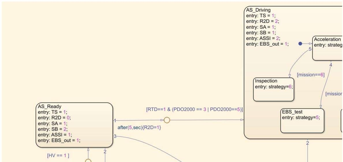
**Figure 69.** Ready-to-drive procedure inside the AS state machine
