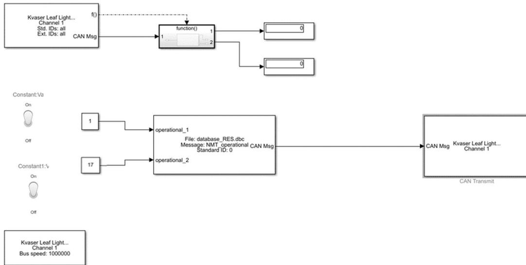
**Figure 38.** NMT transmission and PDO receiving
