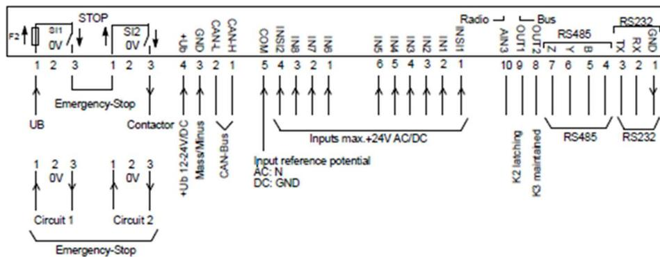
**Figure 24.** Connections at the RES receiver [33]
