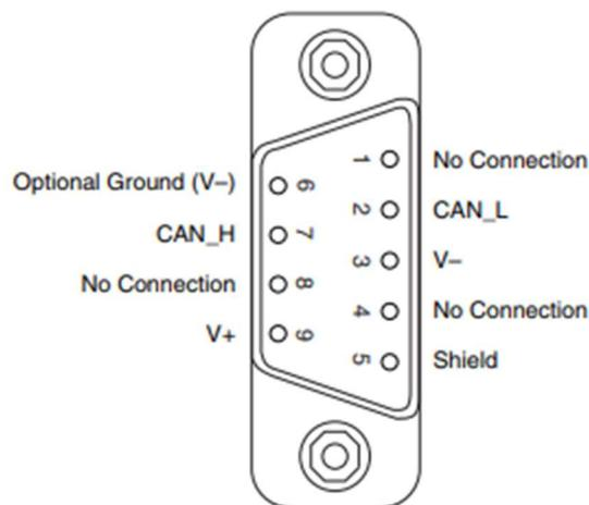
Figure 27. CAN 9-pin D-sub type connector
