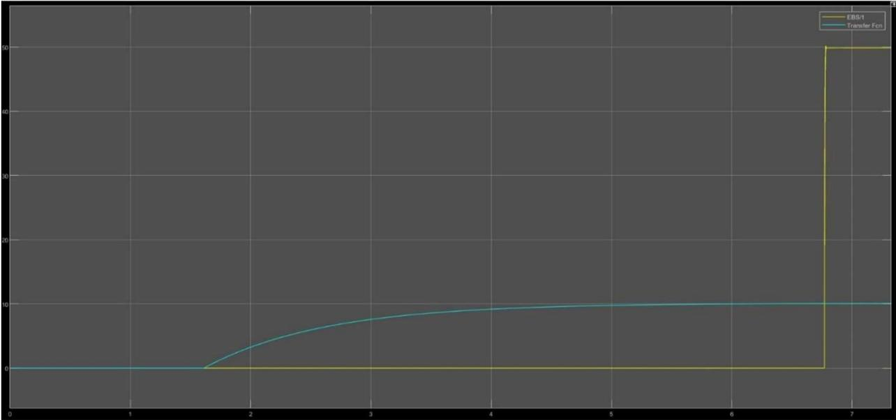
**Figure 60.** EBS simulation: Air (yellow) and Oil (blue) mean pressures vs time
