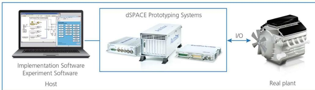
**Figure 20.** Fullpass prototyping [31]
