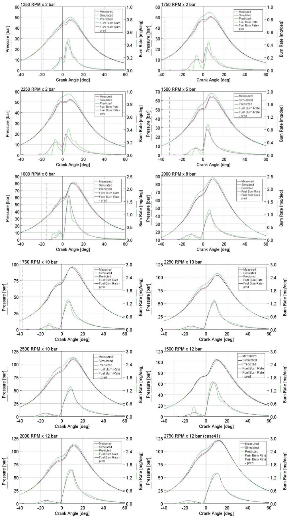
Figure 39: Predicted and Measured cylinder pressure and burn rate as a function of crank angle
