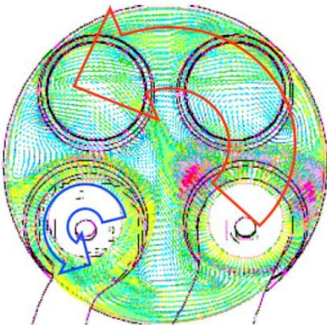
Figure 10: Swirl motion, cylinder top view [11]
