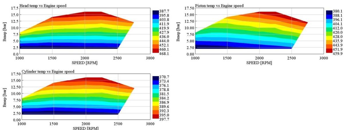
Figure 23: Head, Piston and Cylinder temperature map
