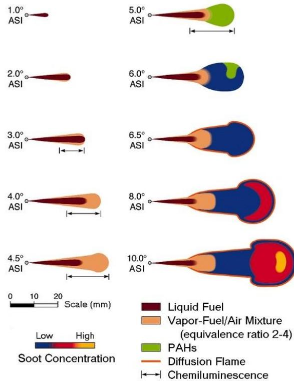
Figure 3: Conceptual model for DI diesel combustion [3]
