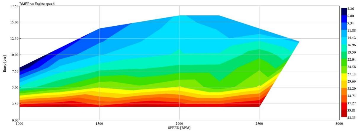
Figure 19: EGR as a function of BMEP and Engine Speed
