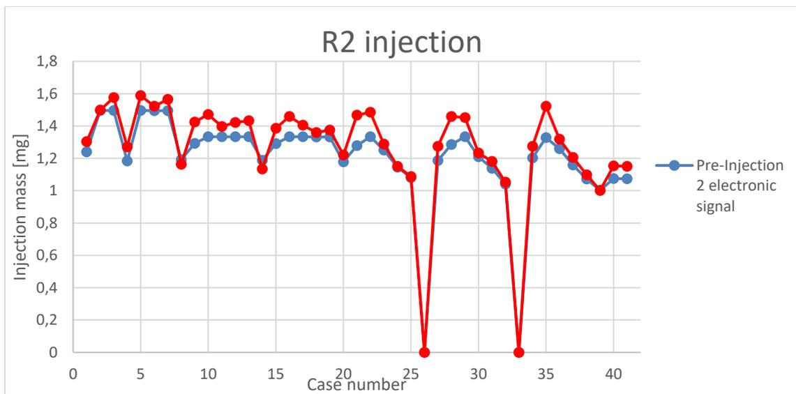
Figure 27: Pre-injection 2 - fuel mass injection
