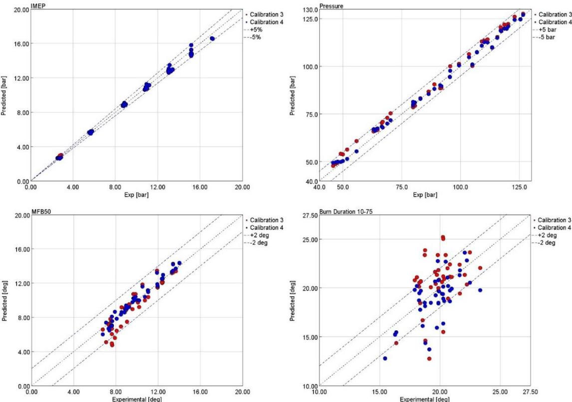
Figure 49: IMEP, maximum pressure, MFB50 and Burn duration 10-75. Predicted vs experimental data, comparison of 3rd and 4th calibration
