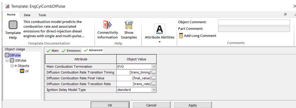
Figure 16: Diffusion combustion advanced parameters
