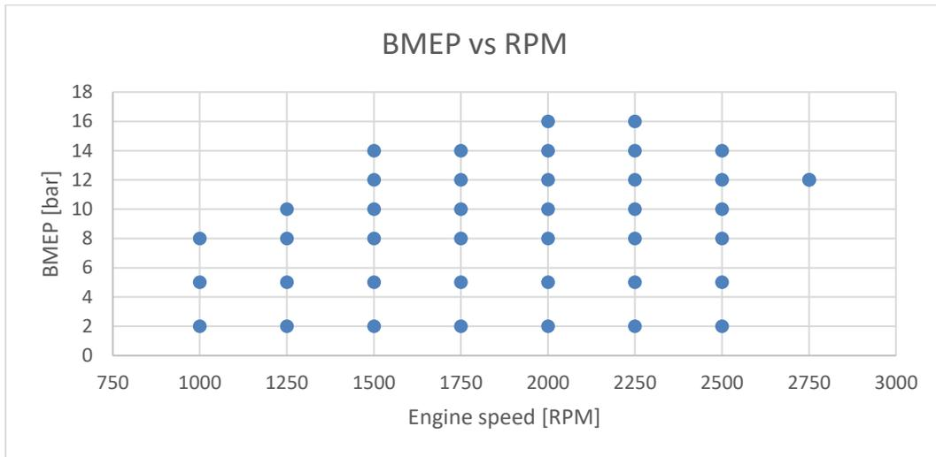
Figure 20: BMEP vs Engine speed for 41 operating points
