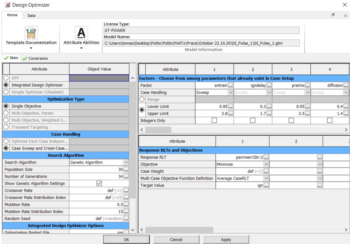
Figure 18: Optimizer setup
