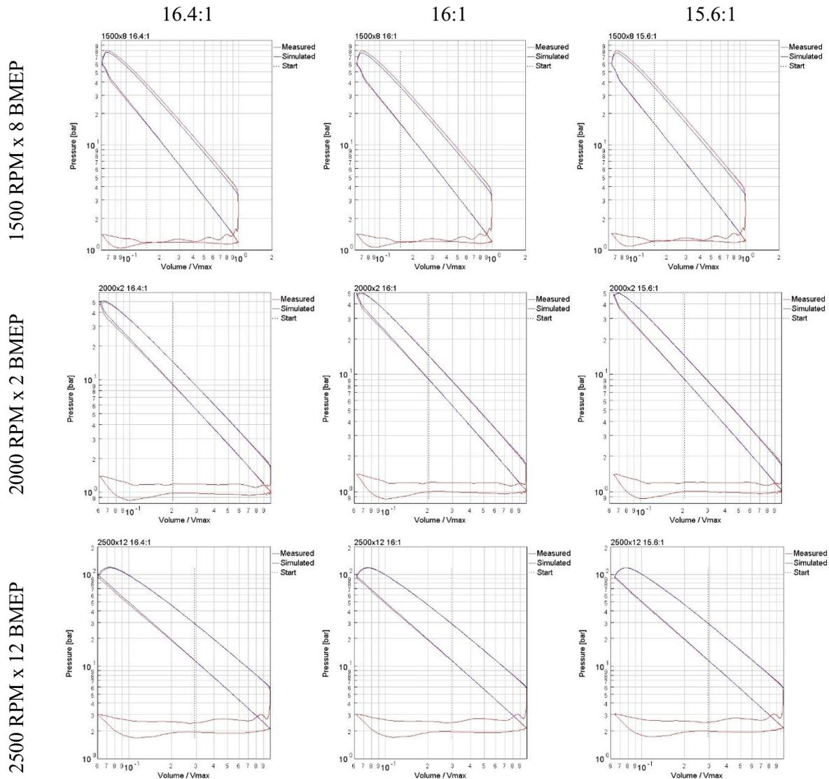
Figure 24: LogP vs LogV diagram for 3 operating points and 3 different compression ratios
