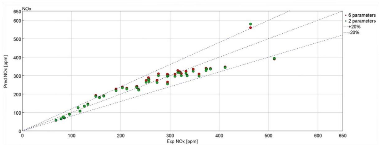
Figure 52: NOx validation, comparison of 2 and 6 parameters model
