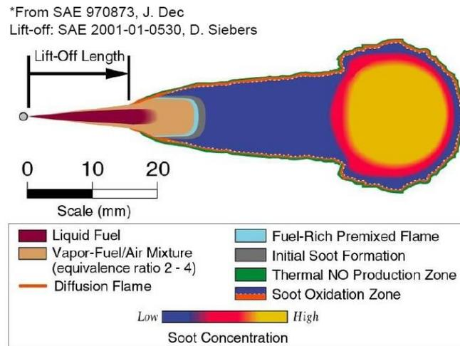
Figure 4: Mixing controlled burn schematics [3]
