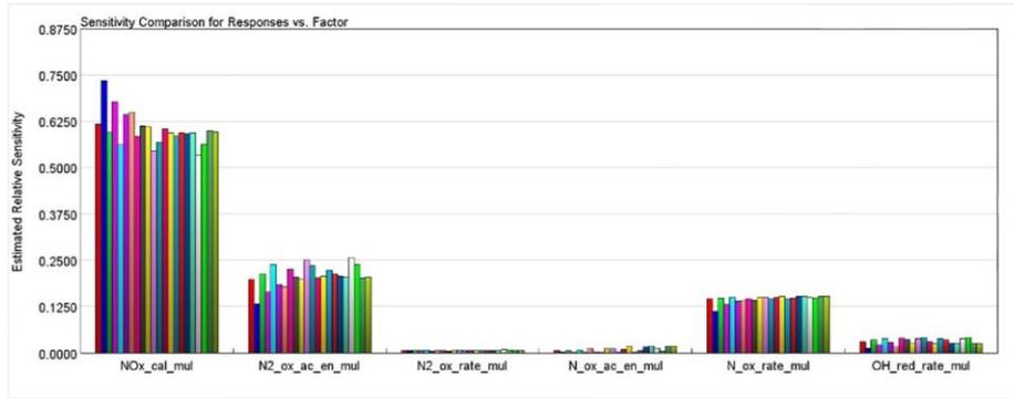
Figure 51: NOx optimization parameters, sensitivity.
