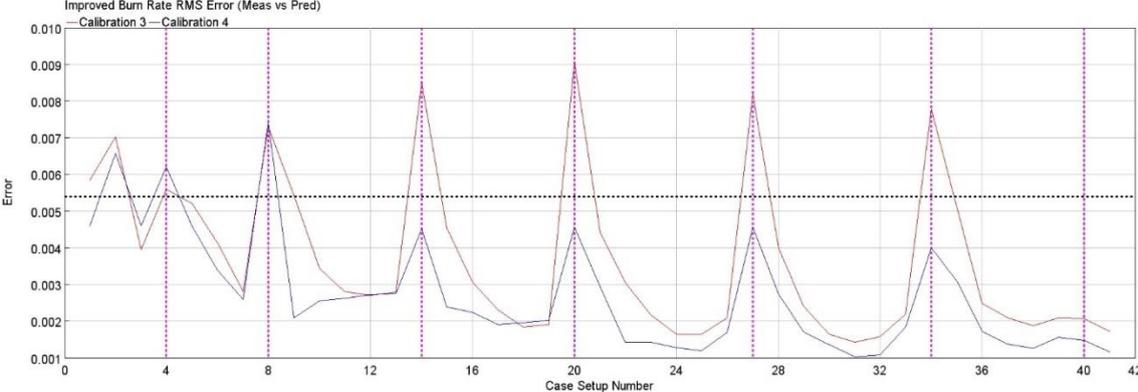
Figure 48: Improved Burn Rate RMS Error, comparison of calibration 3 and 4
