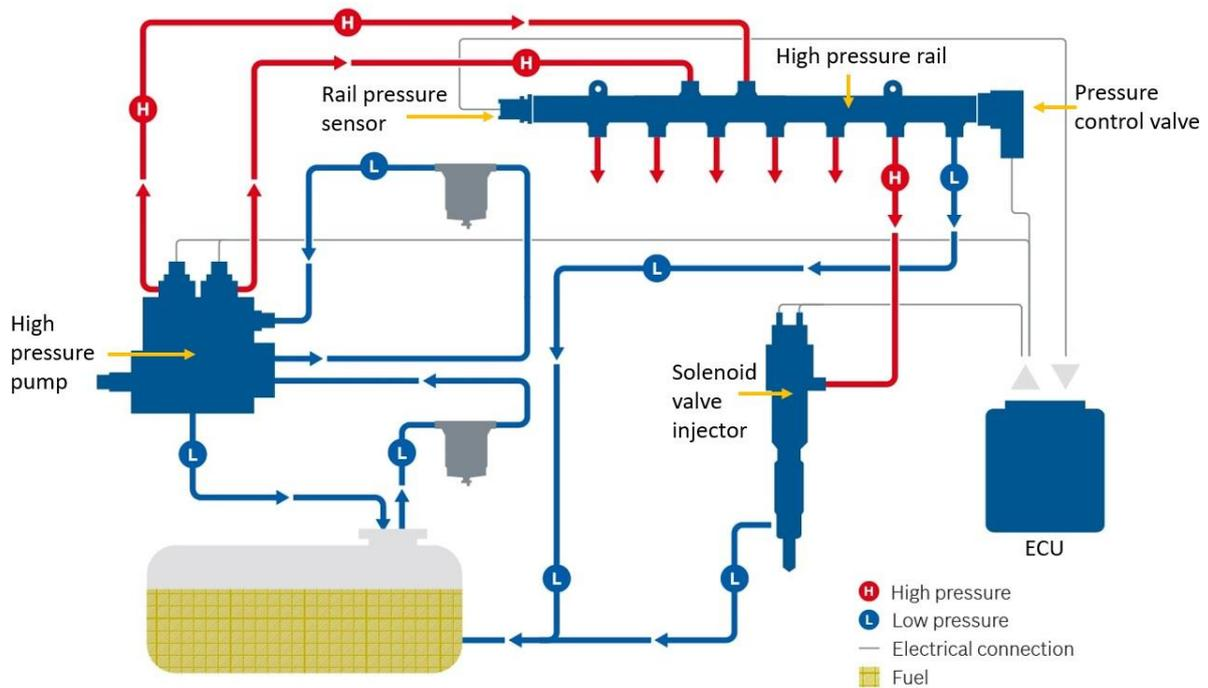
Figure 8: Common rail system schematics [6]
