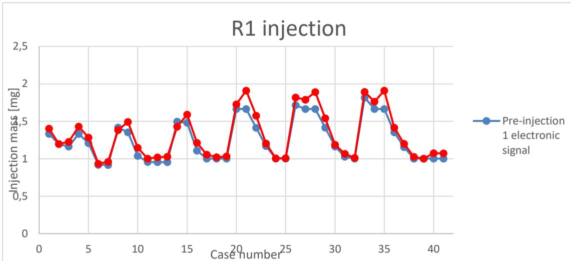
Figure 26: Pre-injection 1 - fuel mass injection
