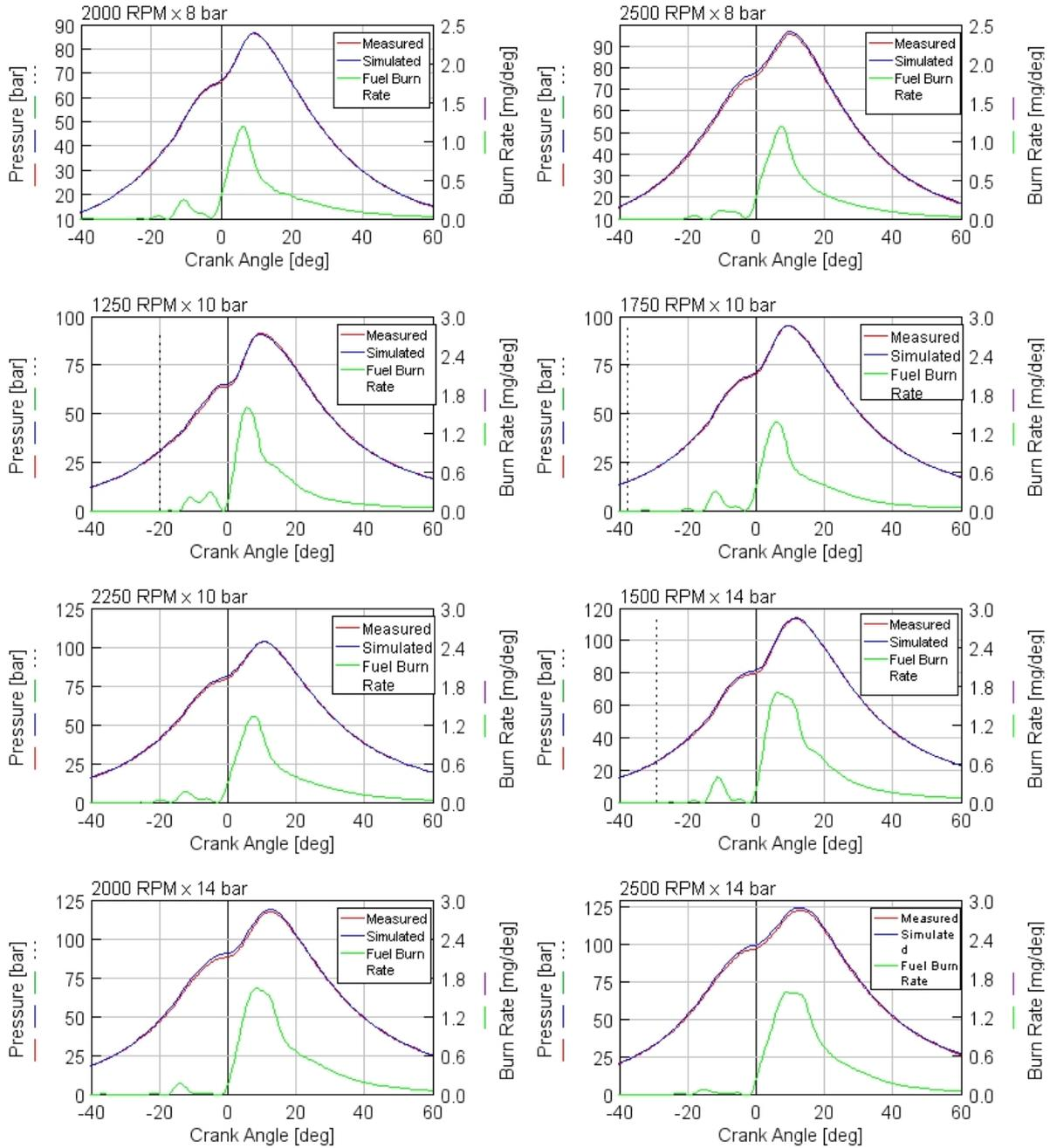
Figure 34: Figures of simulated and measured cylinder pressure, and burn rate as results of CPOA analysis
