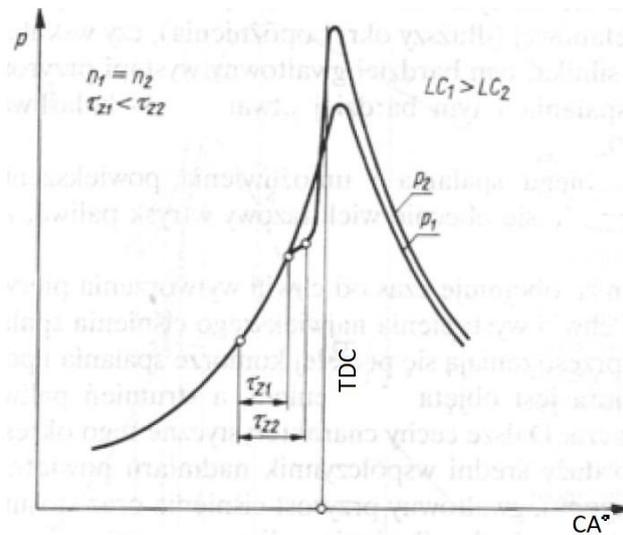
Figure 2: Ignition delay influence on combustion process [2]
