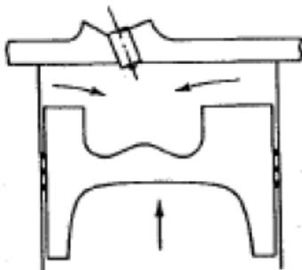
Radially inward gas motion that occurs towards the end of the compression stroke thanks to the generation of different local compression ratios. During compression stroke air is forced to the center of the cylinder, while during the expansion stroke the gases are dragged towards the cylinder walls. Squish is maximal at TDC when other cylinder motions are limited.
