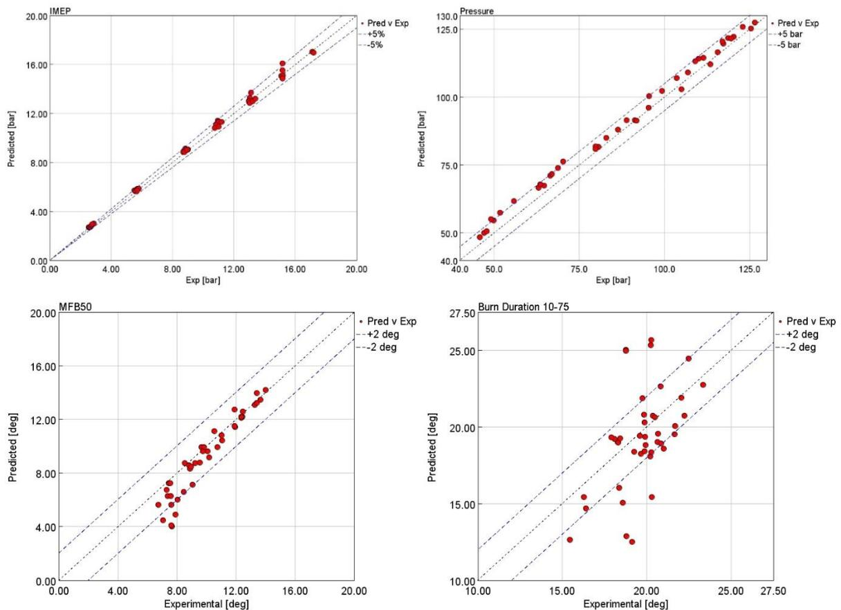
Figure 38: IMEP, maximum pressure, MFB50 and Burn duration 10-75. Predicted vs experimental data for the 1st calibration
