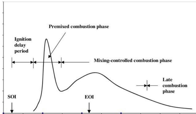
Figure 1: Combustion process in Diesel engine [1]
