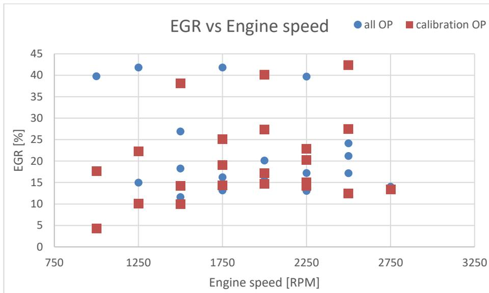
Figure 36: Operating points used for DI Pulse analysis represented on EGR vs RPM map
