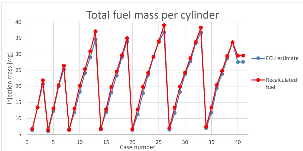
Figure 25: Mass of fuel injected to the cylinder, recalculated vs ECU estimate
