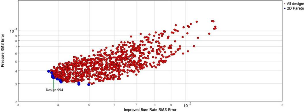
Figure 43: The results of the multi-objective optimization with 7 parameters Calibration 3. Pareto points
