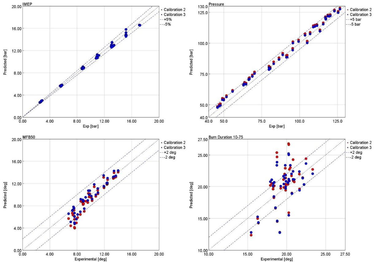
Figure 45: IMEP, maximum pressure, MFB50 and Burn duration 10-75. Predicted vs experimental data, comparison of 2nd and 3rd calibration
