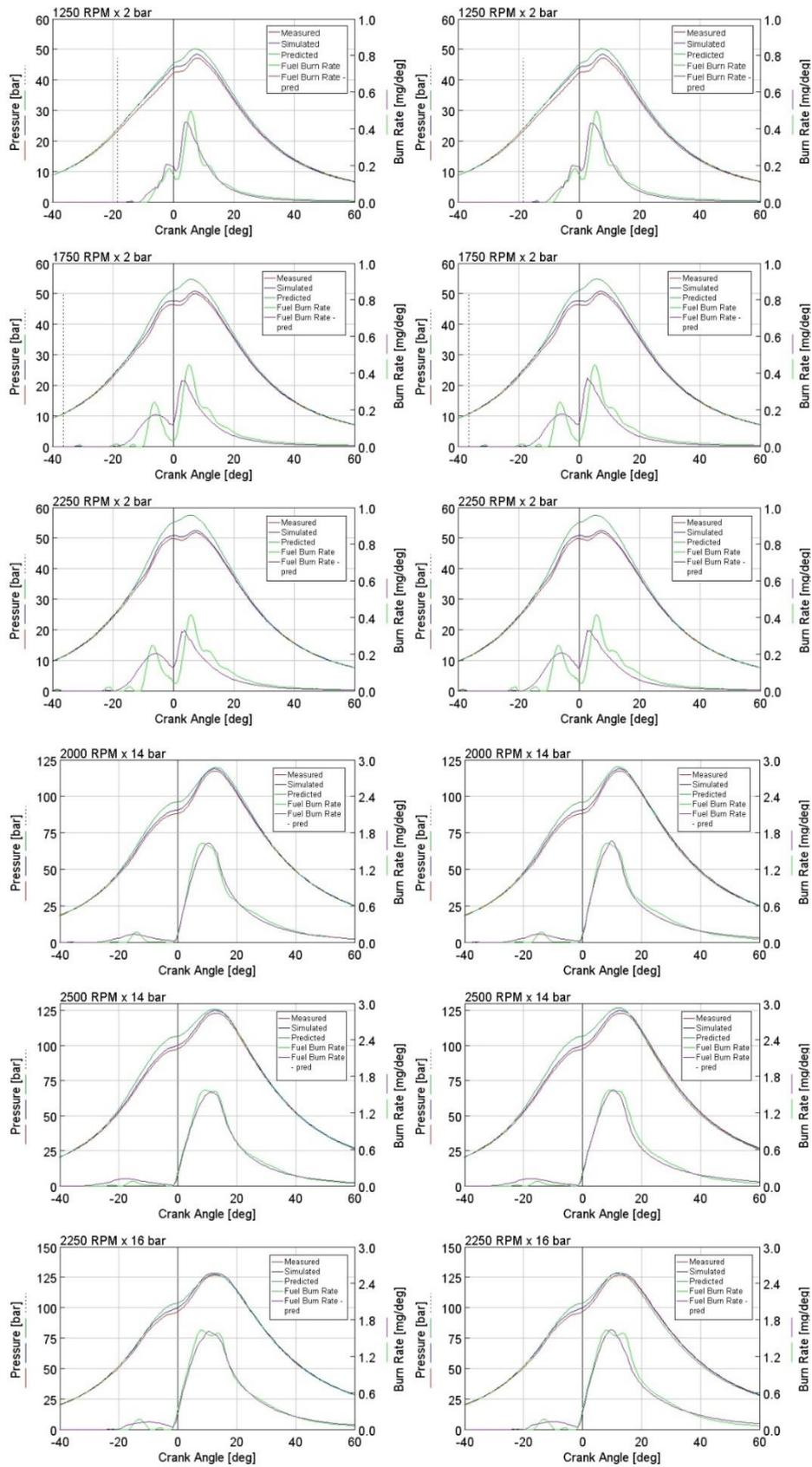
Figure 42: Predicted and Measured cylinder pressure and burn rate as a function of crank angle. Left hand side: calibration 1, right hand side: calibration 2.
