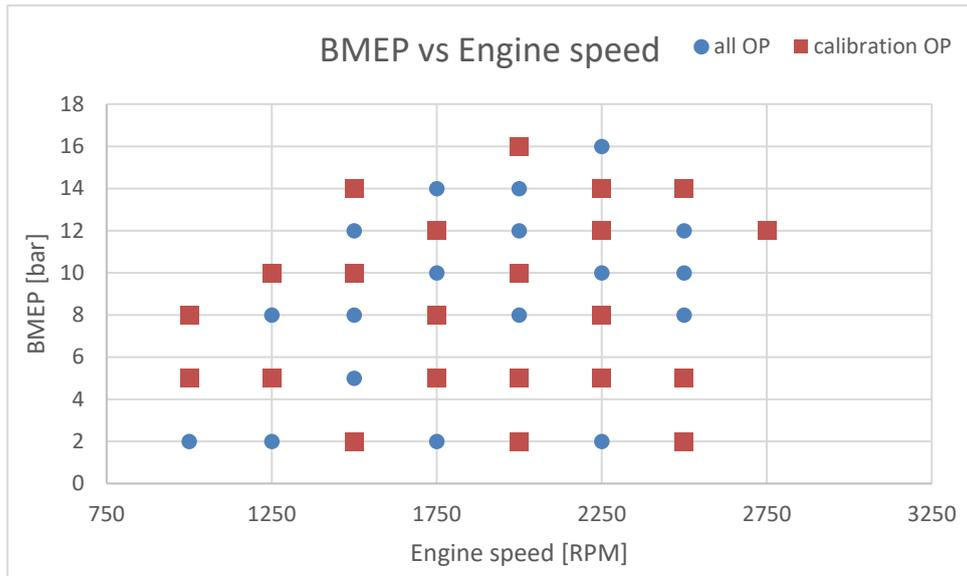
Figure 35: Operating points used for DI Pulse analysis represented on BMEP vs RPM map
