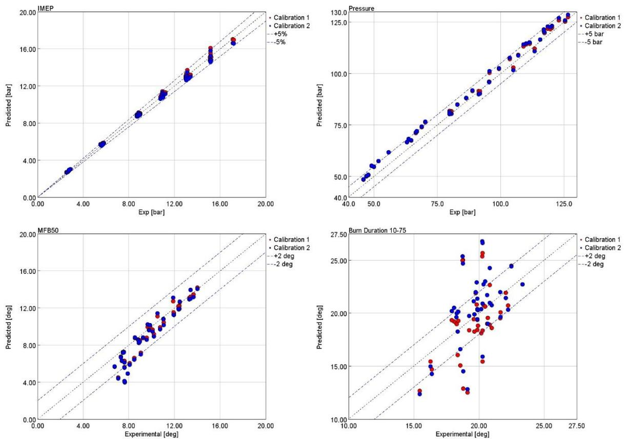
Figure 41: IMEP, maximum pressure, MFB50 and Burn duration 10-75. Predicted vs experimental, comparison of 1st and 2nd calibration
