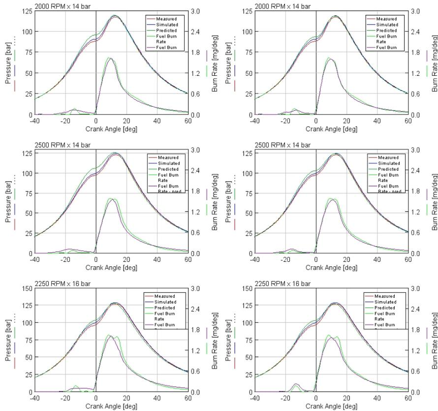
Figure 50: Predicted and Measured cylinder pressure and burn rate as a function of crank angle.
