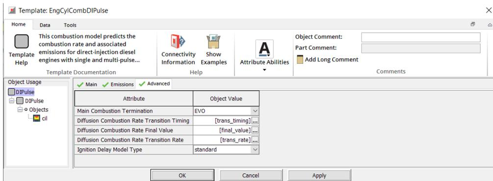
Figure 16: Diffusion combustion advanced parameters
