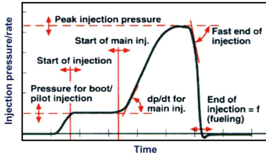
Figure 7: Injection rate shaping [5]
