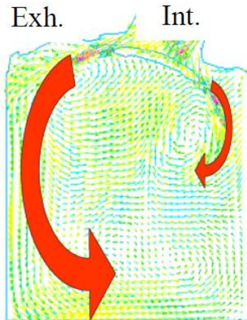
Rotation motion about an axis that is perpendicular to that of the cylinder. Tumble is generated during intake and then amplified during compression stroke. Towards the TDC tumble is converted into turbulence energy at small scales. It is obtained through intake duct shaping.
