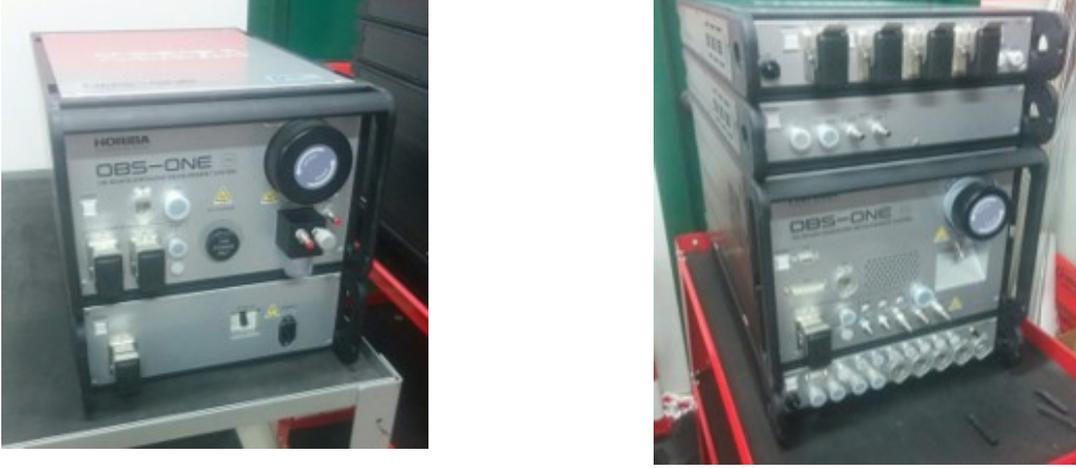
Figure 3.1: The PEMS modules. From left image to the right one, from top to bottom: PN, PS, PE, PF, GA, and CC.
