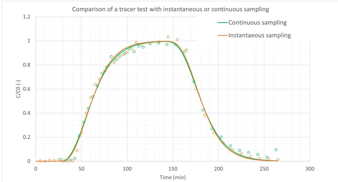
**Figure 4.22.** Lysimeter scale, maximum flow rate tracer tests with the two different sampling methods. Sampling depth: column's exit (70 cm).
