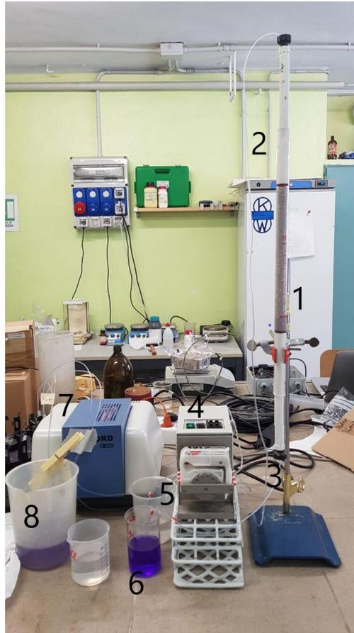
**Figure 3.4.** Small scale tests set-up. 1: column; 2: in-flow; 3: out-flow; 4: 4-channels peristaltic pump; 5: solution for the test; 6:  $C_0$  tank; 7: spectrophotometer; 8: waste tank.
