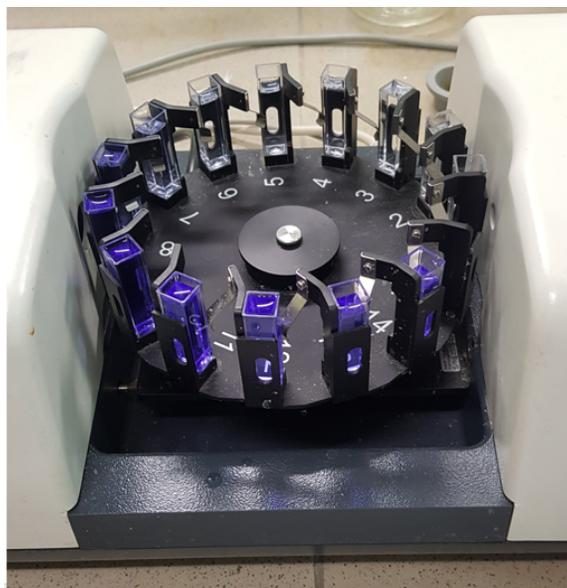
**Figure 3.2.** Spectrophotometer carousel with bromophenol blue samples.
