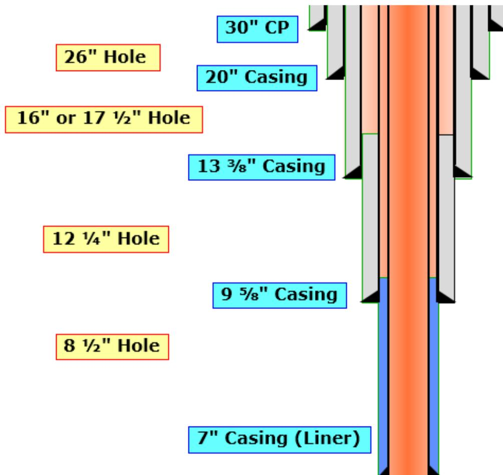
Figure 2.20: Standard casing profile [21]
