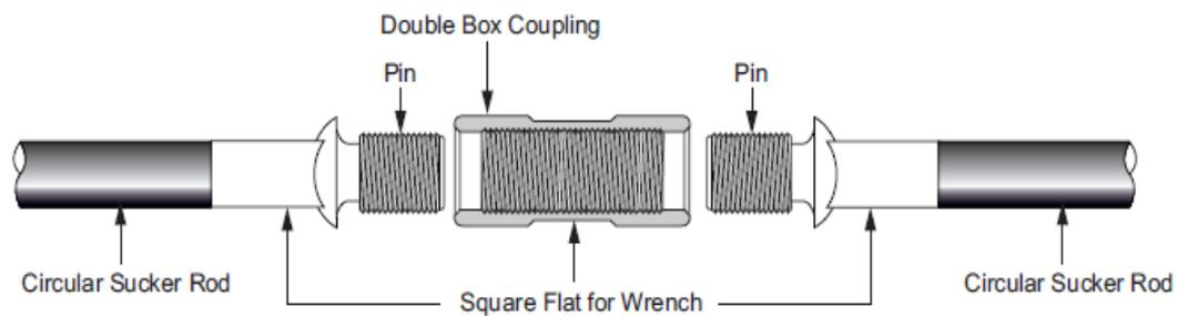
**Figure 4.5:** Sucker rods are joined together by a coupling [34]
