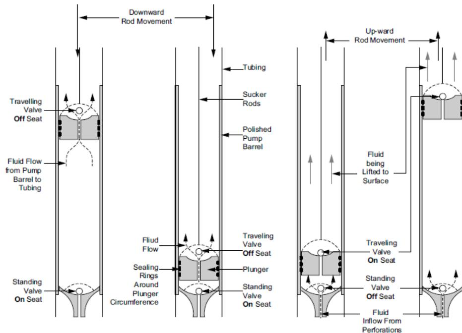
**Figure 4.6:** Operation of rod pump [34]
