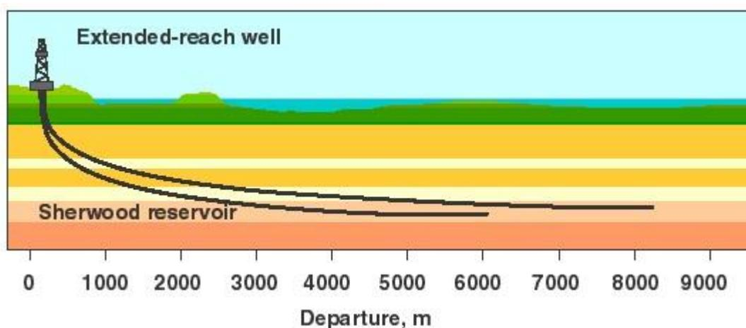
**Figure 3.23:** ERD (adapted from Schlumberger, 2020)
