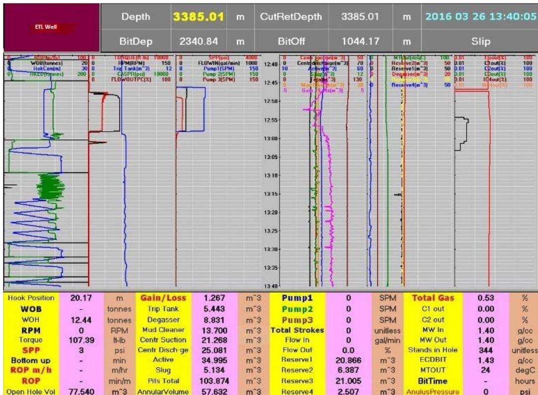
Figure 2.17: Example of a mud logging monitoring screen (Courtesy of ETL)
