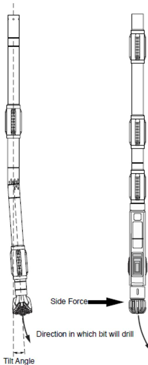
**Figure 3.3:** Bit tilt angle and sideforce [25]
