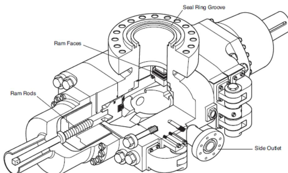
**Figure 2.12:** Ram type preventer (Courtesy of Hydril)
