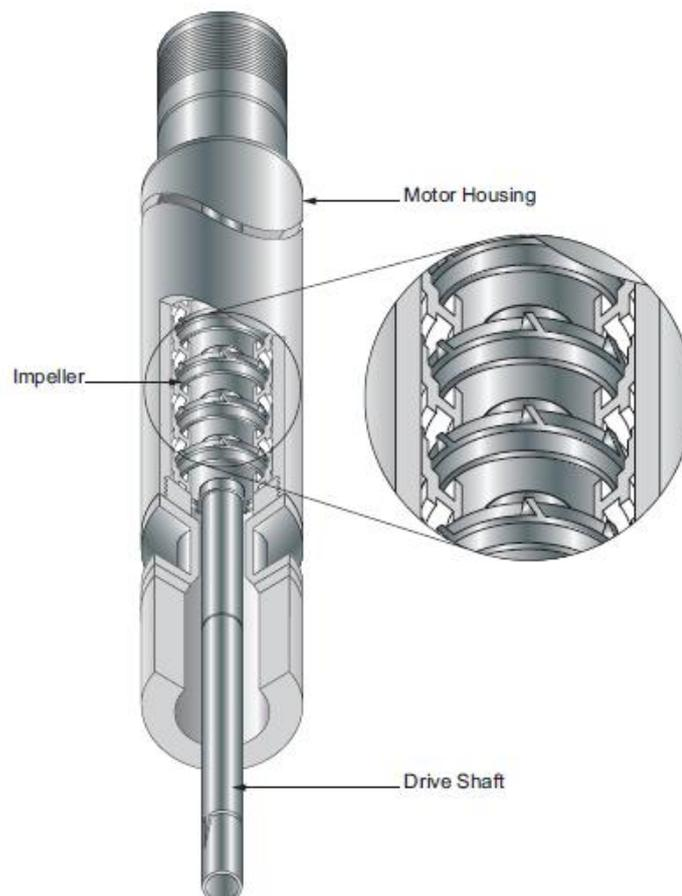
**Figure 4.11:** Cutaway schematic drawing of ESP [34]
