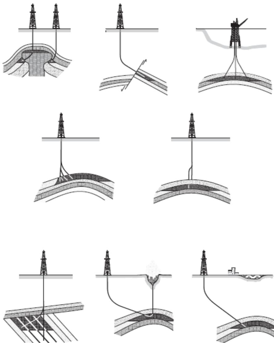
**Figure 3.1:** Applications of directional drilling [7]
