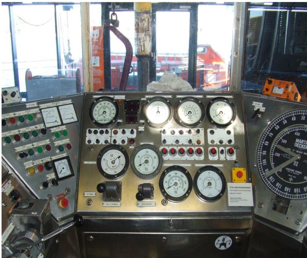
**Figure 2.14:** Driller's control unit
