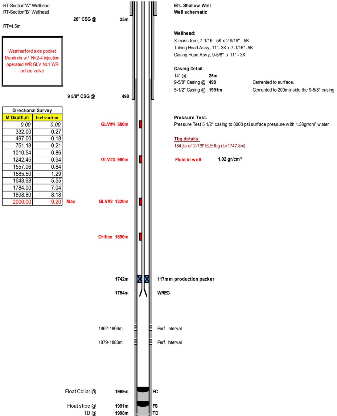
**Figure 2.23:** Typical gas lift completion (Courtesy of ETL)
