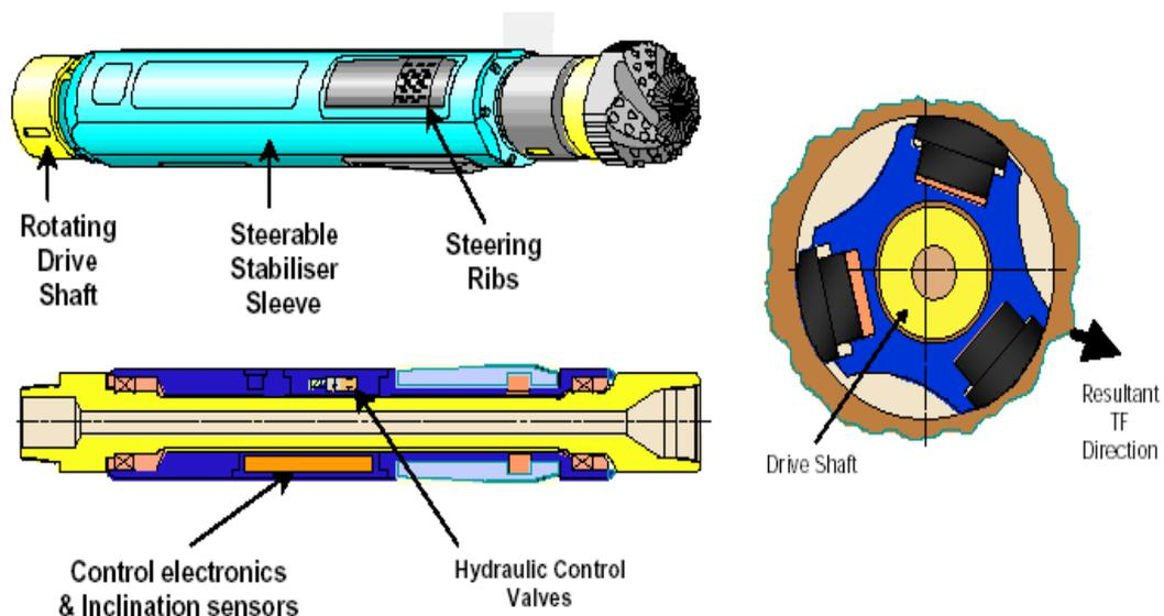
**Figure 3.9:** Non-rotating steerable stabilizer
