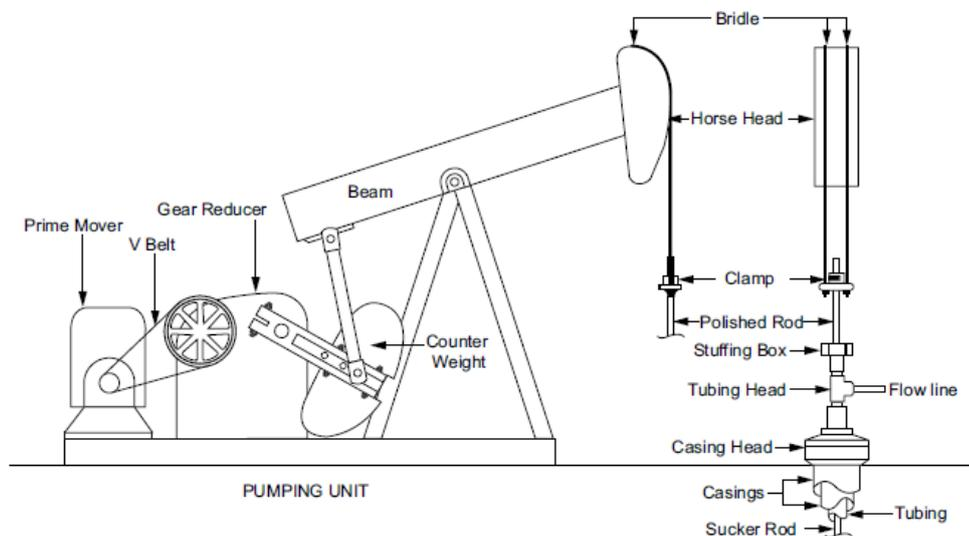
**Figure 4.4:** The surface equipment for a rod pump
