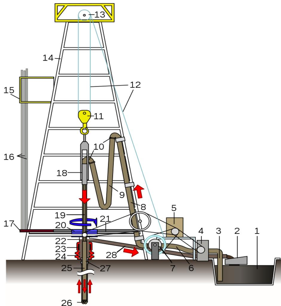
Figure 2.6: Simple diagram of a drilling rig
