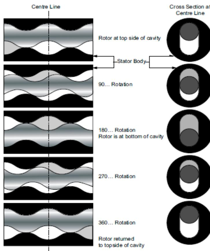
**Figure 4.15:** Operating principle of PCP [34]
