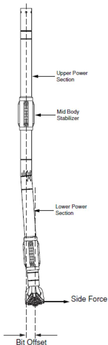
**Figure 3.7:** Steerable drilling system [25]
