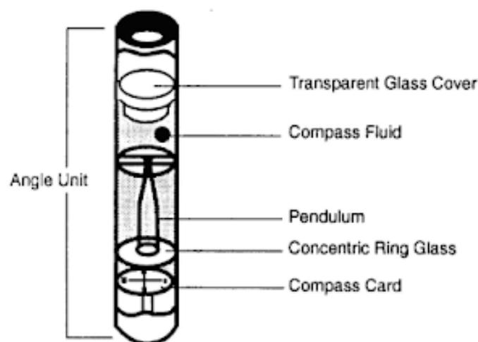
**Figure 3.11:** Angle unit of the tool [25]
