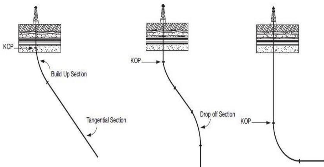
**Figure 3.2:** Standard well trajectories [7]
