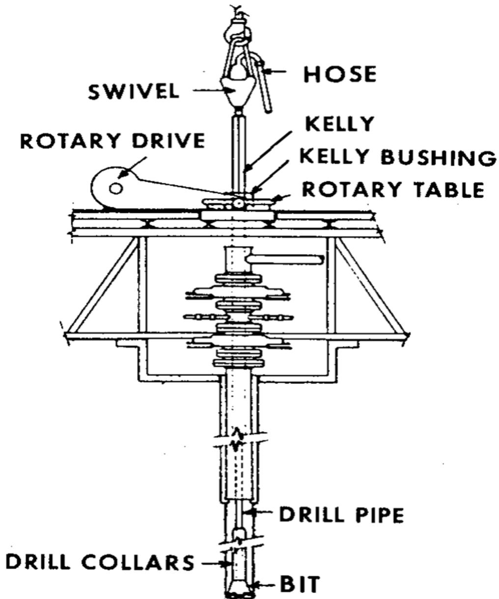
Figure 2.10: Schematic representation of the rotary system [15]
