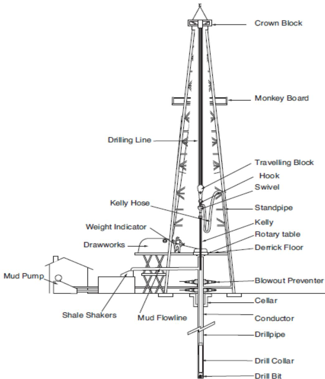
**Figure 2.5:** Rotary drilling rig [7]
