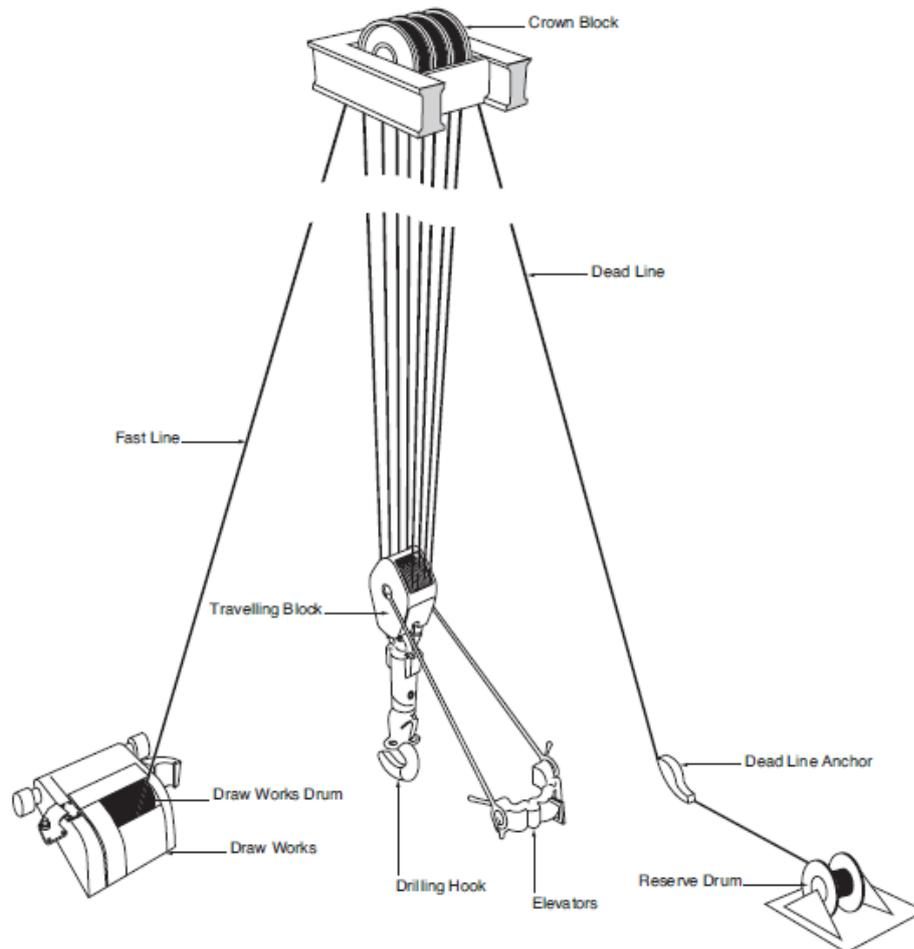
**Figure 2.8:** Schematic representation of rig hoisting system [7]
