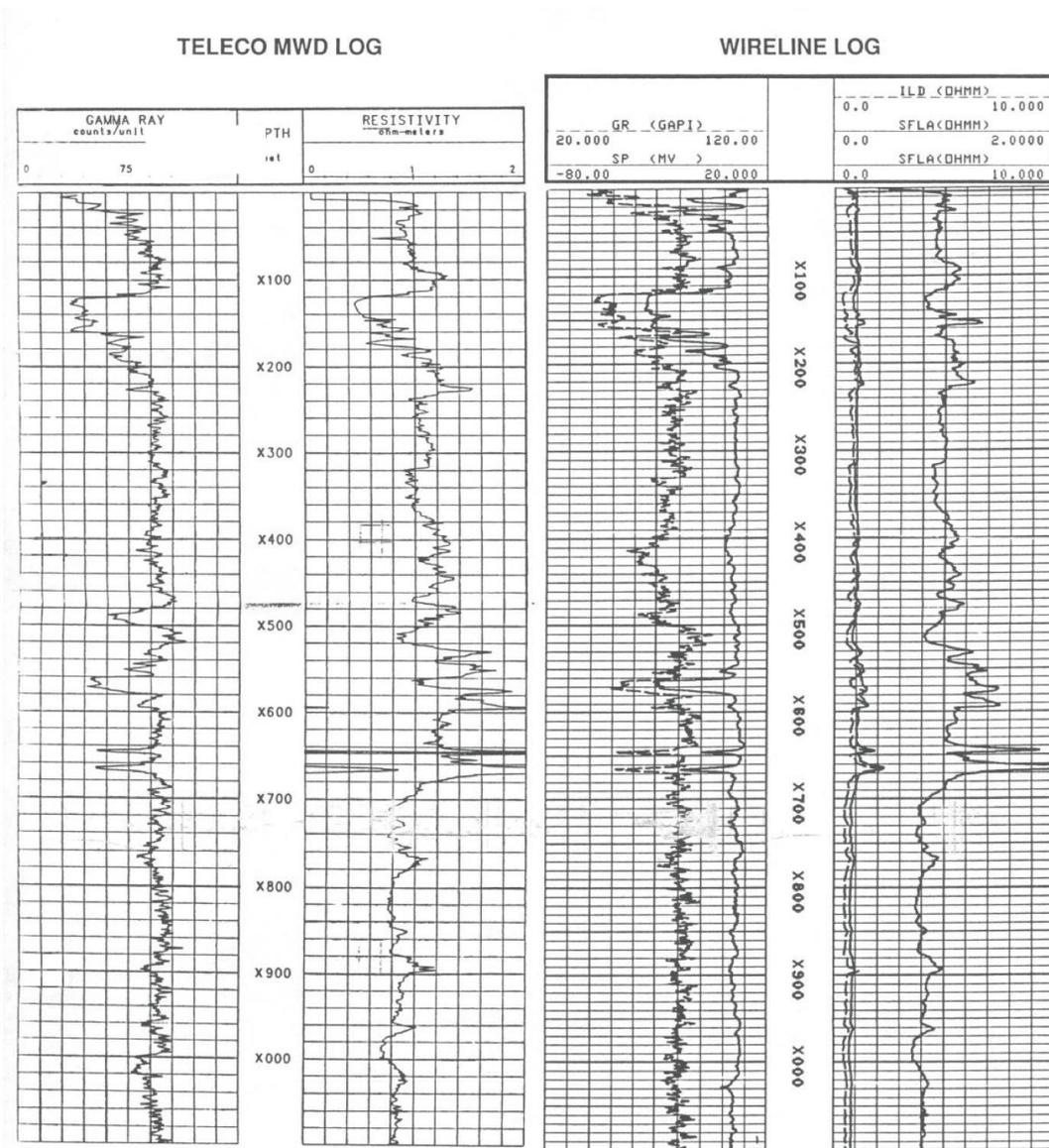
**Figure 3.21:** Comparison of MWD and wireline log [30]
