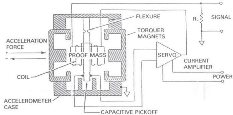
**Figure 3.19:** Accelerometer [7]
