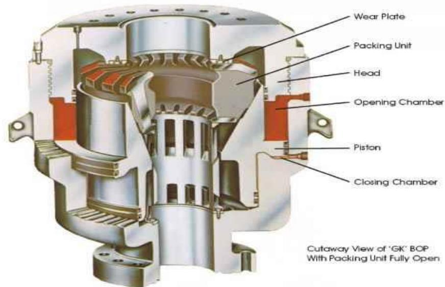
**Figure 2.11:** Annular preventer (Courtesy of Hydril)
