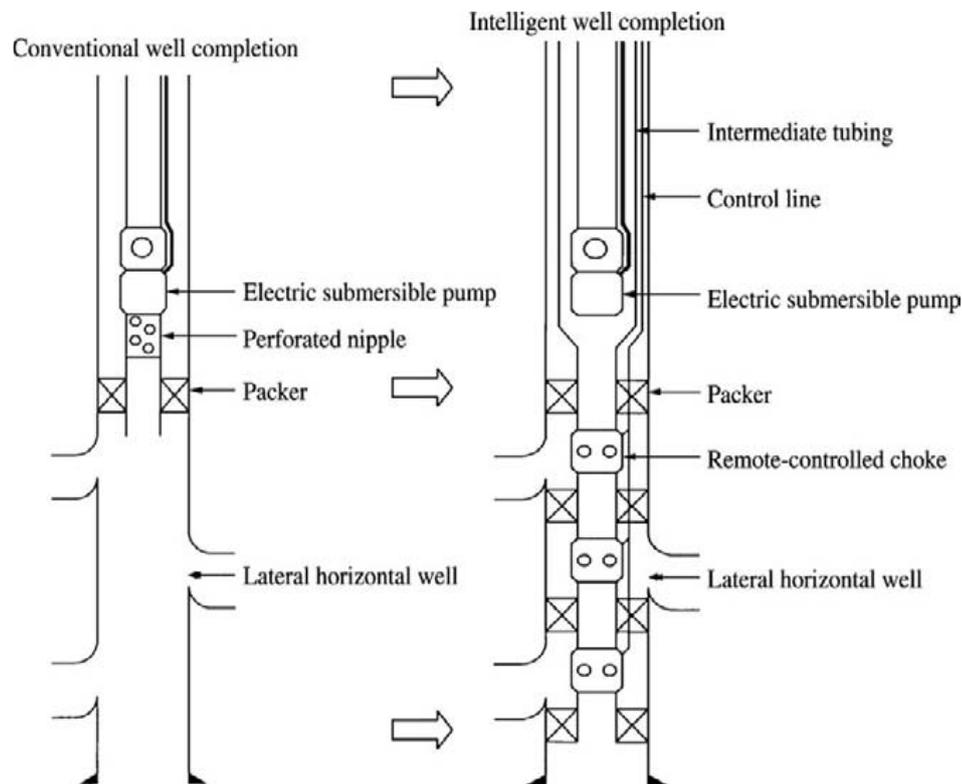
**Figure 4.1:** Hole structures of conventional and intelligent well completions [33]
