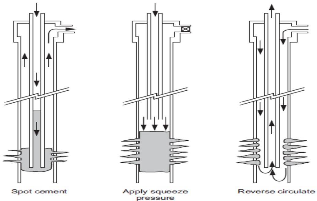
Figure 2.22: Example of secondary or squeeze cementing operation [7]
