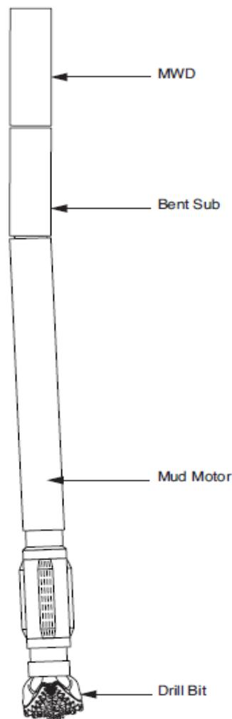
**Figure 3.6:** BHA with bent sub and PDM [7]
