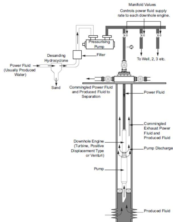
Figure 4.7: Principals of hydraulic lift operation. Turbine pump is illustrated [34]
