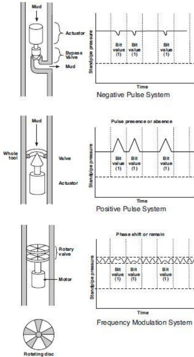
**Figure 3.18:** Mud pulse telemetry systems [25]
