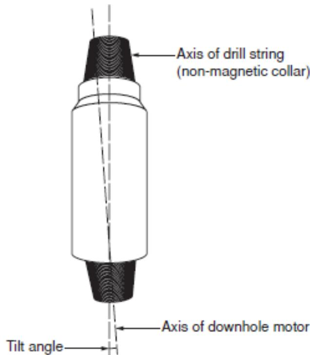
**Figure 3.5:** Directional drilling bent sub [25]
