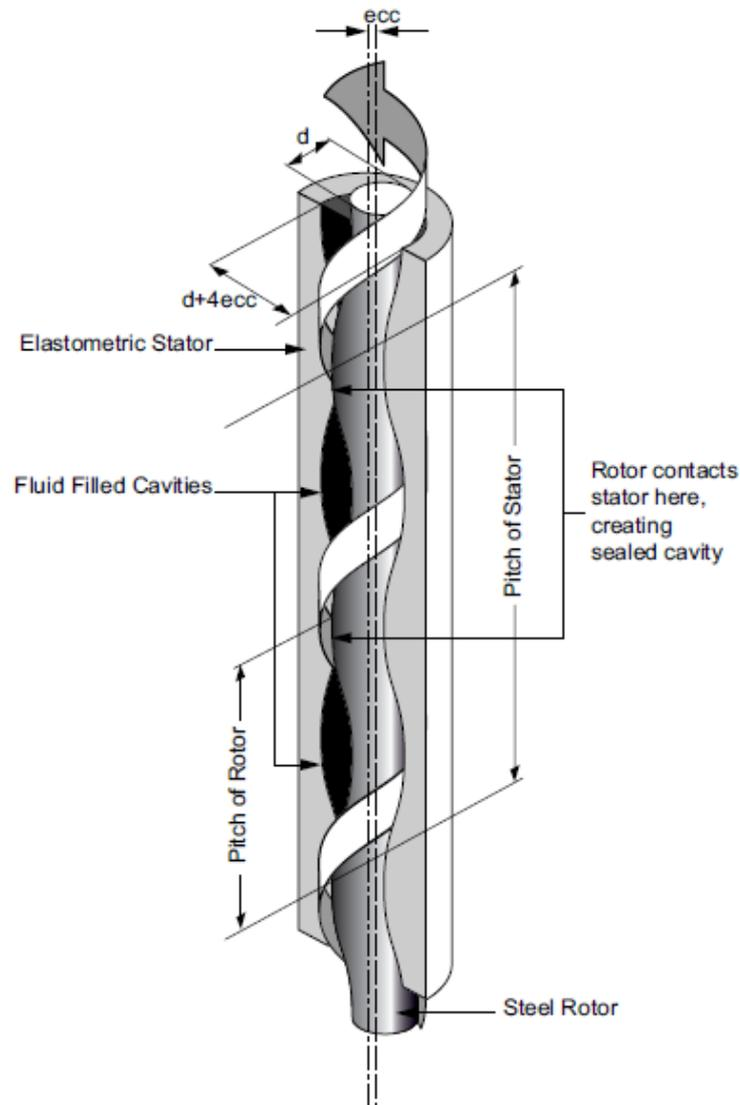
**Figure 4.14:** Perspective view of operating PCP [34]
