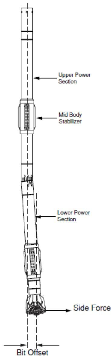
**Figure 3.7:** Steerable drilling system [25]
