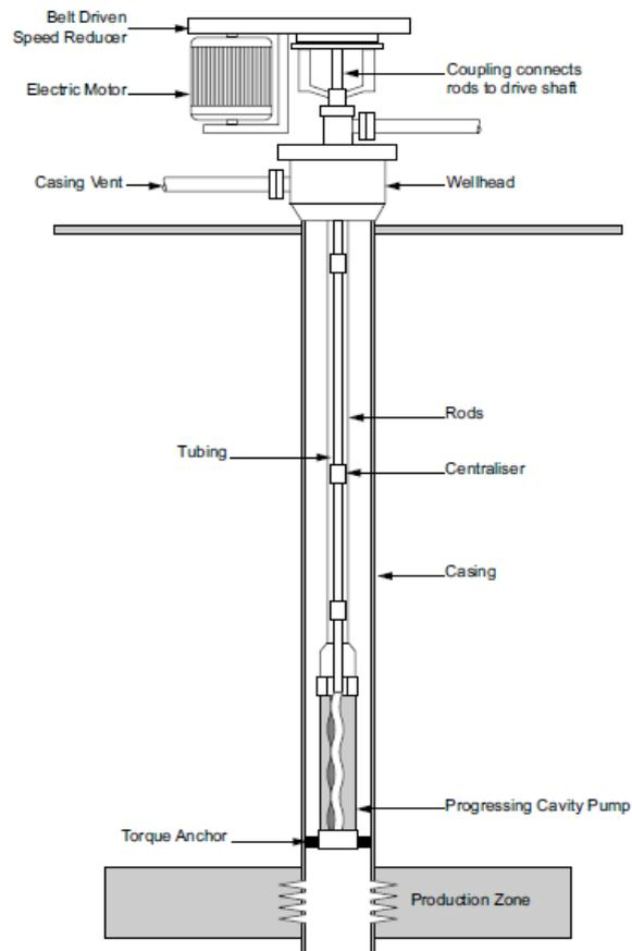
**Figure 4.12:** A well completed with artificial lift using a PCP [34]
