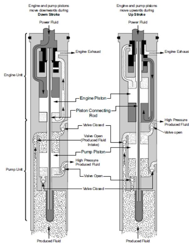
Figure 4.8: Operation of positive displacement hydraulic pump [34]
