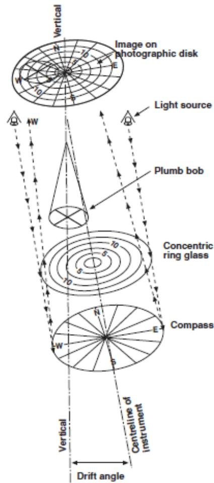
Figure 3.13: Diagrammatic view of magnetic single shot device [29]
