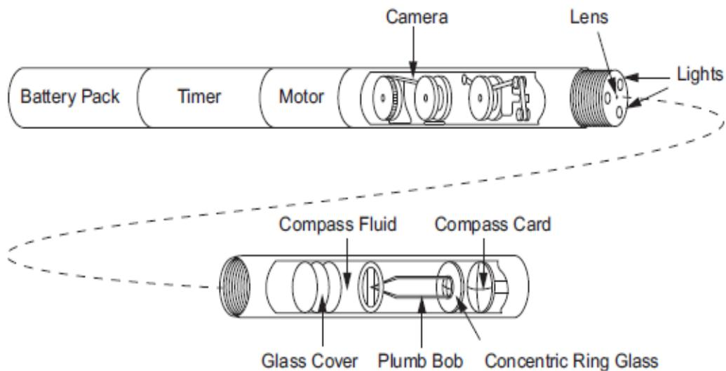
**Figure 3.15:** Magnetic multi-shot instrument [25]
