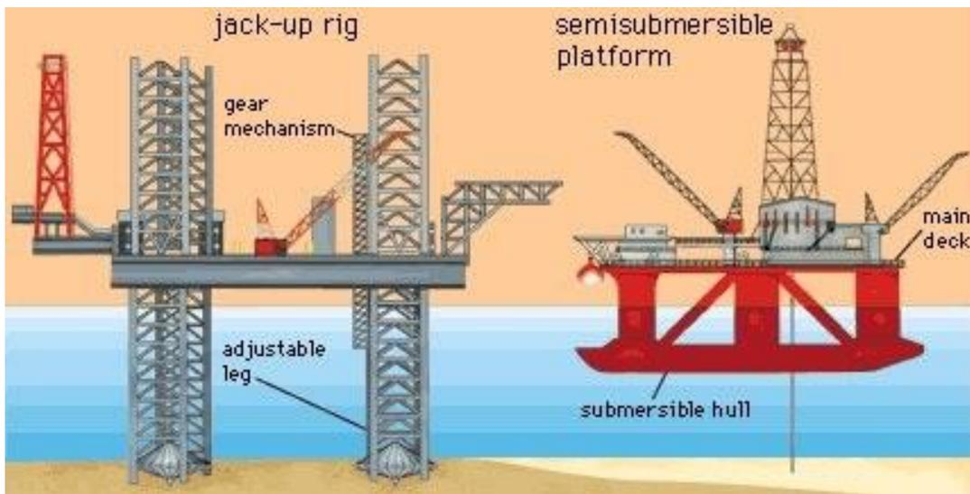
**Figure 2.18:** Jack-up and semisubmersible drilling rigs [20]
