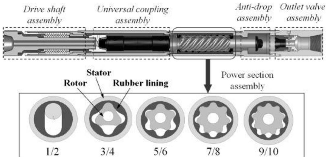
**Figure 3.4:** Bent sub and positive displacement motor [25]
