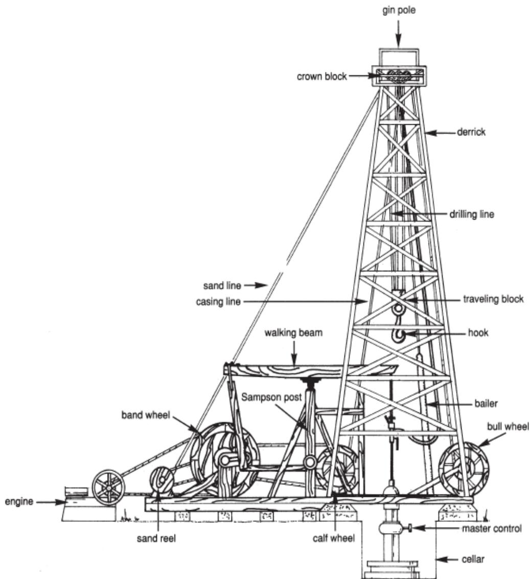
**Figure 2.4:** Cable-tool drilling rig [10]
