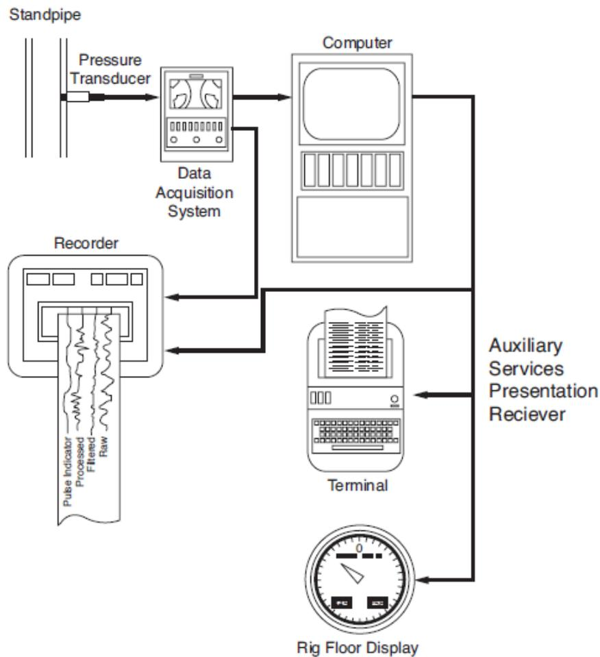
**Figure 3.22:** Surface processing and reporting system [25]
