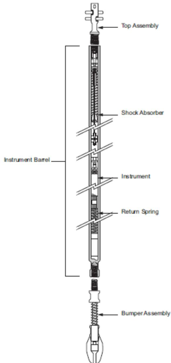
**Figure 3.12:** Main components of magnetic single shot device [25]
