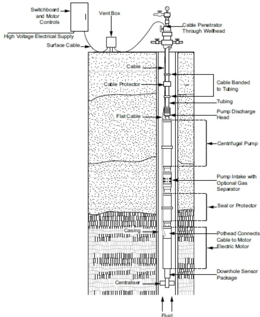
**Figure 4.10:** Artificial lift using an electric submersible centrifugal pump [34]
