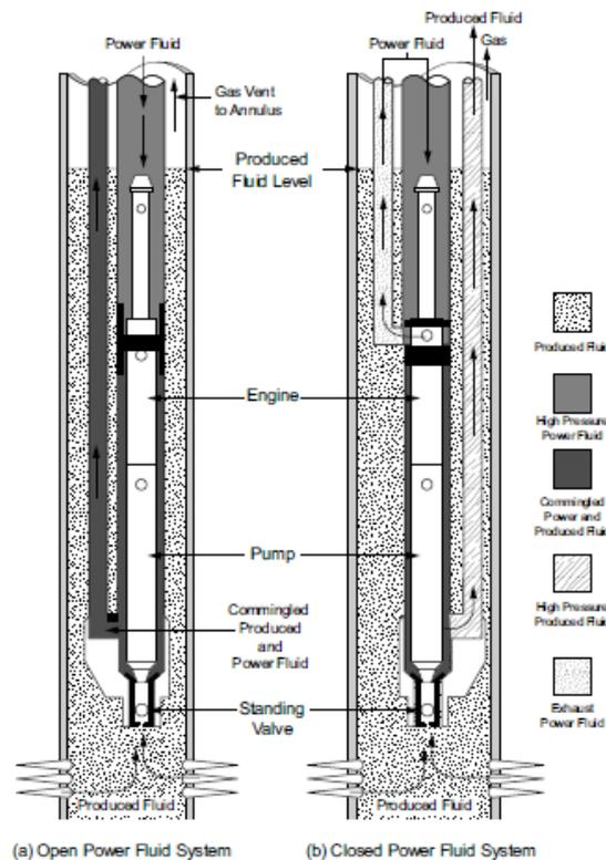
**Figure 4.9:** Types of hydraulic pump installation [34]
