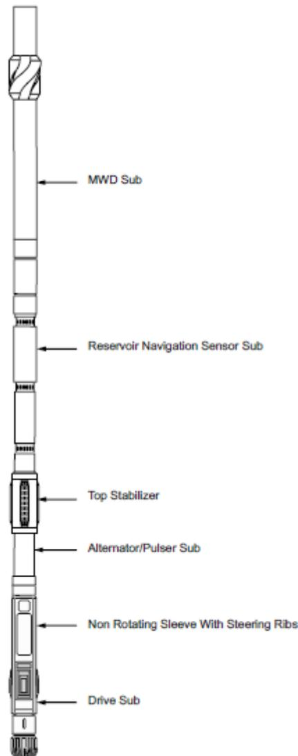
**Figure 3.8:** Rotary steering system (Courtesy of Baker Hughes a GE company)
