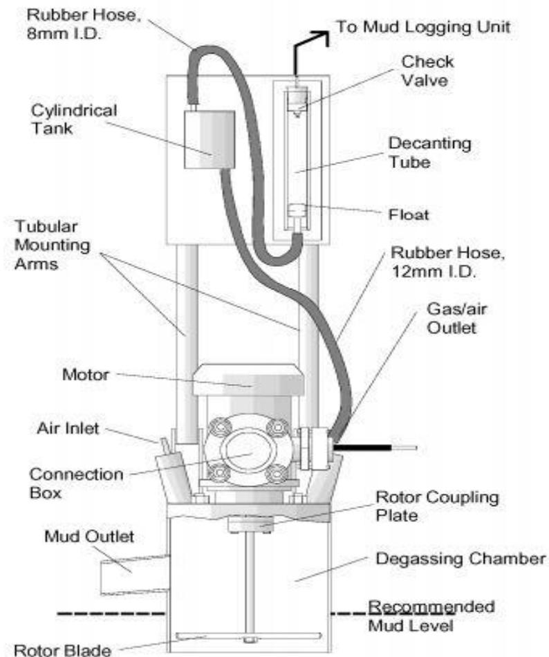
**Figure 2.16:** Schematic view of a gas trap [19]
