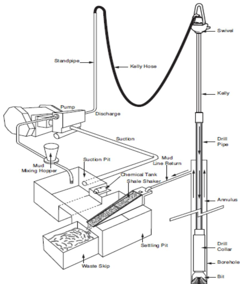
**Figure 2.9:** Schematic representation of fluid circulating system [14]
