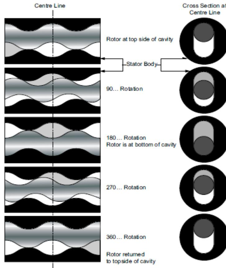
**Figure 4.15:** Operating principle of PCP [34]
