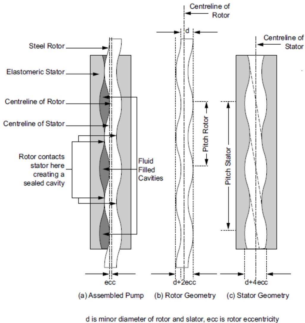
**Figure 4.13:** Cross section PCP and its components [34]
