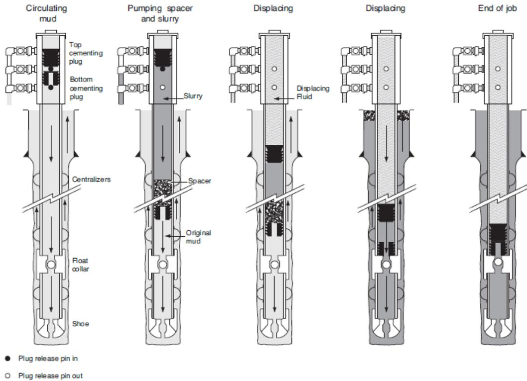
Figure 2.21: Primary cementing operations [7]
