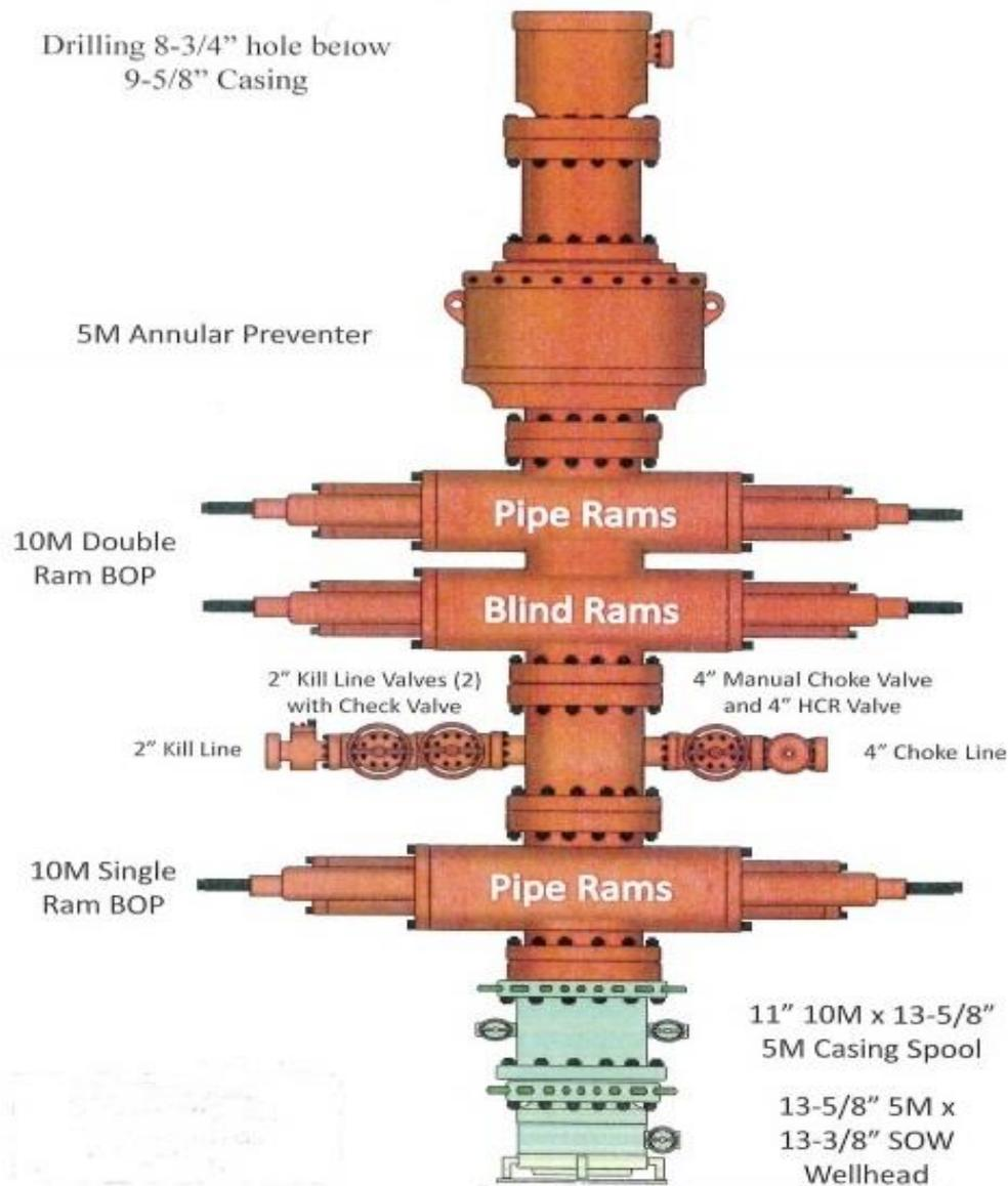
**Figure 2.13:** Schematic of BOP
