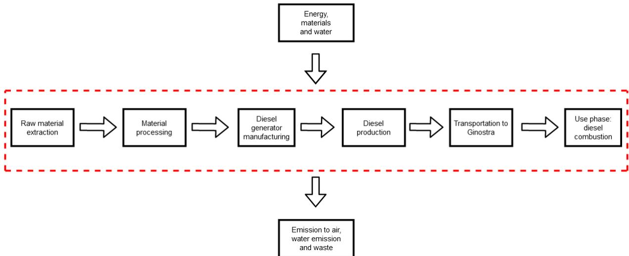
Figure 31: Block diagram for diesel generators in current scenario
