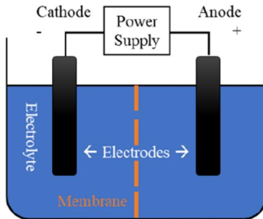
Figure 20: General configuration of a typical electrolysis cell [35]
