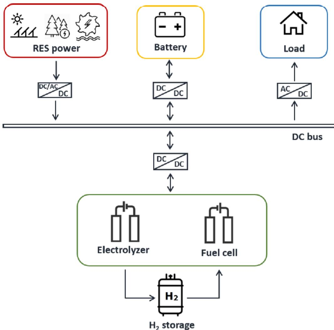
Figure 15: General configuration of a stand-alone RES/H<sub>2</sub>/battery-based hybrid system [16]
