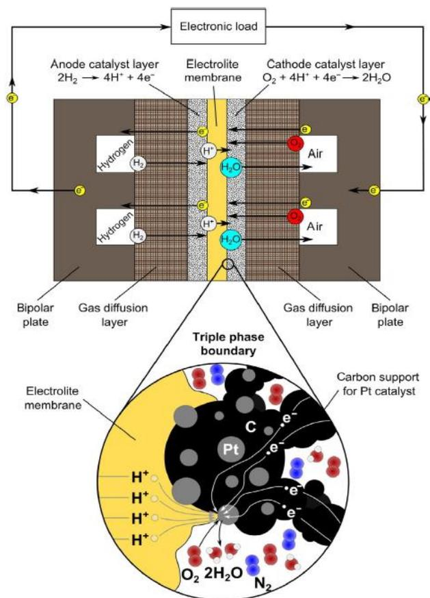
Figure 27: Operating principle of a proton exchange membrane (PEM) fuel cell [46]
