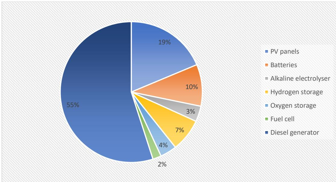
Figure 33: Particulate matter emission from Ginostra plant
