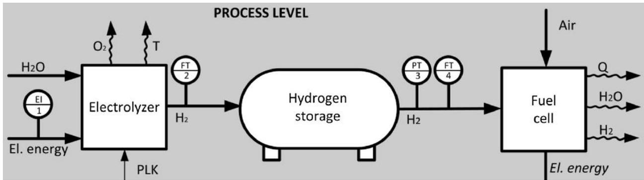
Figure 50: Scheme of the installed HT-UPS system (modified) from paper [41]
