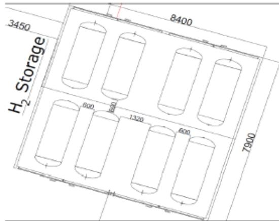
Figure 24: Layout of the H<sub>2</sub> storage
