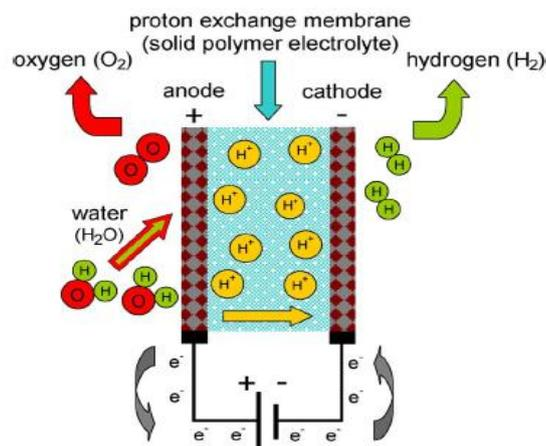
Figure 22: Operating principle of a PEM electrolysis cell [38]
