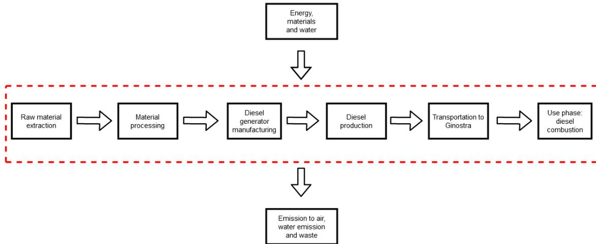
Figure 29: Block diagram for diesel generators
