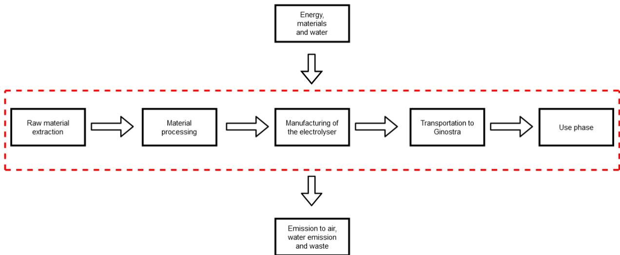
Figure 23: Block diagram for electrolyzers
