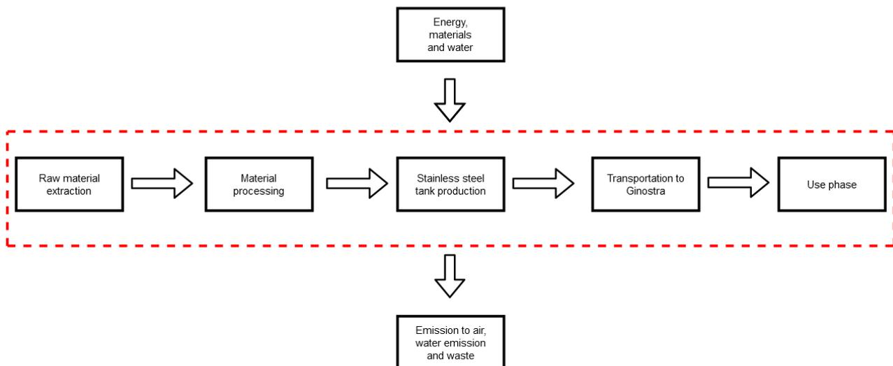
Figure 25: Block diagram for hydrogen tanks
