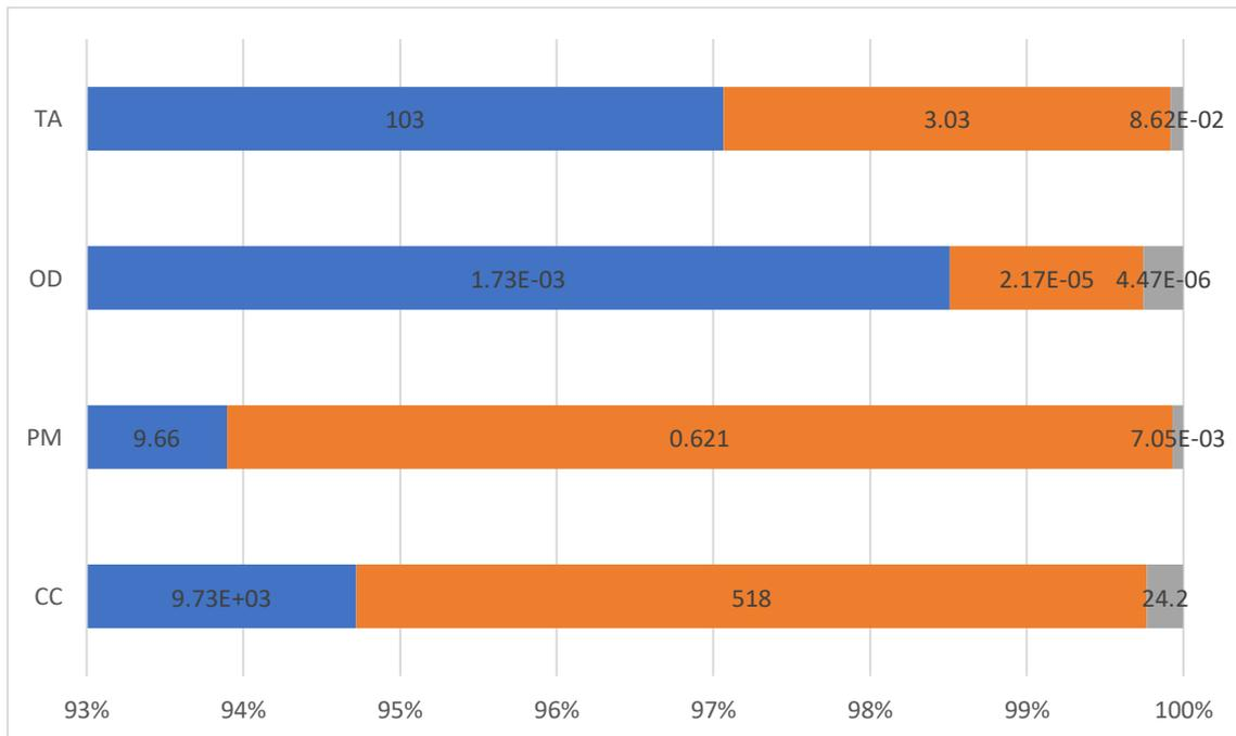
Figure 43: Share of the different emissions from diesel generators in current scenario
