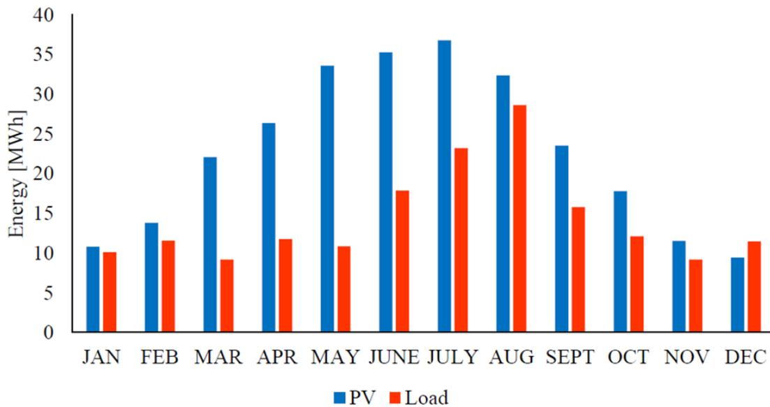
Figure 17: Monthly distribution of PV production and load [16]
