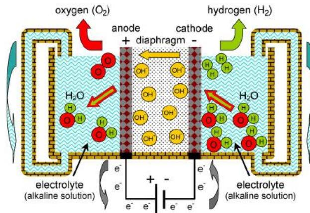
Figure 21: Operating principle of an Alkaline electrolysis cell [38]
