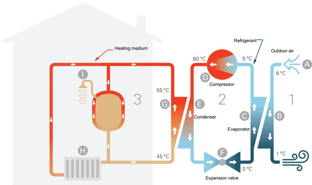
**Figure 2.1:** Conceptual diagram of an air-to-water heat pump. The temperatures are only examples and may vary between different installations and time of year [16].
