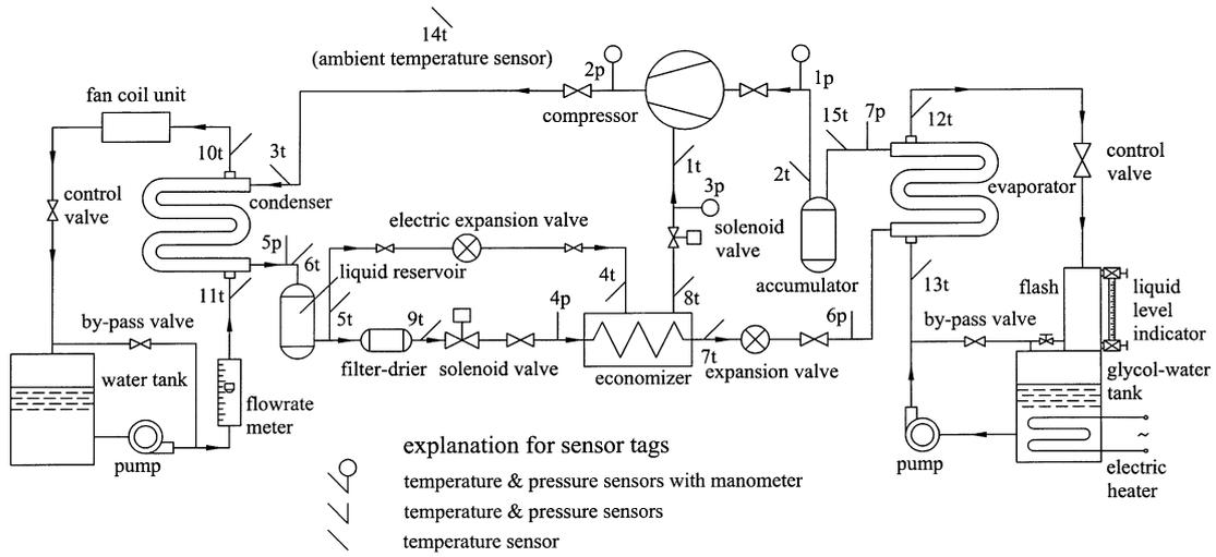
Figure 2.14: Test system and sensor locations for the ASHP prototype [37].
