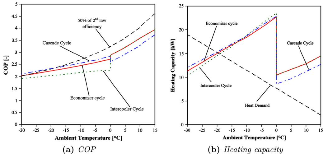
**Figure 2.17:** Simulation results of COP and heating capacity at 50 °C supply temperature [36].
