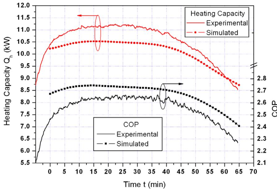
**Figure 2.10:** Comparison of experimental heating capacity and COP with simulated results under condition of  $T_{a,i} = 0^{\circ}\text{C}$ ,  $\text{RH} = 75\%$  [34].
