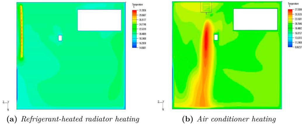
**Figure 2.6:** Horizontal temperature contours at 1.2 m height [33].
