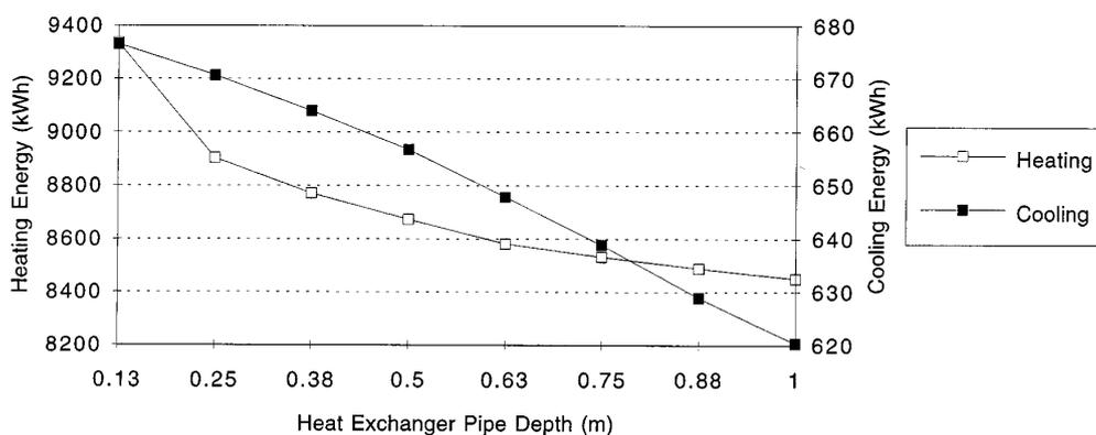
**Figure 2.27:** Effect of ground heat exchanger pipe depth on energy consumption [56].
