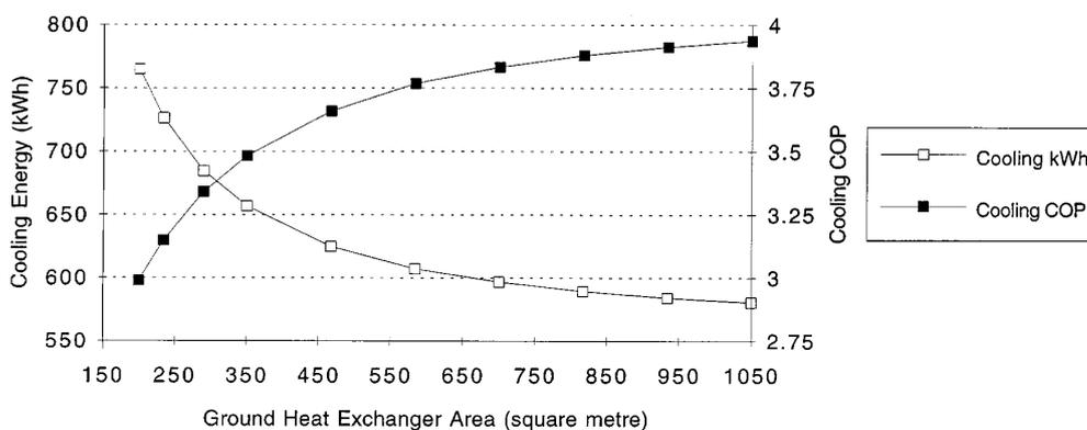
Figure 2.25: Effect of ground heat exchanger area on cooling performance [56].
