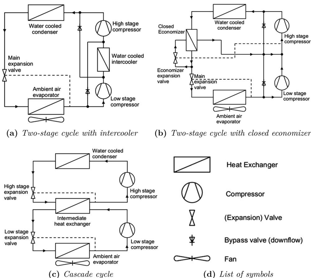
**Figure 2.16:** Simplified schematics of two-stage cycle with intercooler, two-stage cycle with closed economizer, and cascade cycle [36].
