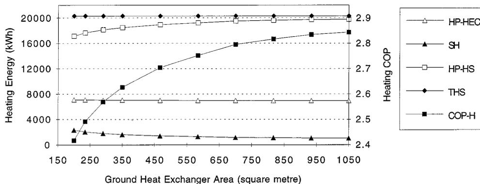
Figure 2.24: Effect of ground heat exchanger area on heating performance [56].
