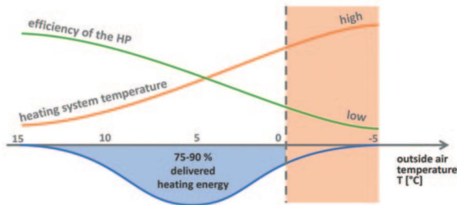
**Figure 2.11:** Correlation between the heat delivered by an average heat pump, the temperature and the efficiency [18].
