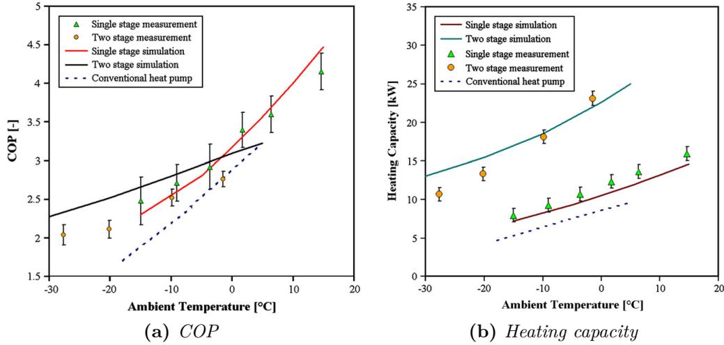
**Figure 2.18:** Simulation results for the systems with the economizer at 50 °C supply temperature and considering auxiliary power [36].
