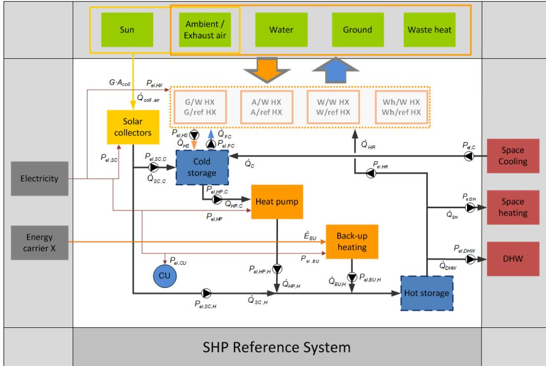
Figure 2.20: Reference SHP system proposed by the IEA SHC Task 44 [49].
