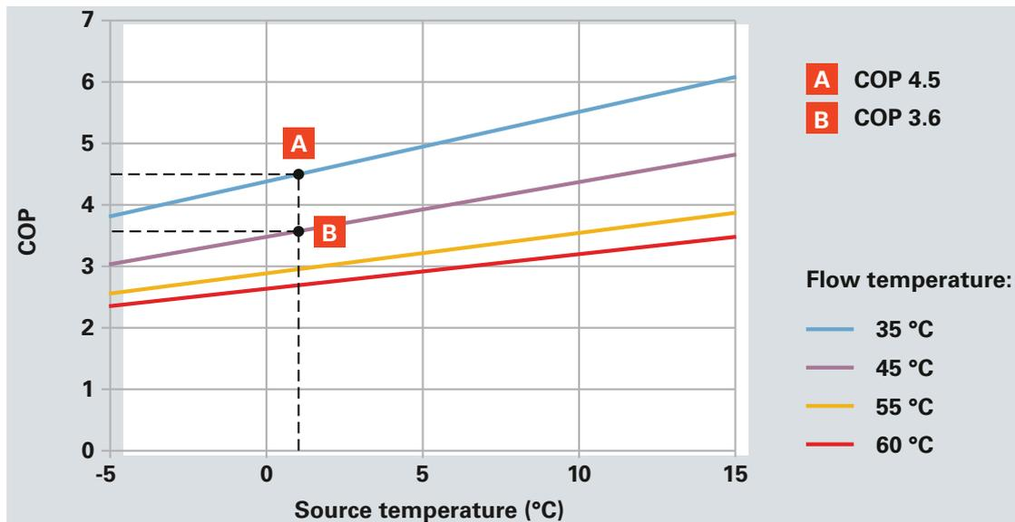
**Figure 2.7:** Heating circuit flow temperature and efficiency [24].
