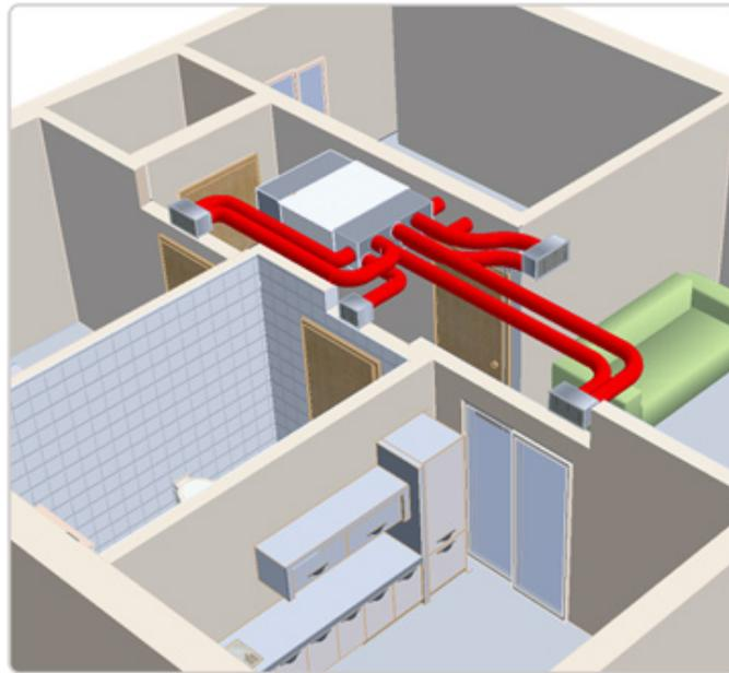
**Figure 2.3:** Design of an aeraulic plant located in a passageway [32].
