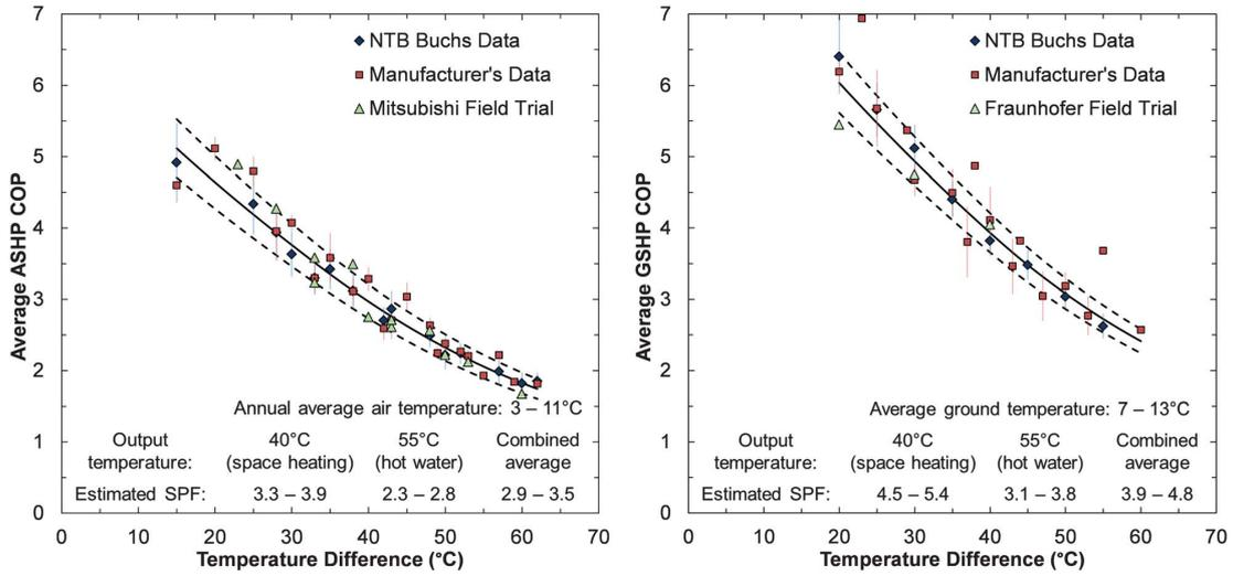
**Figure 2.9:** Average heating COP for air and ground source heat pumps (left and right, respectively) based on data taken from industrial surveys and field trials [10].
