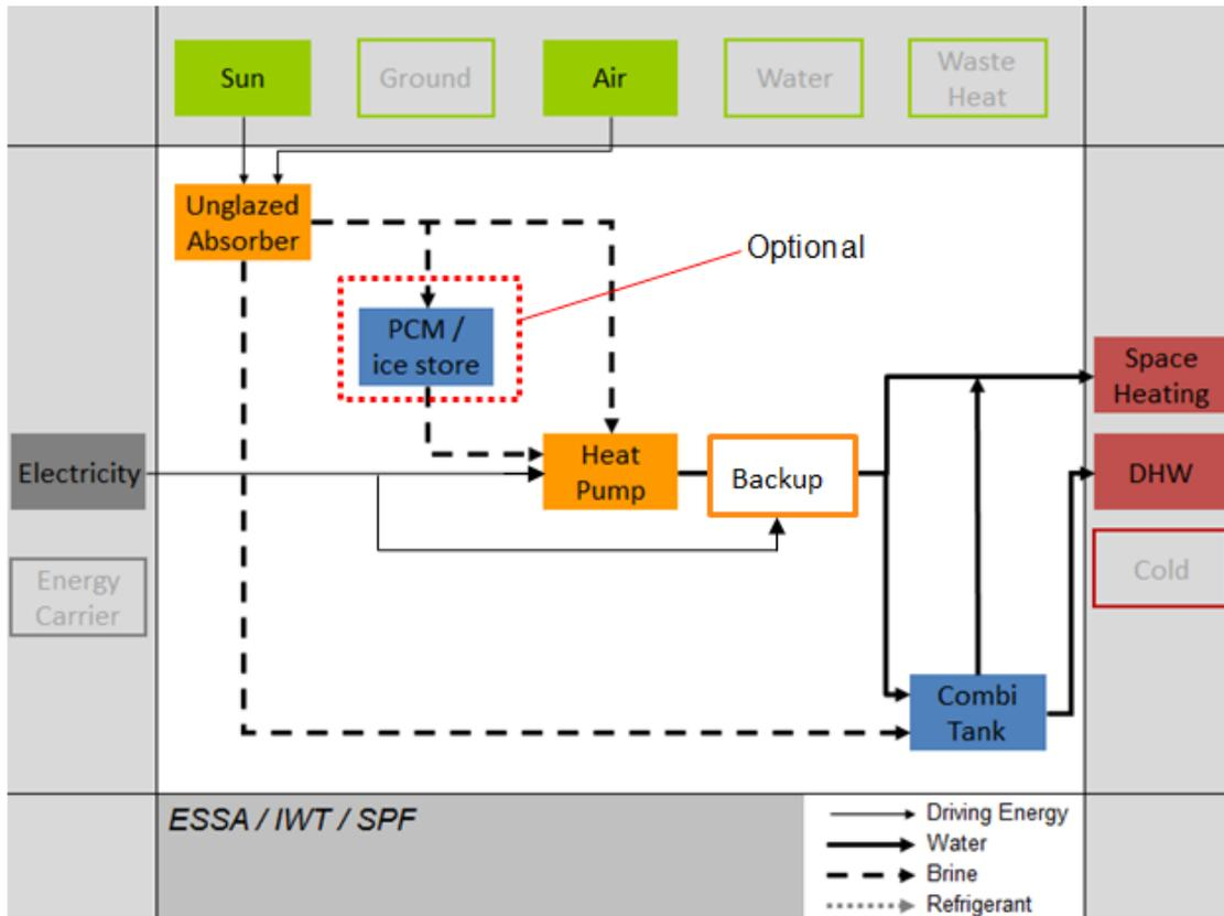
**Figure 2.23:** System diagram of the highly compact solar heat pump [48].
