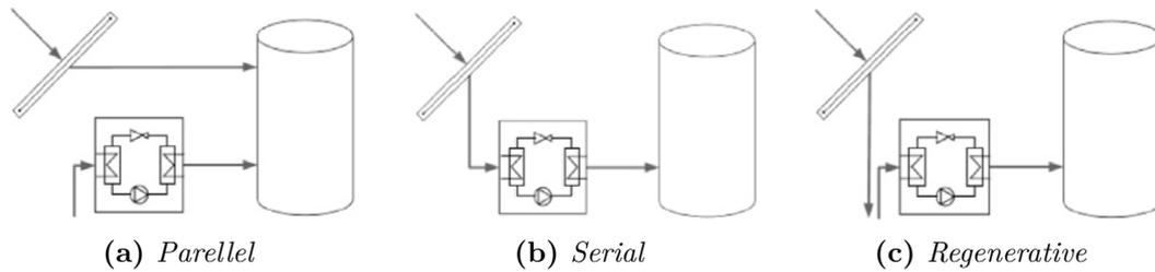
**Figure 2.21:** Classification of solar thermal and heat pump systems in parallel, serial and regenerative system concepts [45, 46].
