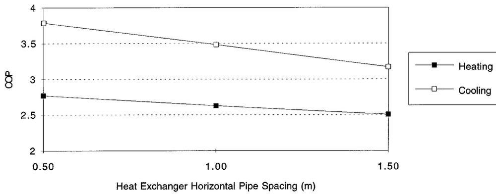
Figure 2.29: Effect of ground heat exchanger horizontal pipe spacing on COP [56].
