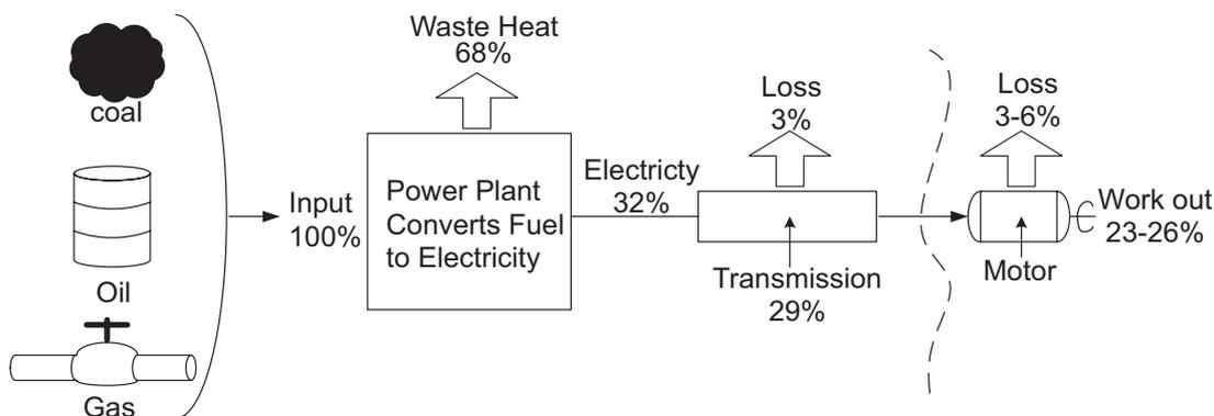
**Figure 2.19:** Losses of the conversion process of an electric heat pump [39].
