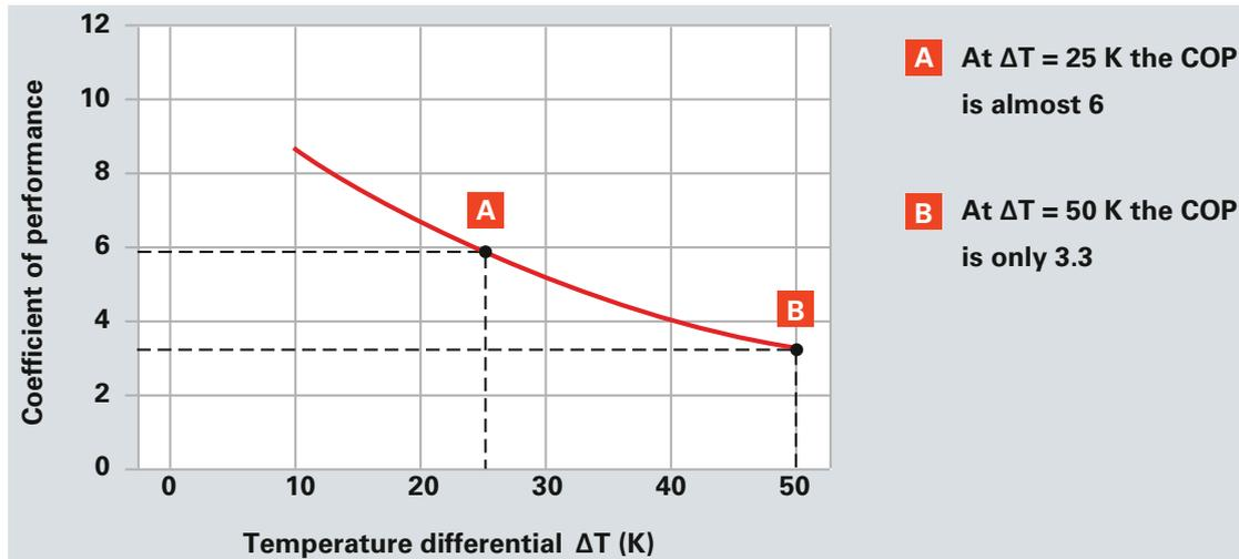
**Figure 2.2:** Temperature differential and coefficient of performance [24].
