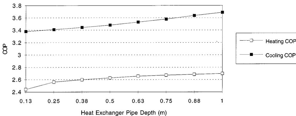
Figure 2.26: Effect of ground heat exchanger pipe depth on COP [56].
