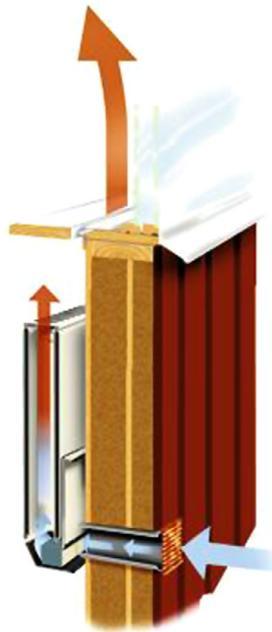
**Figure 2.4:** Sketch of a ventilation-radiator [29].
