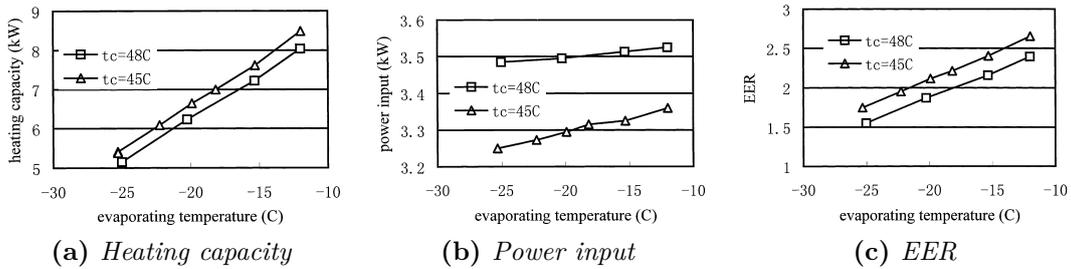
Figure 2.15: Heating capacity, power input and EER depending on evaporating temperature of the improved ASHP [37].
