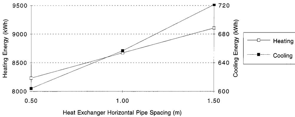
Figure 2.30: Effect of ground heat exchanger horizontal pipe spacing on energy consumption [56].
