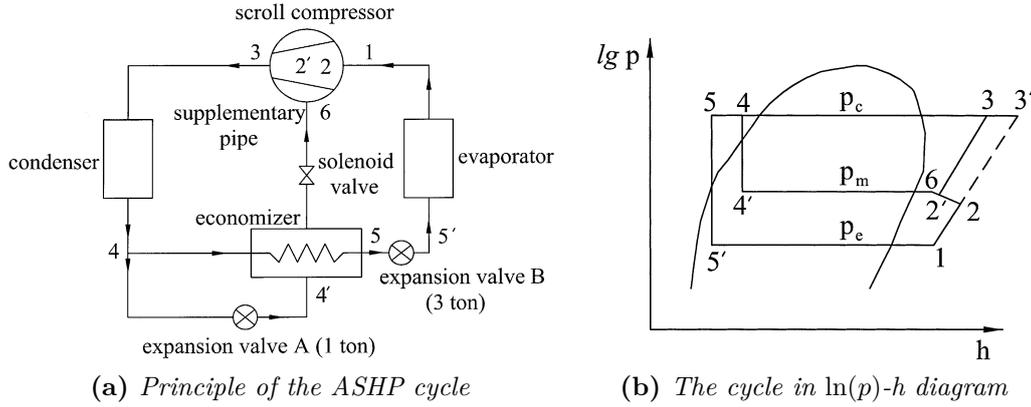
**Figure 2.13:** Enhanced ASHP with scroll compressor and economizer [37].
