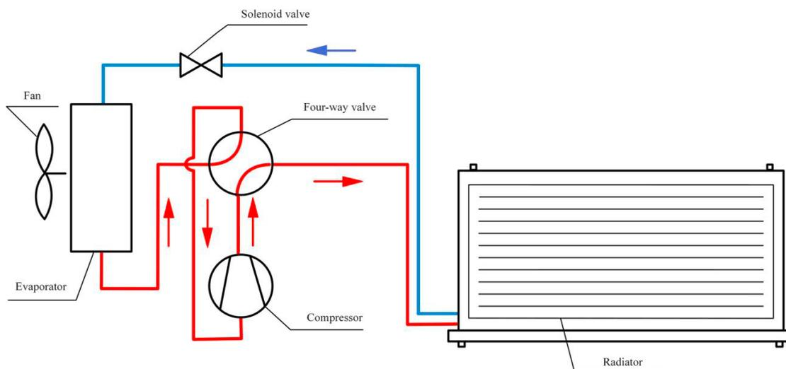
**Figure 2.5:** Schematic diagram of the RRH system [33].
