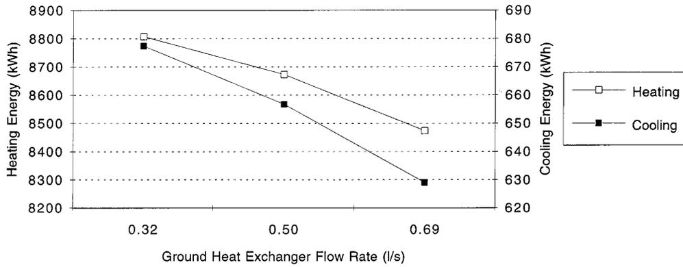
Figure 2.28: Effect of ground heat exchanger flow rate on energy consumption [56].
