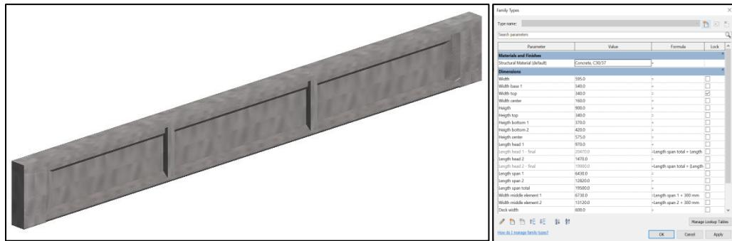
**Figure 27.** Parametric family created on Revit for double T beam.
