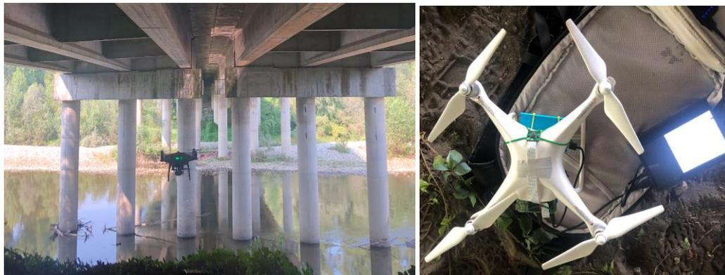
**Figure 44.** Modified drone during the survey activity.
