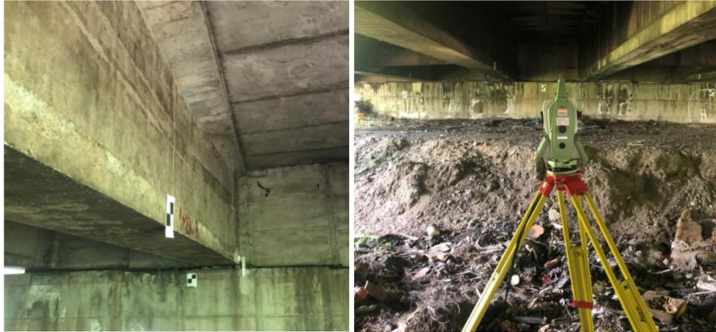
**Figure 41.** Markers positioned in bridge surface and total station used.
