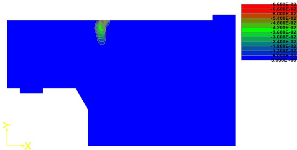
Figure 6.51: step 220, concrete minimum strain at beam failure
