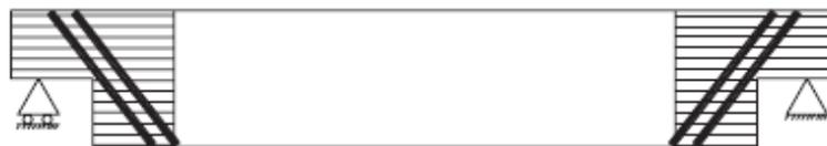
Figure 2.24: Taher reinforced half-joint, with CFRP strips and carbon fibre wrapping
