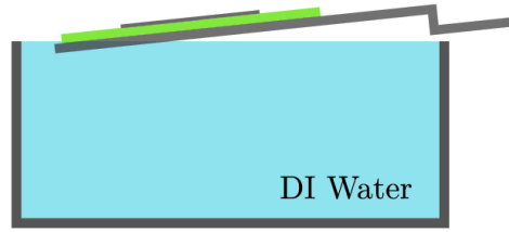
Figure 43: Floating film "fishing"
