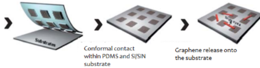
Figure 35: summary sketch of PDMS dry transfer
