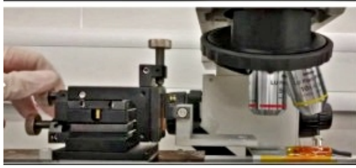
Figure 34: NUS cleanroom's manual transfer station
