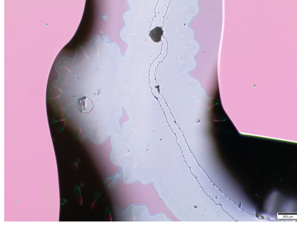
Figure 37: Particular of a circular scratch around the chosen flake
