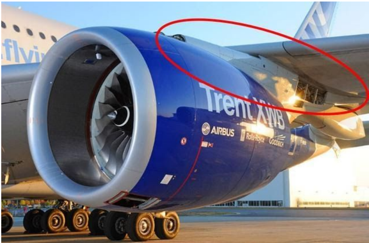
Figure 4.9 Titanium alloy bracket between the aircraft wing and the engine nacelle
