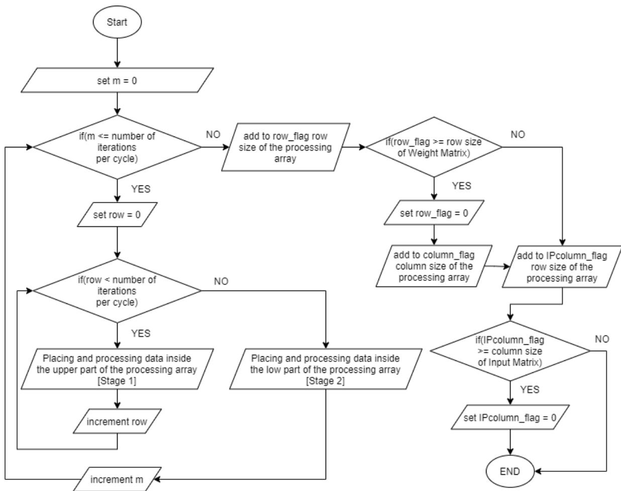
Figure 3-22 Data processing stage flowchart
