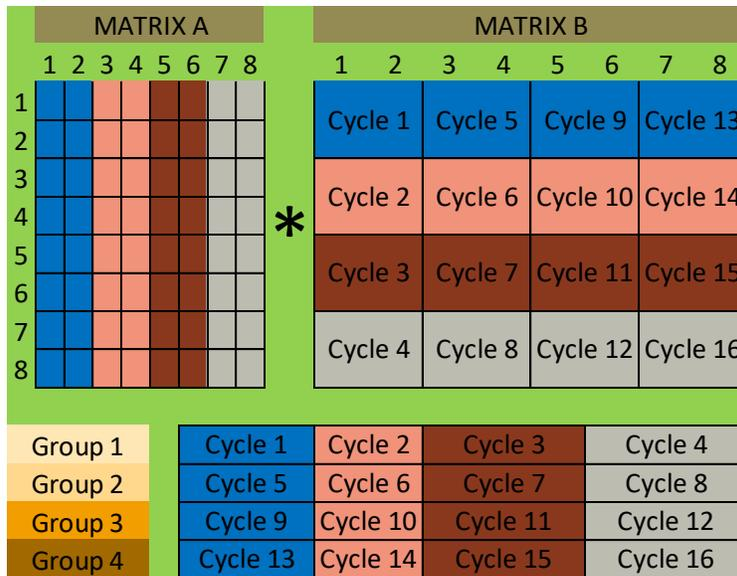
Figure 3-12 Sample of accumulating Weight (8x8) with Input tensor (8x8)
