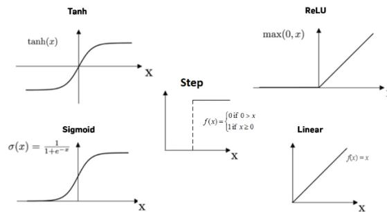
**Figure 2-5 Types of activation functions**
