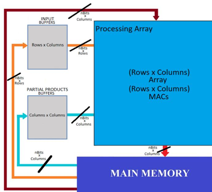
Figure 3-3 Top view of the *Processing Unit*
