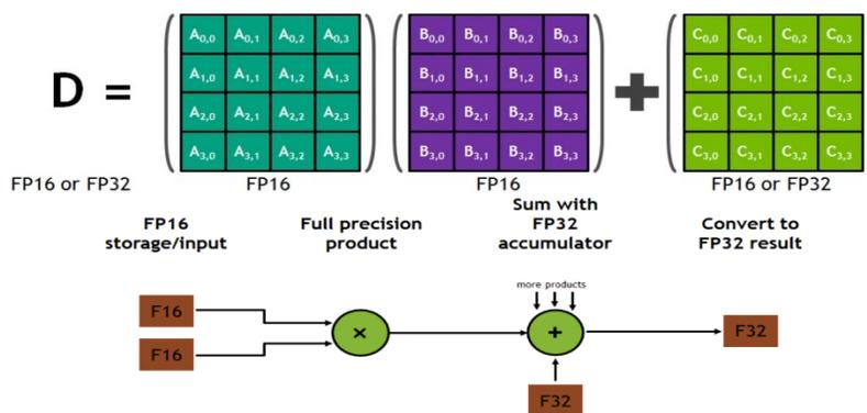
Figure 2-20 Nvidia GA100 Tensor core, [31]
