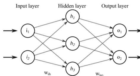
**Figure 2-6 Simple neural network example, [21]**
