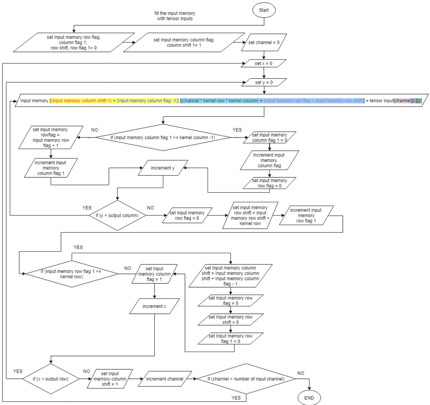
Figure 3-16 Input tensor distribution tensor flowchart
