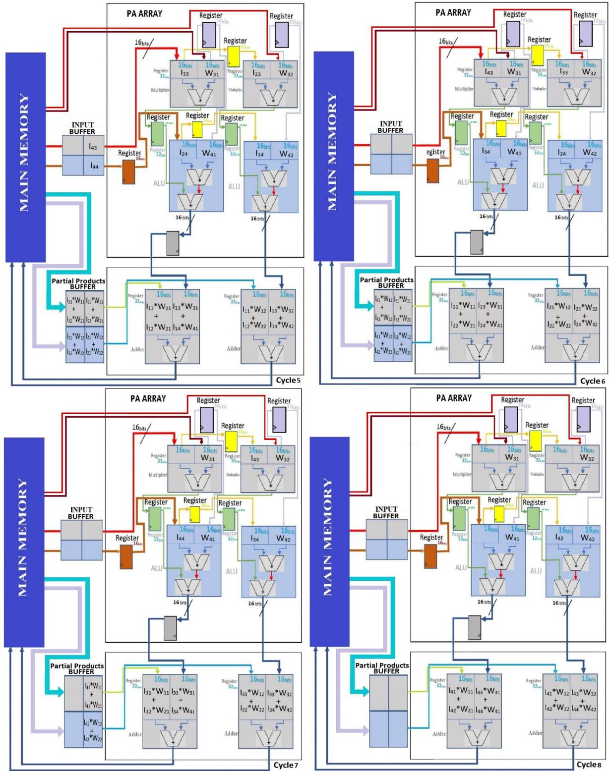
Figure 3-13 Completion of processing and accumulation a Weight (4x4) with Input tensor (4x4) in Processing Array with hardware components
