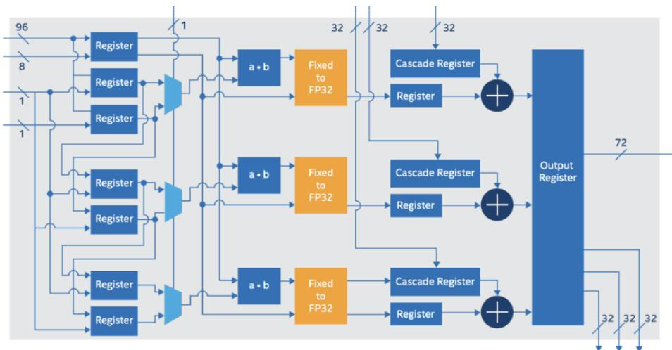
Figure 2-22 Intel Stratix 10 AI Tensor blocks, [32]
