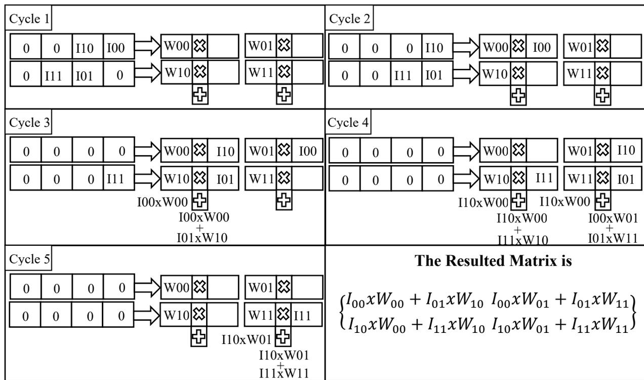
Figure 2-14 Matrix Multiplication using Weight stationary dataflow
