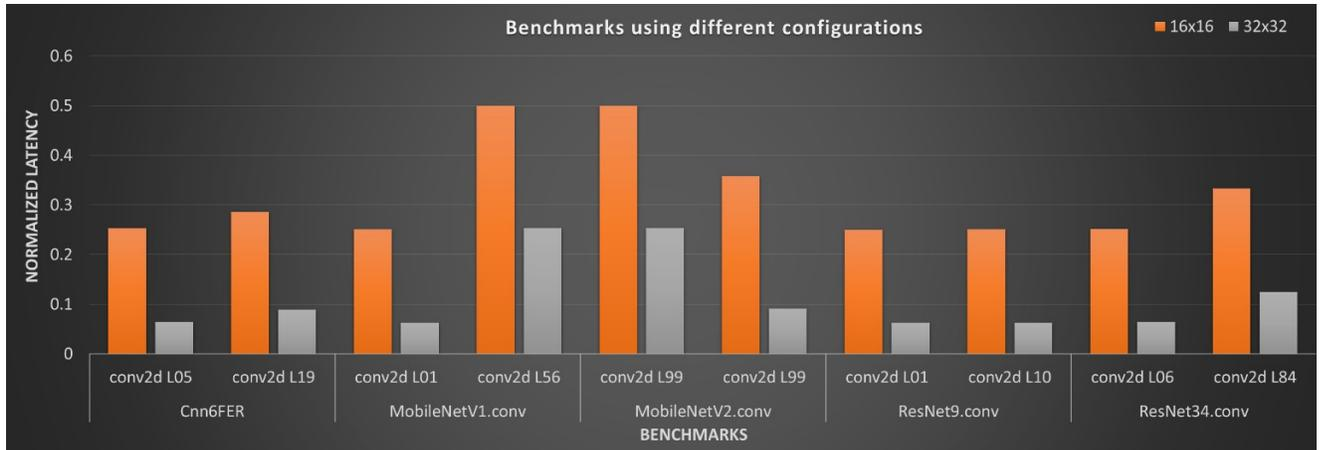
**Figure 4-2 Normalized latency with respect to 8x8 configuration on the proposed benchmarks**
