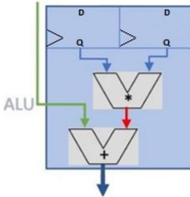
**Figure 3-9 Processing Element Top view**
