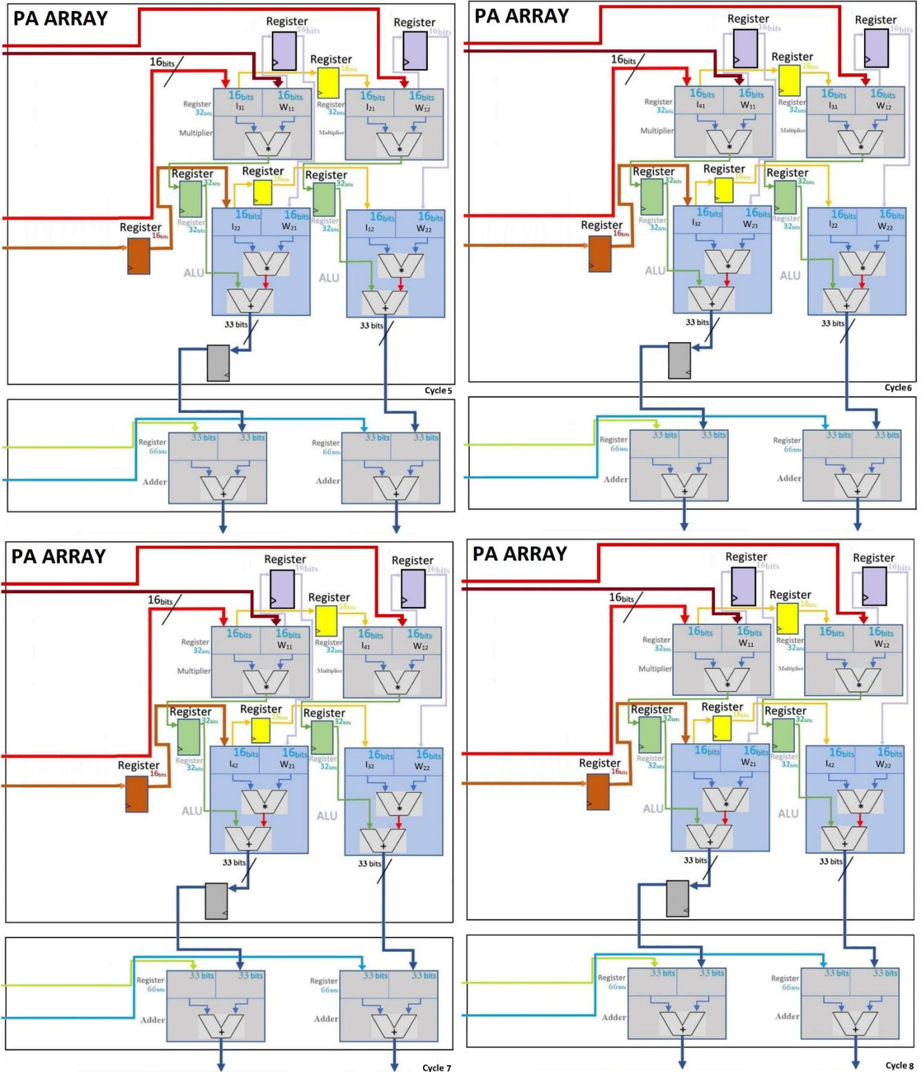
Figure 3-11 Sample of processing a Weight (4x4) with Input tensor (4x2) in Processing Array with hardware components
