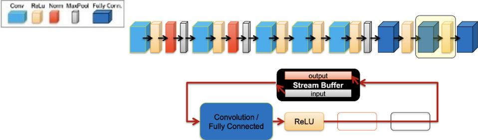
Figure 2-23 Neural network pipelining, [33]
