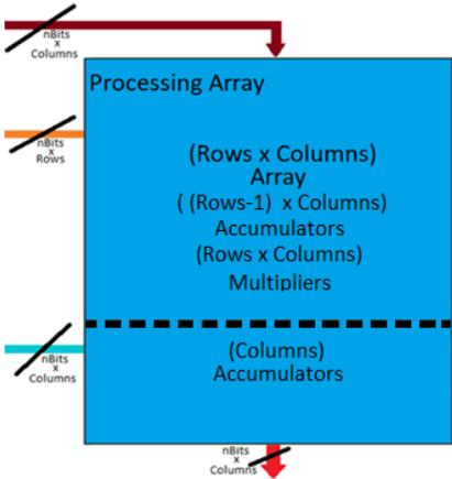
Figure 3-7 Processing Array top view
