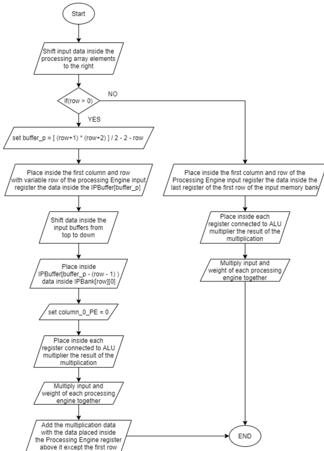
**Figure 3-23 Data processing stage of the upper part**
