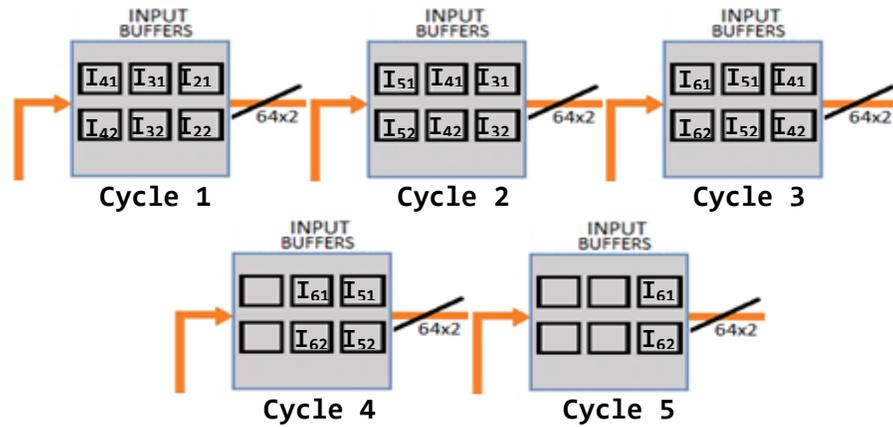
Figure 3-5 Input shifting cycle sample
