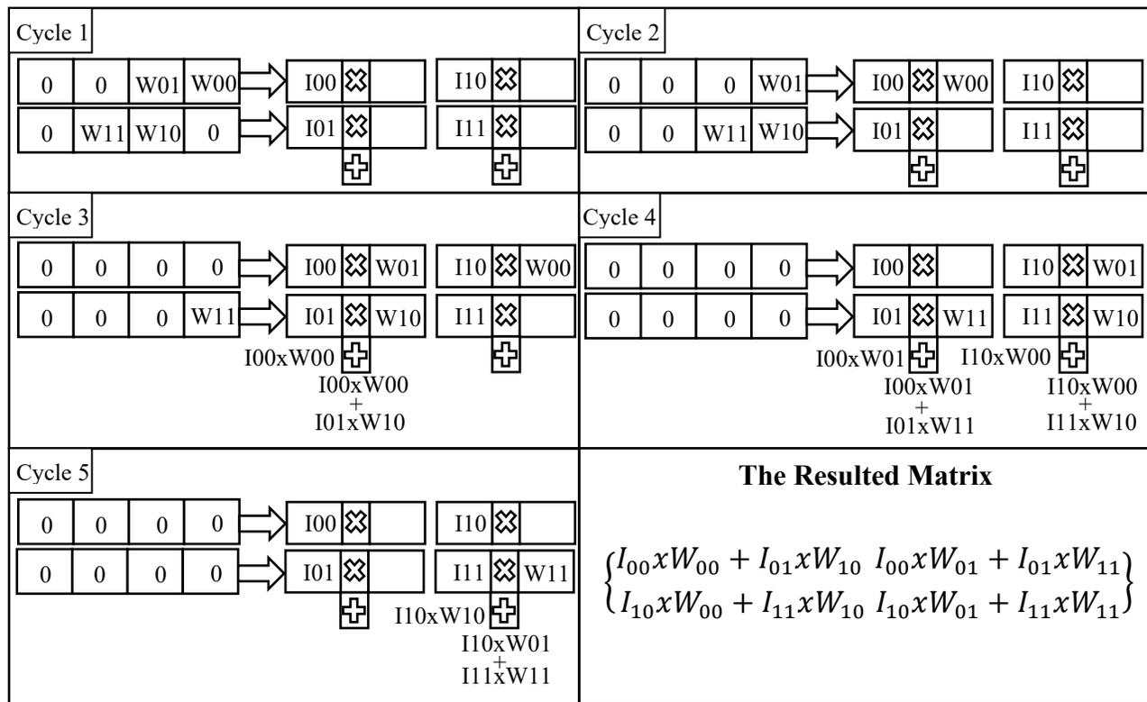
**Figure 2-13 Matrix Multiplication using input stationary dataflow**
