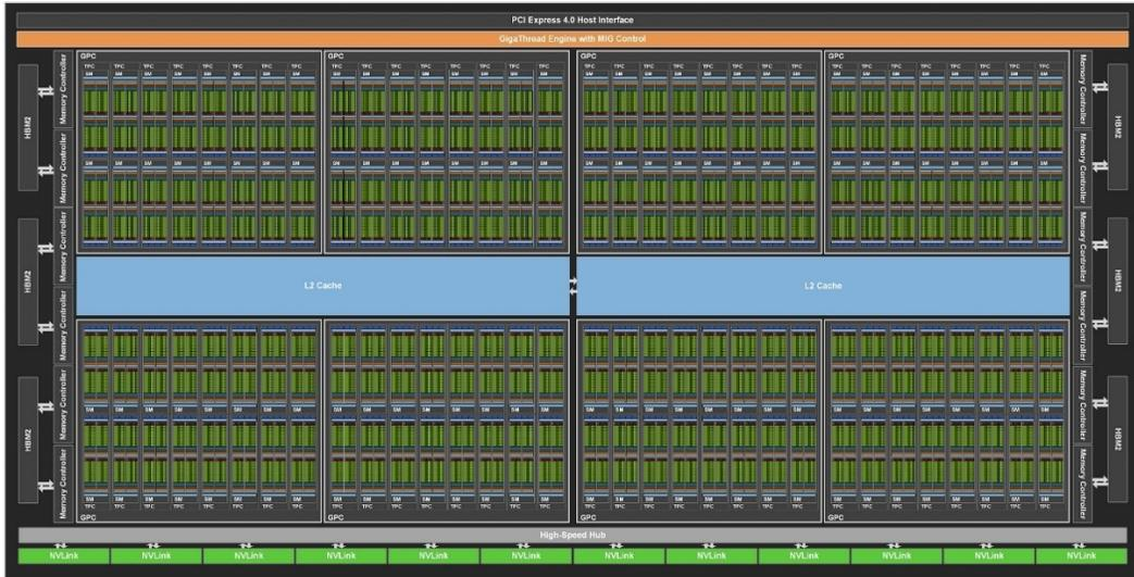
Figure 2-19 Nvidia GA100 Top-level Architecture, [30]
