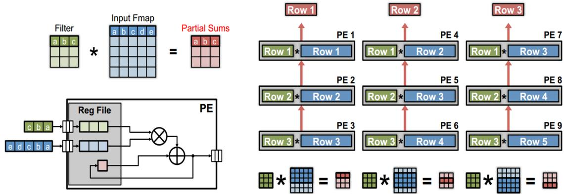
Figure 2-17 Eyeriss dataflow used, [24]
