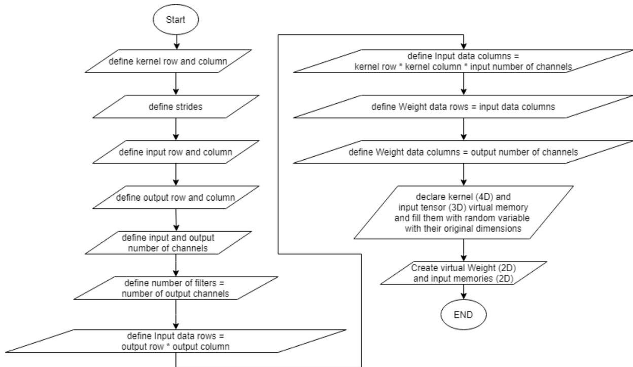
Figure 3-14 Neural network parameters definitions flowchart
