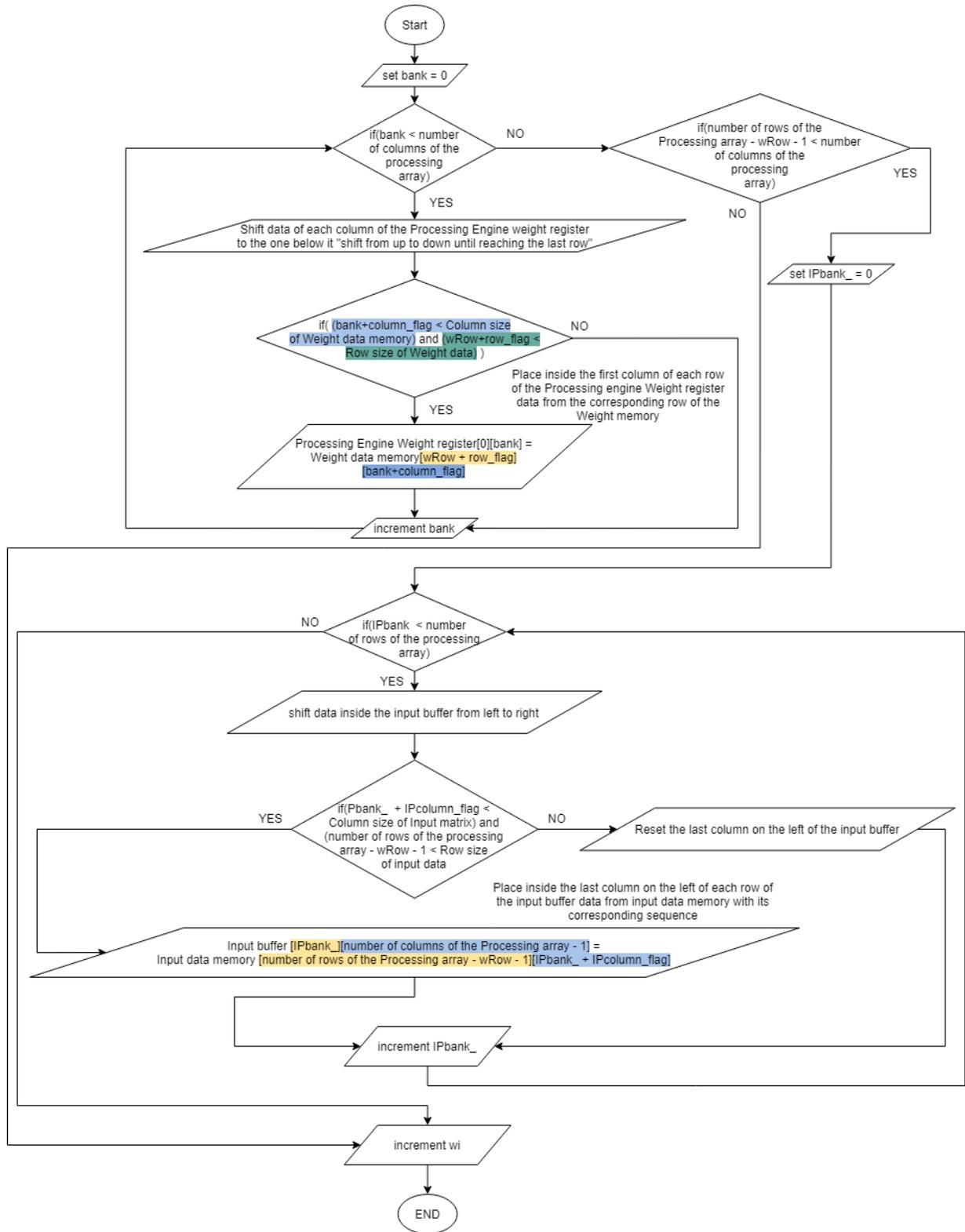
Figure 3-20 Data placement stage by row flowchart
