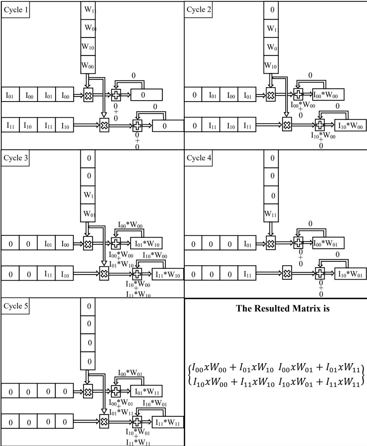
Figure 2-15 Matrix Multiplication using Output stationary dataflow
