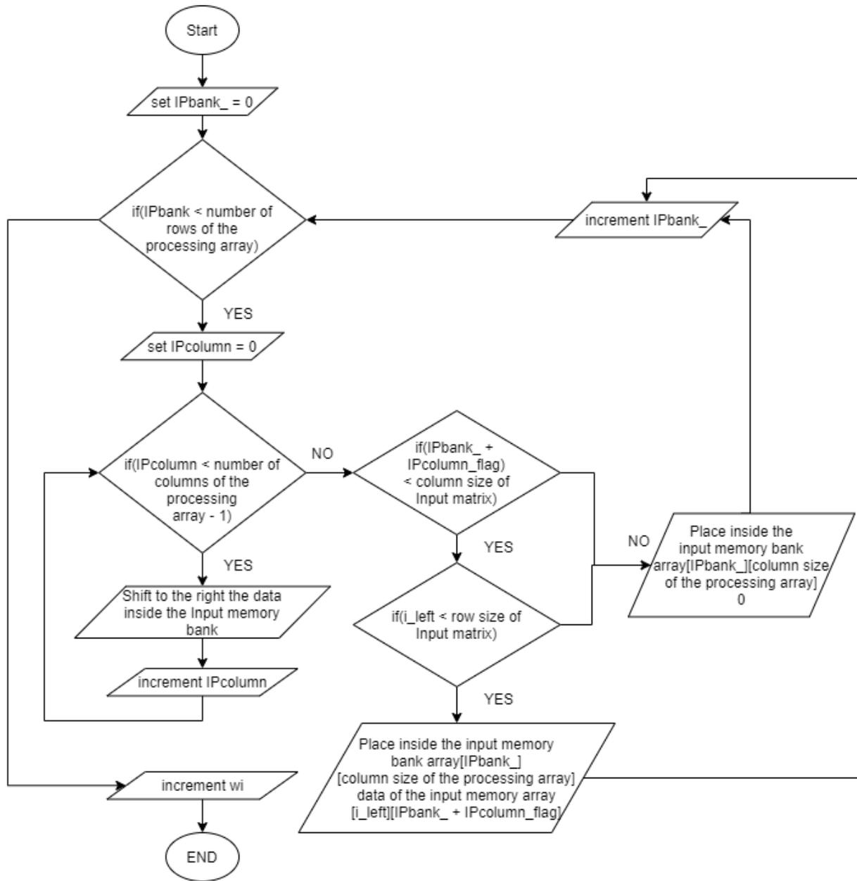
Figure 3-21 Data placement stage by column flowchart
