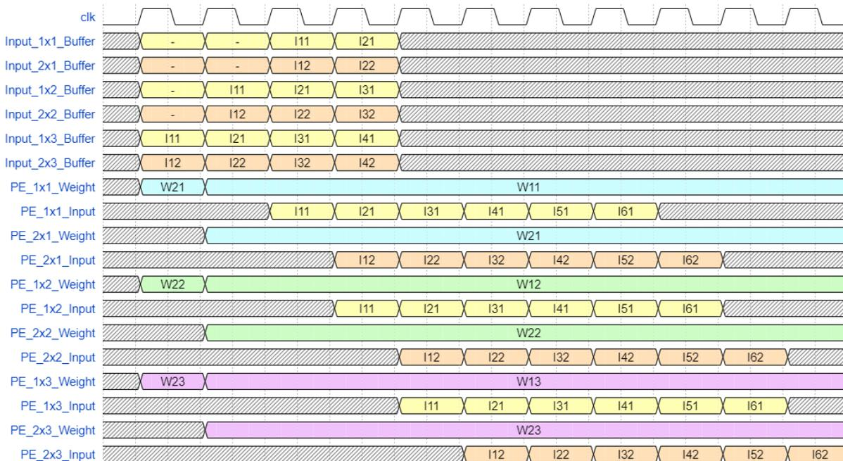
**Figure 3-6 Processing Unit synchronization waveform**
