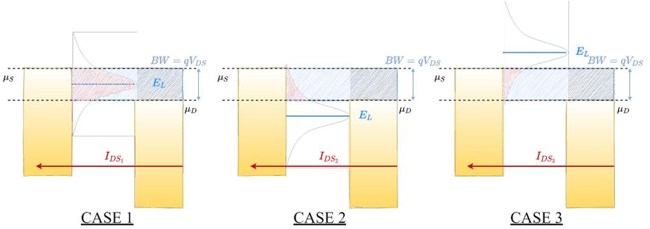
**Figure 3.9:** Case 1,2,3 described above in the case of a single broadened level. The voltage division factor  $\eta = 1/2$  shifts the Fermi level of the source  $qV_{DS}/2$  above and the Fermi level of the drain below. In this case  $I_{DS} \neq 0$  in all the three cases, since always a portion of the transmission spectrum is included within the bias window. In particular:  $I_{DS1} > I_{DS2} > I_{DS3}$  since less and less amount of the  $T(E)$  is integrated to obtain the total current.
