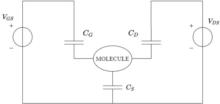
**Figure 2.24:** Equivalent circuitual representation of MolFET.
