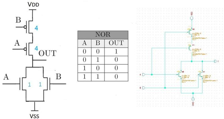
**Figure 6.8:** Conceptual and Cadence schematic of the NOR with transistors properly sized. Also the truth table of the NOR is shown.
