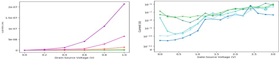
**Figure A.1:** On the left: parametric Output characteristic of n-OPV7 MolFET when it is in the OFF state, with parameter  $V_{BG}$ ; On the right: parametric trans-characteristic in log scale of n-OPV7 MolFET when it is in the OFF state, with parameter  $V_{DS}$ .
