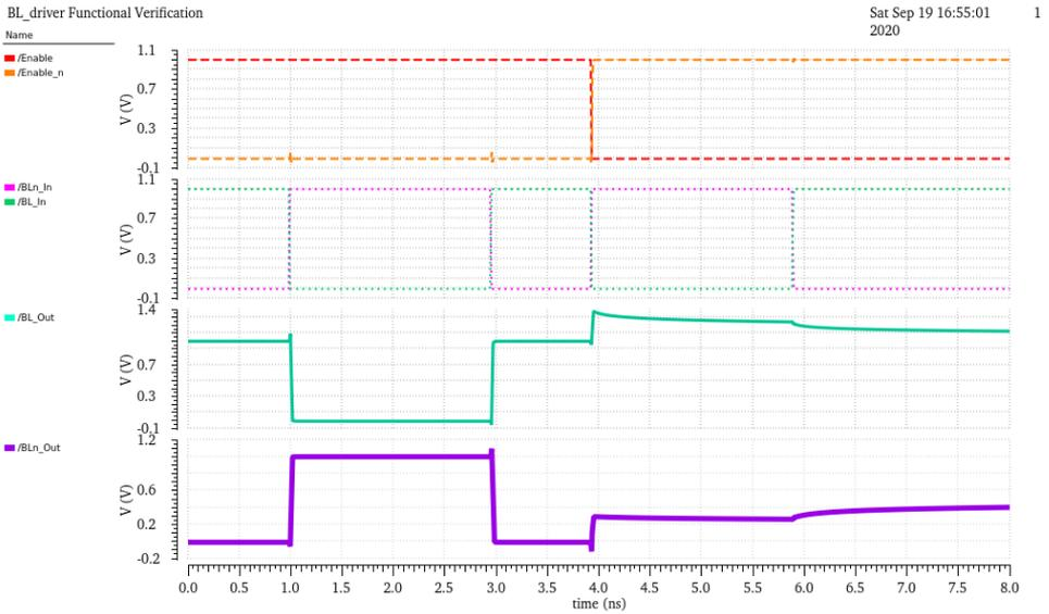
**Figure 7.18:** Spectre functional verification of bitline driver circuit implemented with MOSFET technology.
