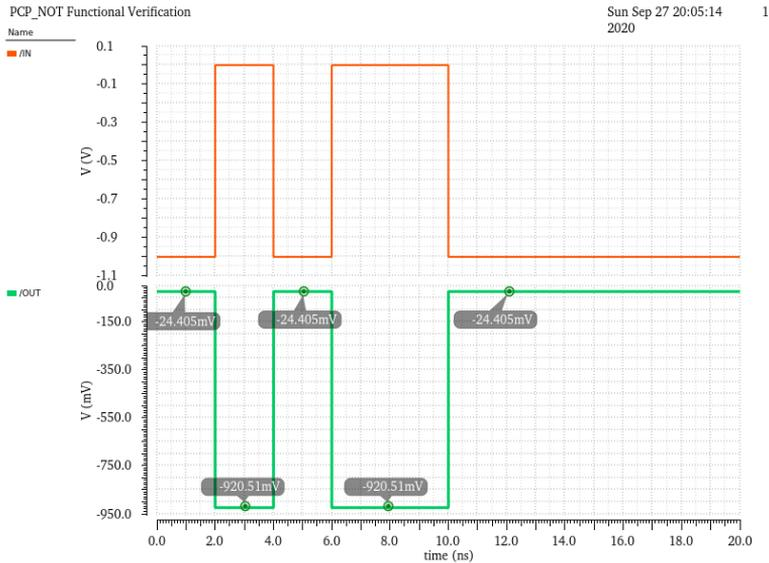
**Figure 6.20:** Functional verification simulation of PCP molFET-based inverter.
