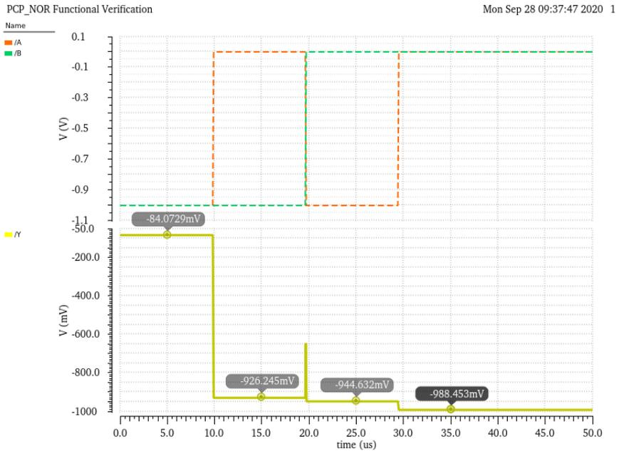
**Figure 6.24:** Functional verification simulation of PCP molFET-based NOR.
