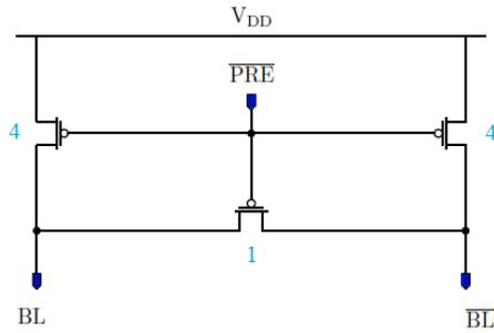
Figure 7.16: In-principle schematic of precharge circuit.
