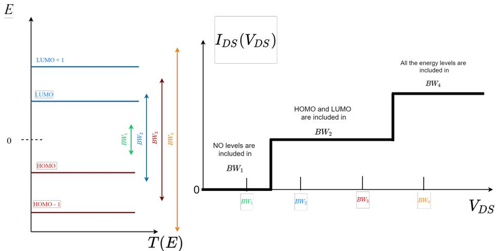
**Figure 3.12:** Discrete energy levels distribution on the left side, the resulting IV curve on the right side.
