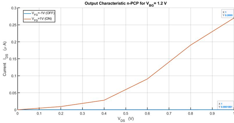
**Figure 4.11:** Output characteristic of n-PCP MolFET. A ratio  $I_{on}/I_{off} \simeq 1452$  is achieved. Here is not present a NDR trend, and the characteristic is almost linear in the range analyzed.
