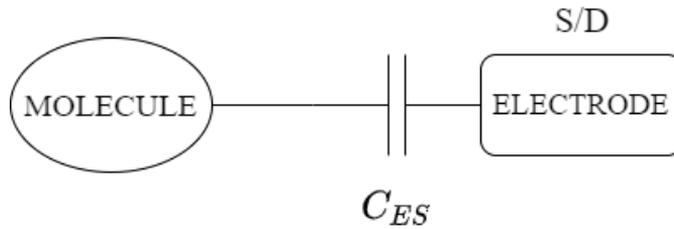
**Figure 2.23:** Equivalent circuit model of two-probe 0D-system.
