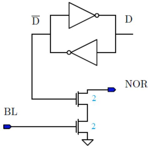
**Figure 8.9:** Special purpose LiM cell with chosen AR of transistors channel width. Only the bistable ring of the SRAM cell is shown, pass transistors and surrounding WLs and BLs are omitted for sake of clarity.
