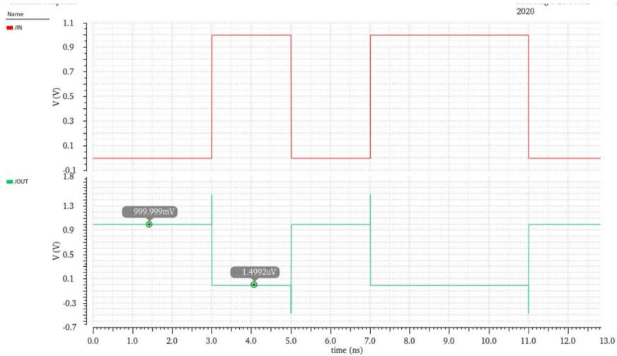
**Figure 6.5:** DC functional verification of the inverter gate. The output is correctly complemented. Obviously the output dynamic is reduced w.r.t. the input one, due to very negligible unwanted voltage drops on the  $R_{ON}$  of the ON transistors.
