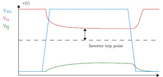
**Figure 7.8:** Data flip in writing operation. If  $V_Q$  does not lower below the bistable ring trip-point, the data is not written to the cell.
