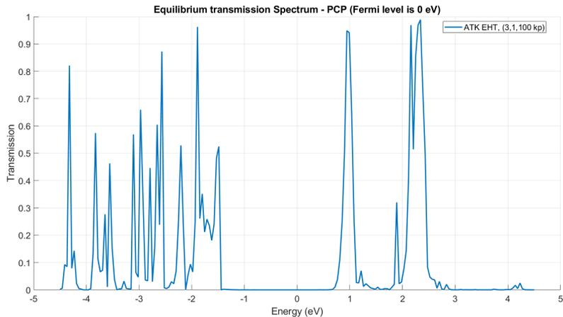
**Figure 4.6:** Equilibrium TS for PCP double gate transistor.
