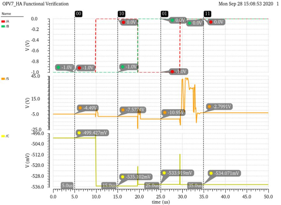
**Figure 6.27:** Functional verification simulation of OPV7 molFET-based HA.
