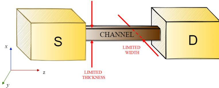
**Figure 2.4:** An example of 1D-system where the thickness and the width of the channel are limited to few nanometers. The direction of confinement are the transversal directions  $x$  and  $y$ , orthogonal to the direction of transport ( $z$ ).
