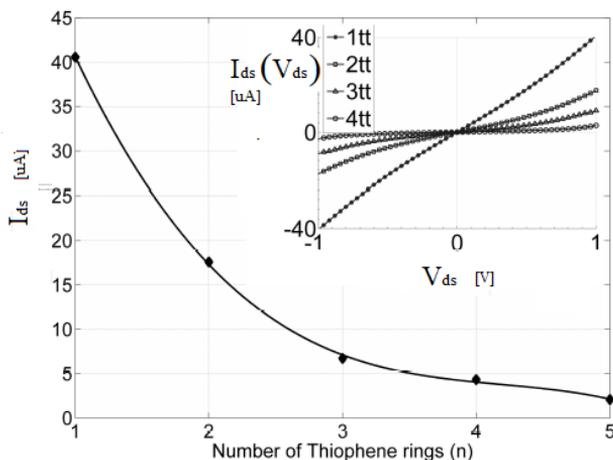
**Figure 3.23:** The resulting drain current  $I_{DS}$  for OT molecules as a function of increasing number of rings at  $V_{DS} = 1V$ . On the right top the IV curve of OT molecules with different lengths in the bias range of  $[-1V$  to  $1V]$
