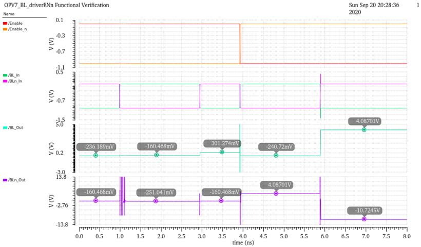
**Figure 7.24:** Spectre functional verification of bitline driver circuit implemented with OPV7-MolFET technology. In this the  $\overline{EN}$  signal is directly generated from an ideal voltage source. Anyway the overall circuit is still not properly working.
