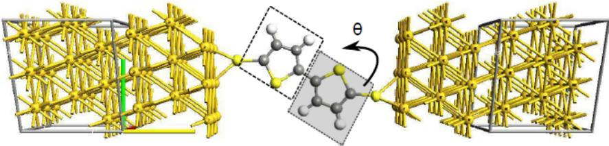
**Figure 3.24:** Dithiol-dithiophenyl (2TT) molecular wire. The plane of OT ring on the left side is fixed while the shaded plane is rotated with respect to the fixed one of an angle  $\theta$ .
