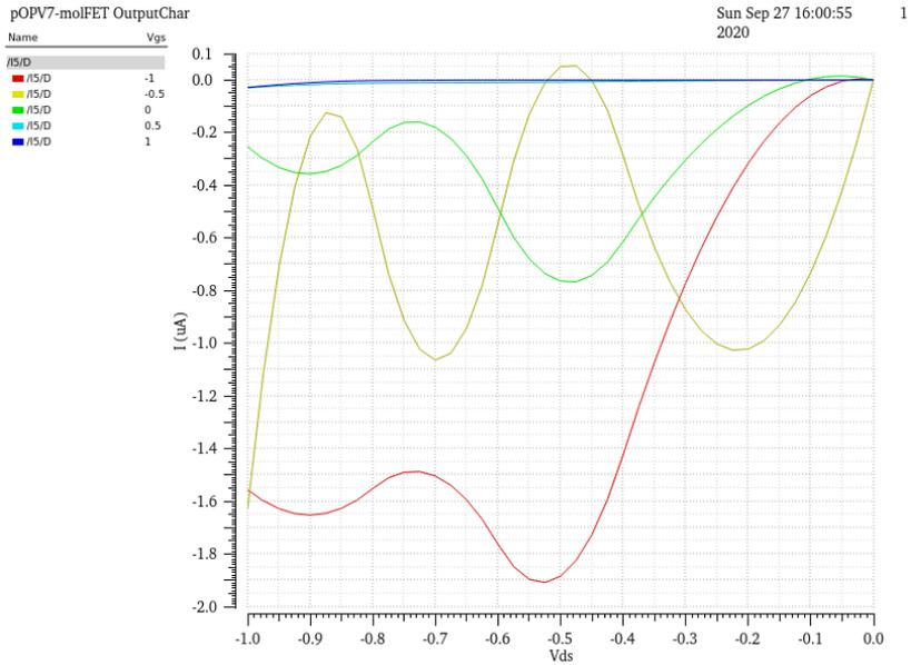
Figure 5.6: Output characteristic of pOPV7-molFET.
