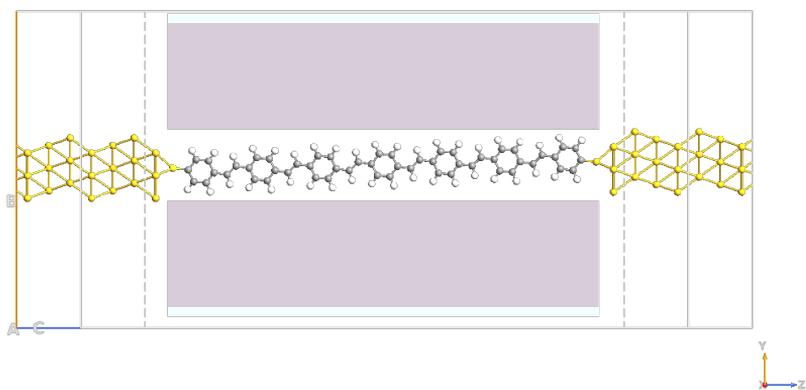
**Figure 4.3:** OPV7 double gate transistor geometry.
