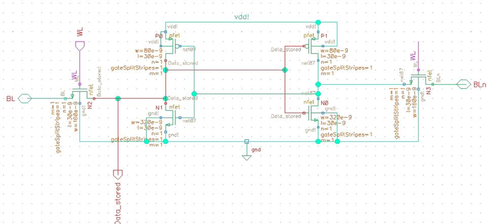
Figure 7.11: 6T SRAM cell Cadence schematic.
