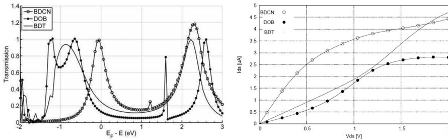
**Figure 3.27:** The equilibrium transmission spectrum on the left side and the resulting current on the right side, in the case of a benzene terminated with thiol (-SH), cyanide (-CN), oxygen (-O) groups.
