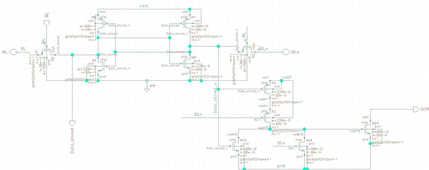
**Figure 8.8:** Static CMOS-like LiM cell Cadence schematic with chosen AR of transistors channel width.
