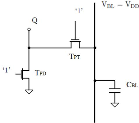
**Figure 7.4:**  $C_{BL}$  is the sum of the parasitic access capacitance of the cells connected to the line (i.e. the drain capacitance of the pass transistor) and the parasitic capacitance of the metal line.
