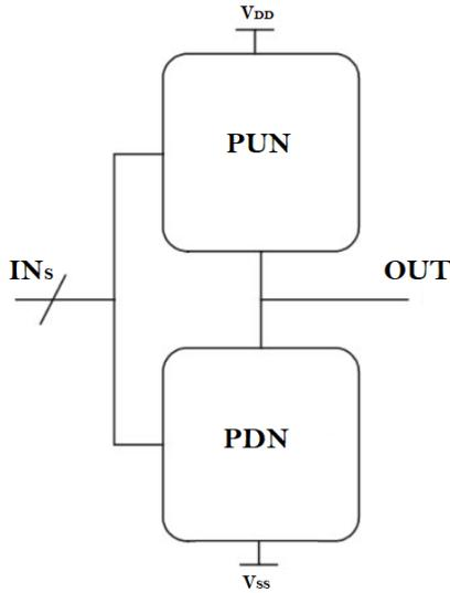
**Figure 6.1:** Conceptual schematic of a static CMOS gate.
