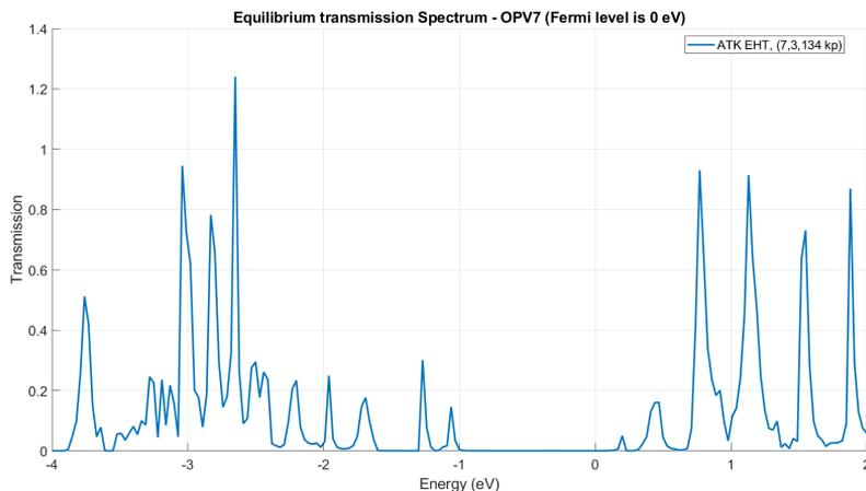
**Figure 4.5:** Equilibrium TS for OPV7 double gate transistor.
