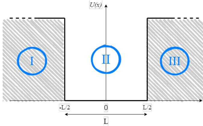
**Figure 2.6:** Potential energy distribution of 1-dimensional finite square well of length  $L$ . The finite height of the well is  $U_0$ .
