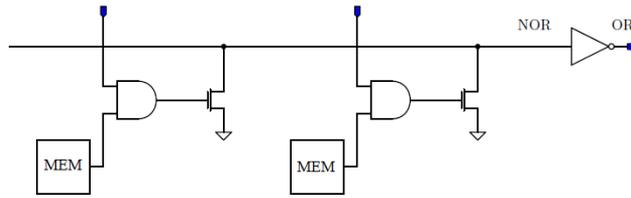
**Figure 8.6:** A row of memory array where all the LiM cells share the same wired-OR line.
