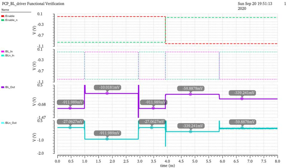
**Figure 7.25:** Spectre functional verification of bitline driver circuits implemented with PCP-MolFET technology.
