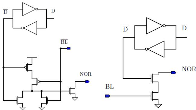
**Figure 8.5:** The two different LiM cells configurations that will be considered in this chapter. In this figure only the MOSFET-based implementation is shown. The configuration on the left is the one labelled in the following as *Static CMOS-like* since is constituted with AND and OR gates implemented in static CMOS logic. The configuration on the right is the one labelled in the following as *Special purpose*.
