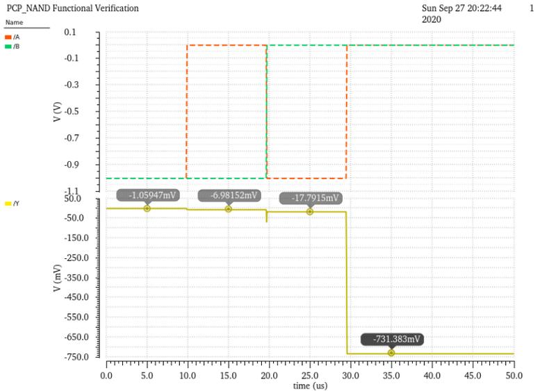
**Figure 6.22:** Functional verification simulation of PCP molFET-based NAND.
