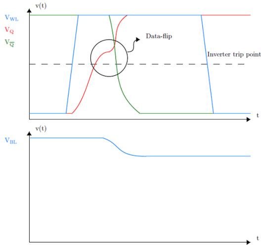
**Figure 7.5:** Data flip of 6T SRAM. The signal  $V_{WL}$  is the voltage applied to the WL (i.e. to the gate of pass transistors),  $V_Q$  the above mentioned voltage on  $Q$  node, and  $\overline{V_Q}$  the complemented one (i.e. the voltage on the opposite inverter  $N2$ ).  $V_{BL}$  is the voltage signal on the bitline connected to the node  $Q$  through the pass transistor  $T_{PT1}$ .
