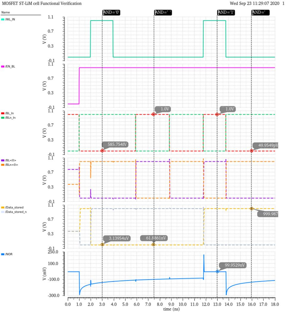
Figure 8.11: Functional verification of the static CMOS-like LiM cell.
