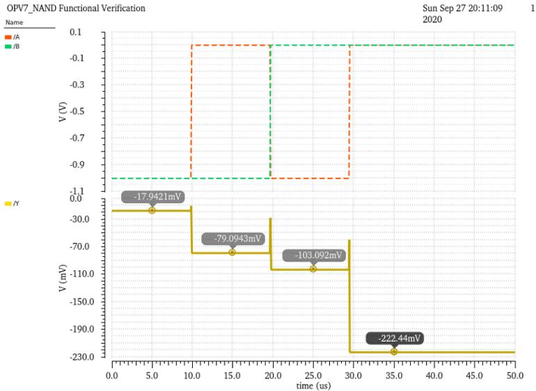
**Figure 6.21:** Functional verification simulation of OPV7 molFET-based NAND.
