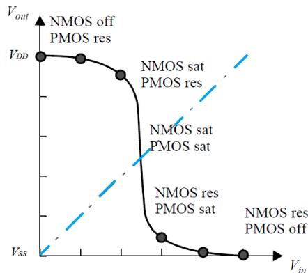
**Figure 6.2:** Voltage-Transfer characteristic (VTC) of the inverter.
