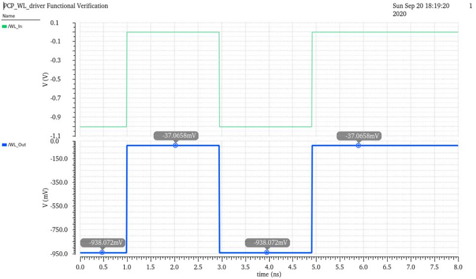
**Figure 7.27:** Spectre functional verification of wordline driver circuit implemented with PCP-MoIFET technology.
