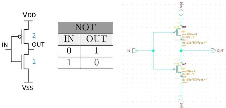
**Figure 6.3:** Conceptual and Cadence schematic of the inverter with transistors properly sized. Also the truth table of the inverter is shown.
