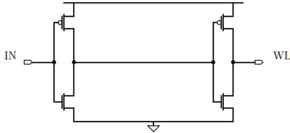
Figure 7.14: In-principle schematic of wordline driver.
