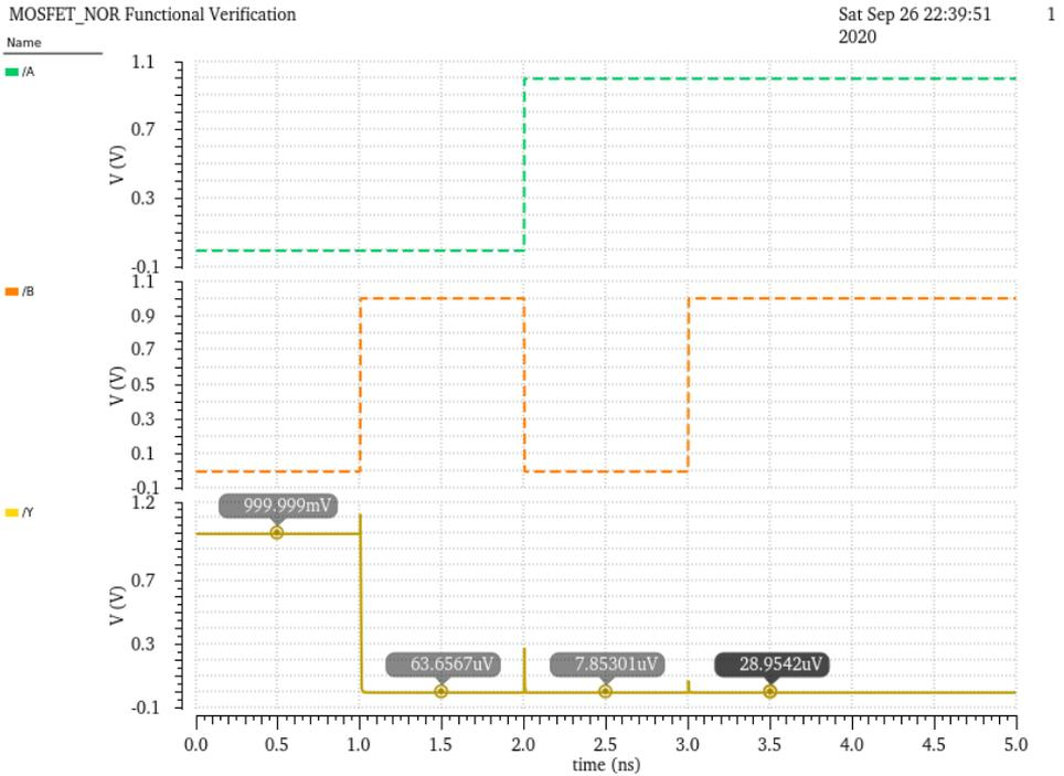
**Figure 6.9:** DC functional verification of the NOR gate. The output correctly follows the NOR truth table.  $A$  (green dash line) and  $B$  (orange dash line) are the inputs.  $Y$  (yellow solid line) is the output.
