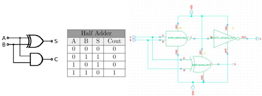
**Figure 6.12:** Conceptual and Cadence schematic of the HA. Also the truth table of the HA is shown.
