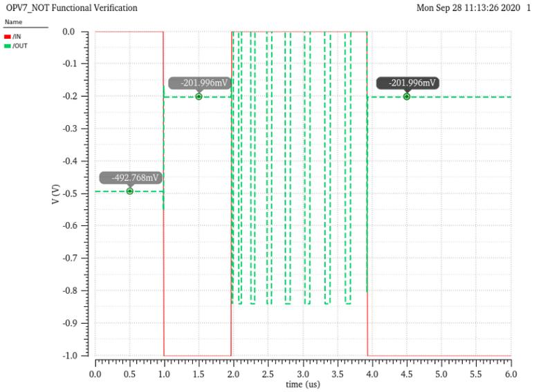
**Figure 6.18:** Functional verification simulation of OPV7 molFET-based inverter.
