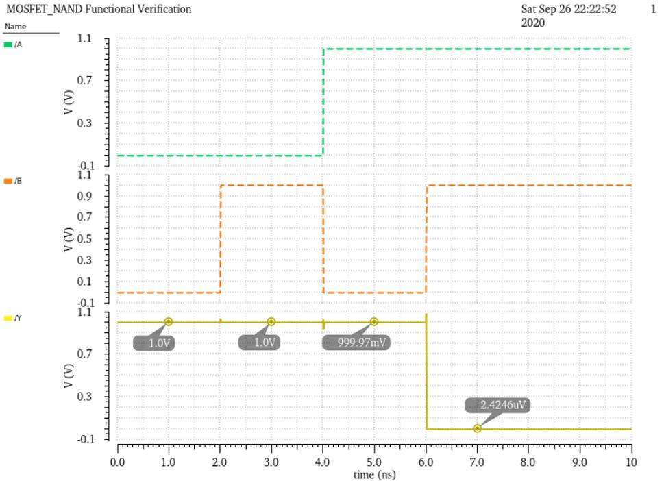
**Figure 6.7:** DC functional verification of the NAND gate. The output correctly follows the NAND truth table. *A* (green dash line) and *B* (orange dash line) are the inputs. *Y* (yellow solid line) is the output.
