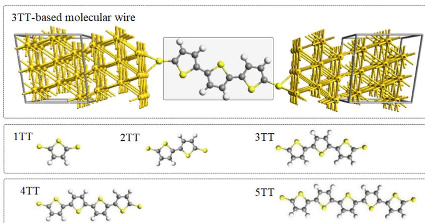
**Figure 3.21:** On top a typical structure of molecular junction. The molecule represented in the scattering region is the dithiol-trithiophenyl (3TT) Thiophene. On the bottom different OT molecules with increasing number of rings.
