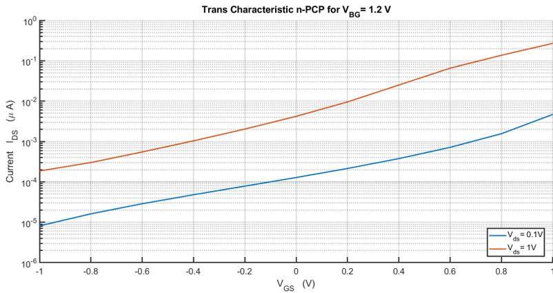
**Figure 4.12:** Trans-characteristic of n-PCP MolFET. Here the deviations wrt conventional MOSFET are very evident: the DIBL at 1V is almost of the order of  $10^2$ . On the other hand, in this range is it possible to better define the threshold voltages (that are evidently subjected to roll off) and the SS that could be defined in a more or less linear portion of bias.
