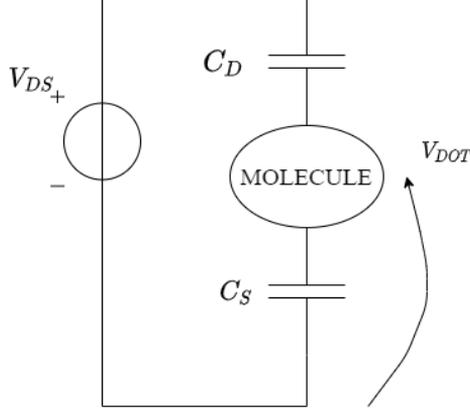
**Figure 2.22:** Equivalent circuitual model of two-probe 0D-system.
