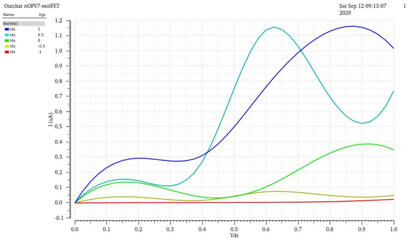
Figure 5.5: Output characteristic of nOPV7-molFET.
