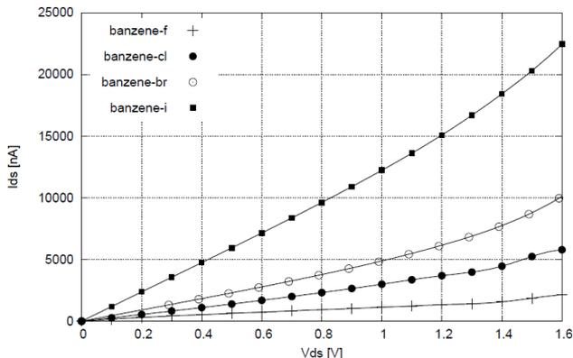
**Figure 3.29:** The drain current of the molecular wire in the case of a benzene terminated with Fluorine F (crosses line), chlorine Cl (full dotted line), bromine Br (empty dotted line) and iodine I (square dotted line).
