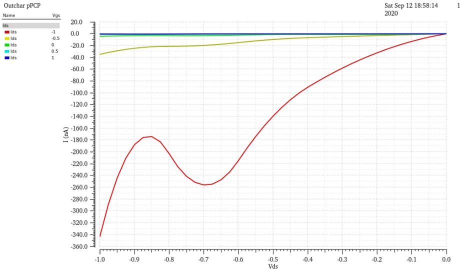
Figure 5.4: Output characteristic of pPCP-molFET.
