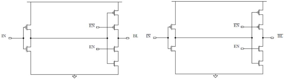
**Figure 7.12:** Schematic of bitline drivers.
