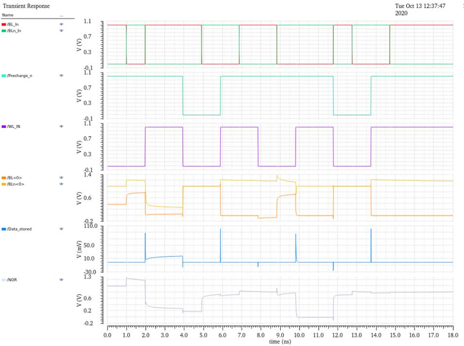
Figure 8.13: Functional verification of the static LiM cell. Case (a).
