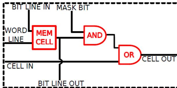
Figure 8.3: LiM cell conceptual schematic from [73].
