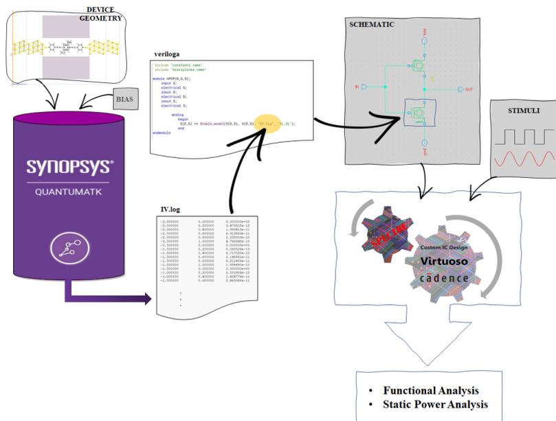
**Figure 5.1:** Methodological flow adopted for functional and static analysis of molFET-based circuit.
