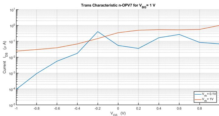
**Figure 4.8:** Trans-characteristic of n-OPV7 MolFET in log scale. Are evident the deviations wrt conventional MOSFET: there is not a well defined threshold voltage especially for the transchar at  $V_{DS} = 0.1V$  and moreover a prominent DIBL is present. The SS that could be defined in a more or less linear portion of bias, is it too low due to the tiny  $I_{on}/I_{off}$  ratio. This will obviously impact at architectural level.
