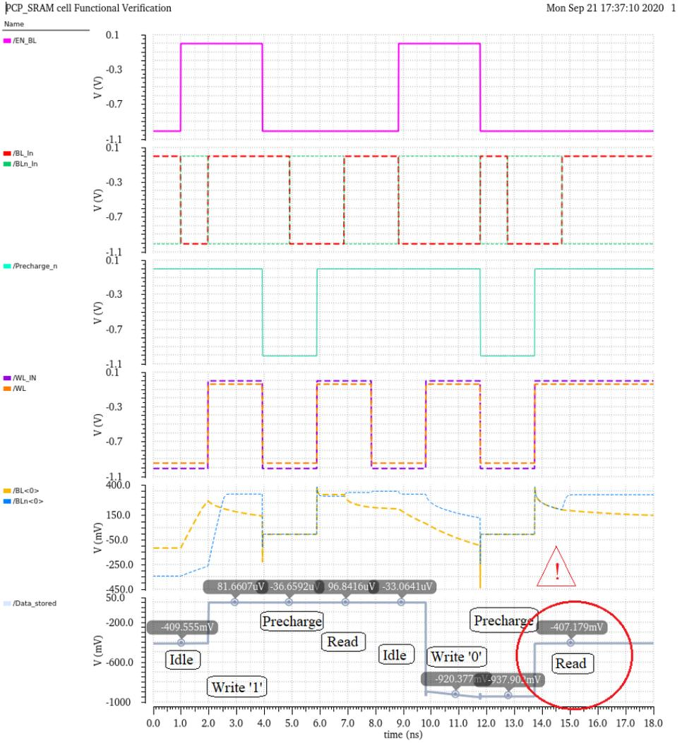
**Figure 7.30:** Spectre functional verification of a single cell of implemented with PCP-MolFET technology.
