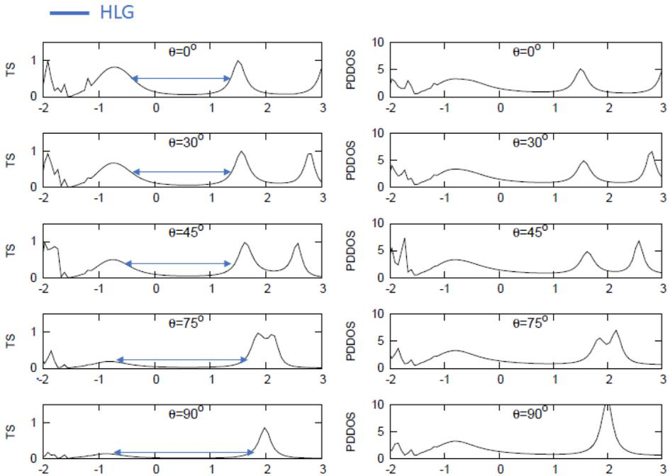
**Figure 3.25:** Equilibrium Transmission spectra and Projected density of states (PDDOS) of 2TT molecule with different degrees of inter-ring torsion. For all molecular systems the average Fermi-level is placed at 0 eV. The peaks on the left side of the Fermi level are the HOMOs and on the right are the LUMOs. Both transmission spectrum and PDDOS are deeply affected by inter-ring torsion angle. The transmission peaks and PDDOS peaks of HOMOs visibly decrease by increasing the torsion angle.
