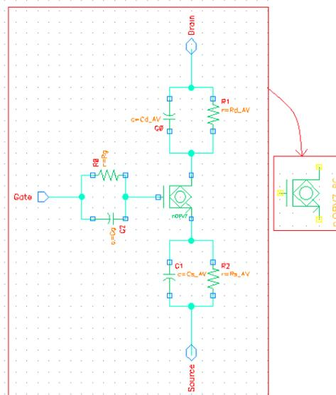
**Figure 5.7:** MolFET circuitual model including  $C_g$ ,  $C_s$ ,  $C_d$ ,  $R_g$ ,  $R_s$  and  $R_d$  and corresponding circuit symbol. In this case the nOPV7-based molFET is considered. It is analogous for the other cases.
