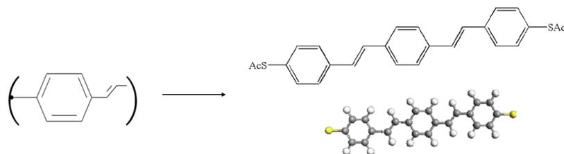
**Figure 3.18:** Elementary block of OPV, made of a phenyl- and vinyne functional groups. On the right side, a chain of three OPVs ended with thiol (OPV3): dithiol-3oligovynil.
