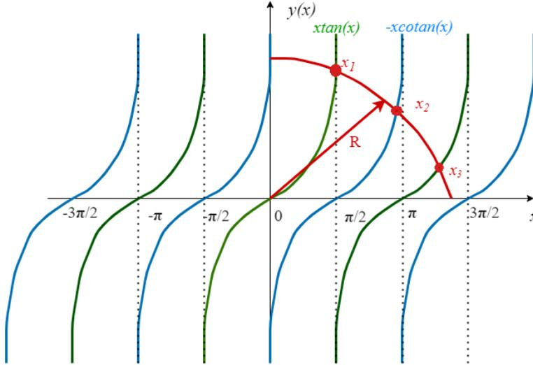
**Figure 2.7:** Graphical representation of the non trivial solutions of the considered 1D finite square well. The red curve is the circle of radius  $R = \sqrt{\frac{2m^*}{\hbar^2} U_0} (L/2)$ . Notice that in the figure there are only three allowed non trivial solutions  $(x_1, x_2, x_3)$
