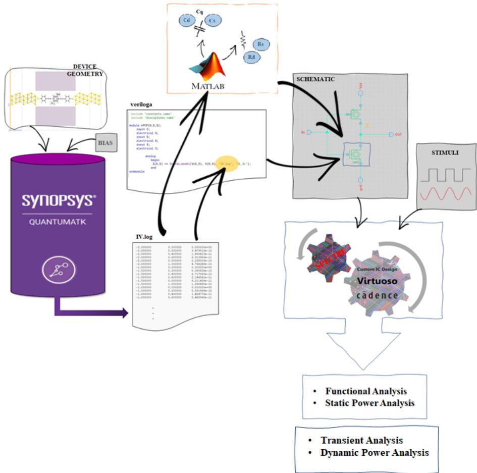
**Figure 5.8:** The definitive methodological flow adopted for functional, static and dynamic analysis of molFET-based circuits
