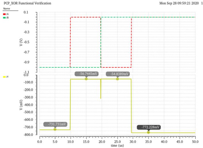
**Figure 6.26:** Functional verification simulation of PCP molFET-based XOR.
