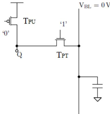
**Figure 7.7:** Voltage divider between the pull-up and pass transistors.
