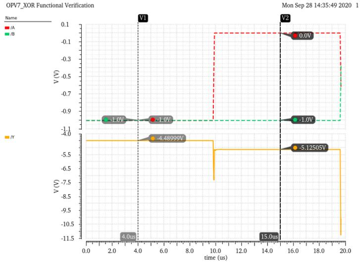
**Figure 6.25:** Functional verification simulation of OPV7 molFET-based XOR. After  $20\mu\text{s}$  the convergence is no more reached.
