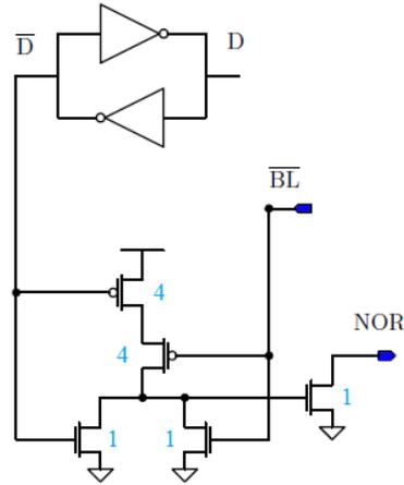
**Figure 8.7:** Static CMOS-like LiM cell with chosen AR of transistors channel width. Only the bistable ring of the SRAM cell is shown, pass transistors and surrounding WLs and BLs are omitted for sake of clarity.
