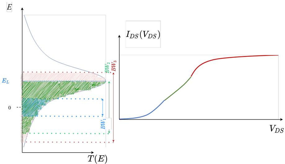
**Figure 3.10:** Transmission spectrum profile  $T(E)$  on the left side and the corresponding drain current on the right side. The Fermi level of the system is placed at the reference value 0.
