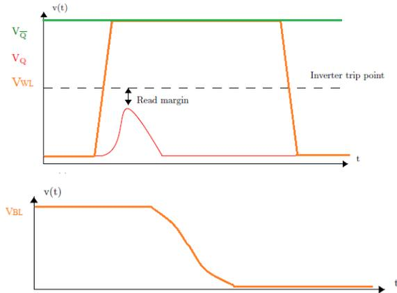
**Figure 7.6:** No data flip of 6T SRAM. The bitline  $V_{BL}$  is discharged to the logic '0'.
