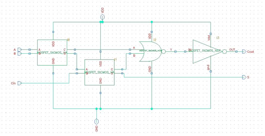
**Figure 6.15:** Cadence schematic of the FA.
