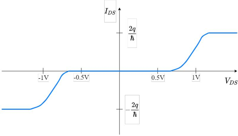
**Figure 2.18:** The resulting IV curve for LUMO conduction.
