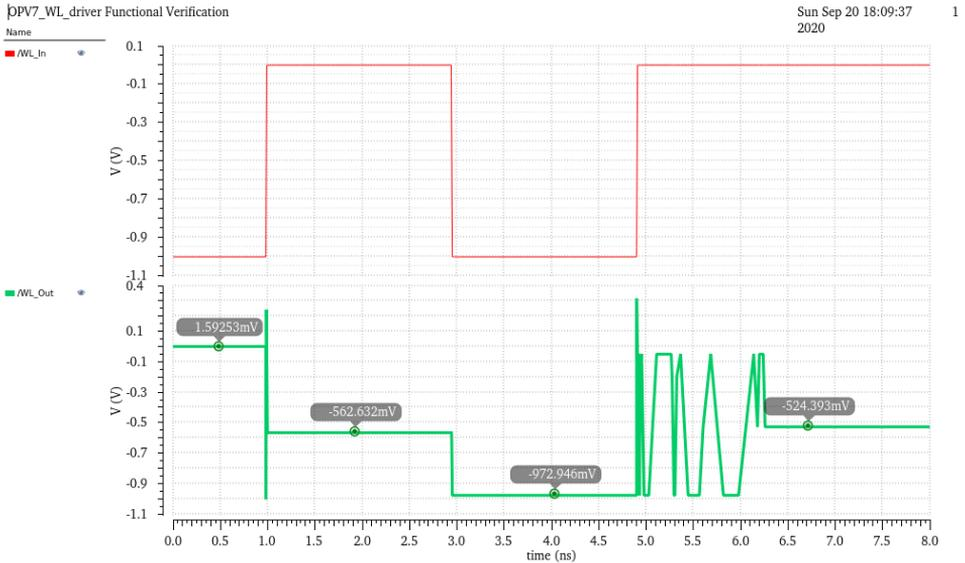
**Figure 7.26:** Spectre functional verification of wordline driver circuit implemented with OPV7-MoFET technology.
