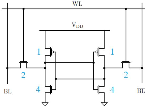
Figure 7.10: 6T SRAM cell schematic with the chosen transistor aspect ratios.
