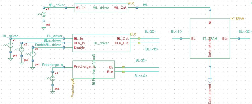
**Figure 7.21:** Cadence RTL schematic of a single cell of SRAM and surrounding driving circuitries.
