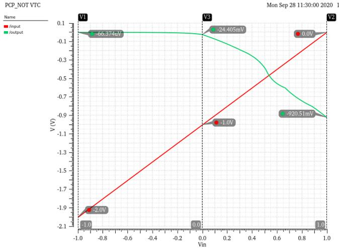
**Figure 6.19:** Simulated VTC of PCP molFET-based inverter. The red line is the input voltage  $V_{in}$  and the green one the output  $V_{out}$ .
