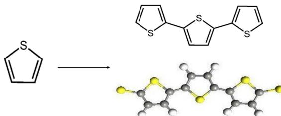
**Figure 3.19:** Elementary block of OT. On the right side, a chain of three OTs ended with thiol (3TT): dithiol-3thiophene.
