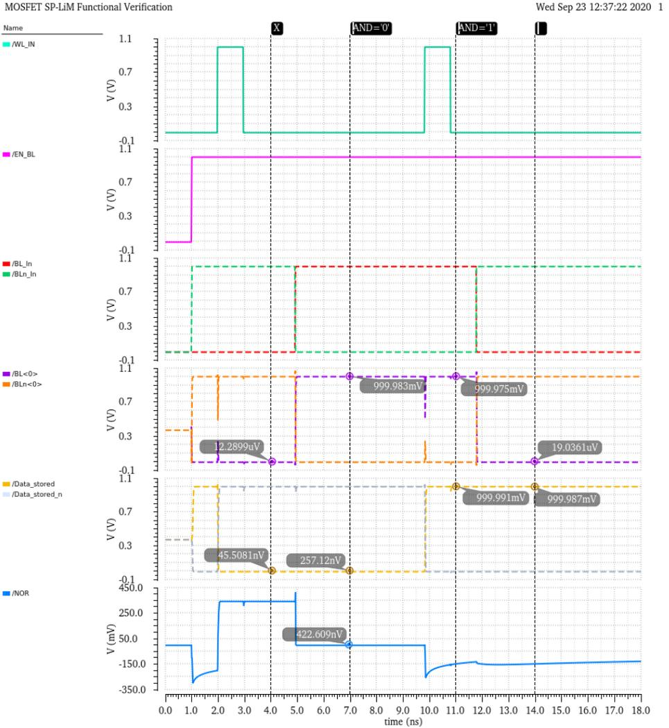
Figure 8.12: Functional verification of the special purpose LiM cell.
