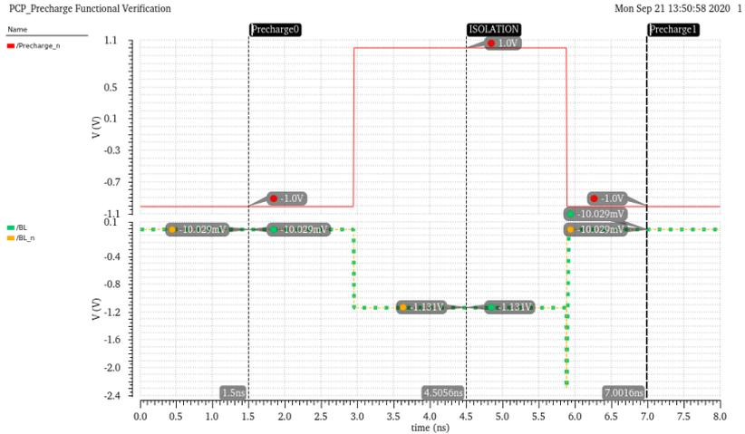
**Figure 7.29:** Spectre functional verification of precharge circuit implemented with PCP-MolFET technology.
