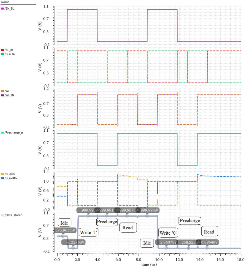
**Figure 7.22:** Spectre functional verification of a single cell of implemented with MOSFET technology.
