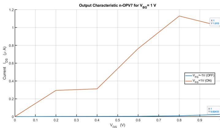
**Figure 4.7:** Output characteristic of n-OPV7 MolFET. A ratio  $I_{on}/I_{off} \simeq 42$  is achieved. There is a little Negative differential resistance (NDR) trend, that poses the question how this trend will impact at circuitual level (for e.g. case of CMOS-like inverter in inversion region?).
