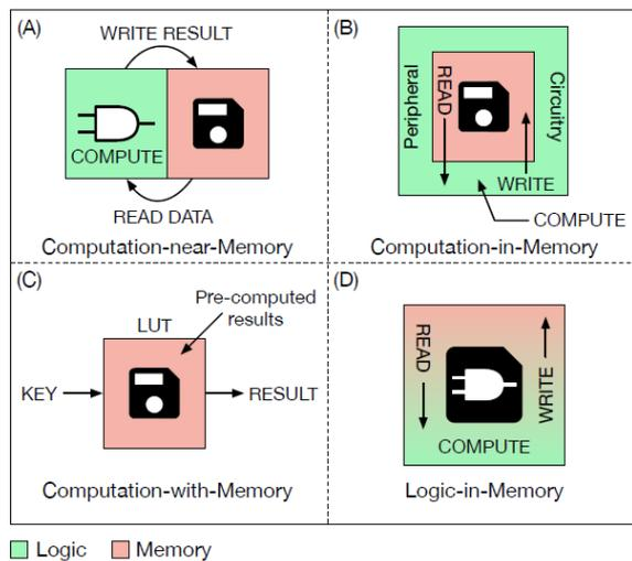
**Figure 8.1:** Different iMC approaches from [69]. Depending on how the memory is used for computing data, four main in-memory computing approaches can be defined. (A) Computation-near-Memory (CnM), (B) Computation-in-Memory (CiM), (C) Computation-with-Memory (CwM), (D) Logic-in-Memory (LiM).
