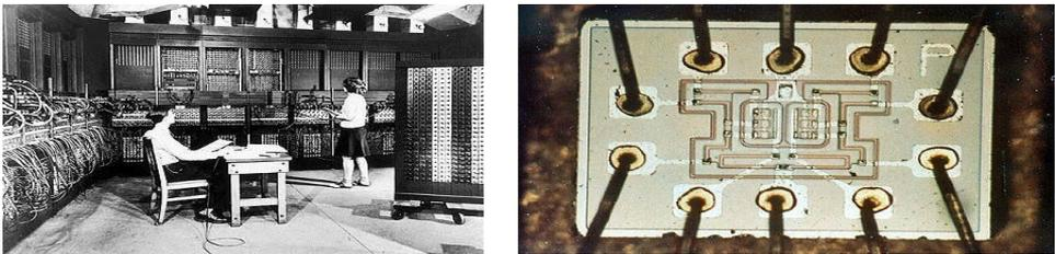
**Figure 1.1:** On the left: a photo of the ENIAC. On the right: the NOR gate chip implemented with RTL (Resistor-Transistor Logic) used to build Apollo guidance computer.
