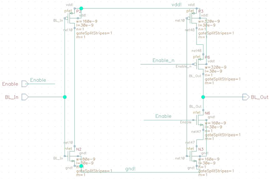
**Figure 7.13:** Cadence schematic of straight bitline driver.
