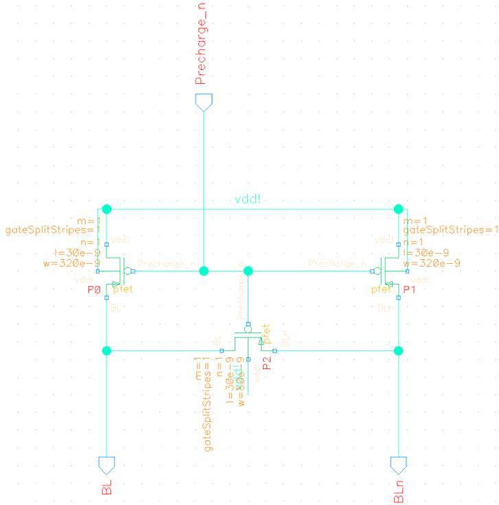
Figure 7.17: Cadence schematic of precharge circuit.
