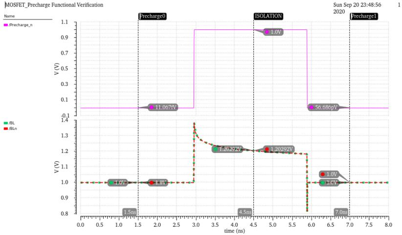
**Figure 7.20:** Spectre functional verification of precharge circuit implemented with MOSFET technology.
