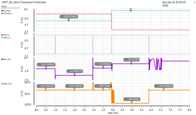
**Figure 7.23:** Spectre functional verification of bitline driver circuits implemented with OPV7-MolFET technology.
