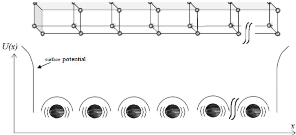
**Figure 2.1:** The 1D potential energy of the crystal lattice, periodic function of the space. It results from the periodic placement of the ions lattice within the crystal. The distance between one ion and the next is the lattice constant  $a$ .
