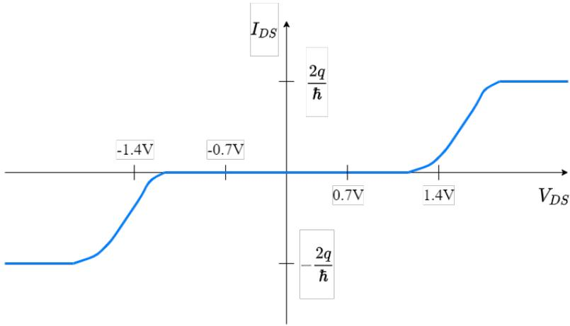
**Figure 2.19:** The resulting IV curve for HOMO conduction.
