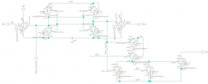
**Figure 8.10:** Special purpose LiM cell Cadence schematic with chosen AR of transistors channel width.
