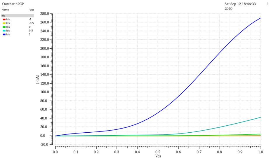
**Figure 5.3:** Output characteristic of nPCP-molFET.
