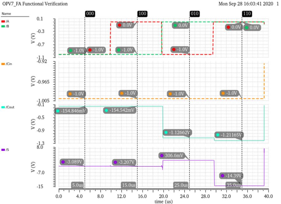
**Figure 6.29:** Functional verification simulation of OPV7 molFET-based FA.
