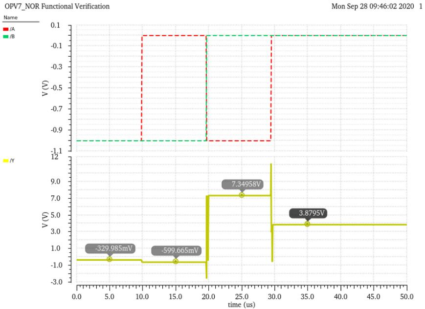
**Figure 6.23:** Functional verification simulation of OPV7 molFET-based NOR.
