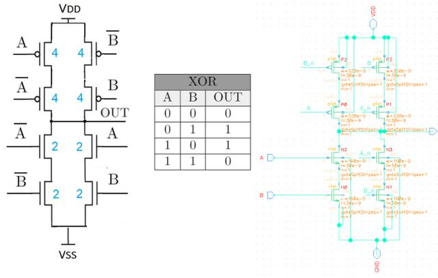
**Figure 6.10:** Conceptual and Cadence schematic of the XOR with transistors properly sized. Also the truth table of the XOR is shown.
