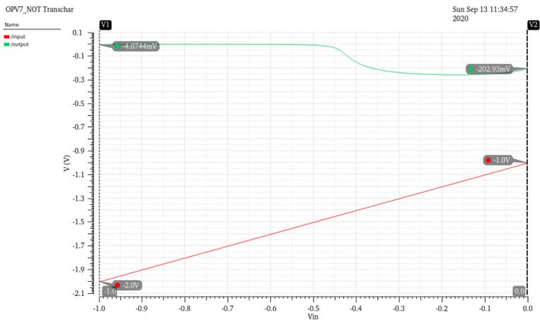
**Figure 6.17:** Simulated VTC of OPV7 molFET-based inverter. The red line is the input voltage  $V_{in}$  and the green one the output  $V_{out}$ .
