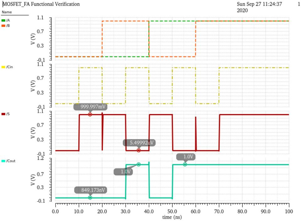
Figure 6.16: DC functional verification of the FA. Glitches are present.
