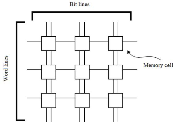
**Figure 7.3:** A typical in principle schematic of 1D memory array. Each square is a 6T memory cell. Additional circuitries like address decoder or I/O circuitry are omitted.
