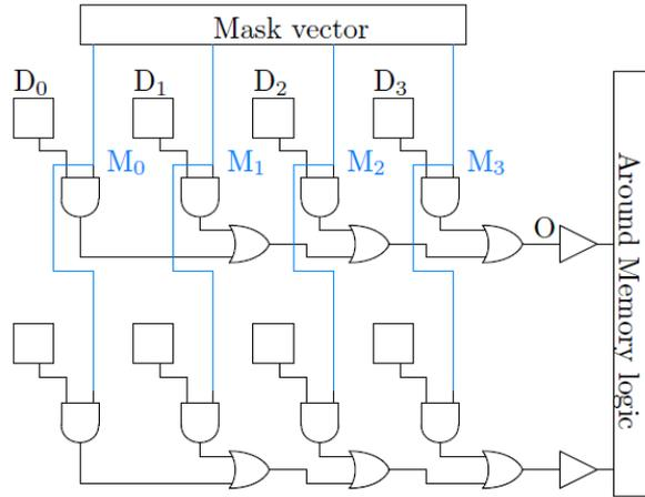
**Figure 8.4:** Memory array conceptual schematic, where  $D_i$  denotes the  $i$ -th bit of the datum stored and  $M_i$  the  $i$ -th bit of the mask vector.
