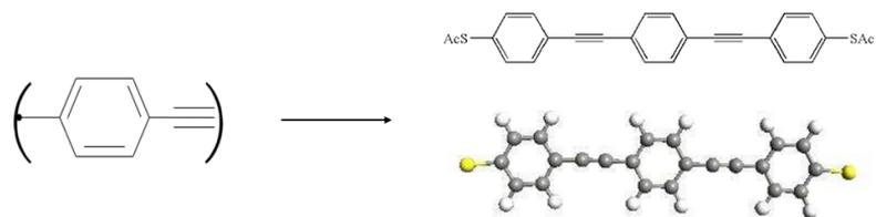
**Figure 3.17:** Elementary block of OPE, made of a phenyl- and ethynylene ( $-C\equiv C-$ ) functional groups. The phenyl one is a benzene ring derivative without either 1 if the point in the figure is the beginning of the chain, or 2 atoms of H if it is in the middle of the chain. On the right side a chain of three Oligo Phenylyne Ethynylene ended with thiol (OPE3).
