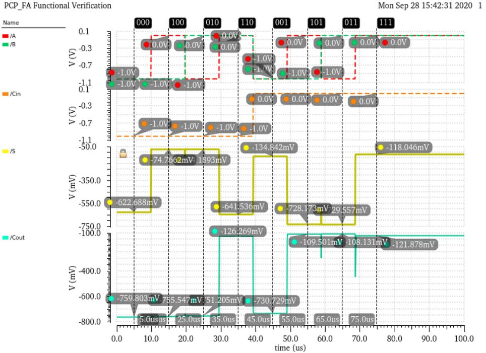
Figure 6.30: Functional verification simulation of PCP molFET-based FA.
