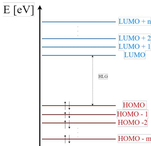
**Figure 3.13:** An example of energy levels distribution of MOs of a molecule. The energy level  $HOMO - m$  is the ground states. All the HOMO levels are occupied at equilibrium, whereas the LUMO levels are unoccupied.
