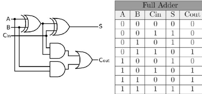
**Figure 6.14:** Conceptual schematic and truth table of the FA.
