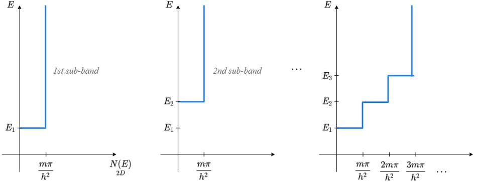
**Figure 2.12:** DOS of 2D system. On the left side the ones for single sub-bands. On the right side 2D-DOS for the entire system, resulted from the sum of DOS of all the sub-bands.
