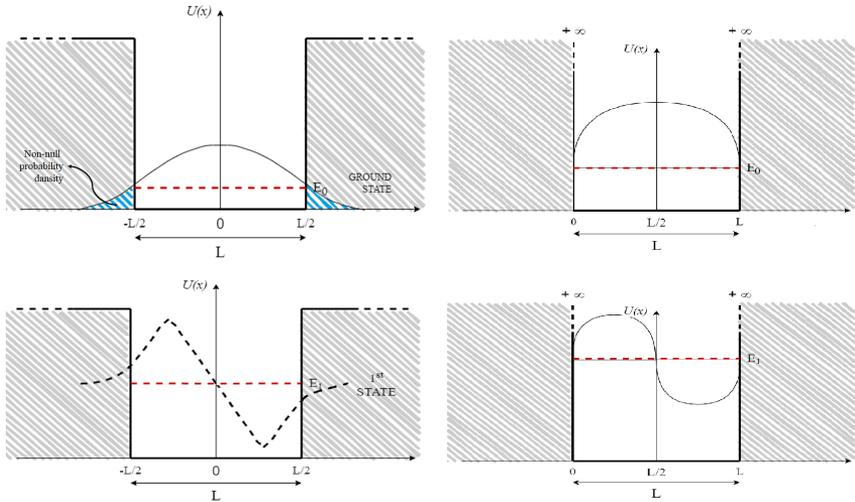
**Figure 2.9:** Differences in the first two energy levels between a 1D ideal finite square well and an infinite one.
