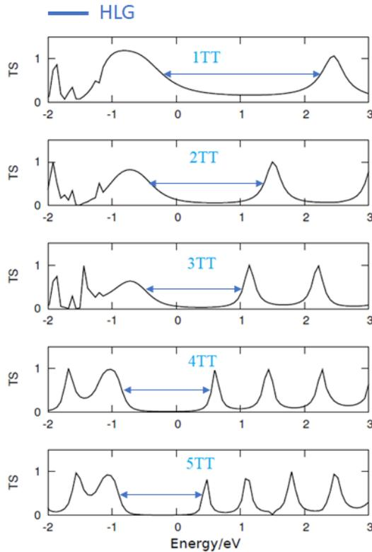
**Figure 3.22:** Equilibrium Transmission spectra of thiophene molecule with different number of rings. For all molecular systems the average Fermi-level is placed at 0 eV. The peaks on the left side of the Fermi level are the HOMOs and on the right are the LUMOs.
