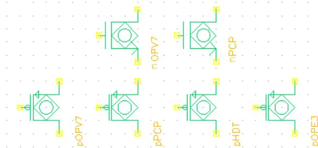
**Figure 5.2:** Circuit symbols for molFETs: on the top the nOPV7 and nPCP molFETs; on the bottom pOPV7, pPCP, pHDT, pOPE3 molFETs in order from left to right.
