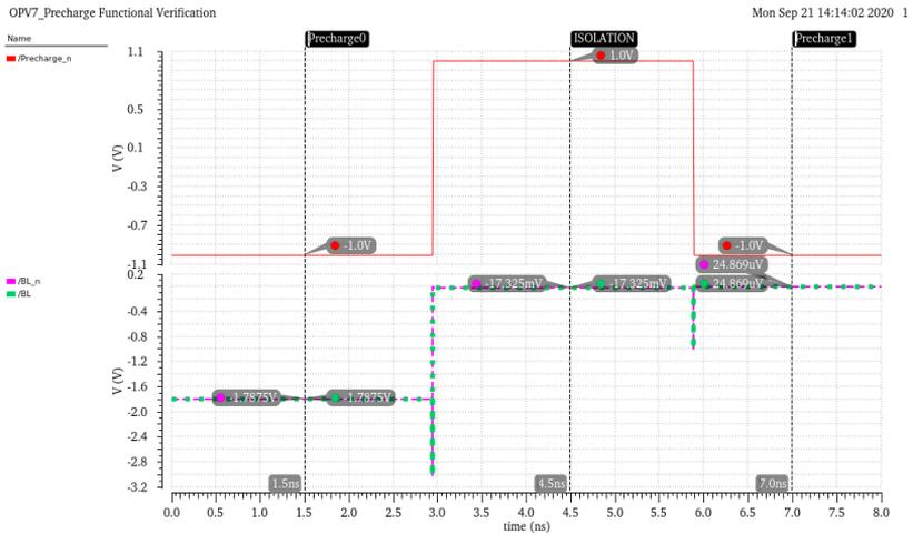
**Figure 7.28:** Spectre functional verification of precharge circuit implemented with OPV7-MoIFET technology.
