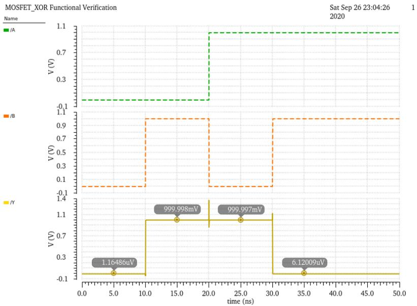
**Figure 6.11:** DC functional verification of the XOR gate. The output correctly follows the XOR truth table. *A* (green dash line) and *B* (orange dash line) are the inputs. *Y* (yellow solid line) is the output.
