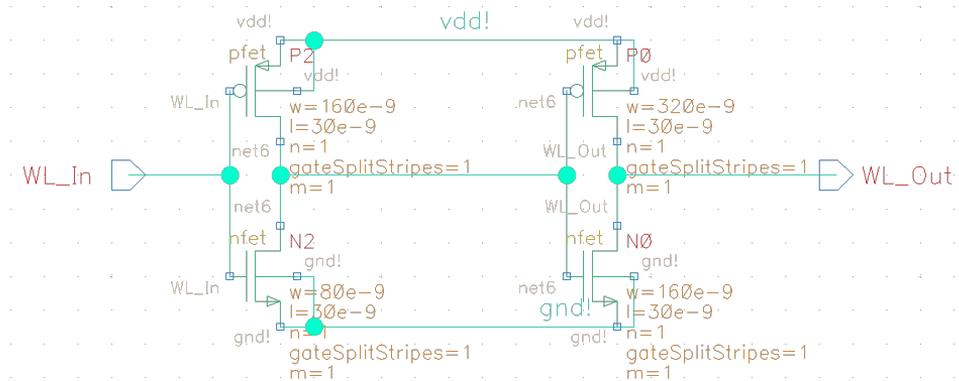
Figure 7.15: Cadence schematic of wordline driver.
