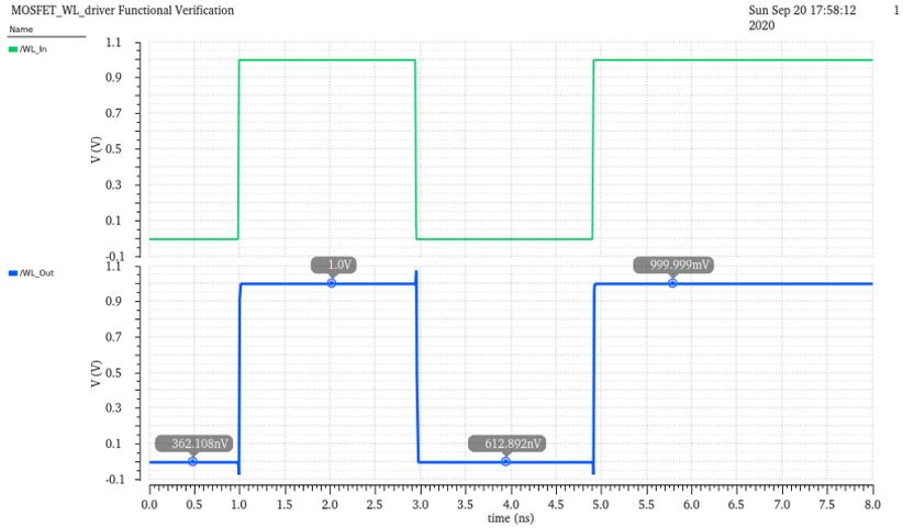
**Figure 7.19:** Spectre functional verification of wordline driver circuit implemented with MOSFET technology.
