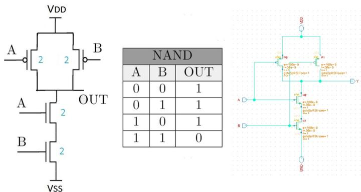
**Figure 6.6:** Conceptual and Cadence schematic of the NAND with transistors properly sized. Also the truth table of the NAND is shown.
