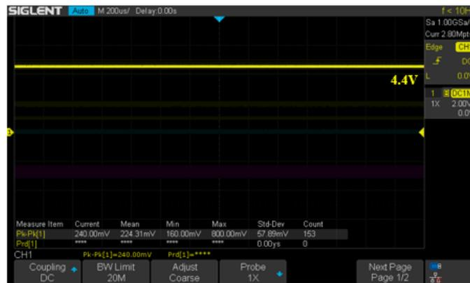
Figure 3.20: Output of the solar cell
