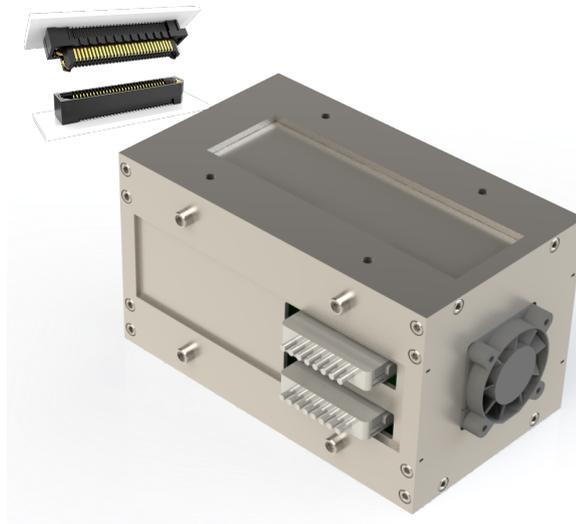
**Figure 4.6:** Final drawing of the sensor case. The chosen dimensions depend mainly on the fan and connectors, and can be easily adjusted according to their availability with suppliers.
