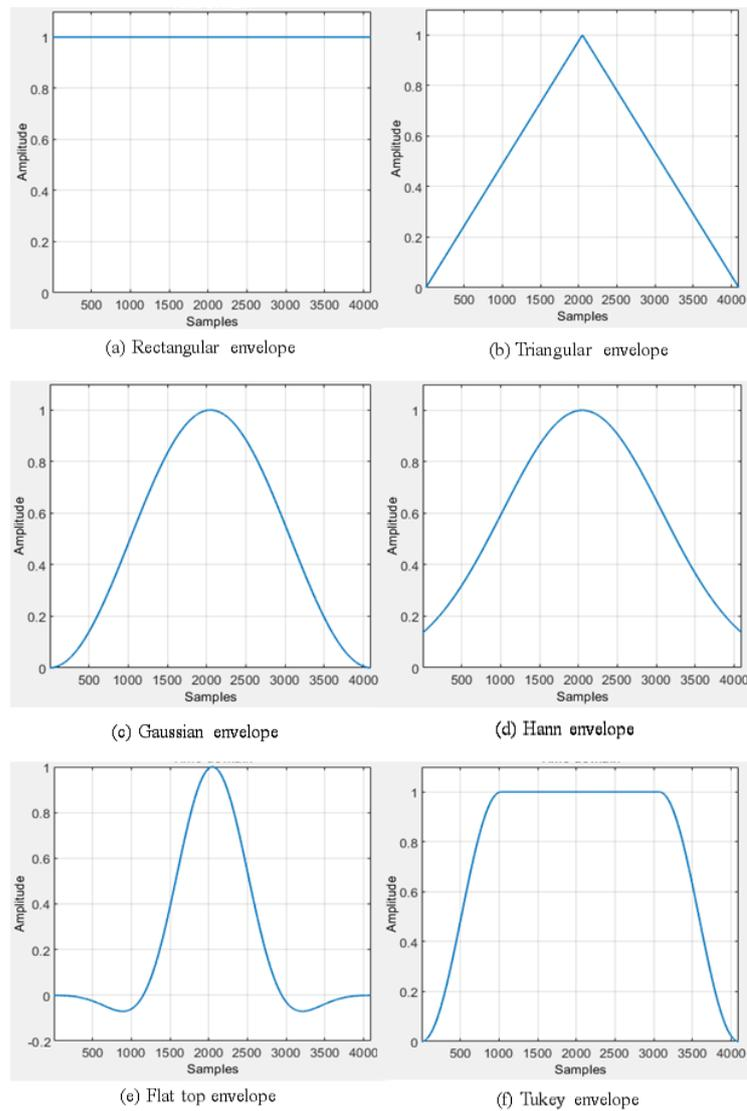
Figure 5.13: Examples of different envelope shapes.
