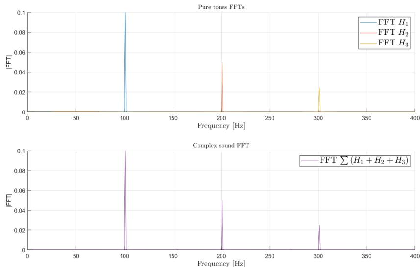
Figure 2.5: Pure tones  $H_1$ ,  $H_2$  and  $H_3$  VS complex sound  $\sum H_1 + H_2 + H_3$ . Frequency domain representation
