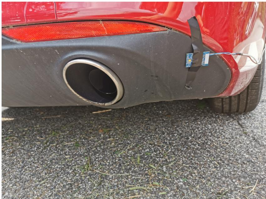
(b) Microphone close to the exhaust pipe
