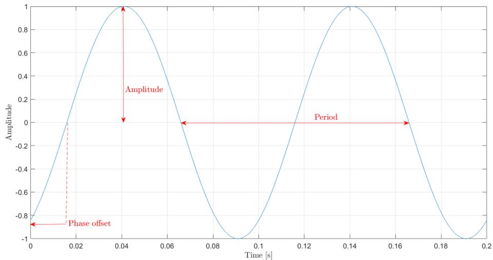
Figure 2.2: Sound wave and its parameters
