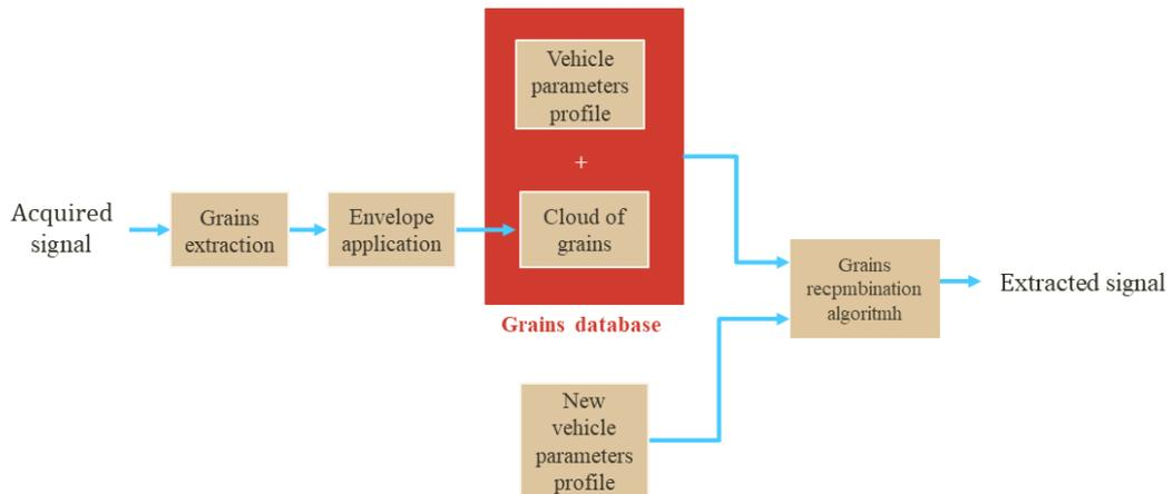
Figure 5.10: Granular synthesis steps
