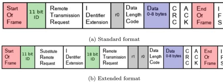
Figure 4.8: CAN data frame structure
