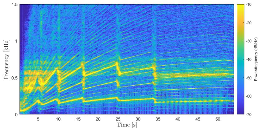
Figure 5.26: Spectrogram with a variable gain proportional to the acceleration on the 1<sup>st</sup> harmonic, constant gain of 20 on the 3<sup>rd</sup> harmonic and 1 otherwise
