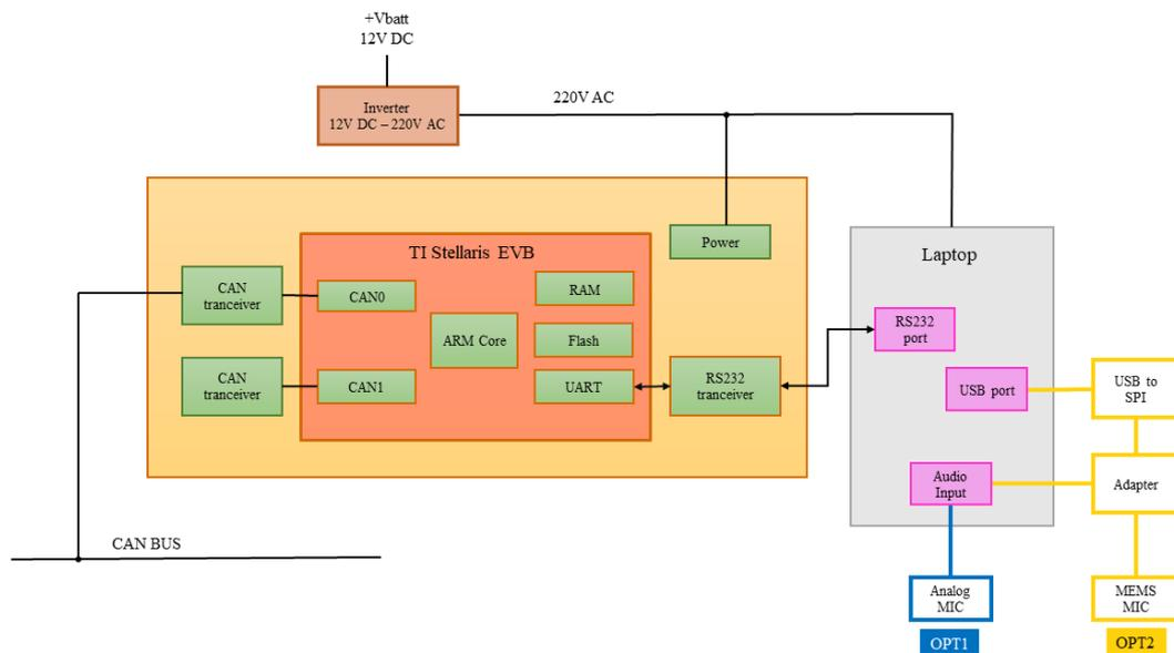
Figure 4.5: CAN messages acquisition system
