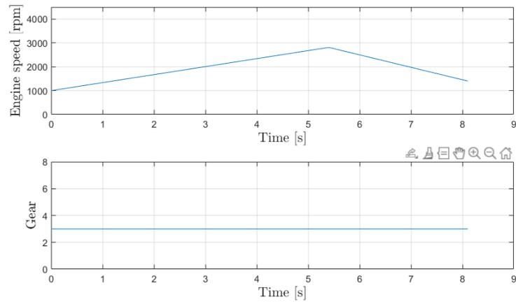
(a) RPM and gear profiles
