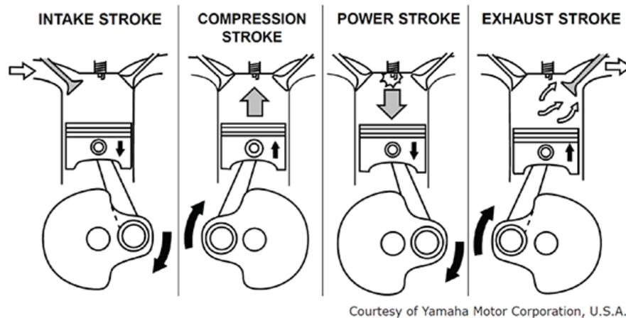
Figure 3.1: Four-stroke engine cylinders
