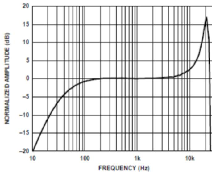
Figure 4.1: MEMS frequency response
