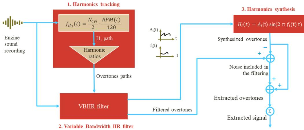
Figure 5.1: Harmonics extraction algorithm
