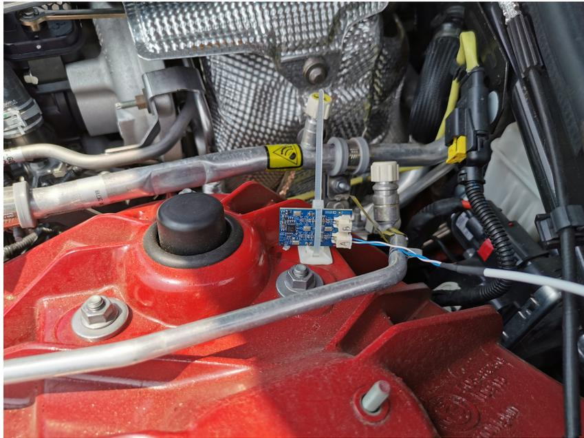
(a) Microphone in the engine compartment
