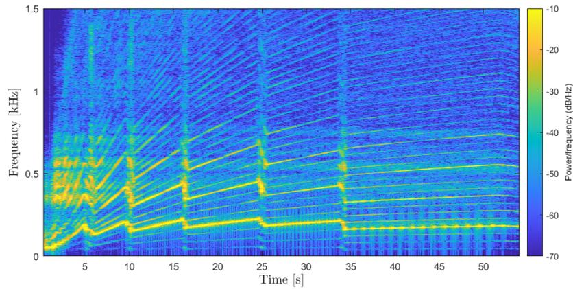
Figure 5.25: Spectrogram with a variable gain proportional to the acceleration on the 1<sup>st</sup> harmonic and 1 otherwise
