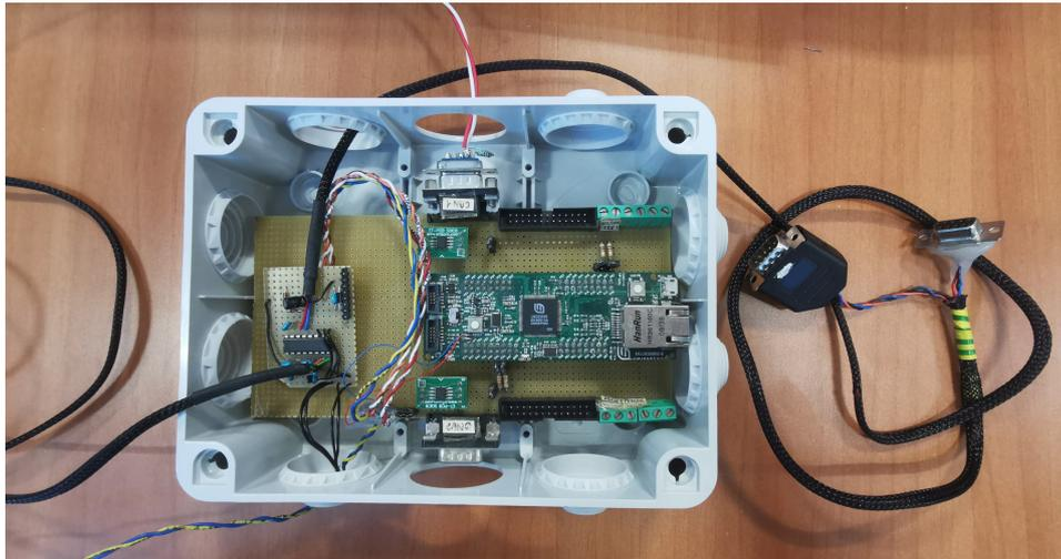
Figure 4.4: CAN messages acquisition system
