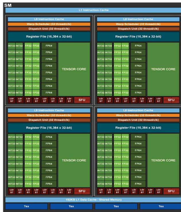
Figure 3.1: Streaming Multiprocessor Architecture [21]
