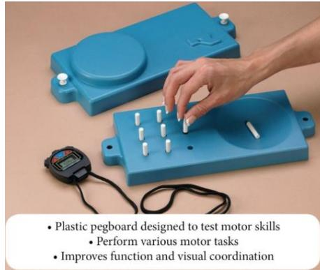
**Figure 2.7:** An example of test kit for NHPT [36]
