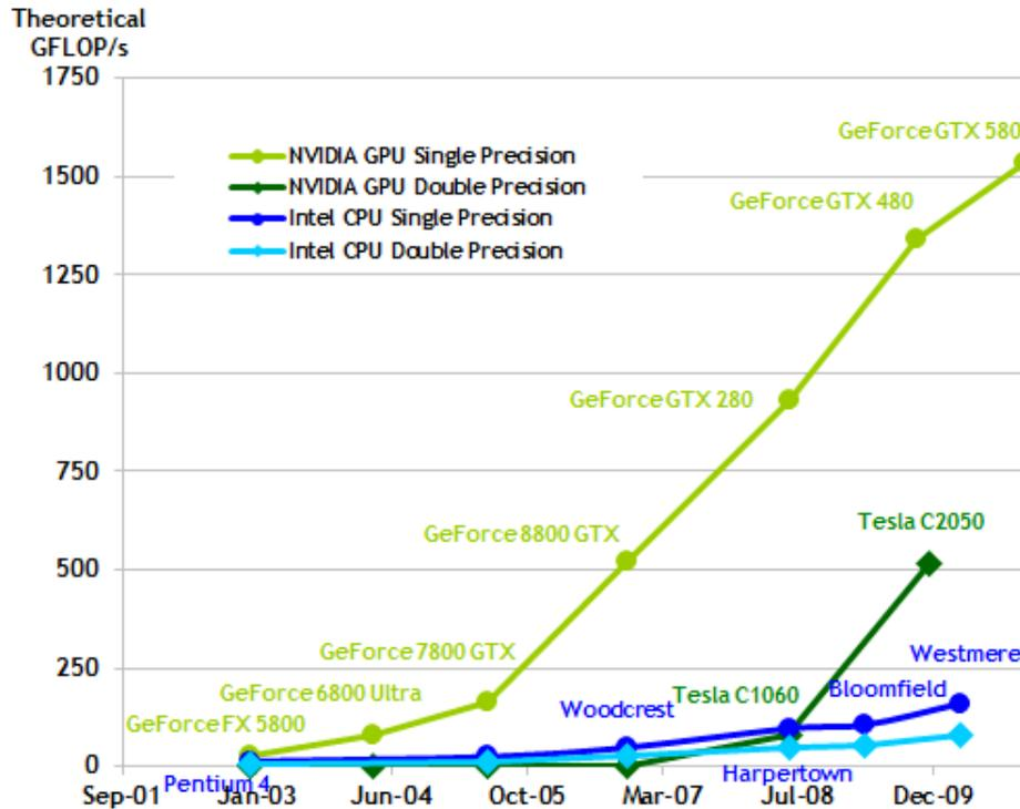
Figure 2.1: GPU vs CPU comparison [3]
