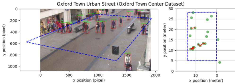
**Figure 2.12:** On the left, video frames output with ROI. On the right, how the BEV looks like. [33]
