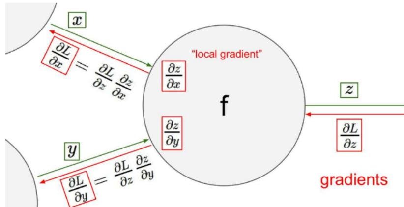
**Figure 2.6:** Gradients computation for each of the the three nodes
