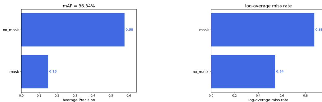
**Figure 4.13:** mAP and lamr for YOLOv4 on surveillance footage
