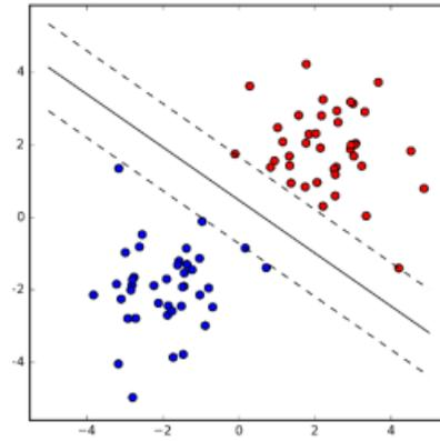
**Figure 2.3:** SVM classifier separates the two classes by the largest margin.
