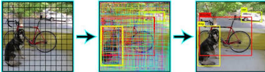
**Figure 2.7:** How YOLO detects and estimates the class object
