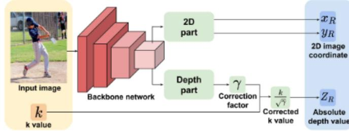
**Figure 3.3:** RootNet architecture
