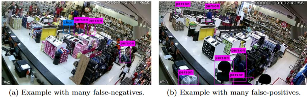
**Figure 2.11:** Inaccurate predictions from YOLO [23]
