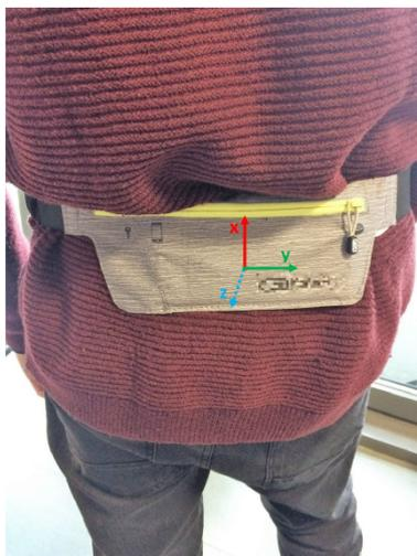
Figure 4: Positioning of the smartphone employed for data recordings. Ref: [15]
