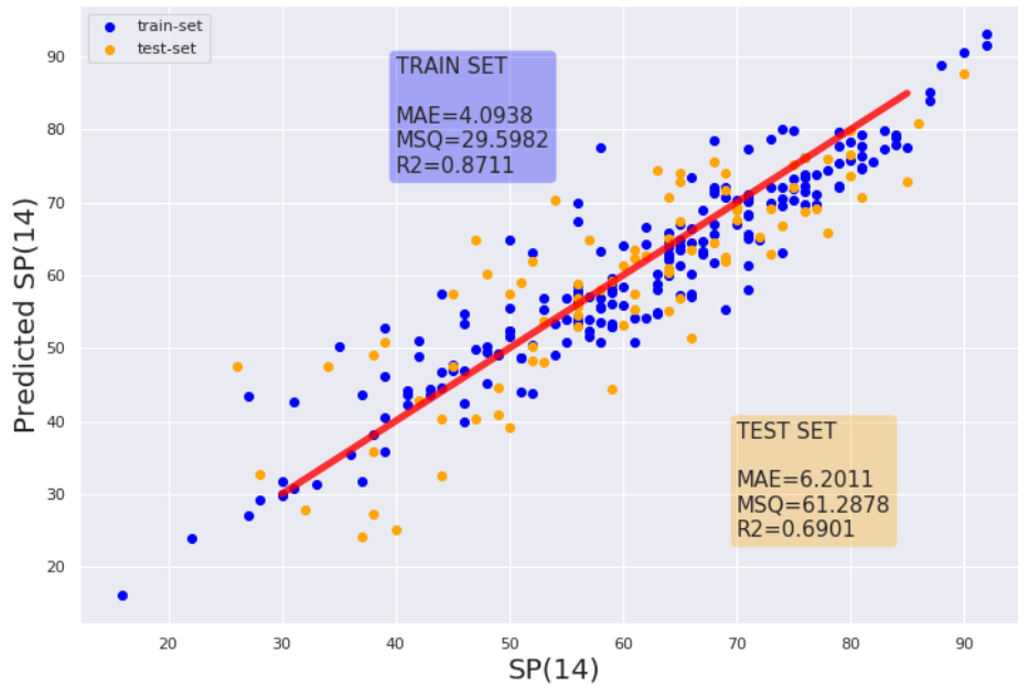
Figure 3.9: Scatter plot between the actual value of the Spotify Popularity index at day 14 (x axis) and its prediction (y axis). In blue the model on the train-set, in orange on the test-set. The red line is the curve y = x .
