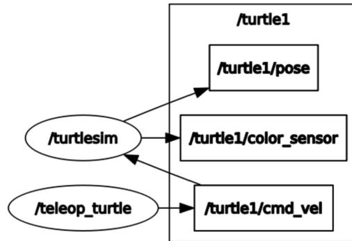
Figure 3.19: Example of graph representing ROS nodes running in a demo application
