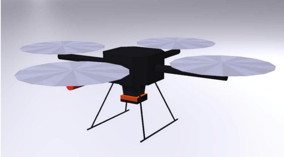
Figure 3.6: Gazebo model of quadrotor UAV implemented in *hector\_quadrotor* package. A Hokuyo UTM-30LX laser scanner is mounted below the main body in this image, but this sensor is not used in this thesis, hence a modified version without it is used.
