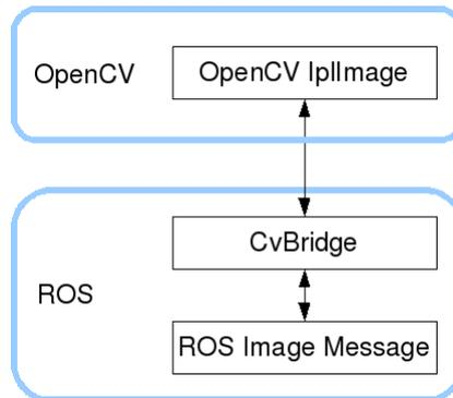
Figure 3.24: CvBridge working principle for translating from ROS Image messages to OpenCV images.
