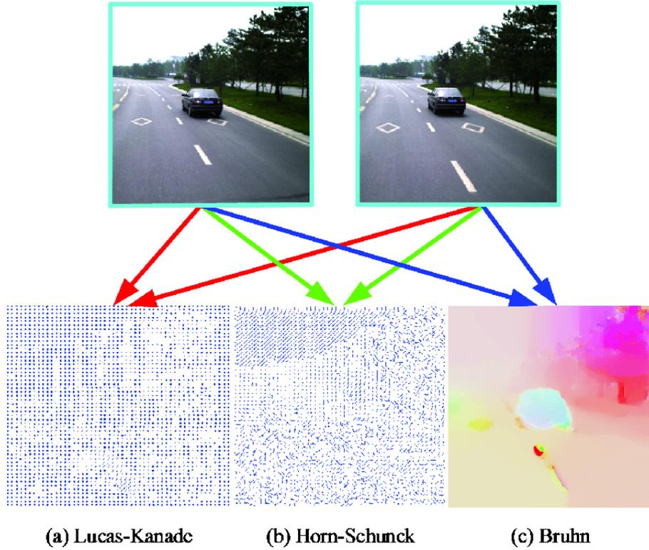
Figure 3.9: The produced optical flow 2D vector field describes the motion of each pixel among subsequent frames. In the picture, taken from [23], results produced from three different algorithms are shown. First two are sparse OF fields while the last one is a dense OF field.
