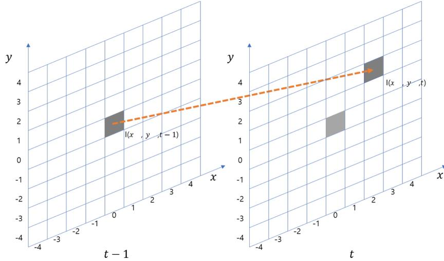
Figure 3.10: The displacement of a pixel obtained among subsequent frame defines the optical flow vector for that specific pixel.
