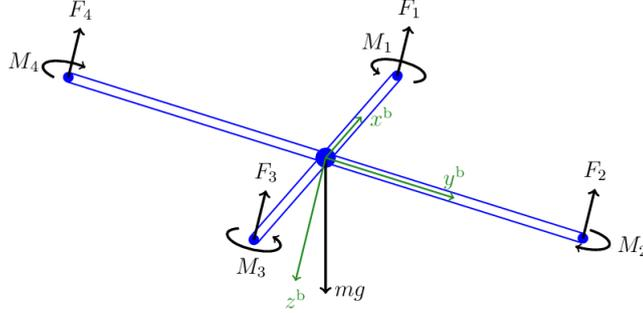
Figure 3.3: Rotations conventions on quadrotor vehicles.
