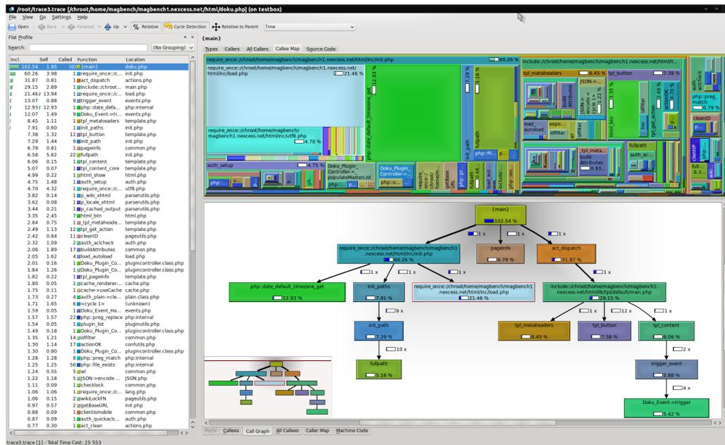
Figure 3.29: KCachegrind is a GUI based tool made for visualizing software profilers outputs, which format is in the form of call graphs. Here a generic example is shown.
