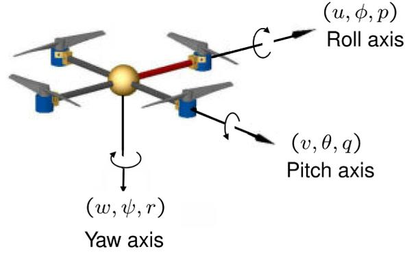
Figure 3.4: States reported on a quadrotor UAV.
