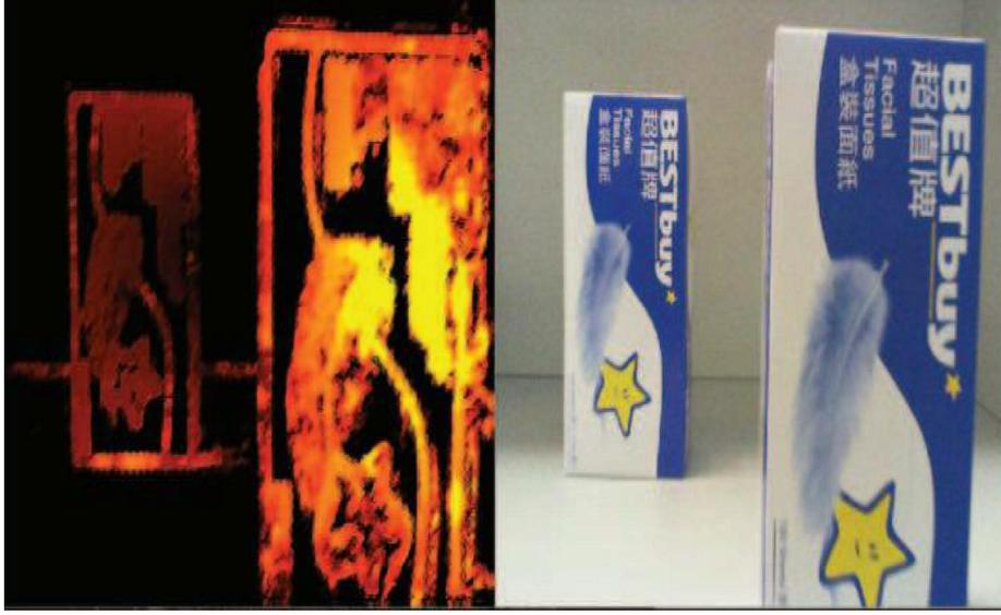
Figure 3.15: On the right, video frame with camera moving forward. On the left, respective elaborated image from TTC computation of the recorded scene. The brighter the pixel, the closer the obstacle. Image from [18].
