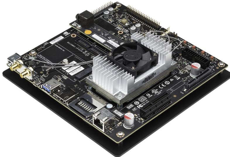
Figure 5.4: NVIDIA Jetson TX1 Development Kit platform for vision computing. The board is hosting the Jetson TX1 module, which offers high computational capabilities with 256 core GPU and low power consumption.
