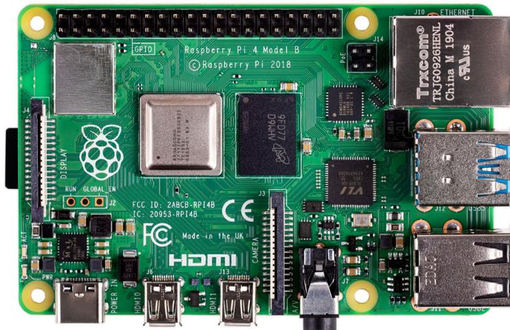
Figure 5.9: RaspberryPi 4 board, a powerful Linux-based embedded system.
