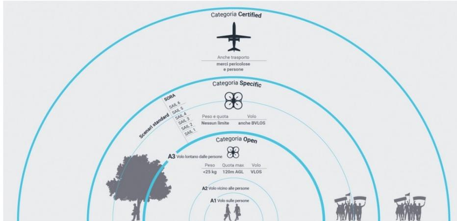
Figure 1.3: UAV classification according to italian ENAC.
