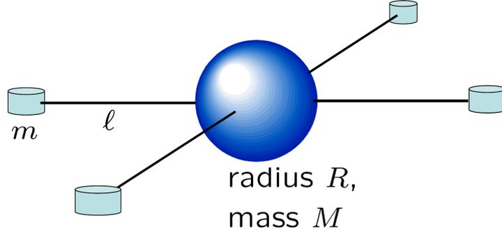
Figure 3.5: Simplified quadrotor model for inertia tensor values computation.
