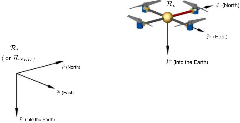
Figure 3.2: The world and the vehicle reference frames.
