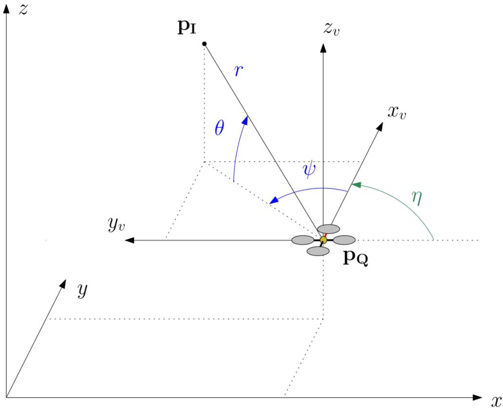
Figure 4.2: Intermediate waypoint computation for obstacle avoidance.
