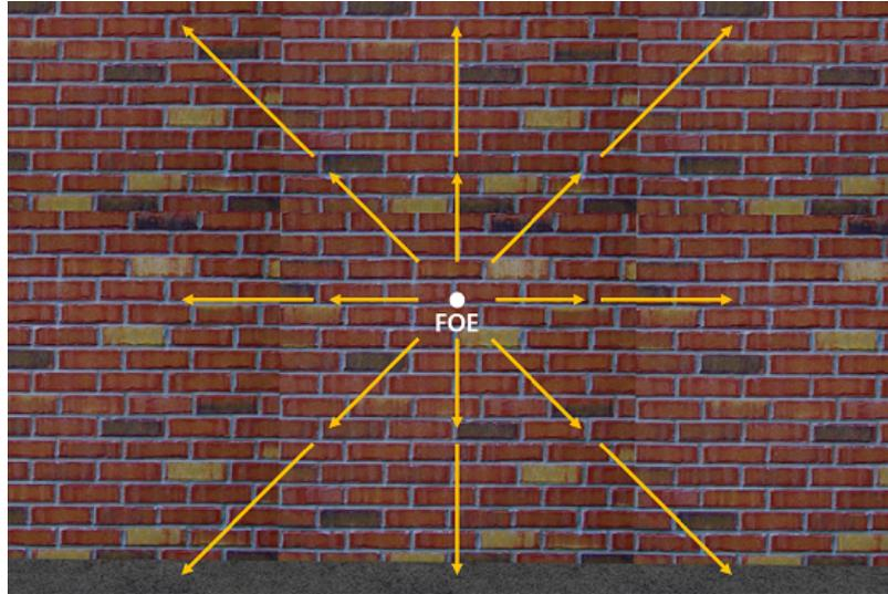
Figure 3.16: An approaching obstacle appears to be expanding in the field of view, hence the optical flow produced by it will ideally have vectors pointing away from the FOE. Image from [15].
