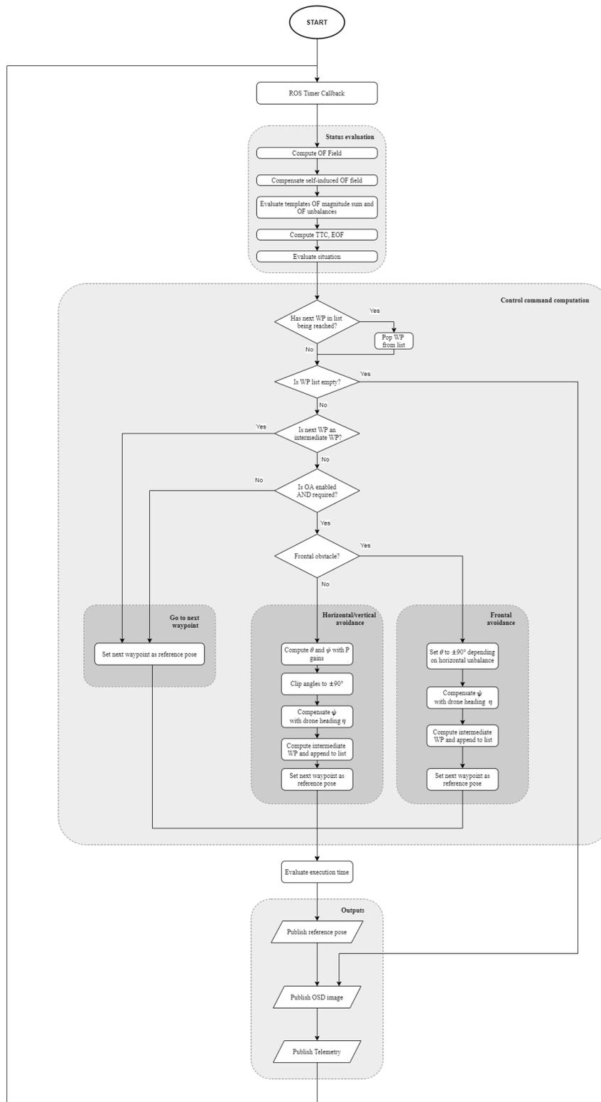
Figure 4.6: Flowchart representing OFOA algorithm Python function, called at a fixed rate in order to solve the obstacle avoidance problem in real-time.
