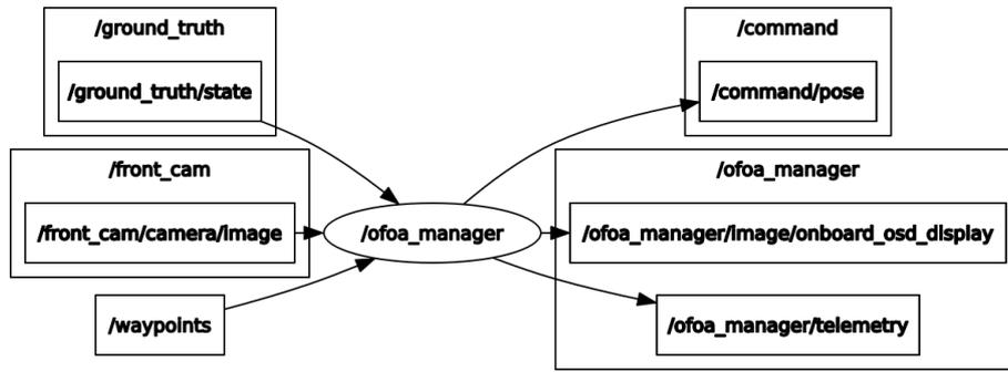
Figure 4.4: Graph of inputs and outputs for node */ofoa\_manager*.
