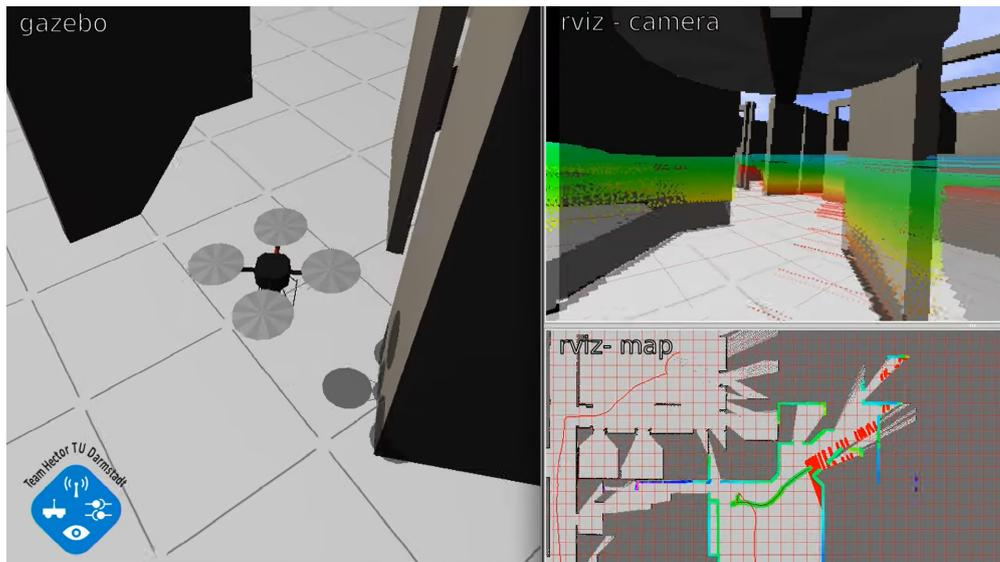
Figure 3.21: In this frame from [43], a demo of *hector\_quadrotor* carrying out an indoor mapping session through a laser scanner is shown. The quadrotor mounts a camera onboard, which view can be seen in the upper-right part of the image. In lower-right part the view from Rviz, a tool for visualizing sensors data coming from ROS and Gazebo, is shown.
