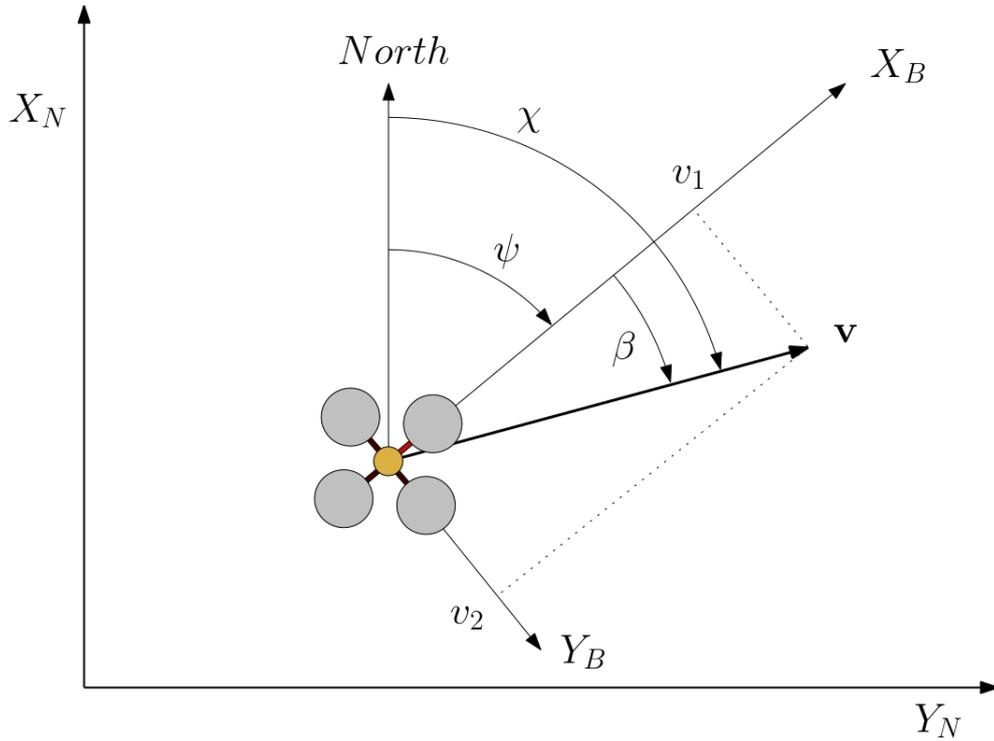
Figure 3.1: In this image different angles are shown. Heading angle  $\psi$  is computed as the clockwise deviation from North. Course angle  $\chi$  refers to actual motion direction (velocity direction  $\mathbf{v}$ ) of the vehicle due to lateral wind perturbation. The angle difference between course and heading is  $\beta$  and is called crab angle or side-slip angle or drift angle.
