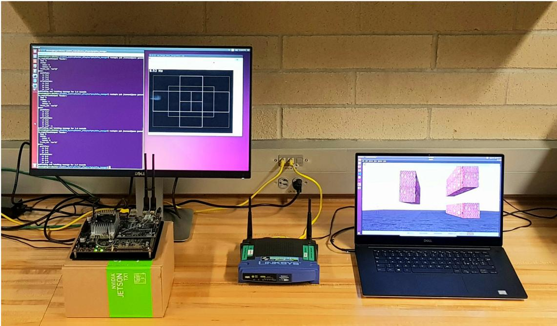
Figure 5.5: Setup for HIL simulation. On the left, the Jetson TX1 Development Kit is connected to a monitor via HDMI cable, running Ubuntu 14.04 and OFOA ROS node. On the right, the laptop with virtualized Ubuntu 18.04 which hosts ROS master node and Gazebo simulator. The Jetson TX1 and the PC are connected by means of the WiFi router acting as a gateway, in the middle.
