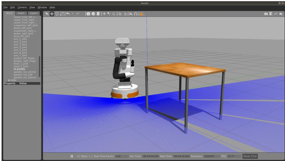
Figure 3.20: A screenshot of Gazebo simulator GUI. Gazebo lets simulate different types of robots in an environment they can interact with. In this case a wheeled robot with a robotic arm mounted on it is shown.
