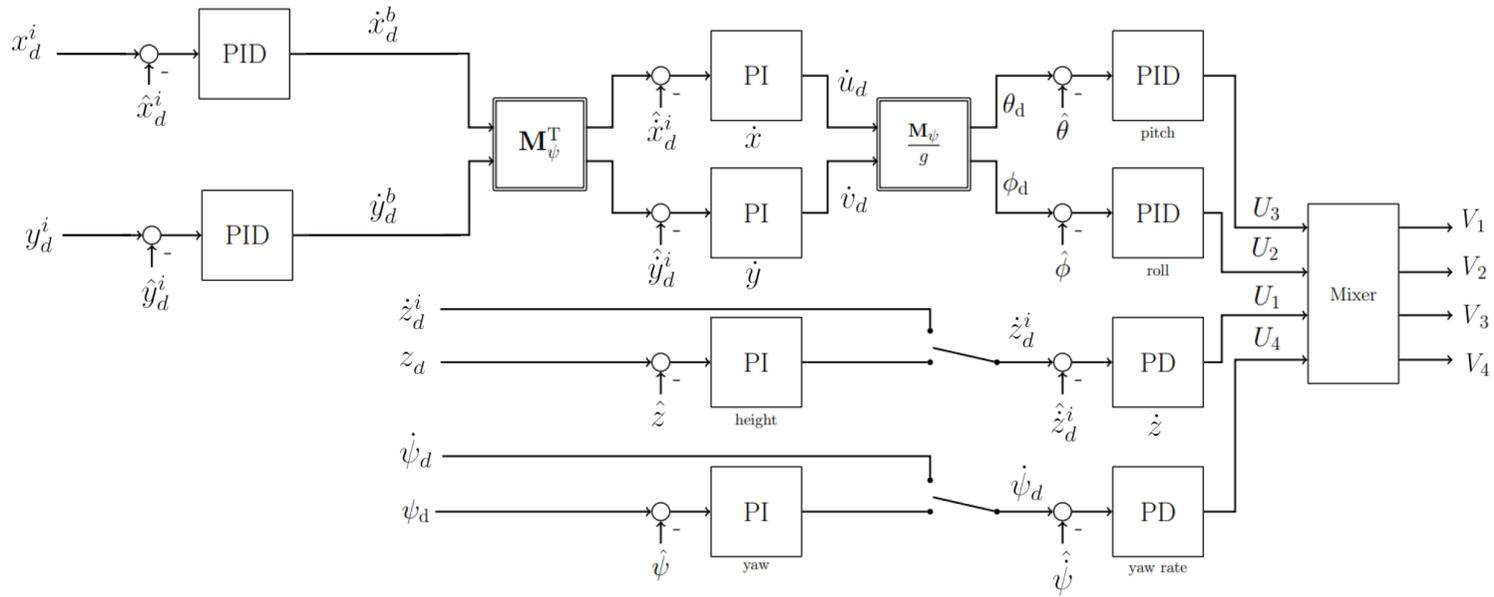
Figure 3.8: Cascaded PID controllers for position control of the quadrotor in the inertial coordinate frame.
