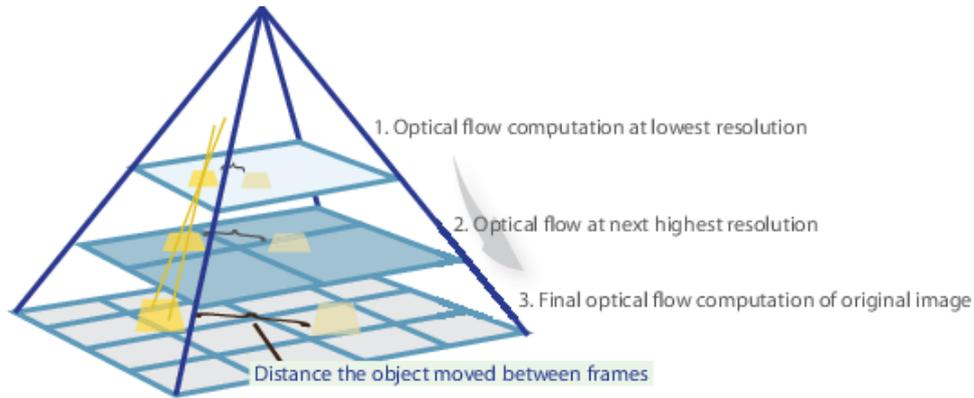
Figure 3.13: Visual representation of pyramid method used to detect larger movement and improve robustness. [34]
