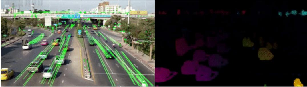
Figure 3.12: Comparison between sparse and dense OF. On the left, OF is computed only for specific features detected by feature-detection algorithm and tracked in following frames by means of OF algorithm. On the right, a dense OF field is shown, where OF is computed for each pixel of the frame and vector information is color-coded: for each pixel, brightness (value in HSV) is the magnitude of the associated motion vector while color (hue in HSV) is vector angle.
