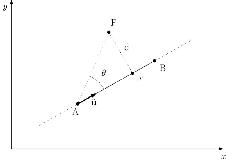
Figure 3.28: Computation of distance of a point from a segment.
