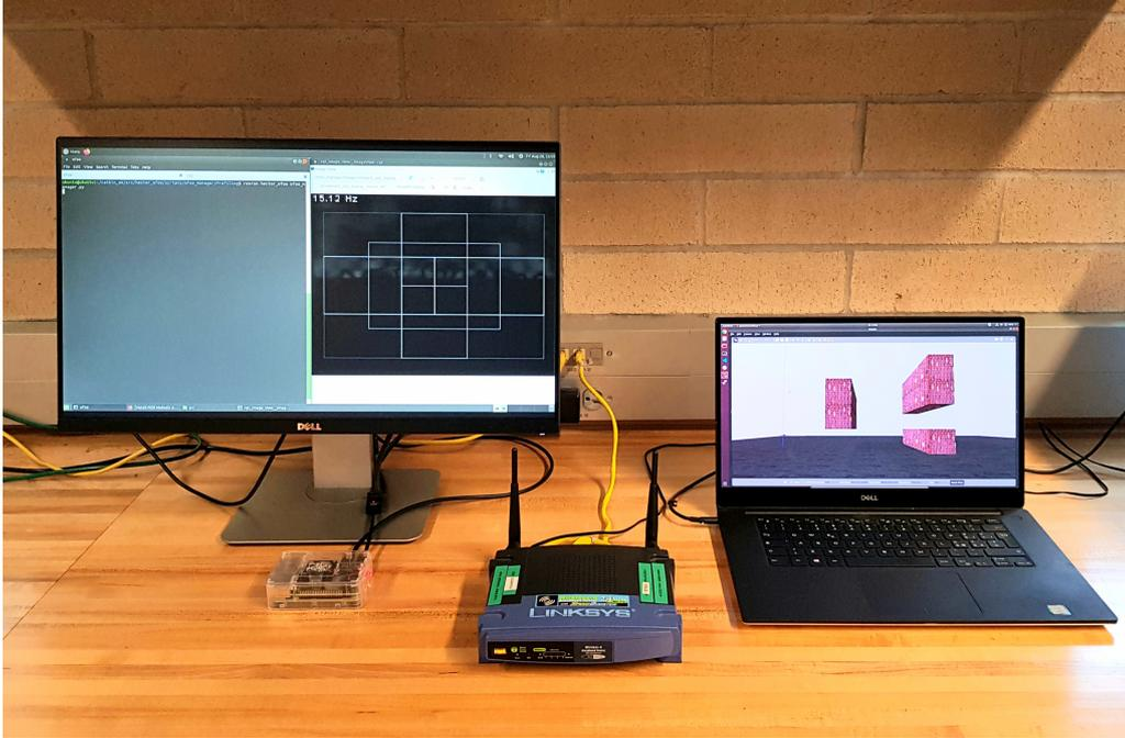
Figure 5.10: Setup for HIL simulation. On the left, the RaspberryPi 4 is connected to a monitor via HDMI cable, running Ubuntu MATE 18.04 and OFOA ROS node. On the right, the laptop with virtualized Ubuntu 18.04 which hosts ROS master node and Gazebo simulator. The RaspberryPi and the PC are connected by means of the WiFi router acting as a gateway, in the middle.
