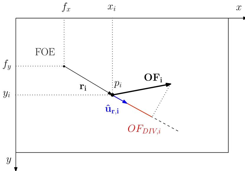
Figure 3.17: Computation of OF divergence component  $OF_{DIV,i}$  for the  $i^{th}$  pixel.
