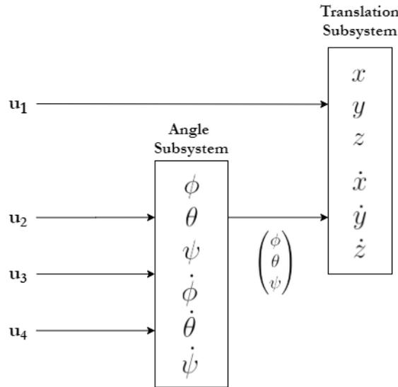
Figure 3.7: Quadrtor's dynamic model decomposition in two subsystems.
