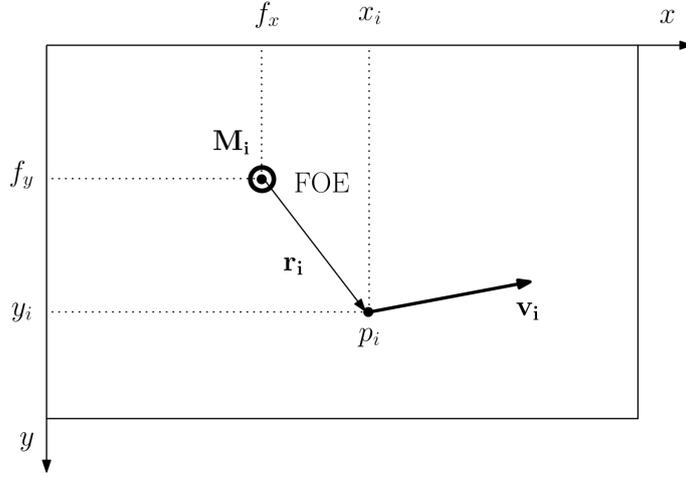
Figure 3.14: Computation of FOE coordinates by minimization of moment  $\mathbf{M}_i$  associated to  $i^{th}$  pixel.
